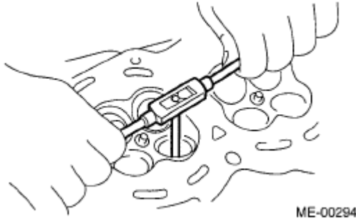
Fig. 170: Reaming Valve Guide Using Valve Guide Reamer 499767400 Courtesy of SUBARU OF AMERICA, INC.
