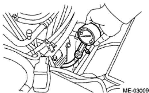
Fig. 7: Checking Engine Compression Using Compression Gauge Courtesy of SUBARU OF AMERICA, INC.
