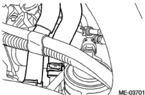
Fig. 30: Identifying Heater Inlet And Outlet Hoses Courtesy of SUBARU OF AMERICA, INC.
