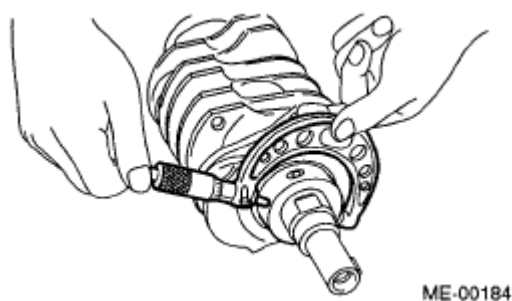
Fig. 237: Checking Crank Journal Courtesy of SUBARU OF AMERICA, INC.
