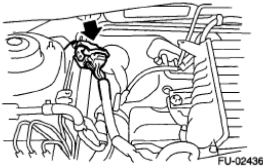
Fig. 24: Locating Harness Connector Courtesy of SUBARU OF AMERICA, INC.
