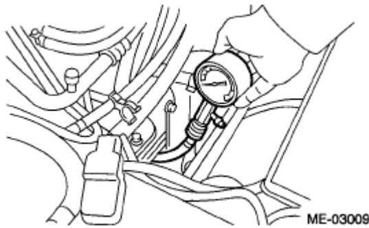
Fig. 7: Measuring Cylinder Compression Courtesy of SUBARU OF AMERICA, INC.
