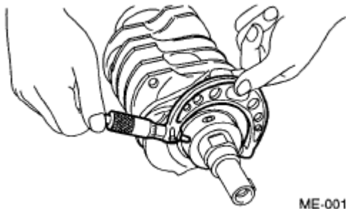
Fig. 207: Inspecting Crank Journal And Crank Pin Courtesy of SUBARU OF AMERICA, INC.
