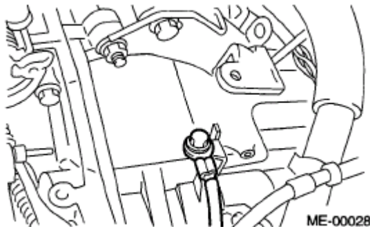
Fig. 25: Identifying Engine Ground Terminal Courtesy of SUBARU OF AMERICA, INC.
