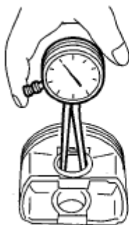
Fig. 248: Checking Clearance Between Piston Pin Hole
