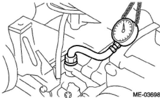
Fig. 14: Measuring Engine Oil Pressure Courtesy of SUBARU OF AMERICA, INC.
