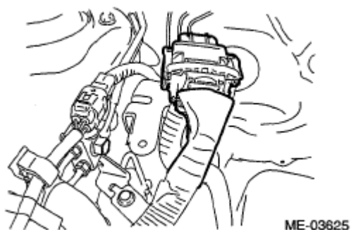
Fig. 30: Identifying Bulkhead Harness Connector And Engine Harness Connector Courtesy of SUBARU OF AMERICA, INC.
