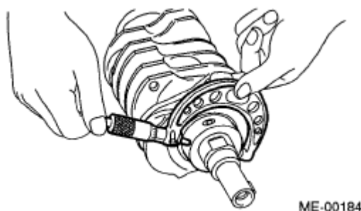
Fig. 260: Measuring Crank Journal And Crank Pin Courtesy of SUBARU OF AMERICA, INC.
