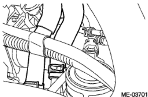
Fig. 36: Identifying Heater Inlet And Outlet Hoses Courtesy of SUBARU OF AMERICA, INC.
