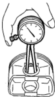
Fig. 235: Measuring Piston Ring Groove Inner Diameter Courtesy of SUBARU OF AMERICA, INC.
