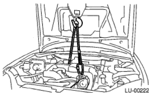
Fig. 50: Identifying Lifting Device And Wire Ropes Courtesy of SUBARU OF AMERICA, INC.
