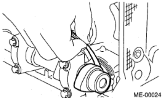
Fig. 20: Measuring Valve Clearances Courtesy of SUBARU OF AMERICA, INC.
