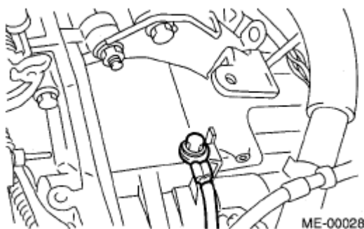
Fig. 25: Identifying Engine Ground Terminal Courtesy of SUBARU OF AMERICA, INC.
