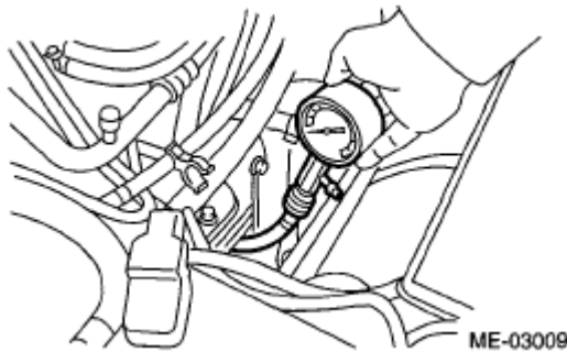
Fig. 7: Screwing Compression Gauge Courtesy of SUBARU OF AMERICA, INC.
