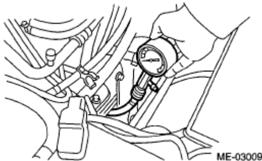
Fig. 8: Installing Compression Gauge To Spark Plug Hole Courtesy of SUBARU OF AMERICA, INC.
