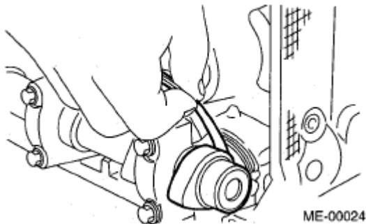
Fig. 23: Measuring Valve Clearances Courtesy of SUBARU OF AMERICA, INC.
