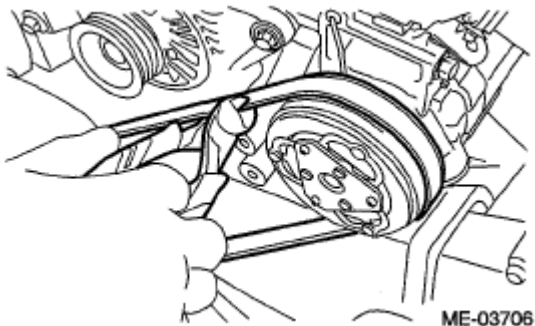
Fig. 61: Cutting Rear Side Belt Courtesy of SUBARU OF AMERICA, INC.
