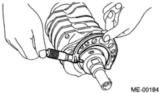
Fig. 232: Inspecting Crank Journal And Crank Pin Courtesy of SUBARU OF AMERICA, INC.
