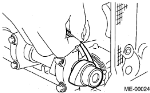
Fig. 22: Measuring Valve Clearances Courtesy of SUBARU OF AMERICA, INC.
