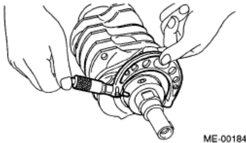
Fig. 214: Inspecting Crank Journal And Crank Pin Courtesy of SUBARU OF AMERICA, INC.
