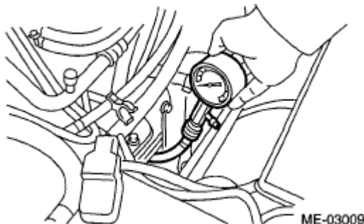
Fig. 7: Holding Compression Gauge Courtesy of SUBARU OF AMERICA, INC.
