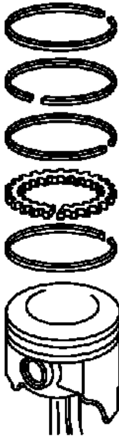
Fig. 352: Exploded View Of Piston Rings Courtesy of GENERAL MOTORS CORP.
