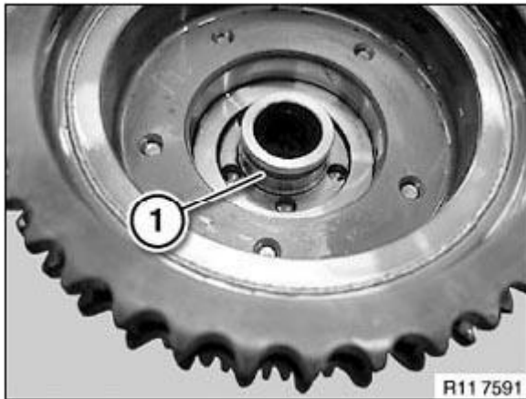
Fig. 339: Identifying VANOS Gear O-Ring Courtesy of BMW OF NORTH AMERICA, INC.
