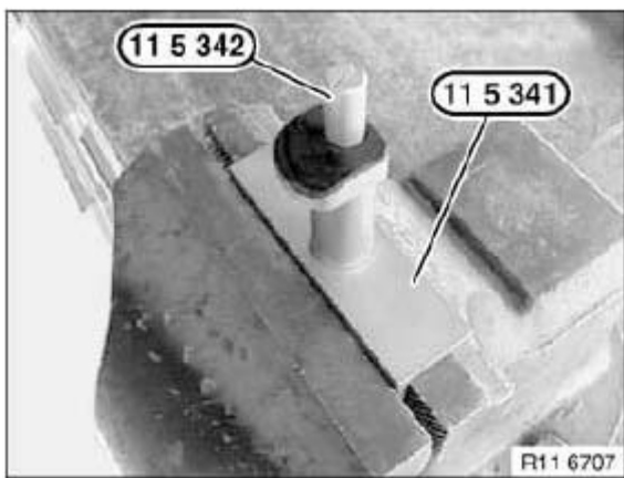
Fig. 159: Identifying Special Tool (11 5 342 And 11 5 341)
