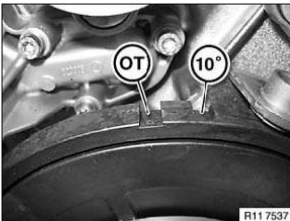
Fig. 347: Identifying Timing Marks Courtesy of BMW OF NORTH AMERICA, INC.
