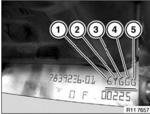
Fig. 126: Identifying Color Allocation In Crankcase Courtesy of BMW OF NORTH AMERICA, INC.
