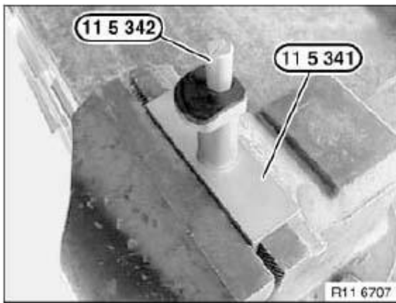
Fig. 148: Identifying Special Tools (11 5 342) And (11 5 341)
