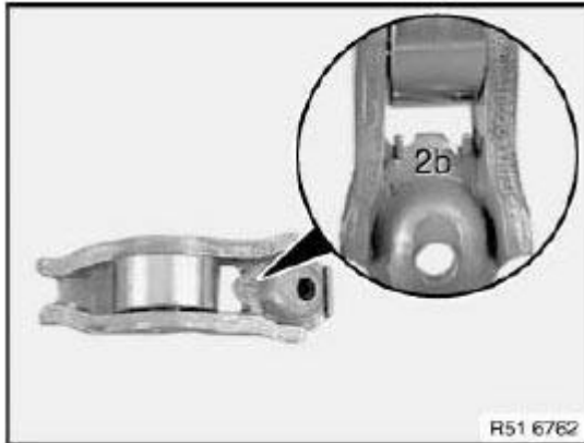
Fig. 537: Identifying Rocker Arms Tolerance Classes Courtesy of BMW OF NORTH AMERICA, INC.
