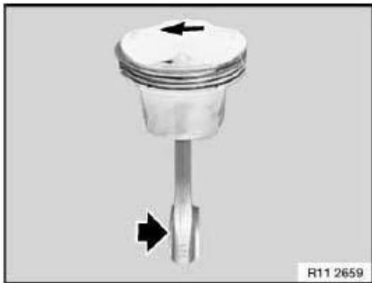
Fig. 217: Installing Piston Pin Courtesy of BMW OF NORTH AMERICA, INC.
