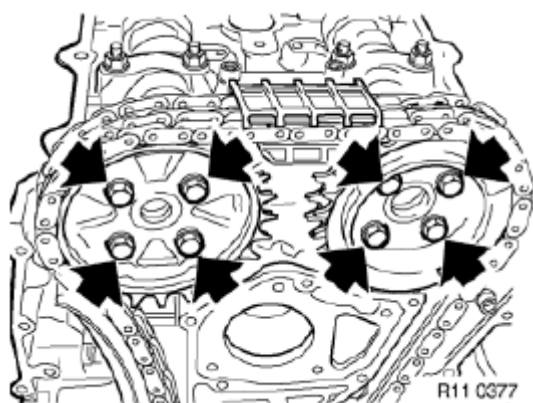
Fig. 231: Locating Chain Wheels Screws Courtesy of BMW OF NORTH AMERICA, INC.
