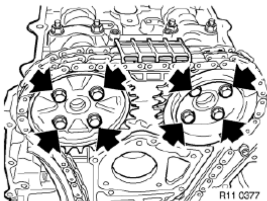
Fig. 209: Locating Chain Wheels Screws
