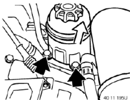
Fig. 12: Locating Oil Tank Bolts For Hydraulic Steering Courtesy of BMW OF NORTH AMERICA, INC.
