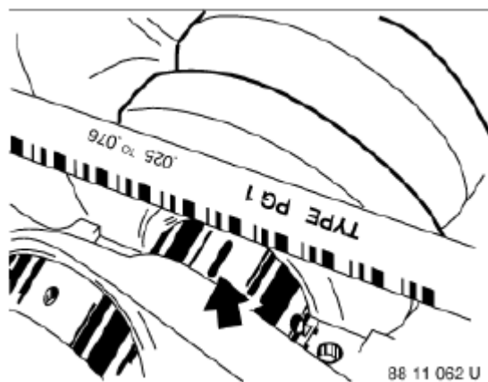
Fig. 147: Checking Bearing Clearance Courtesy of BMW OF NORTH AMERICA, INC.
