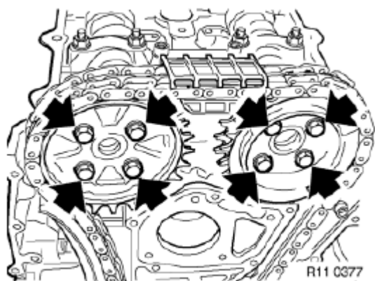
Fig. 47: Locating Chain Wheel Bolts
