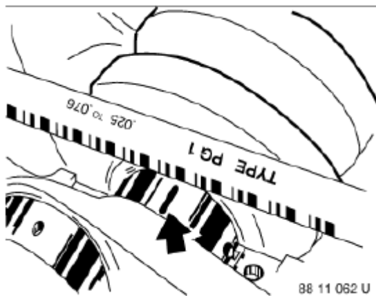
Fig. 126: Identifying Plastic Thread (Plastigage) On Crankshaft Courtesy of BMW OF NORTH AMERICA, INC.
