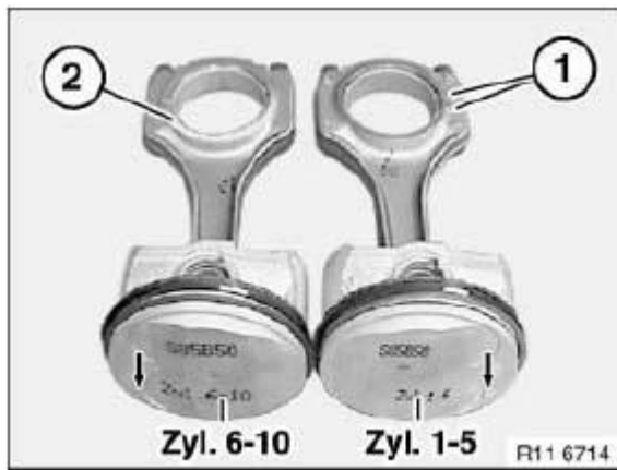
Fig. 156: Identifying Connecting Rod Elevation - Cylinders 6-10 And 1-5 (2 Of 2) Courtesy of BMW OF NORTH AMERICA, INC.
