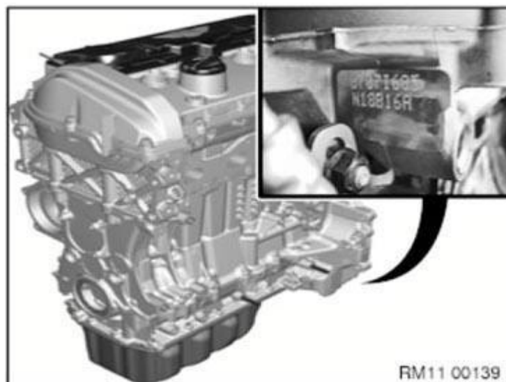
Fig. 16: Identifying Engine Identification Numbers Location - N12/N14/N16/N18 Courtesy of BMW OF NORTH AMERICA, INC.
