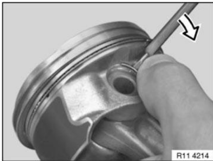
Fig. 162: Installing Retaining Ring Courtesy of BMW OF NORTH AMERICA, INC.
