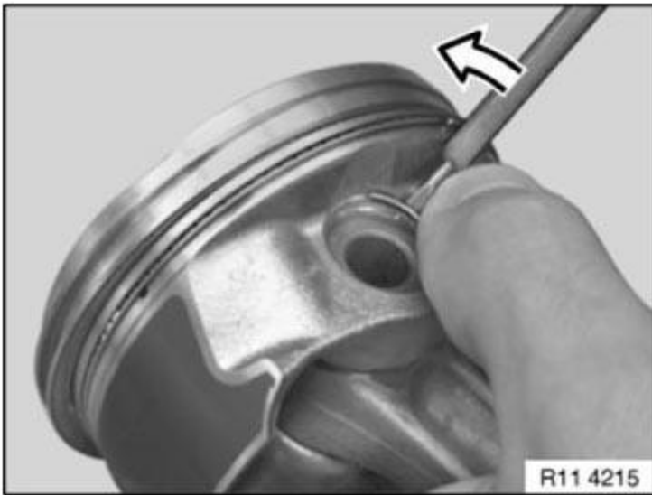
Fig. 156: Removing Retaining Ring From Piston Courtesy of BMW OF NORTH AMERICA, INC.
