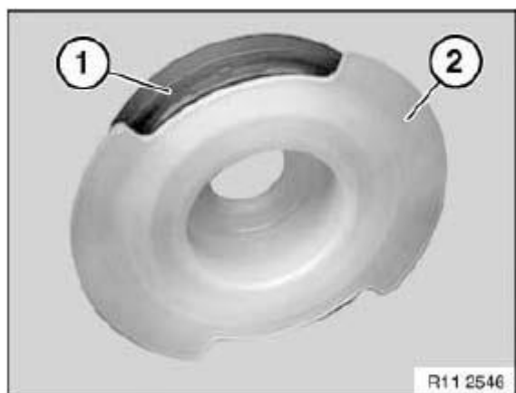
Fig. 122: Identifying Support Sleeve
