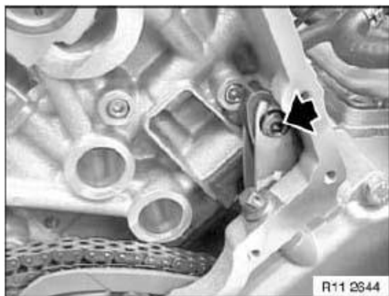
Fig. 84: Identifying Guide Rail Screw
