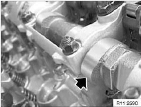
Fig. 239: Locating Inlet Camshaft Position
