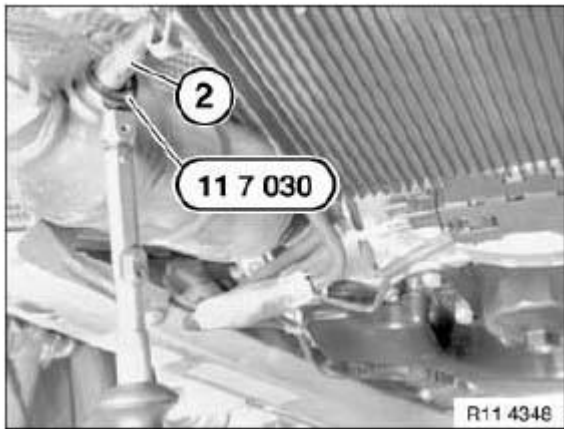
Fig. 616: Identifying Special Tool (11 7 030) On Monitor Sensor Courtesy of BMW OF NORTH AMERICA, INC.
