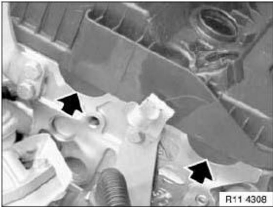
Fig. 41: Locating Gasket Seated Position
