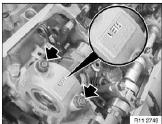
Fig. 373: Locating Camshaft Bearing Caps Of Cylinders Courtesy of BMW OF NORTH AMERICA, INC.
