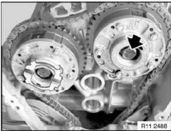
Fig. 459: Identifying Exhaust Adjustment Unit Screw Courtesy of BMW OF NORTH AMERICA, INC.
