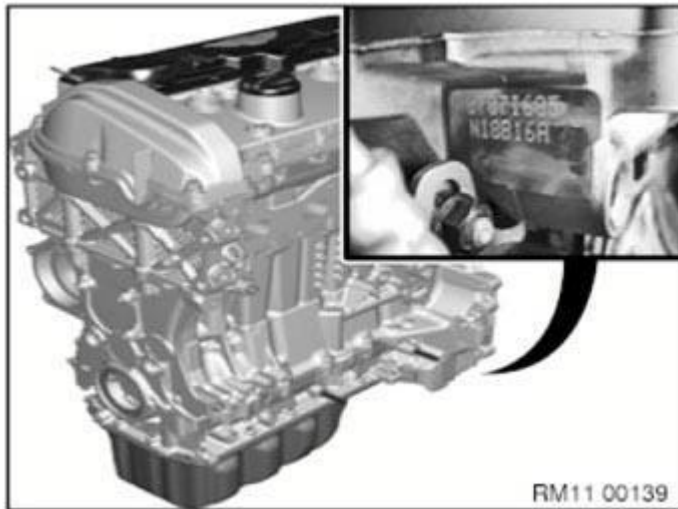
Fig. 16: Identifying Engine Identification Mark - N12/N14/N16/N18 Courtesy of BMW OF NORTH AMERICA, INC.
