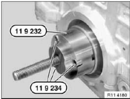
Fig. 113: Inserting Special Tool (11 9 232) With Screws Into Crankshaft Courtesy of BMW OF NORTH AMERICA, INC.
