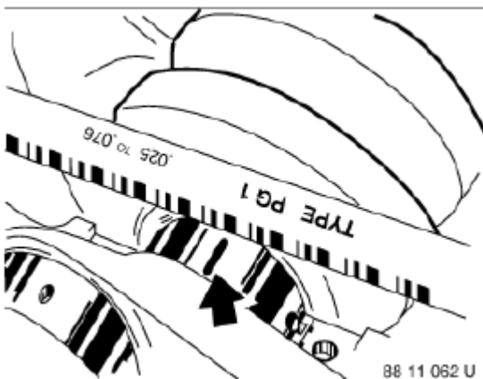
Fig. 141: Reading Off Bearing Play At Width Of Flattened Plastic Courtesy of BMW OF NORTH AMERICA, INC.
