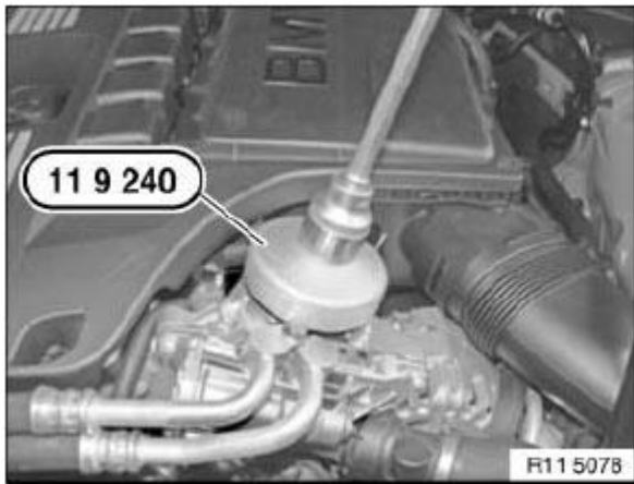
Fig. 345: Identifying Special Tool 11 9 240 Courtesy of BMW OF NORTH AMERICA, INC.
