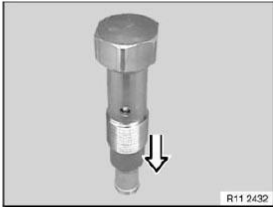
Fig. 290: Compressing Chain Tensioner Courtesy of BMW OF NORTH AMERICA, INC.
