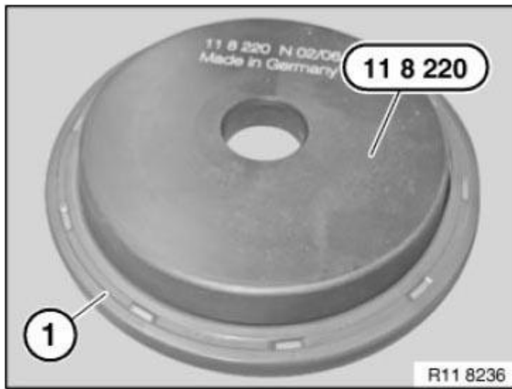
Fig. 112: Identifying Radial Shaft Seal On Special Tool 11 8 220 Courtesy of BMW OF NORTH AMERICA, INC.
