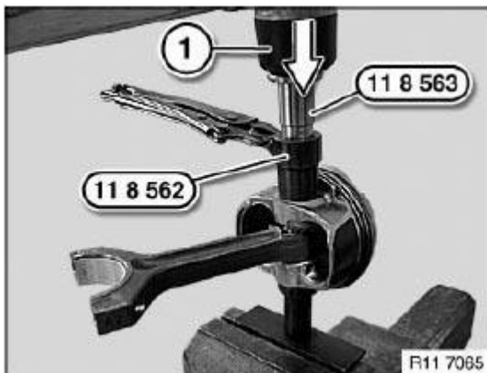
Fig. 207: Installing Piston Pin Circlip Courtesy of BMW OF NORTH AMERICA, INC.
