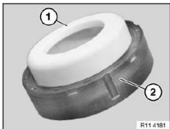
Fig. 63: Identifying Support Sleeve With Radial Seal Courtesy of BMW OF NORTH AMERICA, INC.
