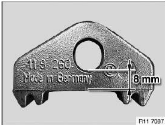
Fig. 138: Identifying Enlarge Dimension Of Slot On Special Tool 11 9 260 Courtesy of BMW OF NORTH AMERICA, INC.
