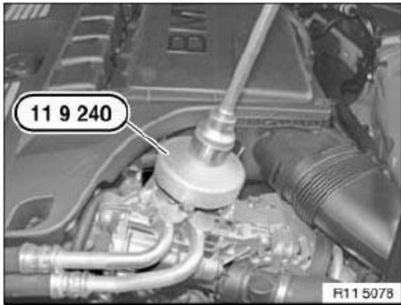
Fig. 350: Releasing Oil Filter Cap Using Special Tool 11 9 240 Courtesy of BMW OF NORTH AMERICA, INC.
