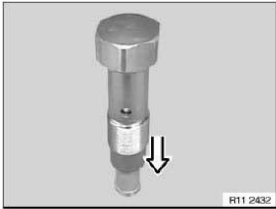
Fig. 201: Identifying Chain Tensioner
