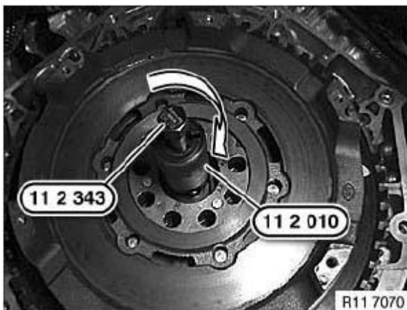
Fig. 121: Identifying Special Tool (11 2 010) And (11 2 343) Courtesy of BMW OF NORTH AMERICA, INC.
