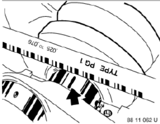
Fig. 156: Reading Bearing Play At Width Of Flattened Plastic Thread And Measurement Scale Courtesy of BMW OF NORTH AMERICA, INC.
