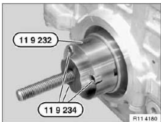
Fig. 101: Mounting Special Tool 11 9 232 With Screws To Crankshaft Courtesy of BMW OF NORTH AMERICA, INC.
