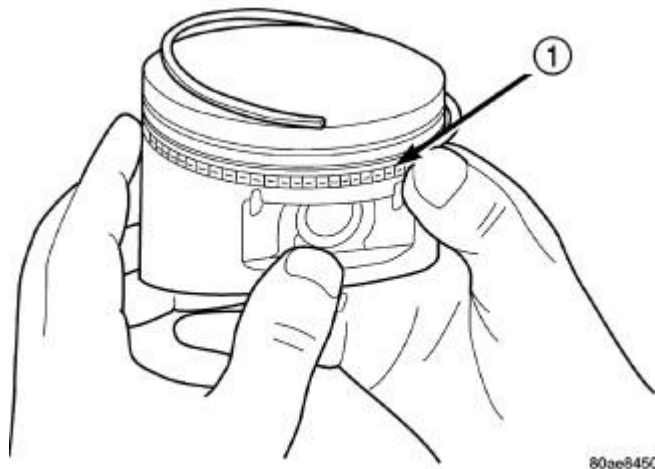
Fig. 409: Removing/Installing Piston Ring Side Rail Courtesy of CHRYSLER GROUP, LLC
