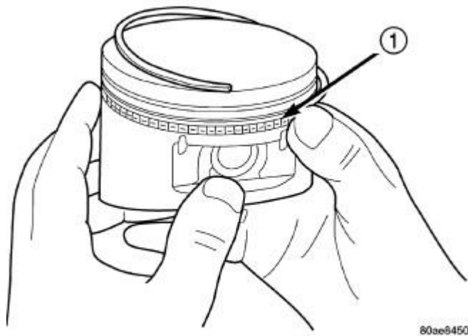
Fig. 138: Removing/Installing Piston Ring Side Rail Courtesy of CHRYSLER GROUP, LLC
