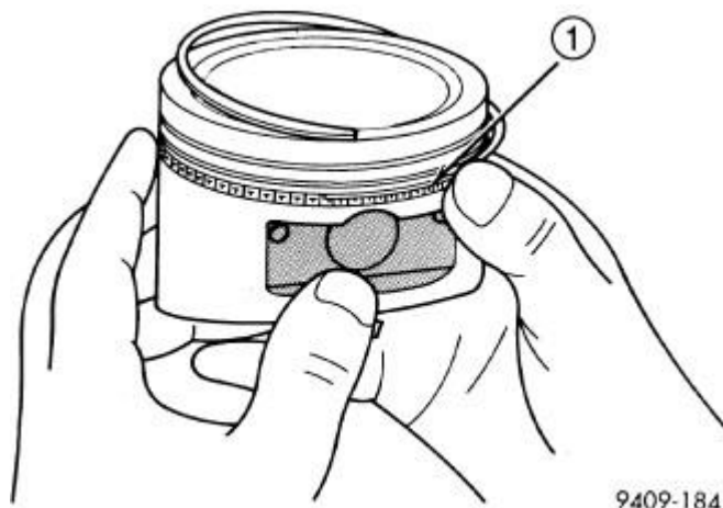
Fig. 156: Installing Side Rail Courtesy of CHRYSLER LLC
