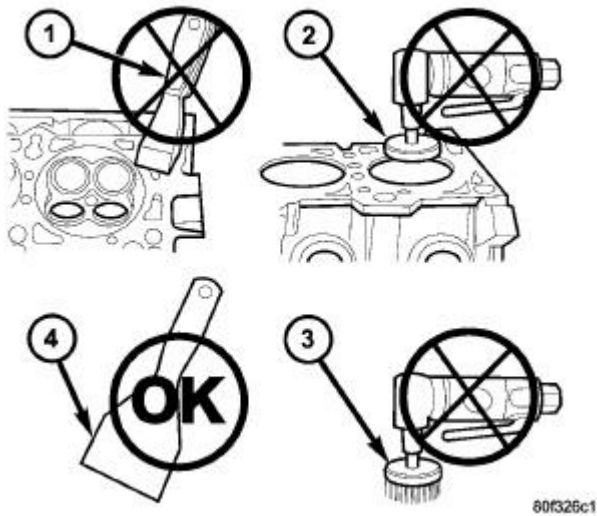
Fig. 1: Proper Tool Usage For Surface Preparation
