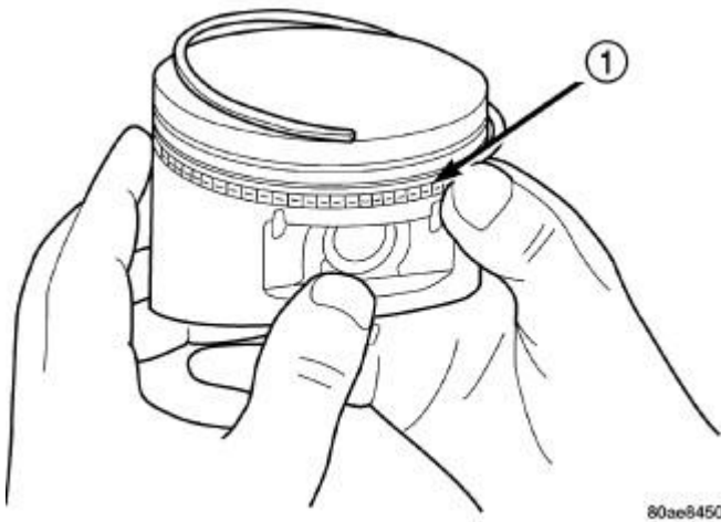
Fig. 244: Installing Piston Ring Side Rail Courtesy of CHRYSLER GROUP, LLC
