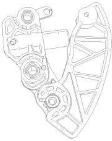
Fig. 458: Timing Chain Tensioner Arm Courtesy of CHRYSLER GROUP, LLC
