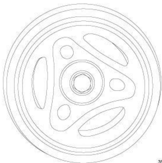
Fig. 213: Crankshaft Damper & Harden Steel Bolt Courtesy of CHRYSLER GROUP, LLC
