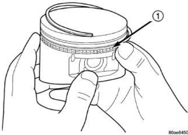
Fig. 167: SIDE RAIL - INSTALLATION Courtesy of CHRYSLER LLC
