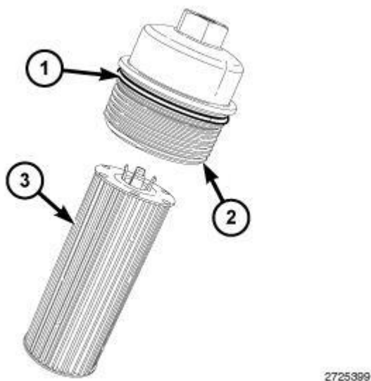
Fig. 551: O-Ring Seal, Oil Filter Cap & Oil Filter
