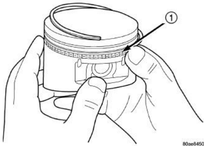
Fig. 438: Removing/Installing Piston Ring Side Rail Courtesy of CHRYSLER GROUP, LLC
