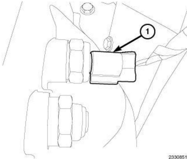
**Fig. 61: Reverse Lamp Switch Harness Connector**
