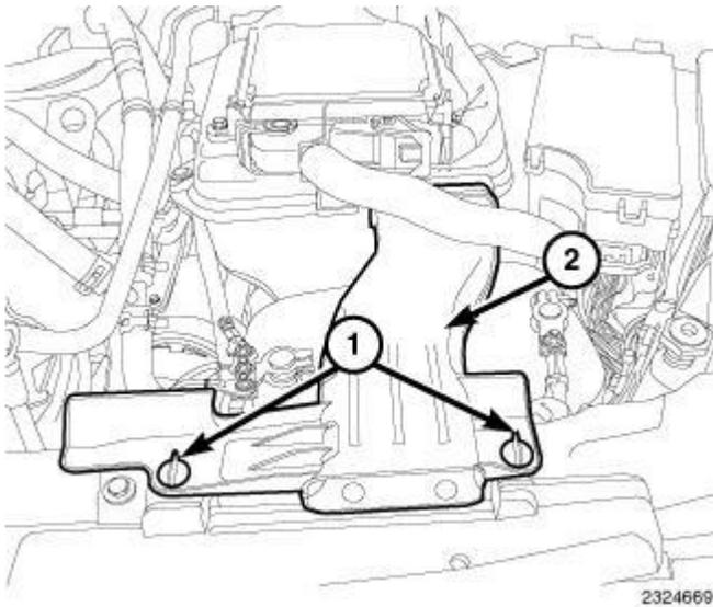
**Fig. 448: Quarter Turn Lock Tabs & Air Inlet Duct**
