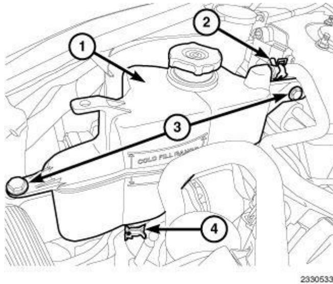
**Fig. 129: Coolant Recovery Reservoir, Clamps & Bolts**
