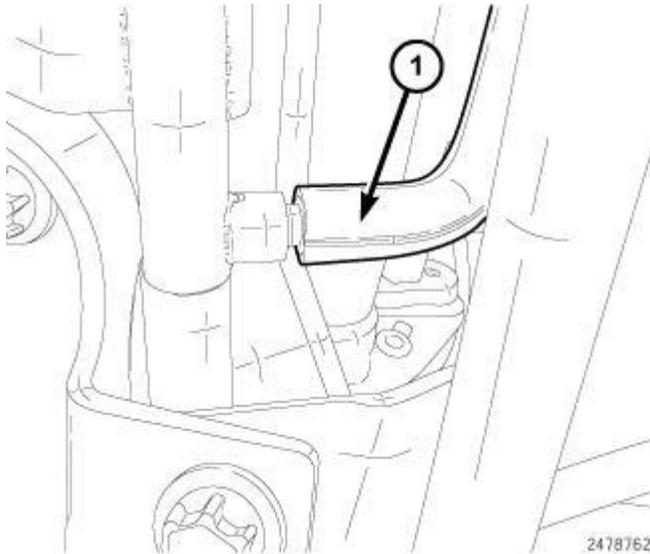
**Fig. 472: Vacuum Supply Line At EGR Solenoid**
