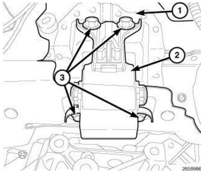
**Fig. 283: Left Side Engine Mount & Bolts**
