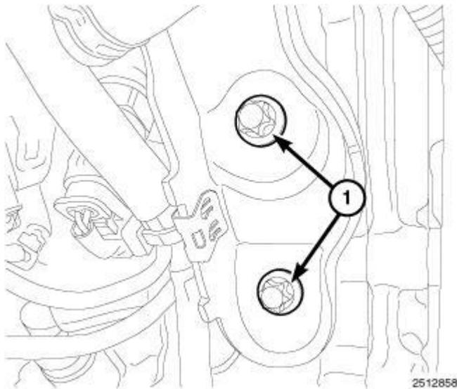
**Fig. 642: EGR Support Bracket Bolts**
