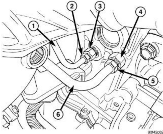
**Fig. 594: Oil Supply Line - Engine Block Fitting**
