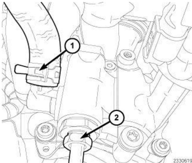
**Fig. 221: Power Steering Supply Line & Feed Line**
