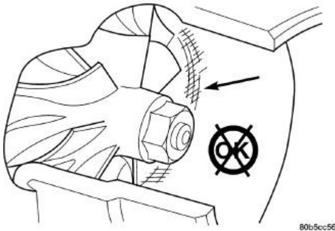
**Fig. 613: Inspect Compressor Housing For Impeller Rubbing Condition**
