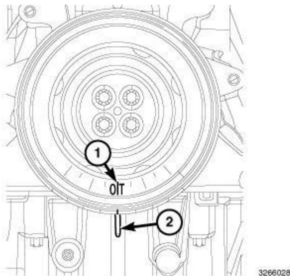
**Fig. 140: Crankshaft Alignment Timing Marks**
