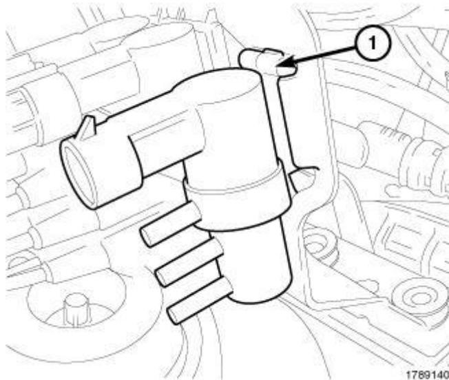
**Fig. 598: Solenoid Mounting Bracket**
