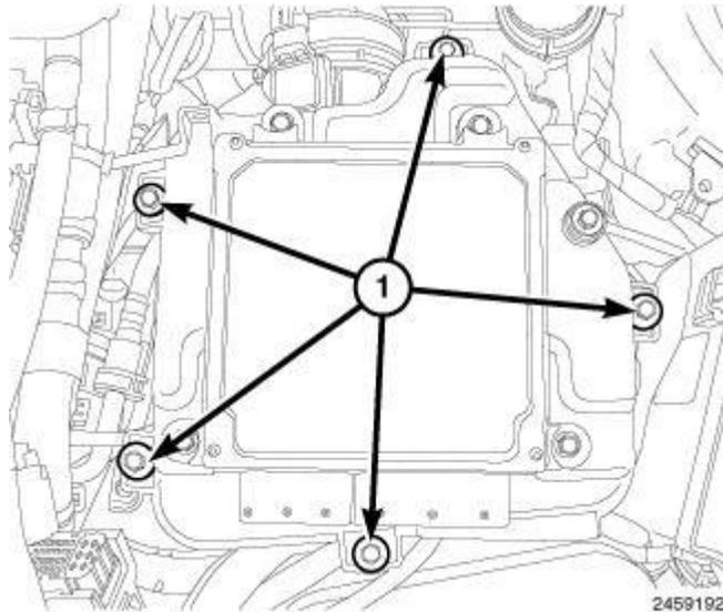
**Fig. 94: Air Cleaner Cover Screws**
