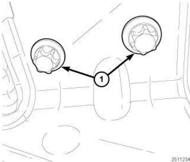
**Fig. 707: CAC Tube And Bracket Assembly Bolts**
