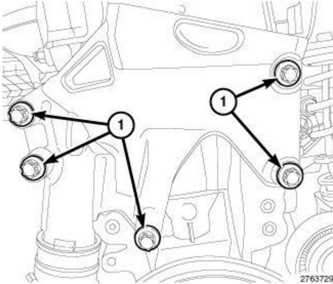
**Fig. 296: Engine Mount Carrier Bracket & Bolts**
