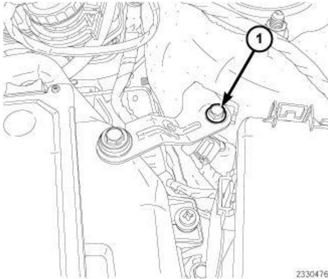
**Fig. 84: Air Cleaner Upper Support Bracket Retaining Bolt**
