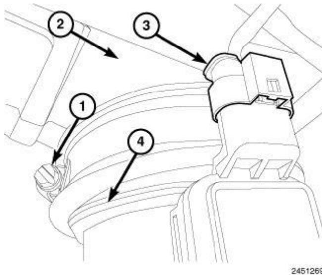
**Fig. 109: Mass Air Flow Sensor, Harness Connector, Turbocharger Inlet Tube & Clamp**
