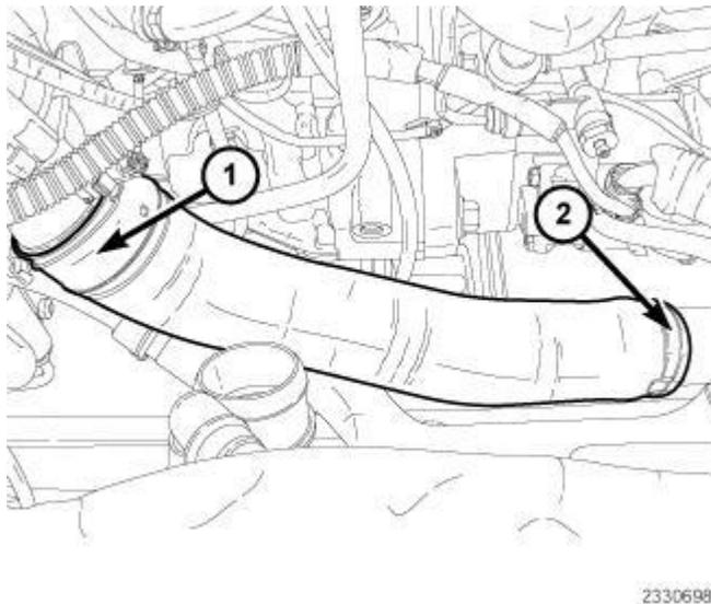
**Fig. 19: EGR Air Flow Control Valve & Clamp**
