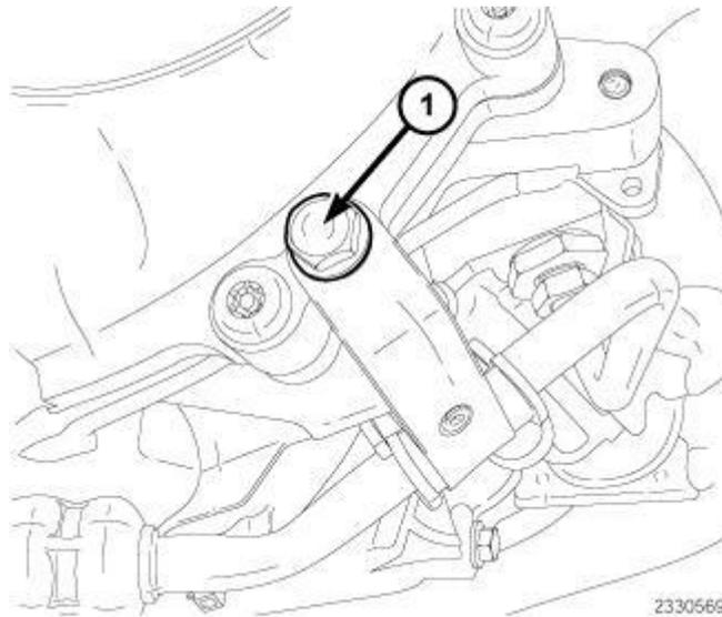
**Fig. 40: Power Steering Line Support Bracket Retaining Bolt**
