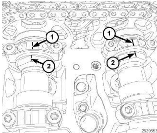
**Fig. 695: Ensuring Camshaft Mark Is Aligned With Bearing Cap Mark**
