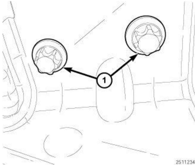
**Fig. 690: CAC Tube And Bracket Assembly Bolts**
