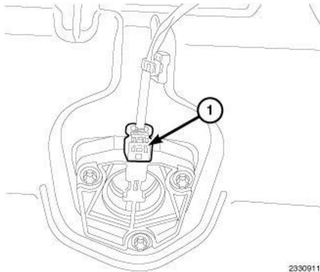
**Fig. 56: Oil Level Switch Wire Harness Connector**
