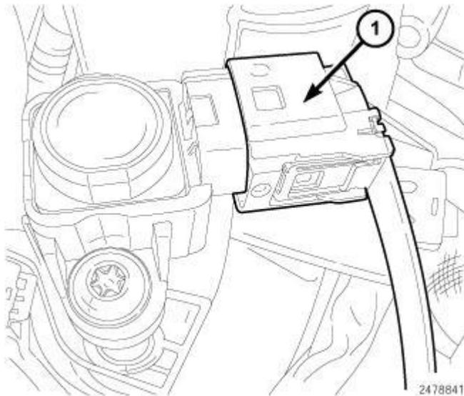
**Fig. 483: Boost Pressure Sensor Harness Connector**
