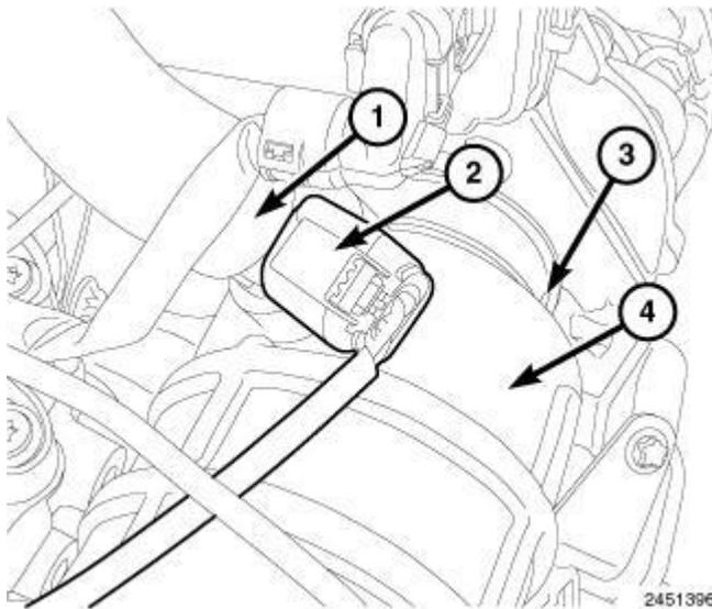
**Fig. 107: CCV Hose, Heater Harness Connector, Turbocharger Inlet Tube & Clamp**
