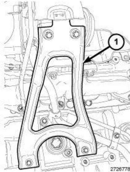
**Fig. 608: Turbocharger Bracket**
