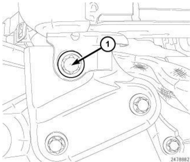
**Fig. 489: Lower EGR Cooler Bolt**
