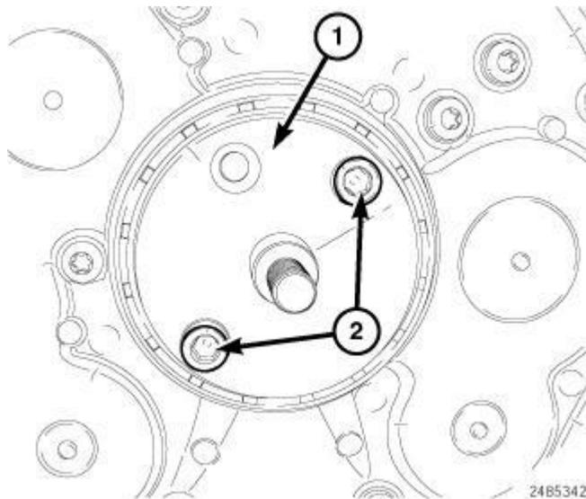
**Fig. 267: Rear Main Seal Ring Adaptor & Bolts**
