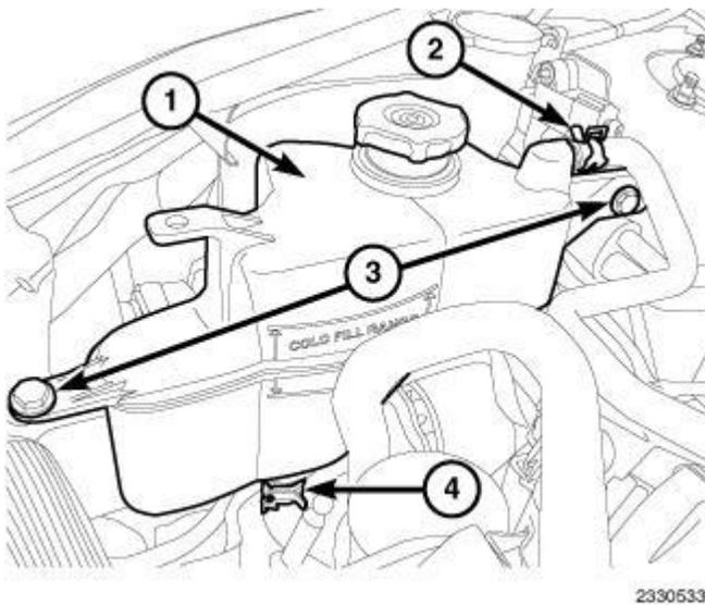
**Fig. 21: Coolant Recovery Reservoir, Clamps & Bolts**
