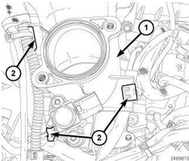
**Fig. 551: Mixing Chamber & Wire Harness Retainer Clips**
