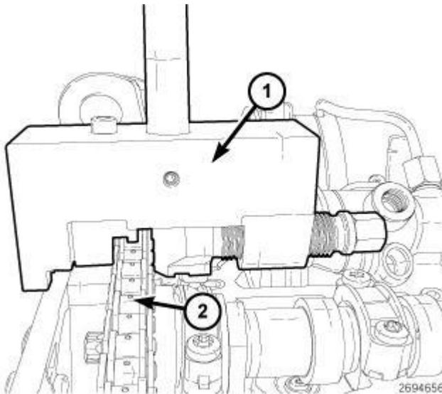
**Fig. 626: Installing Rivet Press Tool Onto Timing Chain**
