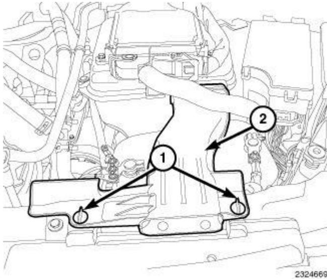
**Fig. 258: Quarter Turn Lock Tabs & Air Inlet Duct**
