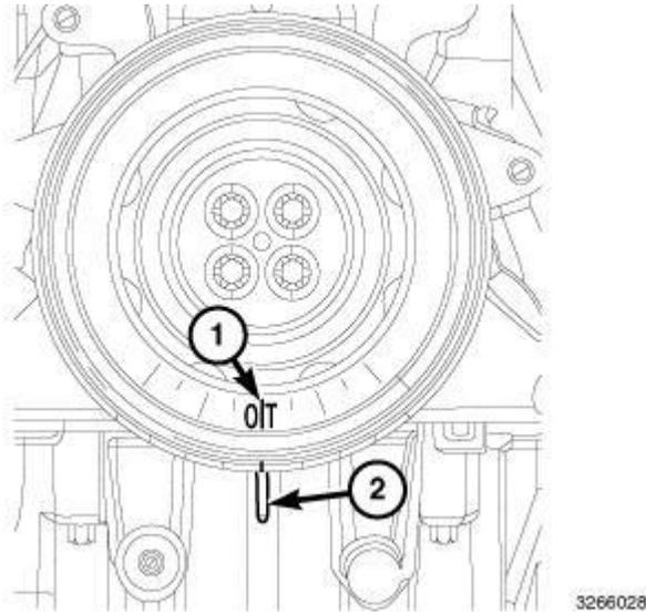
**Fig. 694: Crankshaft Alignment Timing Marks**
