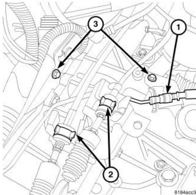
**Fig. 30: Hydraulic Line & Shift Cables**
