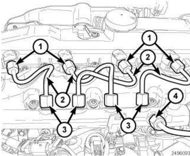
**Fig. 170: Identifying Fuel Injectors, High Pressure Fuel Tubes, Fuel Rail & High Pressure Feed Line**
