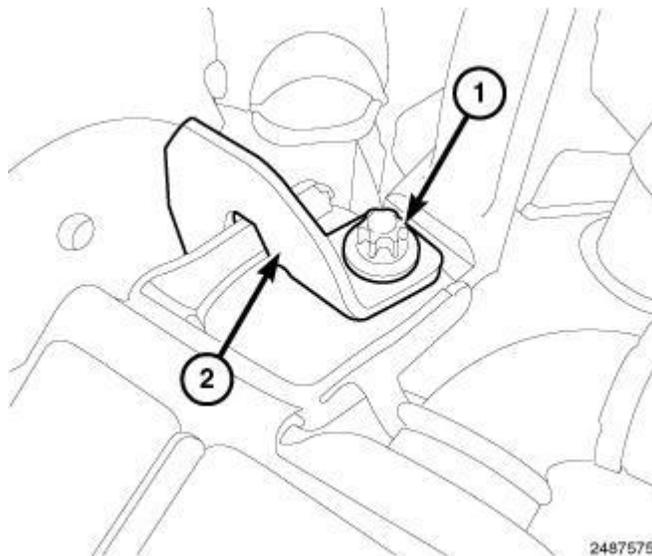
**Fig. 425: Upper EGR Cooler Bolt & Bracket**
