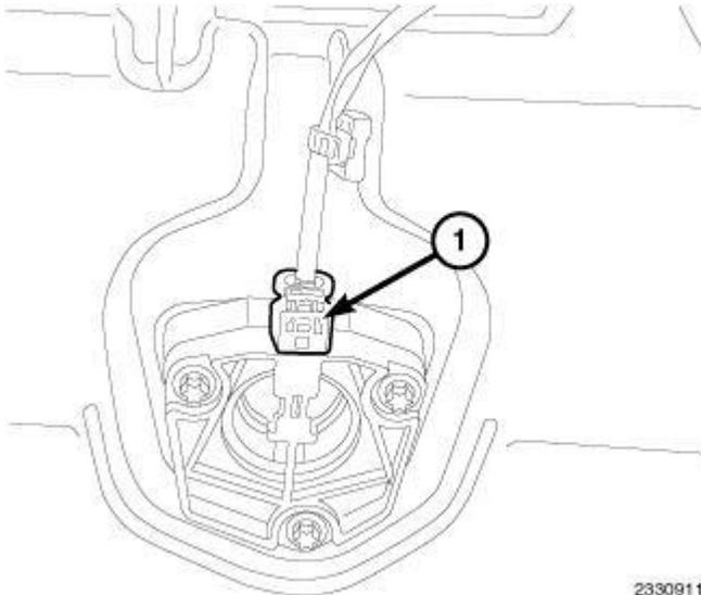
**Fig. 387: Oil Level Switch Wire Harness Connector**
