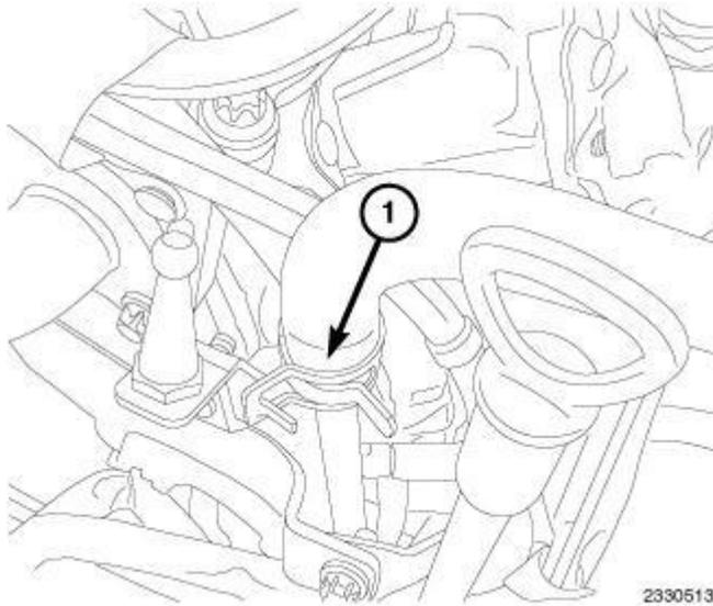
**Fig. 18: Brake Booster Vacuum Hose**
