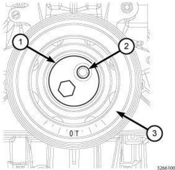
**Fig. 218: Vibration Damper Holder Tool, Vibration Damper & Bolts**
