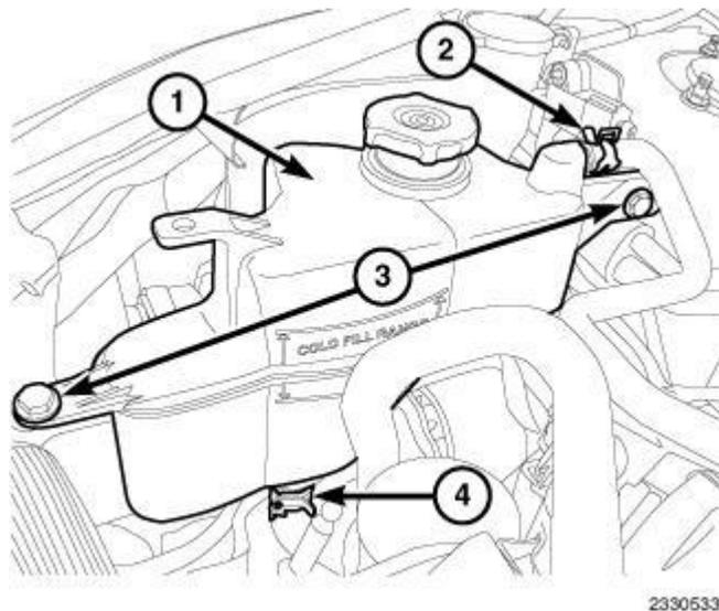
**Fig. 12: Coolant Recovery Reservoir, Clamps & Bolts**
