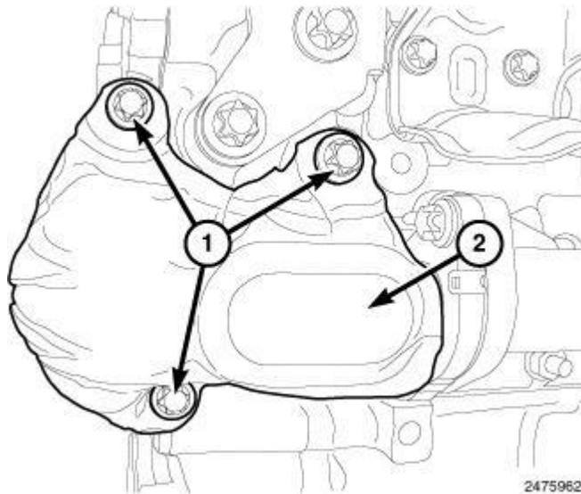
**Fig. 634: EGR Pipe Heat Shield & Bolts**
