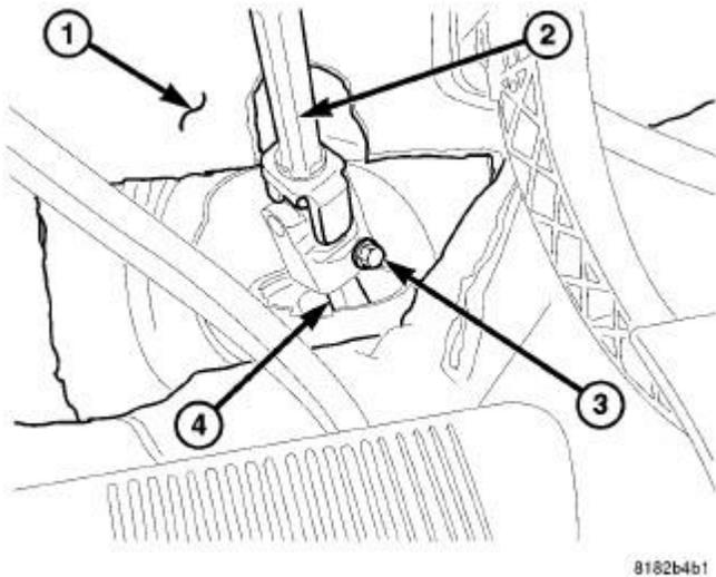
**Fig. 13: Lower Coupling Bolt**
