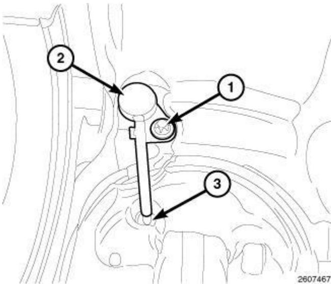
**Fig. 343: Removing & Installing Oil Jets**
