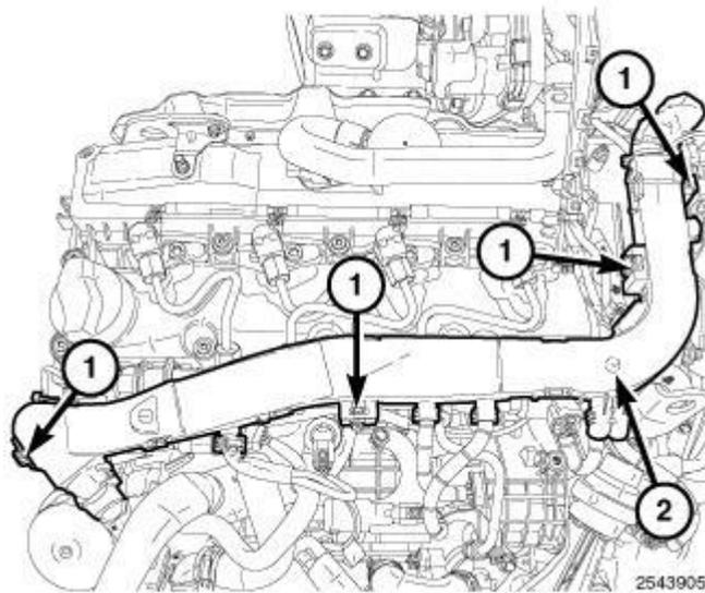
**Fig. 182: Lock Tabs & Engine Wire Harness**
