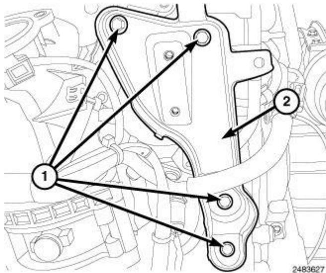
**Fig. 371: Identifying Bolts & EGR Support Bracket**
