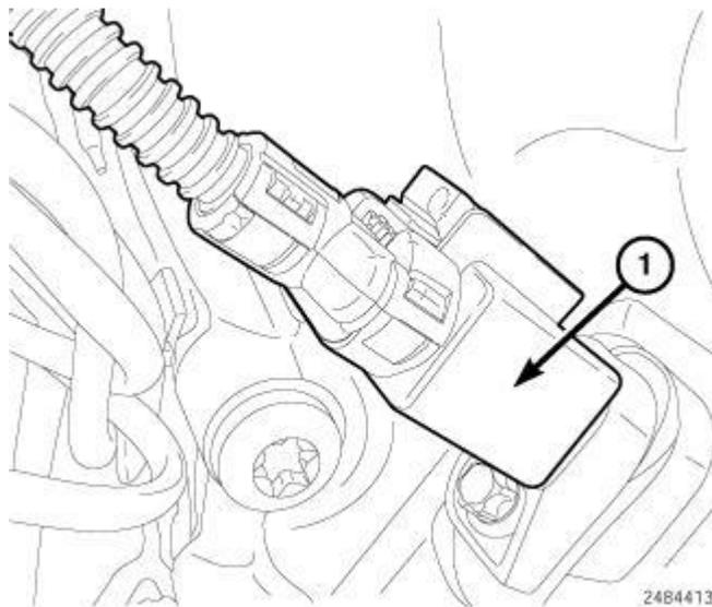
**Fig. 471: Crankshaft Position Sensor Harness Connector**
