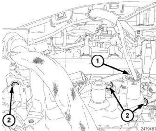
**Fig. 334: Coolant Temp Sensor & Cooling Manifold Bolts**
