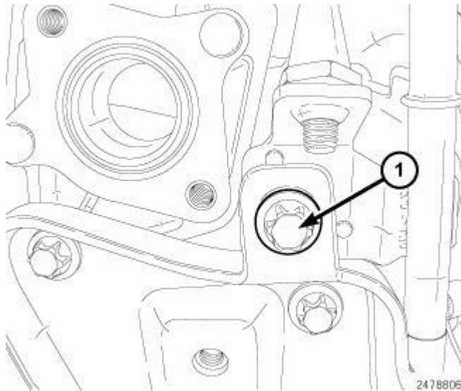
**Fig. 638: Vacuum Tube Bolt**
