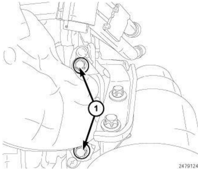
**Fig. 544: Identifying EGR Cooler Manifold Bolts**
