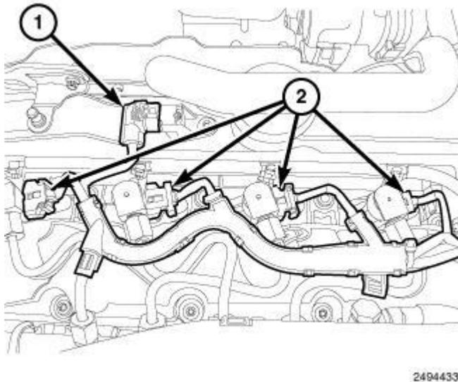
**Fig. 163: Identifying Camshaft Position Sensor (CMP) Harness Connector & Fuel Injector Harness Connectors**
