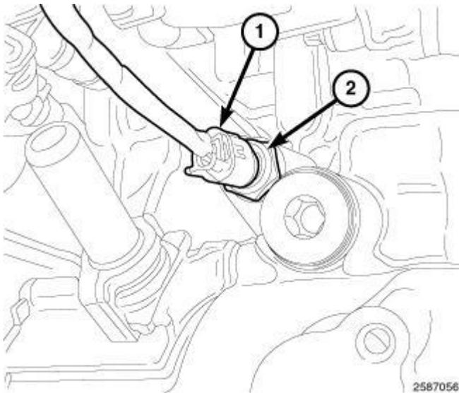
**Fig. 375: Oil Temperature Sensor Harness Connector & Sensor**
