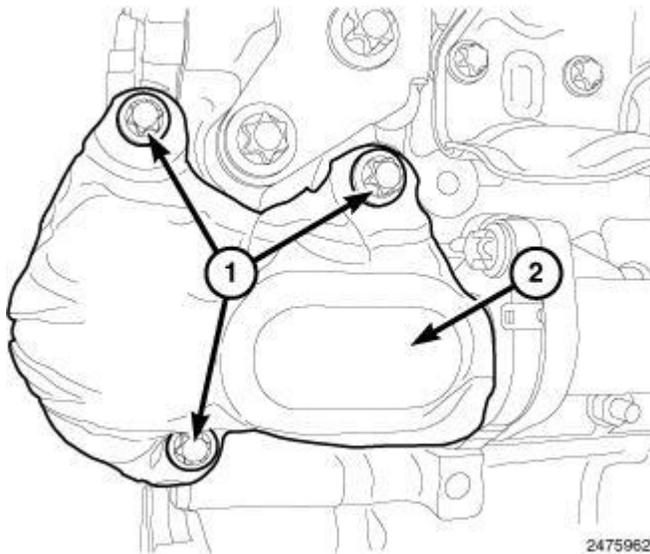
**Fig. 664: EGR Pipe Heat Shield & Bolts**
