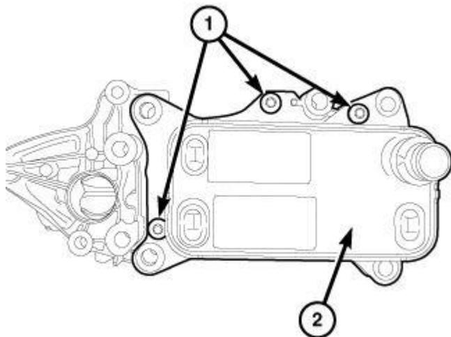
**Fig. 309: Oil Cooler & Bolts**
