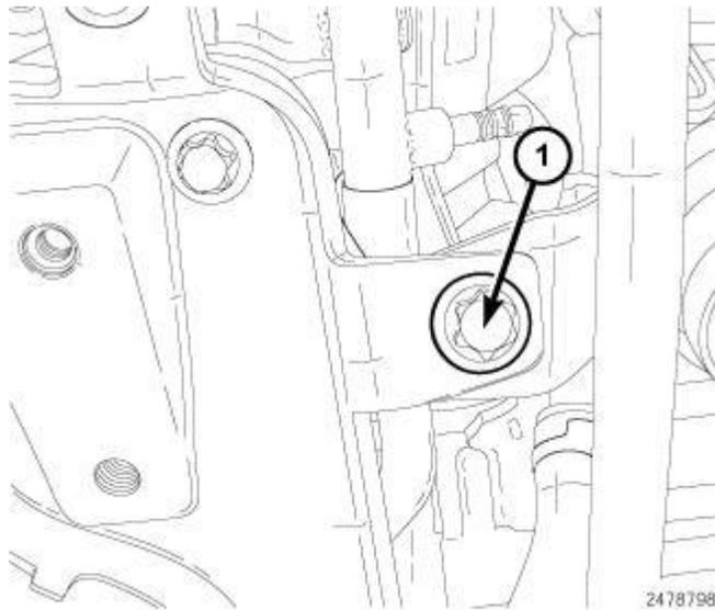
**Fig. 637: Oil Dip Stick Bolt**
