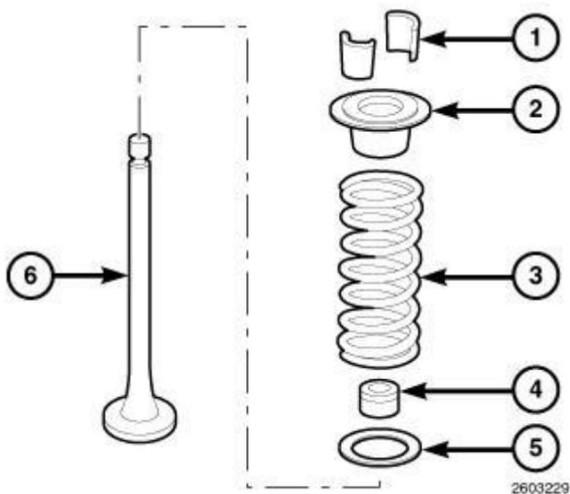
**Fig. 204: Valve Spring, Keeper, Retainer, Spring Seat, Valve Stem Seals & Valve**
