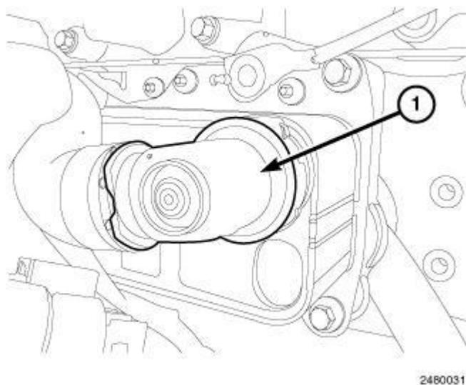
**Fig. 505: Identifying Coolant Hose**
