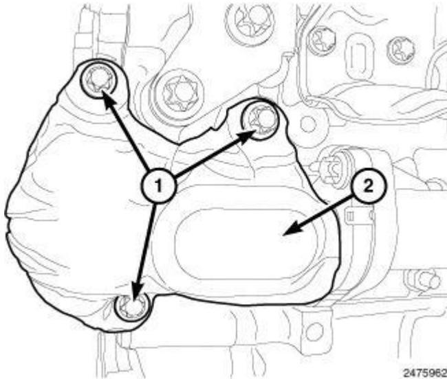
**Fig. 447: EGR Pipe Heat Shield & Bolts**
