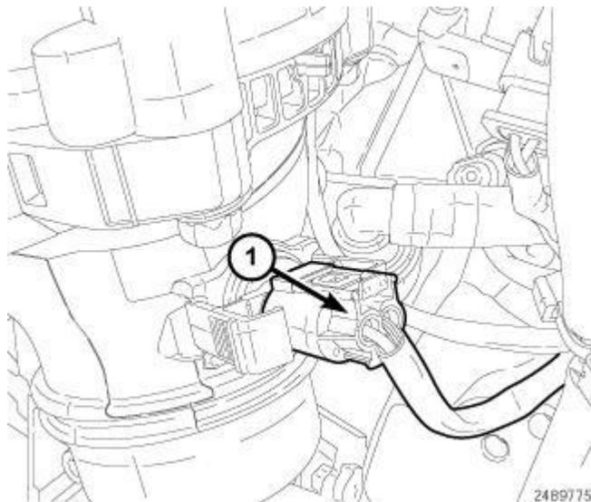
**Fig. 509: Identifying Charge Air Temperature Sensor Connectors**
