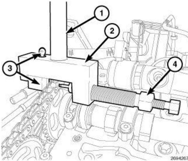
**Fig. 622: Chain Link Tool, Handle, Insert & Thrust Screw/Pin**
