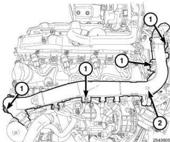
**Fig. 535: Lock Tabs & Engine Wire Harness**
