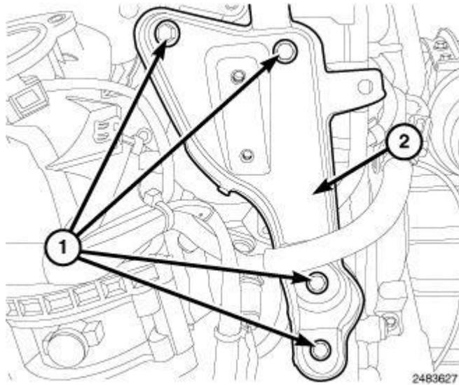
**Fig. 428: Identifying Bolts & EGR Support Bracket**
