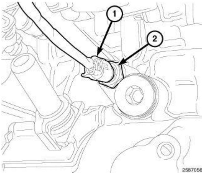
**Fig. 553: Oil Temperature Sensor Harness Connector & Sensor**
