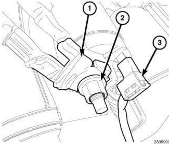
**Fig. 70: Battery Feed Wire To Starter, Starter Harness Connectors & Nut**
