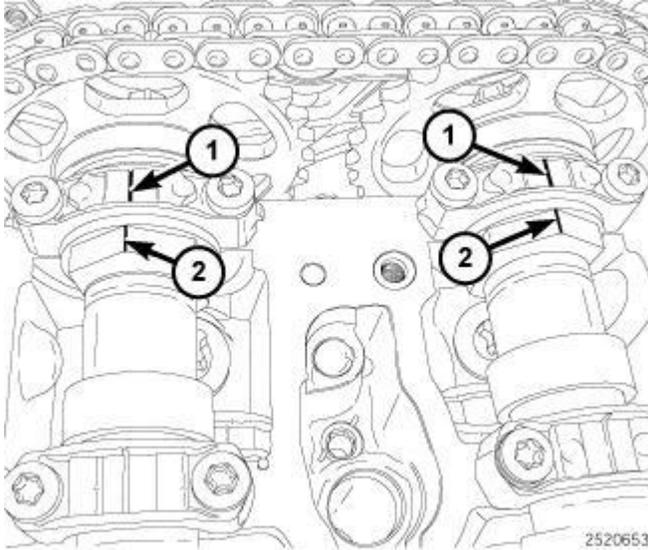
**Fig. 141: Ensuring Camshaft Mark Is Aligned With Bearing Cap Mark**
