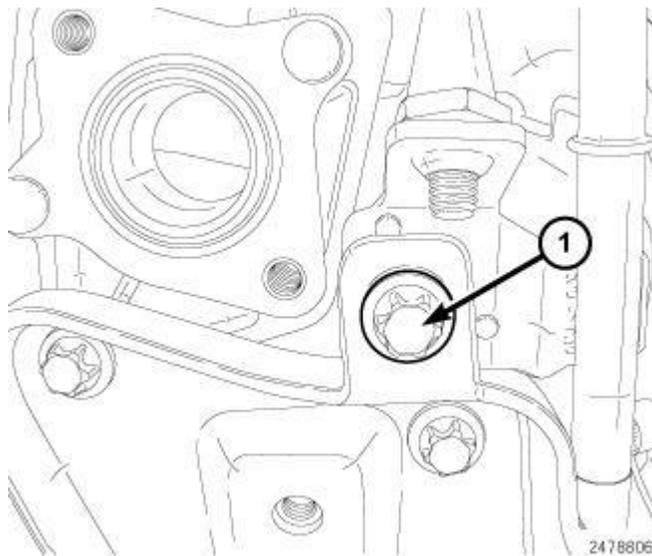
**Fig. 475: Vacuum Tube Bolt**
