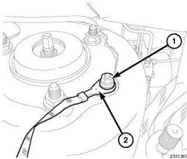
**Fig. 74: Engine Ground Strap & Retaining Nut**
