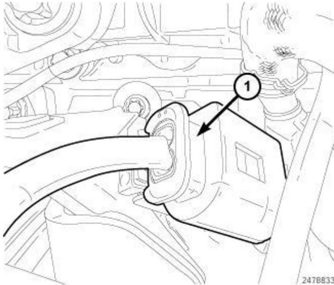
**Fig. 480: Identifying Fuel Quantity Control Valve Harness Connector**
