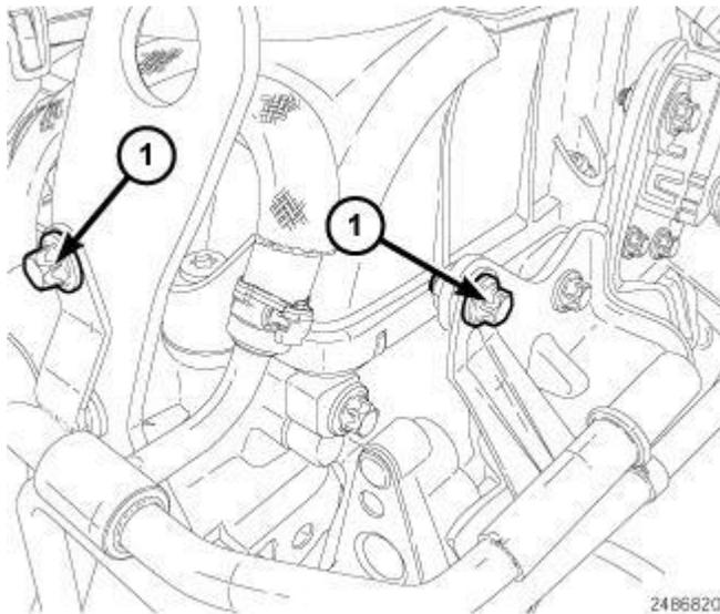
**Fig. 421: Upper Fuel Line Bracket Bolts**
