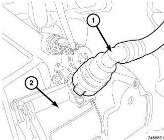
**Fig. 376: Vacuum Hose At Vacuum Pump**
