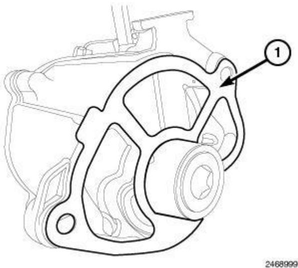
**Fig. 238: Vacuum Pump Gasket**
