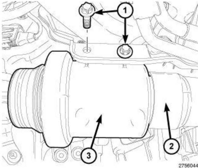
**Fig. 578: Air Charge Resonator, Rear Air Charge Tube & Mounting Bolts**
