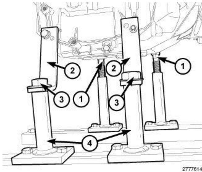
**Fig. 46: Dolly, Cradle & Engine Cradle Post Kit Components**
