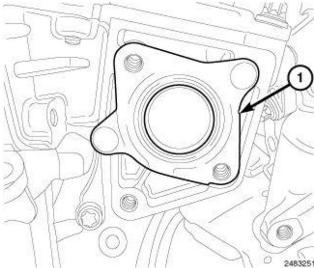
**Fig. 434: Installing/Removing EGR Tube Gasket Onto EGR Actuator**
