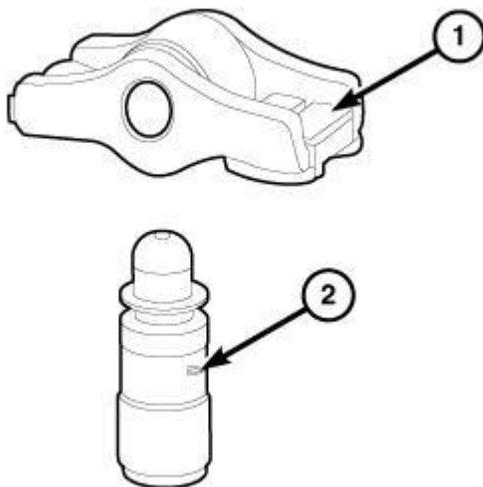
**Fig. 189: Hydraulic Lifter & Rocker Arm**
