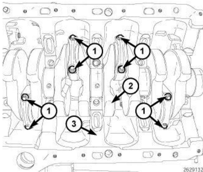
**Fig. 214: Identifying Crankshaft, Engine Block, Connecting Rod Bearing Caps & Bolts**
