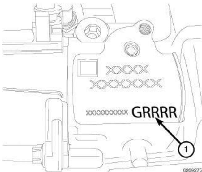
**Fig. 208: Bearing Selection Letters On Engine Block**
