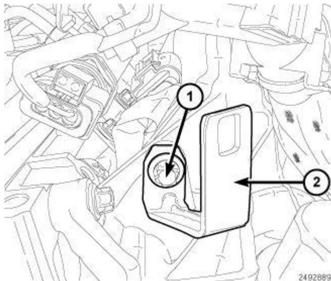
**Fig. 499: Wire Harness Support Bracket & Bolts**
