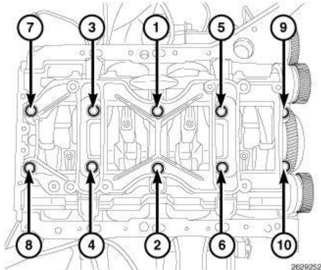
**Fig. 228: Crankshaft Main Bearing Cap Bolts Torque Sequence**
