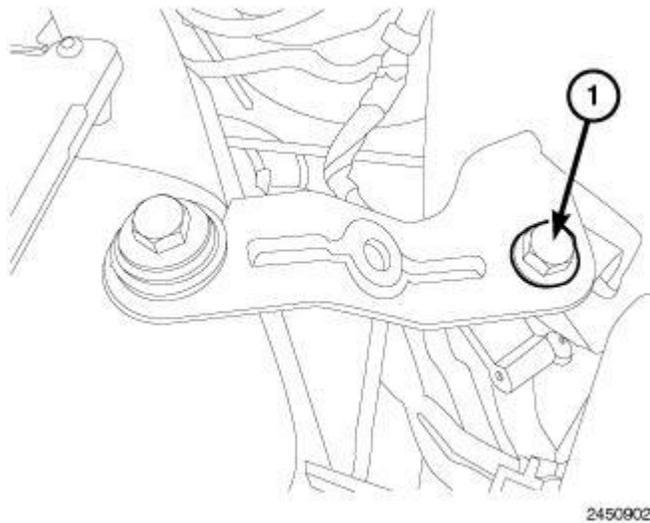
**Fig. 103: Air Cleaner Support Bracket Bolt**
