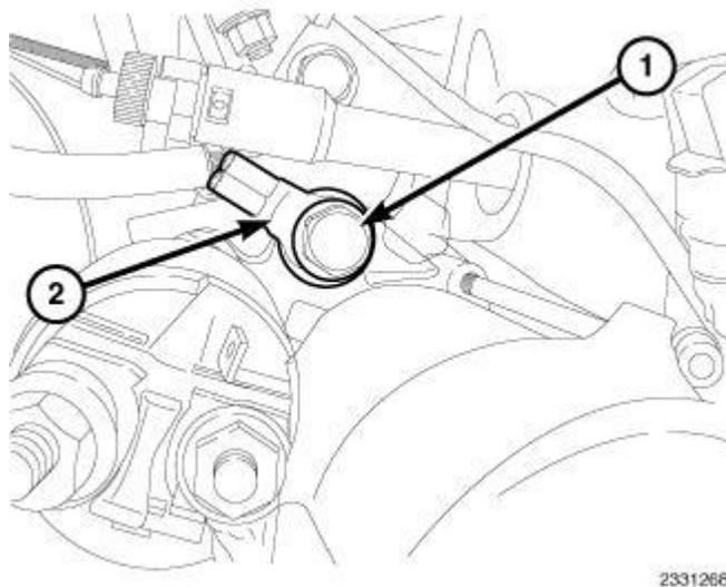
**Fig. 29: Battery Ground Cable At Engine Block**
