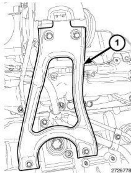
**Fig. 618: Turbocharger Bracket**
