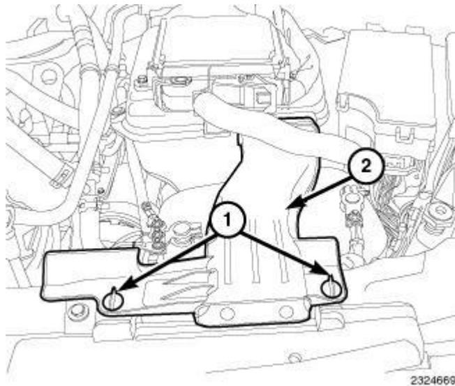
**Fig. 263: Quarter Turn Lock Tabs & Air Inlet Duct**
