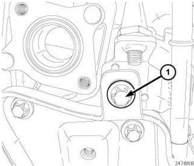
**Fig. 382: Vacuum Tube Bolt**
