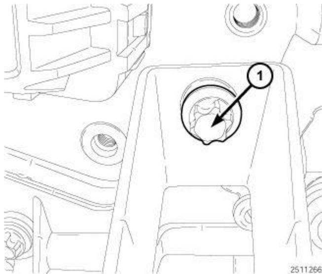
**Fig. 666: Bolt Securing CAC Tube To Glow Plug Module**
