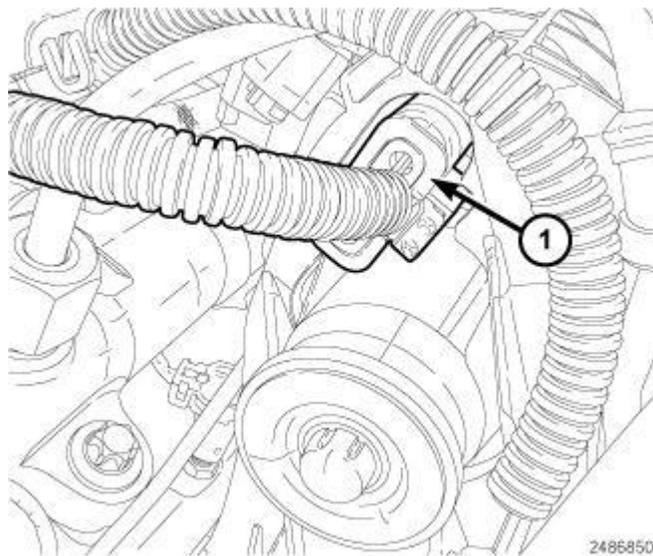
**Fig. 413: Swirl Valve Actuator Harness Connector**
