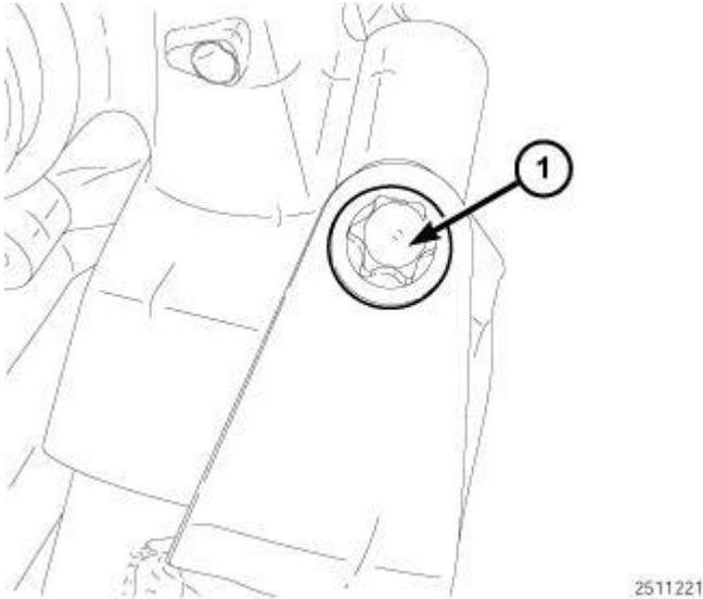
**Fig. 631: Charge Air Cooler CAC Tube Bolt**
