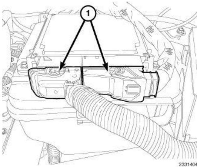
**Fig. 85: PCM Harness Connectors**
