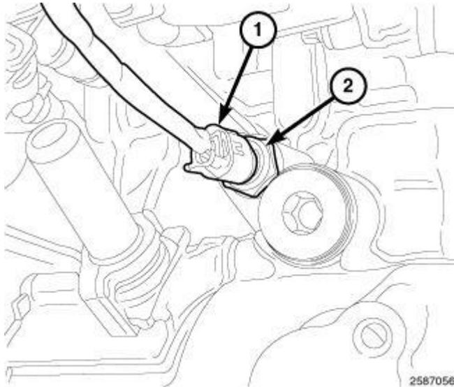
**Fig. 482: Oil Temperature Sensor Harness Connector & Sensor**
