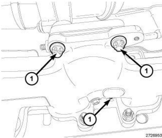
**Fig. 614: Turbocharger-To-Exhaust Manifold Mounting Bolts**
