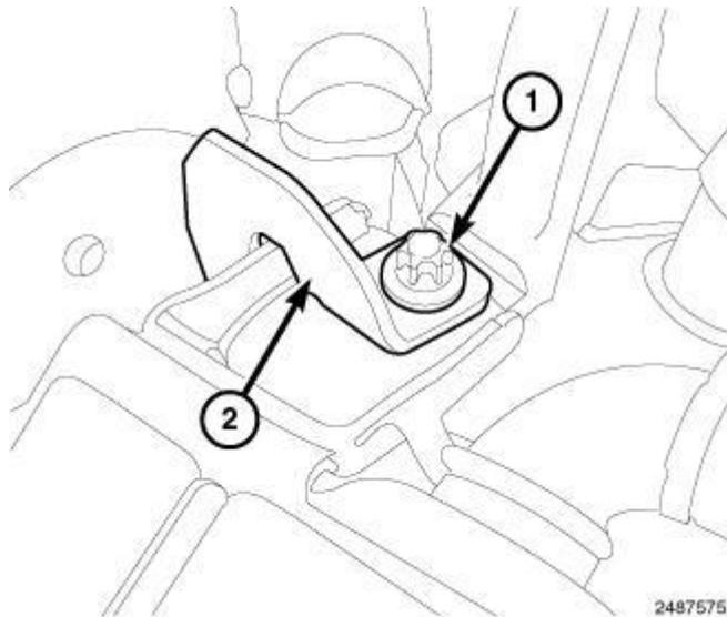
**Fig. 488: Upper EGR Cooler Bolt & Bracket**
