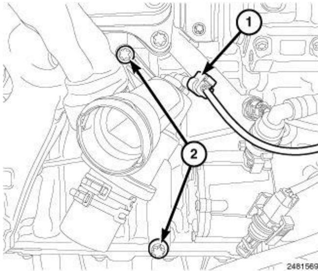
**Fig. 323: Identifying Thermostat Heater Connector & Upper Thermostat Housing Bolt**
