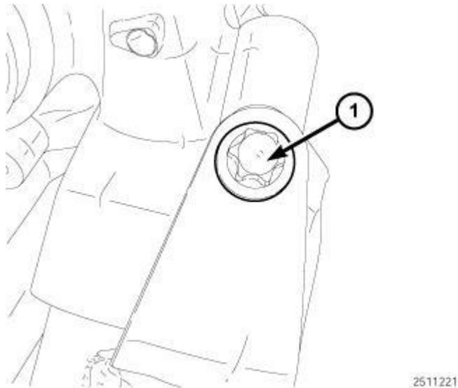
**Fig. 691: Charge Air Cooler CAC Tube Bolt**
