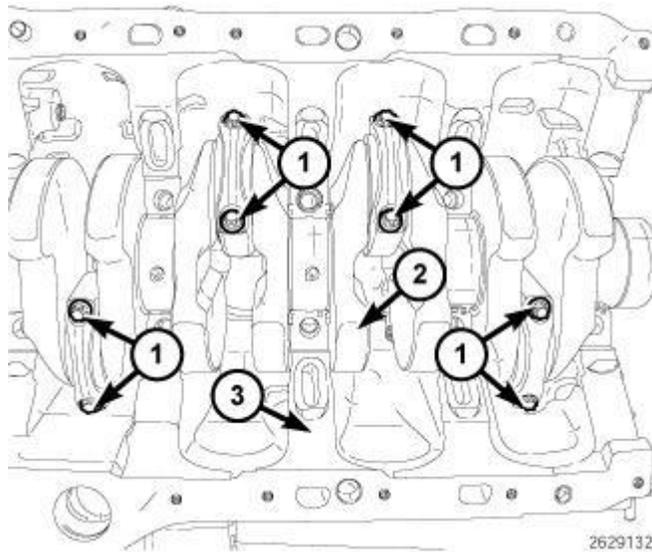
**Fig. 243: Identifying Crankshaft, Engine Block, Connecting Rod Bearing Caps & Bolts**
