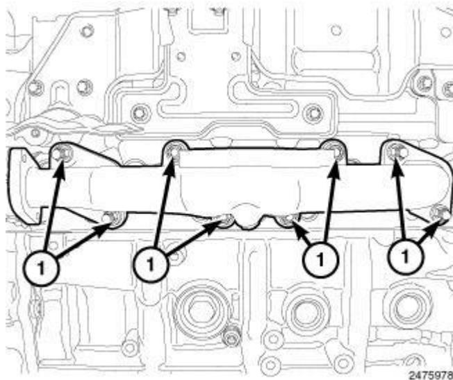
**Fig. 121: Exhaust Manifold Retaining Nuts**
