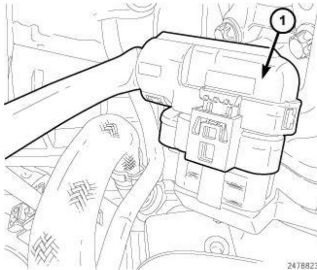
**Fig. 479: Identifying EGR Valve Harness Connector**
