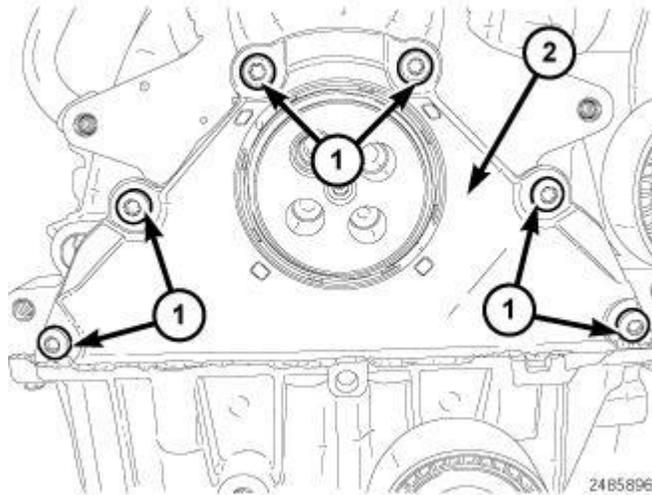
**Fig. 252: Front Oil Seal Carrier & Bolts**
