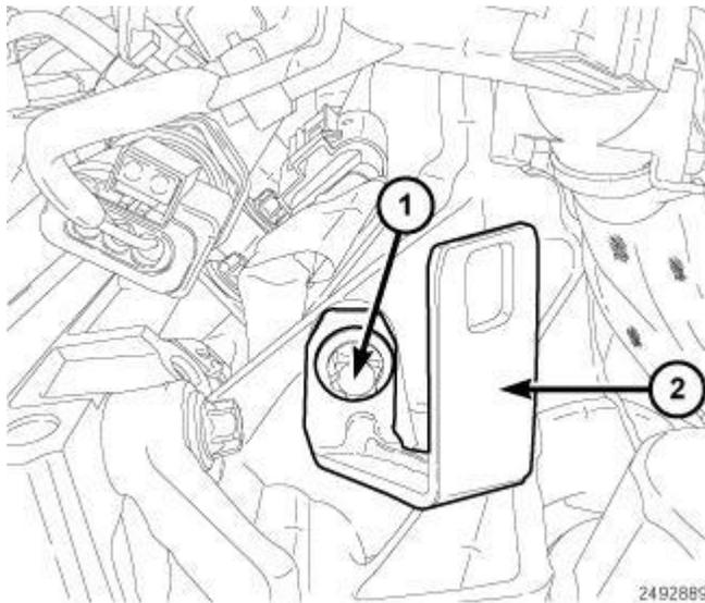
**Fig. 320: Wire Harness Support Bracket & Bolts**
