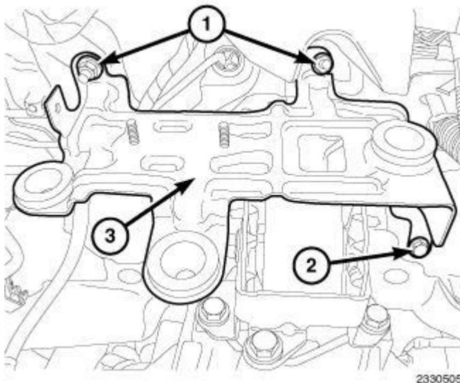
**Fig. 17: Air Cleaner Mounting Bracket, Nuts & Bolt**
