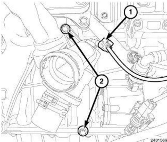
**Fig. 531: Identifying Thermostat Heater Connector & Upper Thermostat Housing Bolt**
