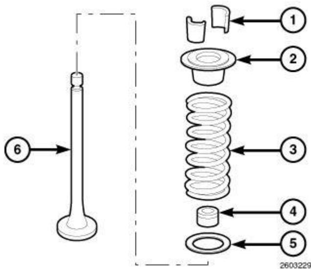
**Fig. 203: Valve Spring, Keeper, Retainer, Spring Seat, Valve Stem Seals & Valve**
