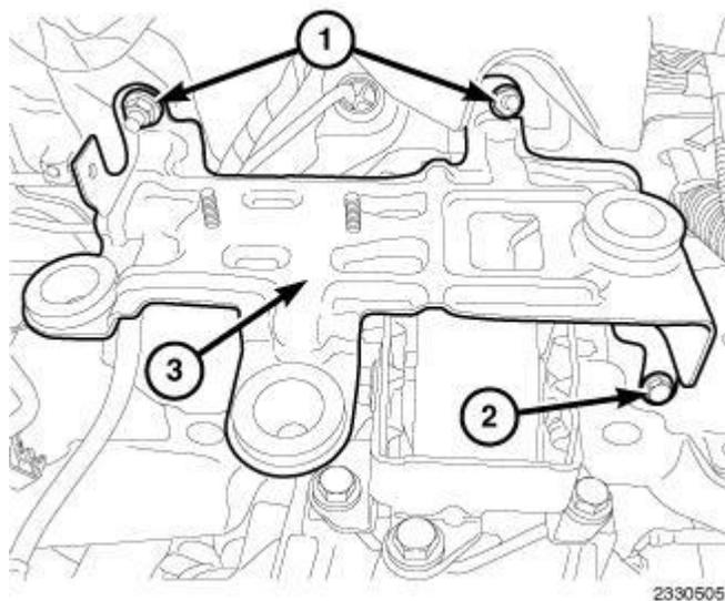
**Fig. 81: Air Cleaner Mounting Bracket, Nuts & Bolt**
