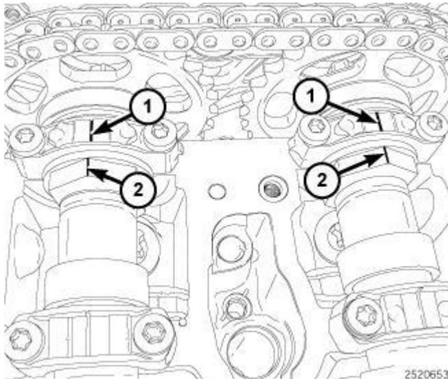
**Fig. 136: Ensuring Camshaft Mark Is Aligned With Bearing Cap Mark**
