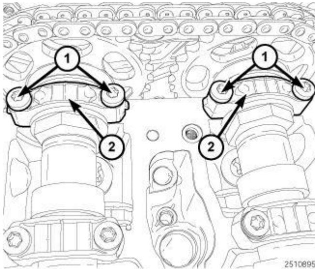
**Fig. 676: No. 1 Camshaft Bearing Caps & Bolts**
