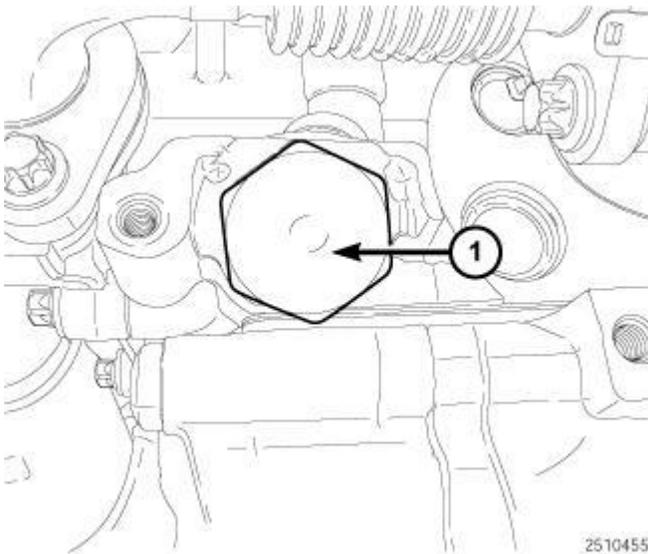
**Fig. 701: Timing Chain Tensioner**
