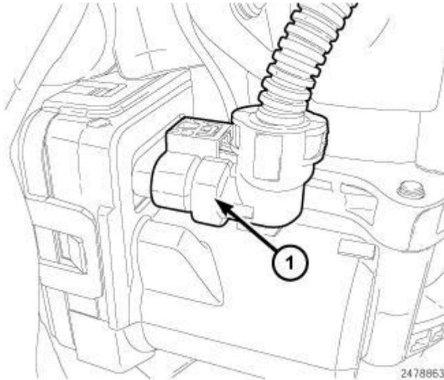
**Fig. 510: EGR Air Flow Control Valve Harness Connector**
