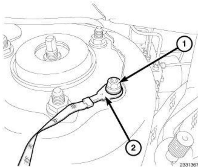
**Fig. 24: Engine Ground Strap & Retaining Nut**
