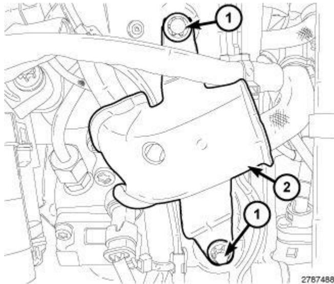
**Fig. 401: Identifying Bolts & Heat Shield**
