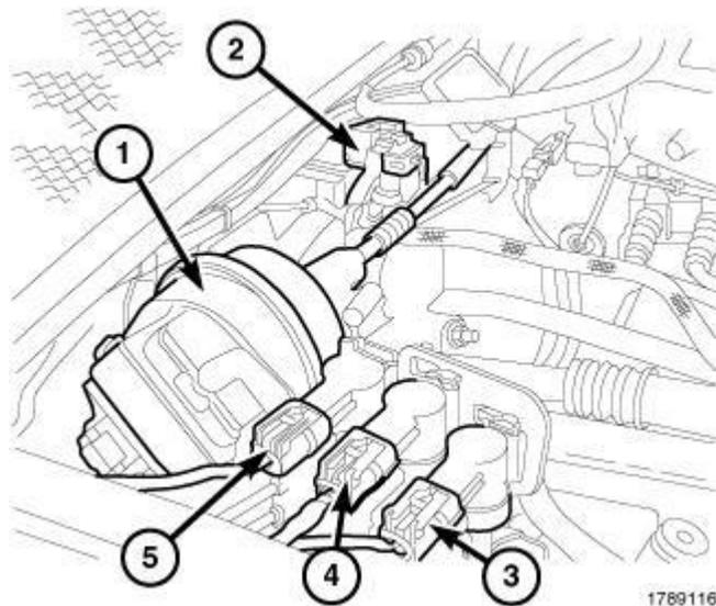
**Fig. 601: Wastegate Solenoid & Electrical Connectors**
