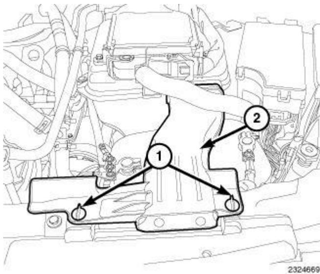
**Fig. 119: Quarter Turn Lock Tabs & Air Inlet Duct**
