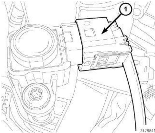
**Fig. 512: Boost Pressure Sensor Harness Connector**
