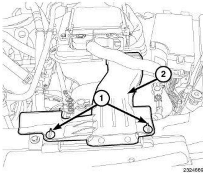
**Fig. 524: Quarter Turn Lock Tabs & Air Inlet Duct**
