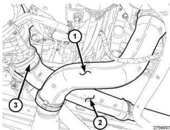
**Fig. 575: Identifying Front Upper & Lower Air Charge Hose**
