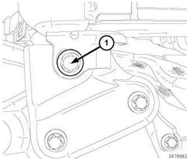
**Fig. 424: Lower EGR Cooler Bolt**
