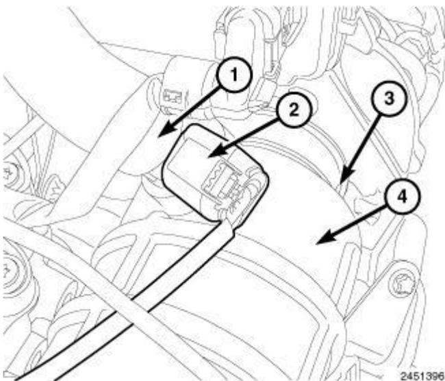
**Fig. 115: CCV Hose, Heater Harness Connector, Turbocharger Inlet Tube & Clamp**
