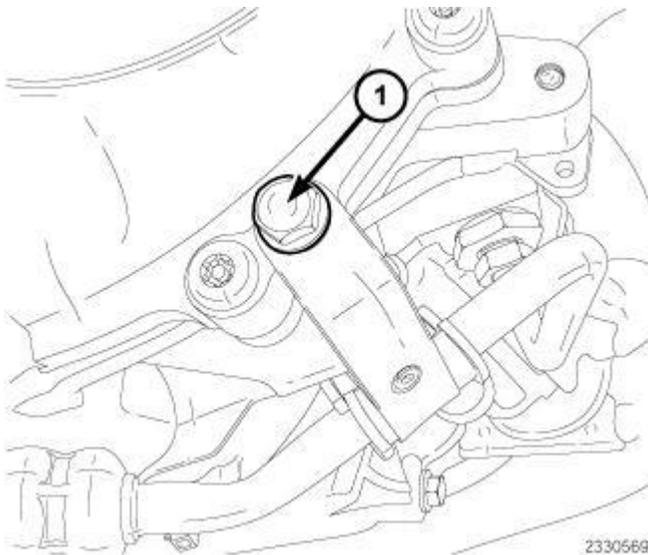
**Fig. 59: Power Steering Line Support Bracket Retaining Bolt**
