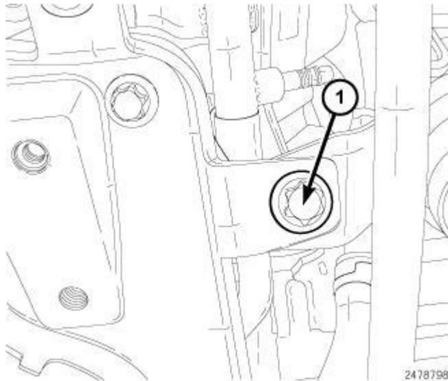
**Fig. 517: Oil Dip Stick Bolt**
