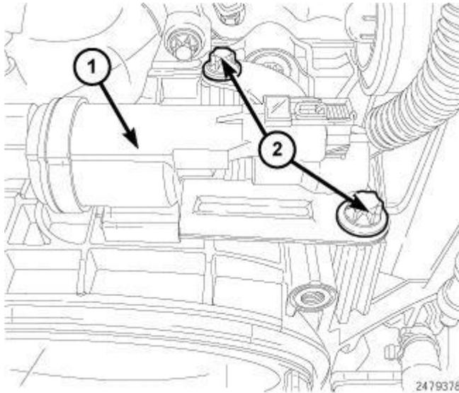
**Fig. 339: EGR Vacuum Solenoid & Bolts**
