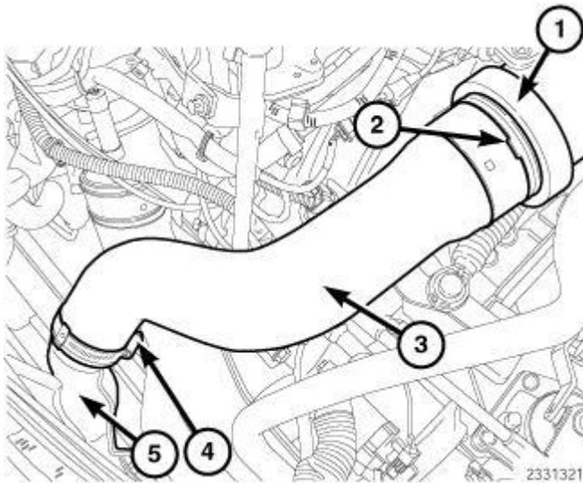
**Fig. 20: Upper Charge Air Tube, Lock Ring, Lower Charge Air Tube, Clamp & Charge Air Cooler (CAC) Inlet**
