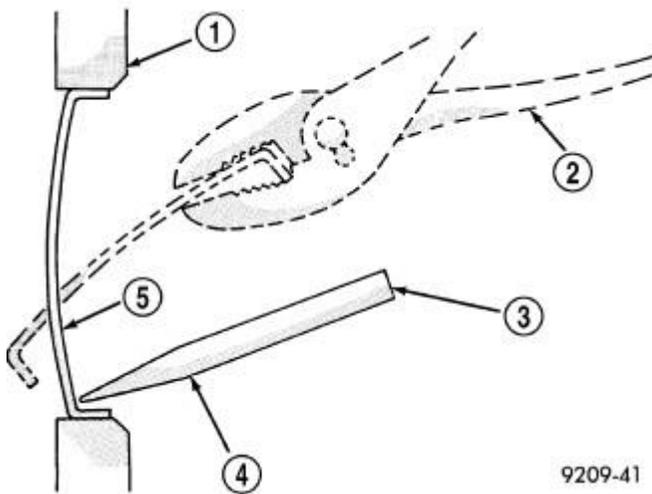
**Fig. 206: Core Hole Plug Removal**
