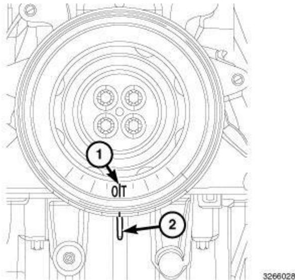
**Fig. 674: Crankshaft Alignment Timing Marks**
