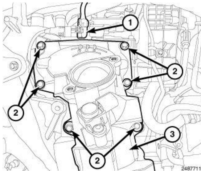
**Fig. 463: Knock Sensor Electrical Connector, Mixing Chamber & Bolts**
