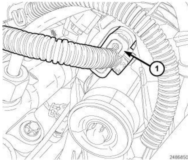
**Fig. 418: Swirl Valve Actuator Harness Connector**
