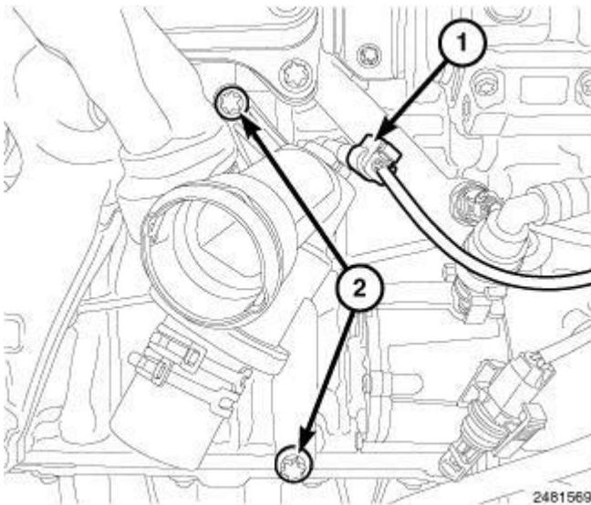
**Fig. 332: Identifying Thermostat Heater Connector & Upper Thermostat Housing Bolt**
