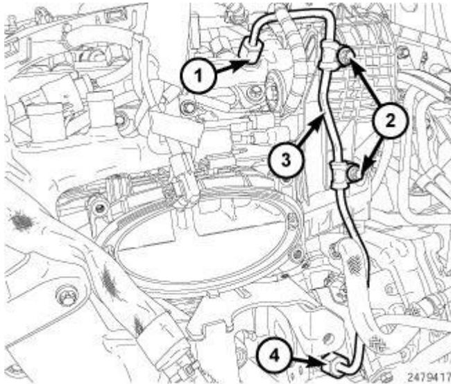
**Fig. 540: Identifying Fuel Rail, Bolts, High Pressure Fuel Tube & Pump**
