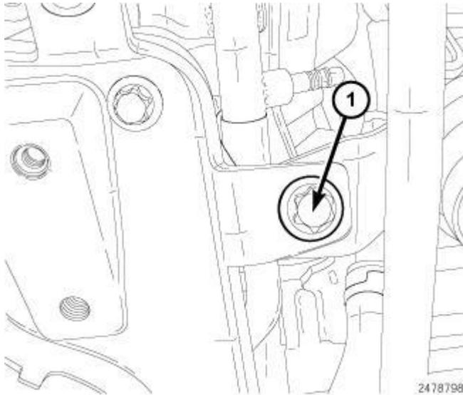
**Fig. 381: Oil Dip Stick Bolt**
