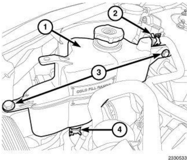
**Fig. 7: Coolant Recovery Reservoir, Clamps & Bolts**
