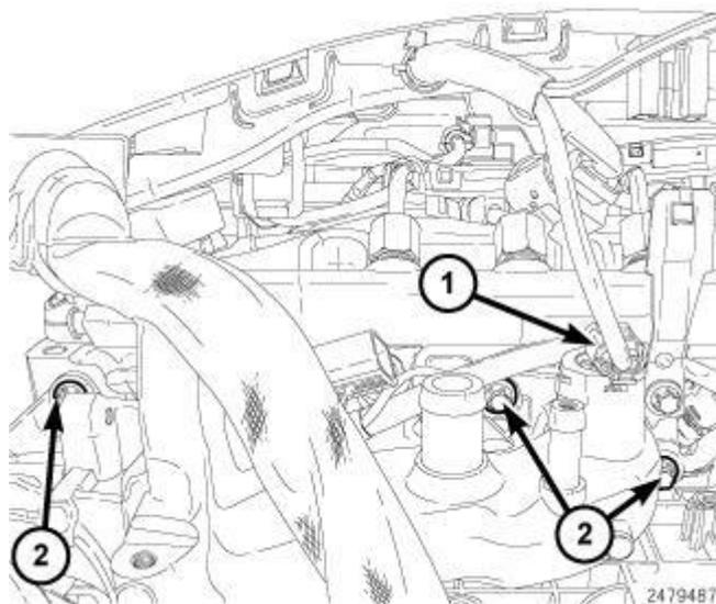
**Fig. 321: Coolant Temp Sensor & Cooling Manifold Bolts**
