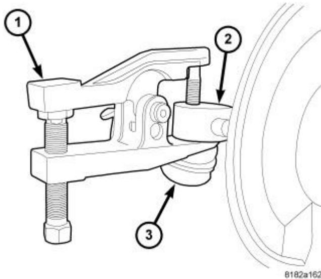
**Fig. 34: Separating Tie Rod End From Knuckle Using Ball Joint Remover 9360**
