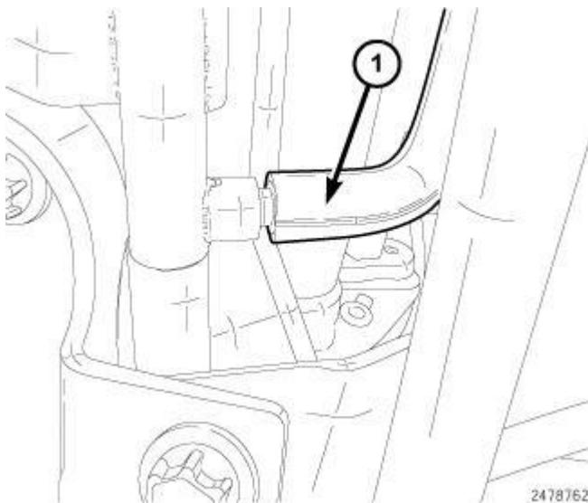
**Fig. 397: Vacuum Supply Line At EGR Solenoid**
