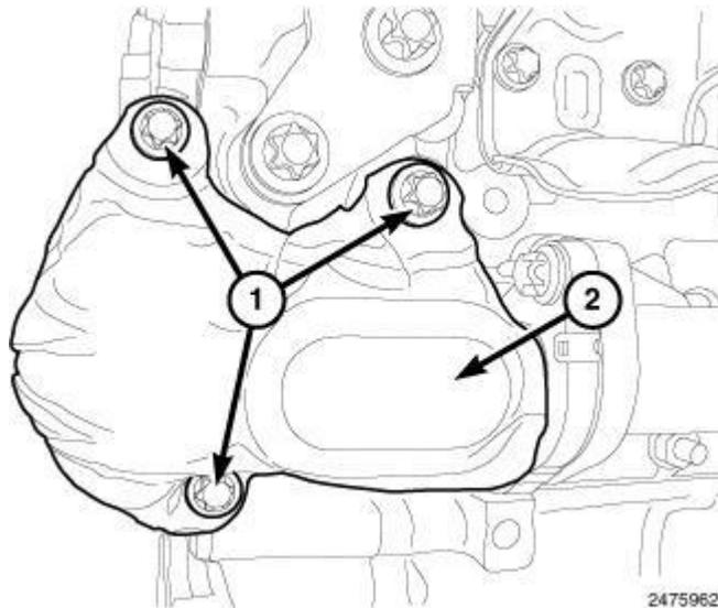
**Fig. 440: EGR Pipe Heat Shield & Bolts**
