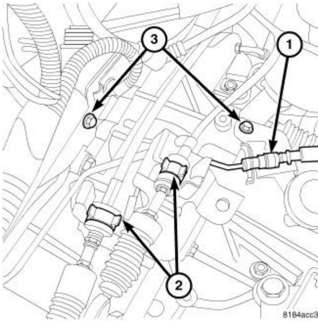
**Fig. 68: Hydraulic Line, Shift Cables & Bolts**
