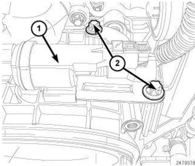
**Fig. 316: EGR Vacuum Solenoid & Bolts**
