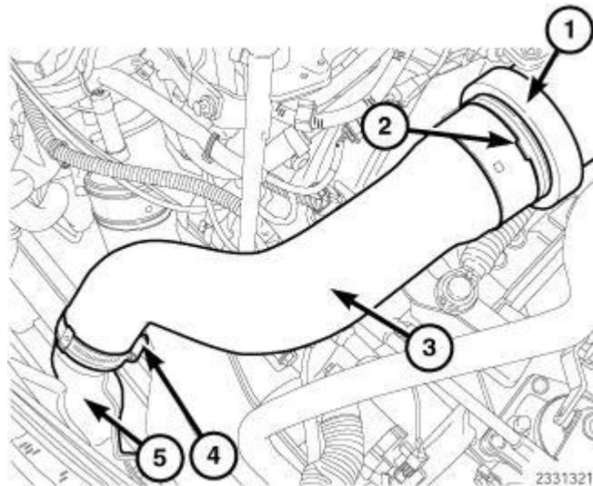
**Fig. 620: Upper Charge Air Tube, Lock Ring, Lower Charge Air Tube, Clamp & Charge Air Cooler (CAC) Inlet**
