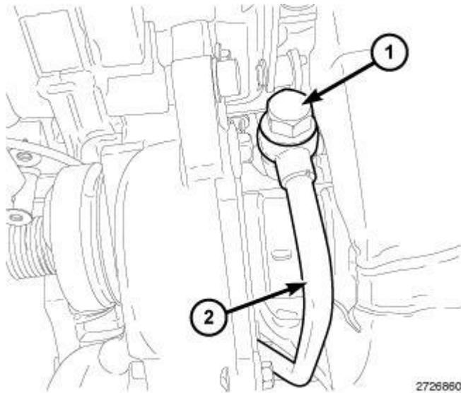
**Fig. 610: Oil Supply Line & Banjo Bolt At Turbocharger**
