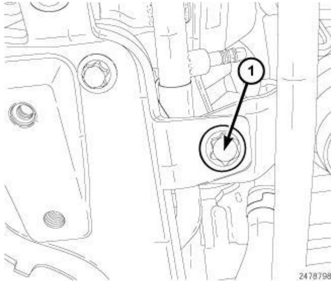
**Fig. 432: Oil Dip Stick Bolt**
