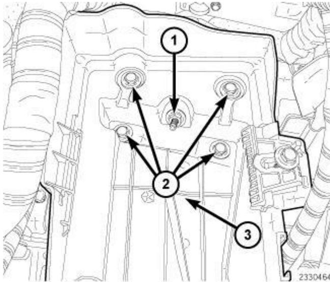
**Fig. 287: Battery Tray, Nut & Retaining Bolts**
