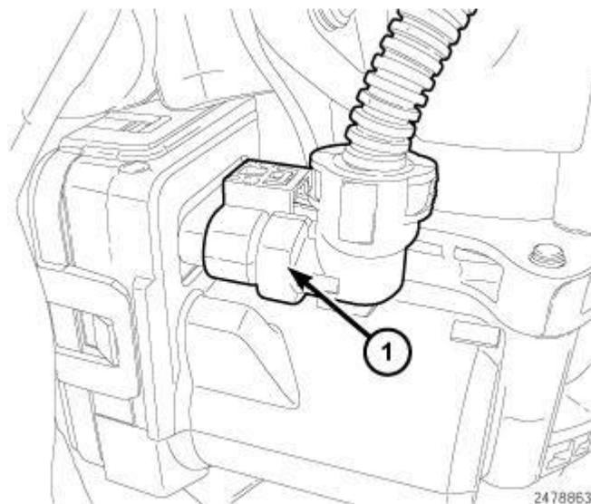
**Fig. 461: EGR Air Flow Control Valve Harness Connector**
