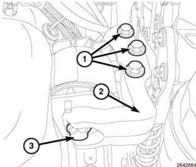
**Fig. 297: Engine Mount, Bracket & Through Bolt**
