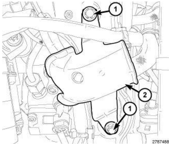
**Fig. 380: Identifying Bolts & Heat Shield**
