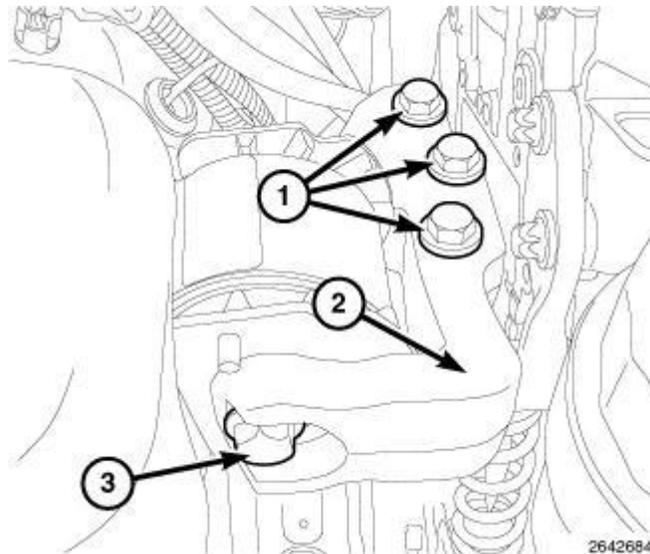
**Fig. 290: Engine Mount, Bracket & Through Bolt**
