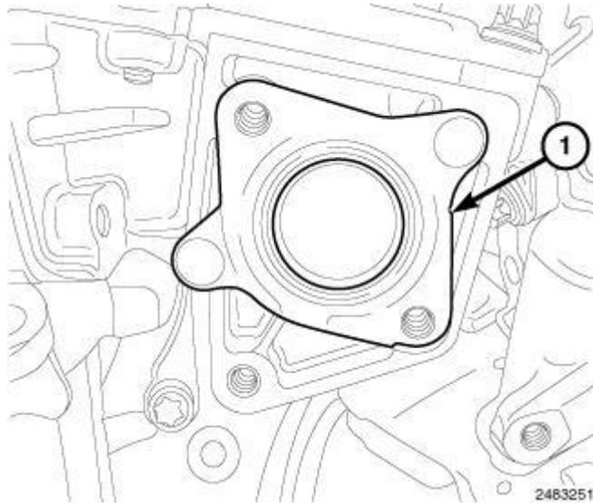
**Fig. 661: Installing/Removing EGR Tube Gasket Onto EGR Actuator**
