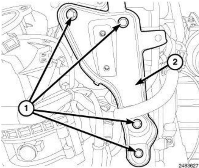
**Fig. 513: Identifying Bolts & EGR Support Bracket**
