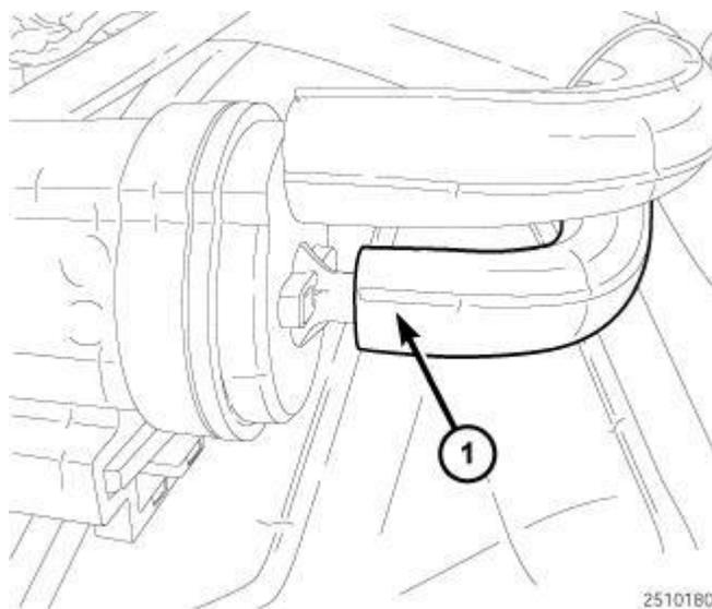
**Fig. 233: Coolant Pump Actuator Vacuum Line**
