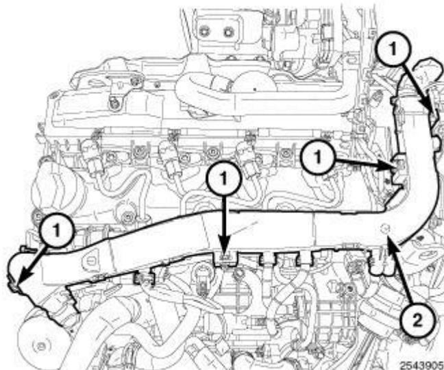
**Fig. 167: Lock Tabs & Engine Wire Harness**
