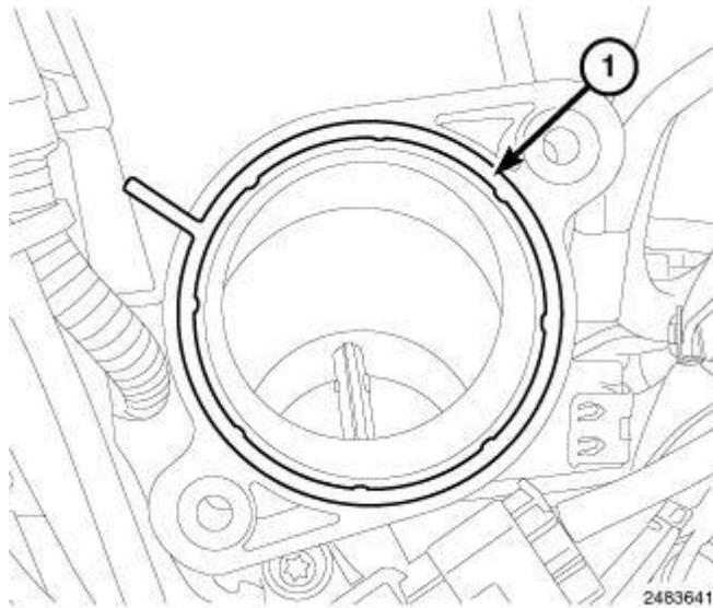
**Fig. 562: Installing/Removing EGR Tube Gasket Onto Mixing Chamber**
