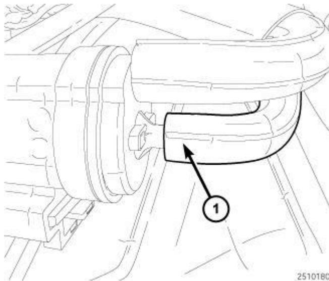
**Fig. 57: Coolant Pump Actuator Vacuum Line**
