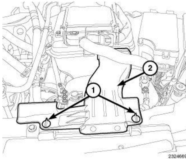
**Fig. 131: Quarter Turn Lock Tabs & Air Inlet Duct**
