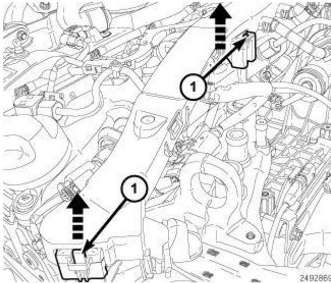
**Fig. 319: Locating Lock Tabs And Lifting Up On Wire Harness**
