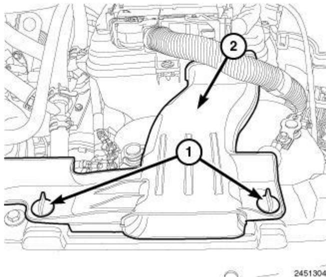
**Fig. 112: Air Inlet Duct & Fasteners**
