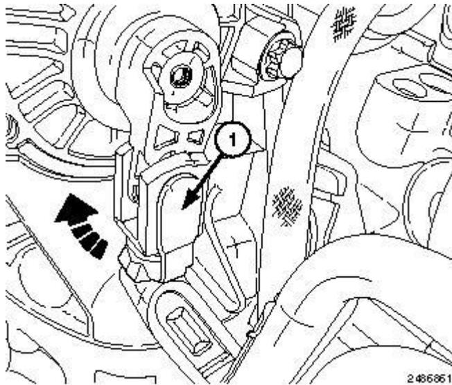
**Fig. 414: Releasing Lock Clip At Swirl Valve Linkage**
