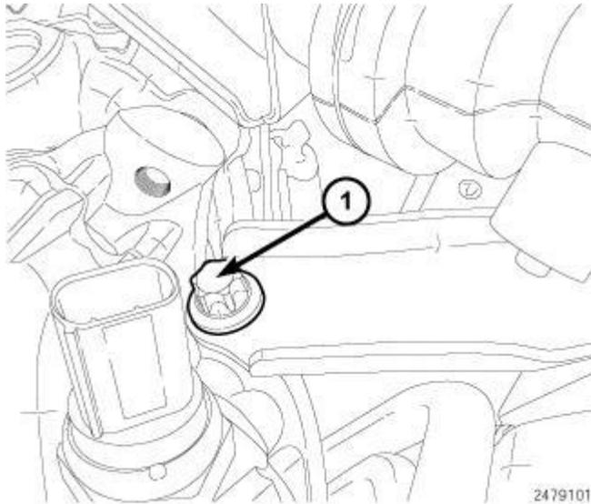
**Fig. 653: Support Bracket Bolt**
