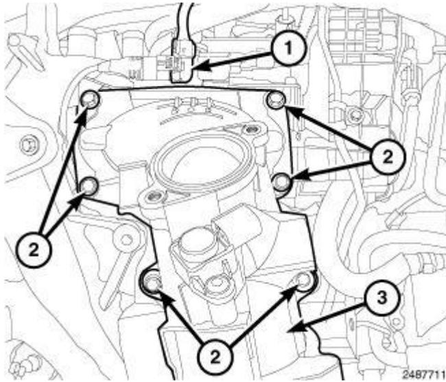
**Fig. 542: Knock Sensor Electrical Connector, Mixing Chamber & Bolts**
