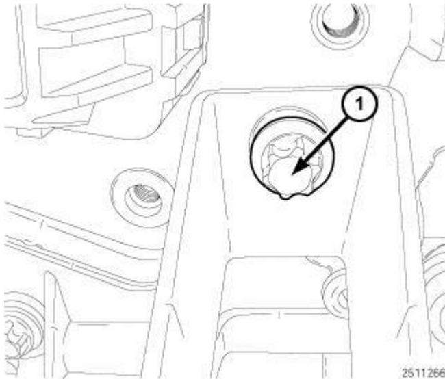
**Fig. 705: Bolt Securing CAC Tube To Glow Plug Module**
