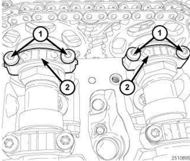
**Fig. 143: No. 1 Camshaft Bearing Caps & Bolts**
