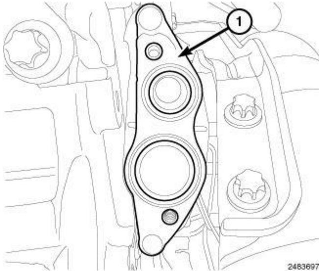
**Fig. 543: Identifying EGR Manifold Gasket**
