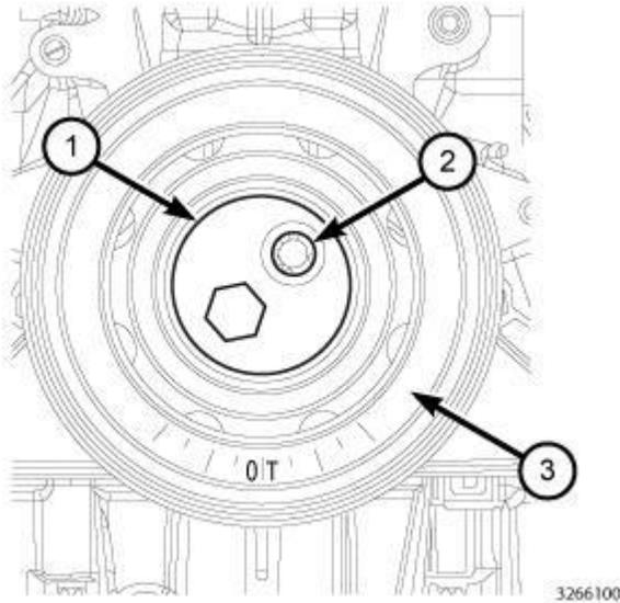
**Fig. 247: Vibration Damper Holder Tool, Vibration Damper & Bolts**
