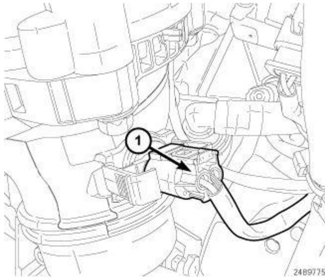
**Fig. 462: Identifying Charge Air Temperature Sensor Connectors**
