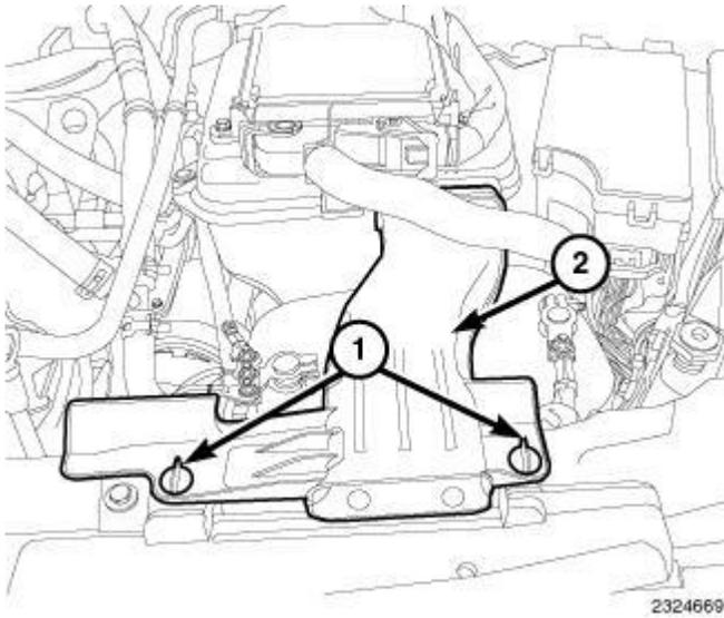
**Fig. 248: Quarter Turn Lock Tabs & Air Inlet Duct**
