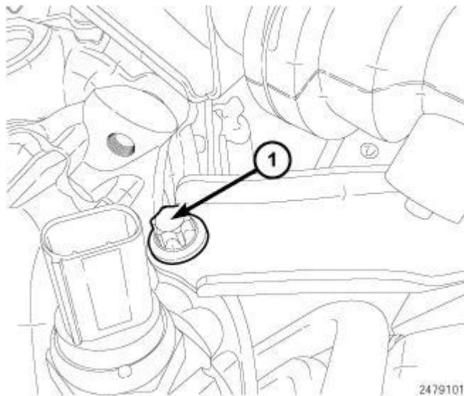
**Fig. 545: Support Bracket Bolt**
