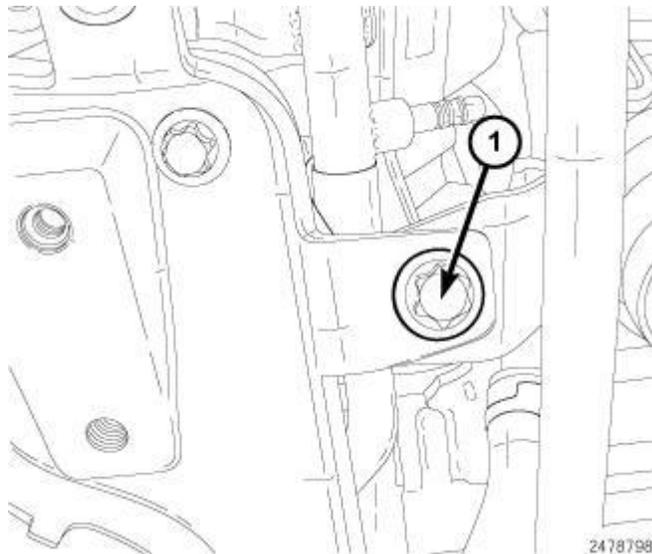
**Fig. 659: Oil Dip Stick Bolt**
