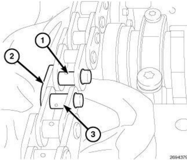
**Fig. 623: Connecting New Timing Chain With Old Timing Chain With Assembly Link**
