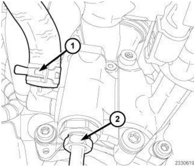
**Fig. 60: Power Steering Supply Line & Feed Line**
