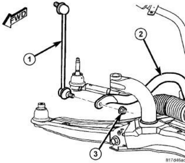
**Fig. 66: Stabilizer Link Mounting To Bar**
