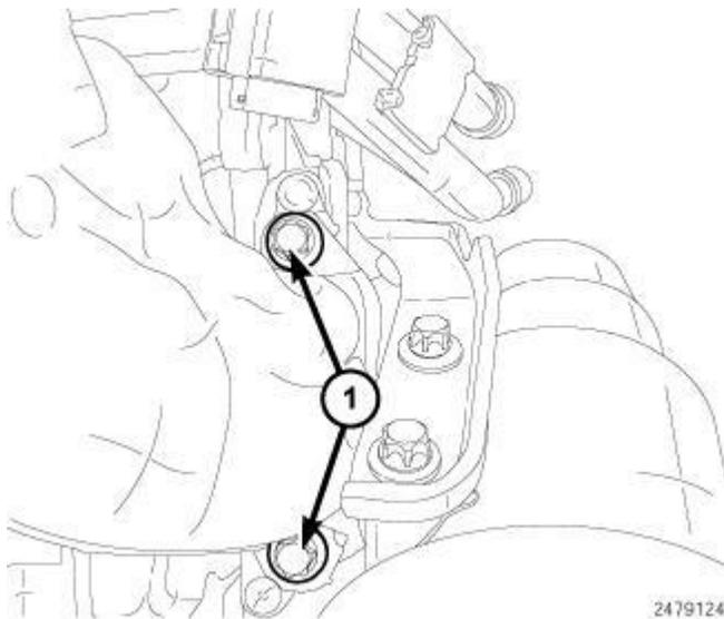
**Fig. 491: Identifying EGR Cooler Manifold Bolts**
