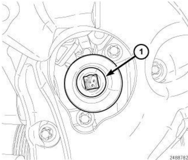
**Fig. 306: Removing/Installing Piston Cooling Oil Control Valve Using Shift Valve Socket**
