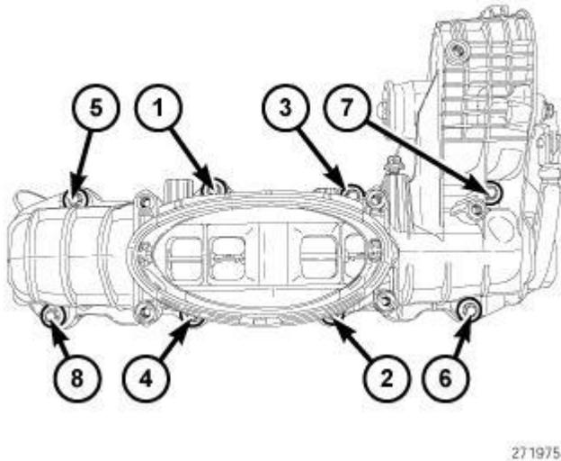
**Fig. 527: Intake Manifold Bolt Torque Sequence**
