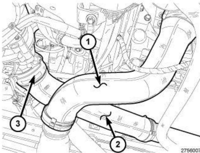
**Fig. 582: Identifying Front Upper & Lower Air Charge Hose**
