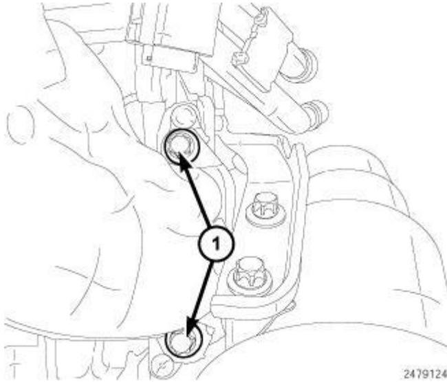
**Fig. 422: Identifying EGR Cooler Manifold Bolts**
