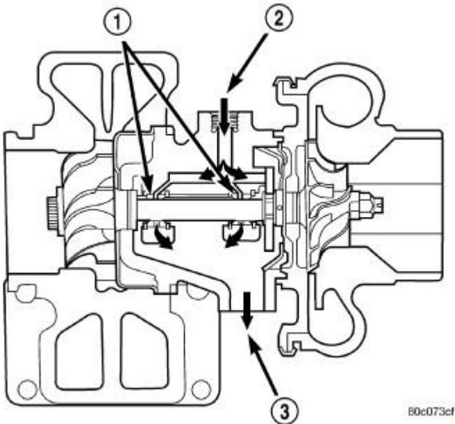
**Fig. 604: Turbocharger Oil Supply And Drain**
