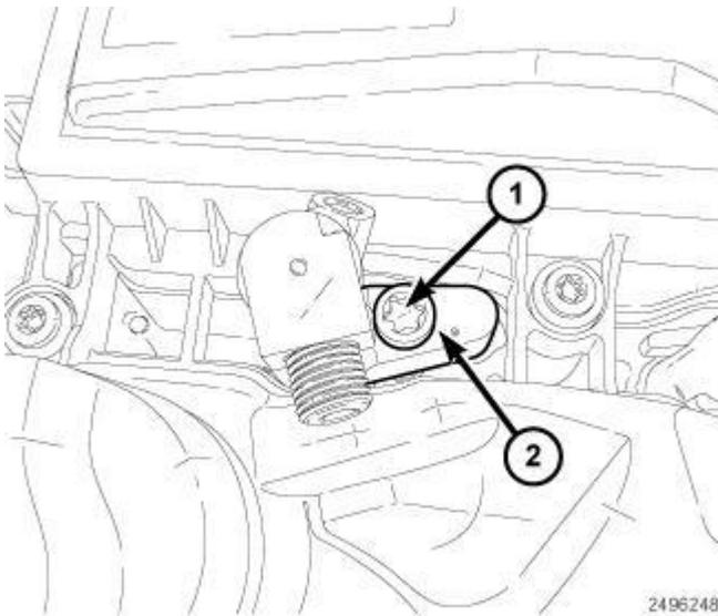
**Fig. 171: Identifying Bolt & Clamping Claw**
