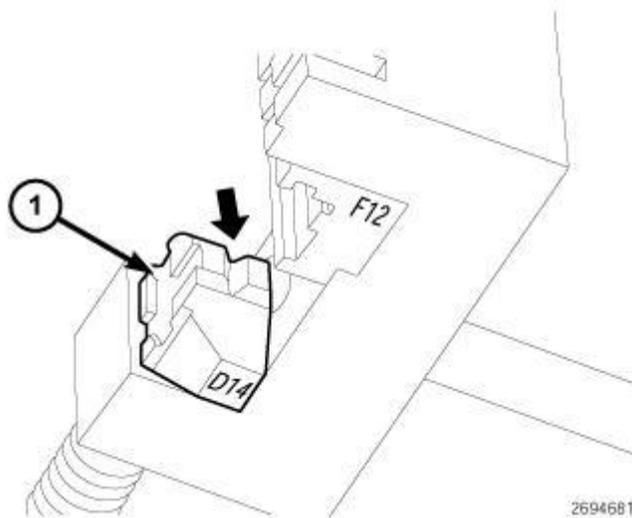
**Fig. 627: Turning Over Thrust Piece With Digit D14**
