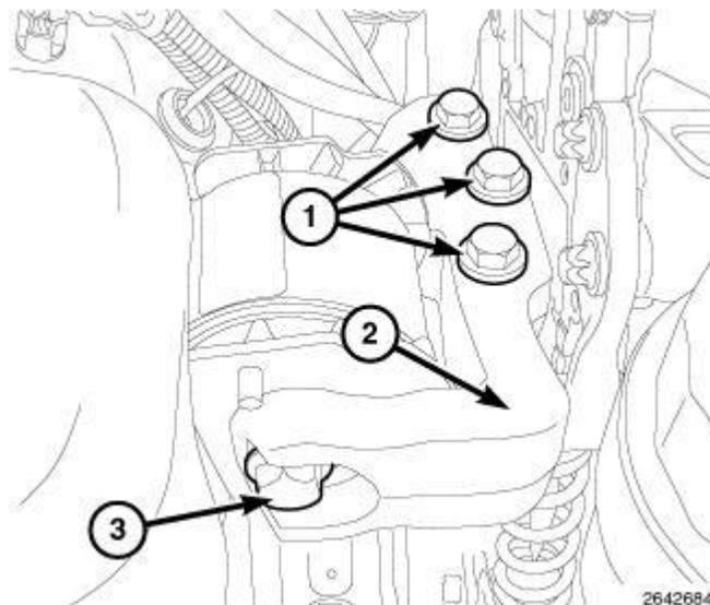
**Fig. 293: Engine Mount, Bracket & Through Bolt**
