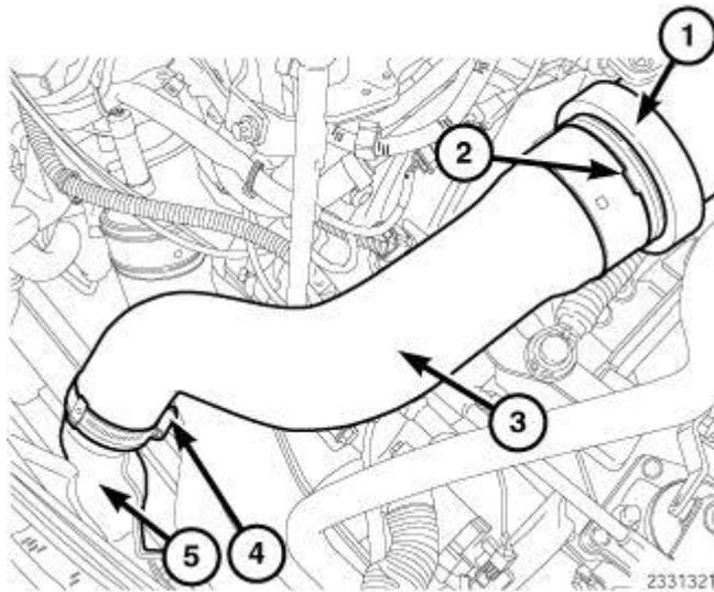
**Fig. 78: Upper Charge Air Tube, Lock Ring, Lower Charge Air Tube, Clamp & Charge Air Cooler (CAC) Inlet**
