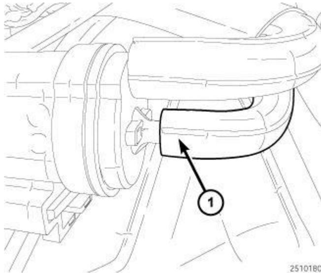
**Fig. 223: Coolant Pump Actuator Vacuum Line**
