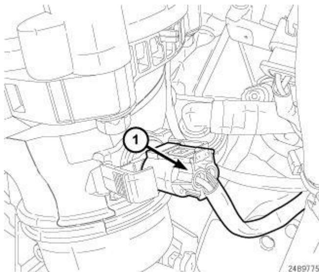
**Fig. 549: Identifying Charge Air Temperature Sensor Connectors**
