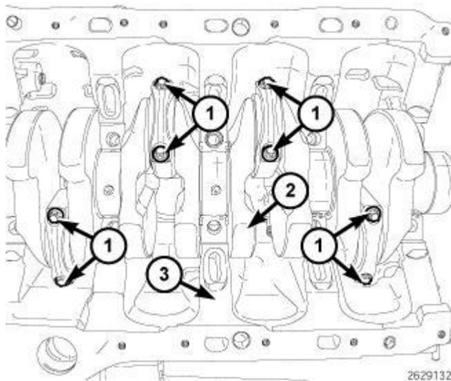
**Fig. 244: Identifying Crankshaft, Engine Block, Connecting Rod Bearing Caps & Bolts**
