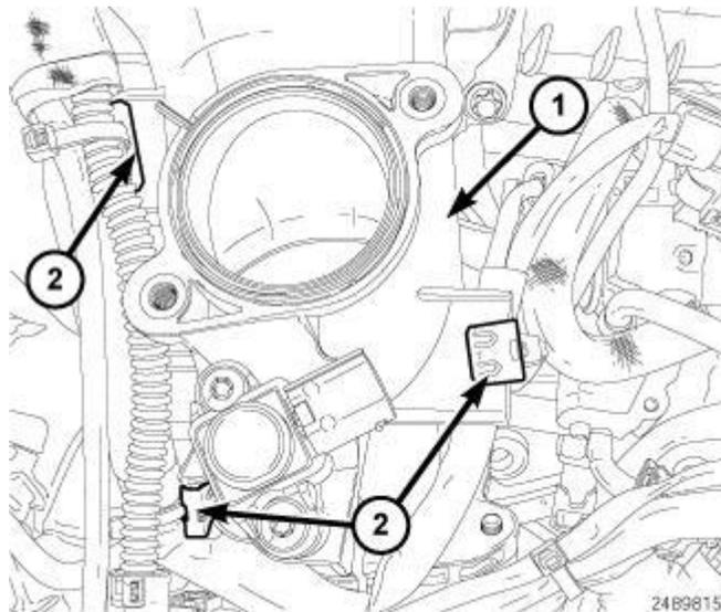
**Fig. 460: Mixing Chamber & Wire Harness Retainer Clips**
