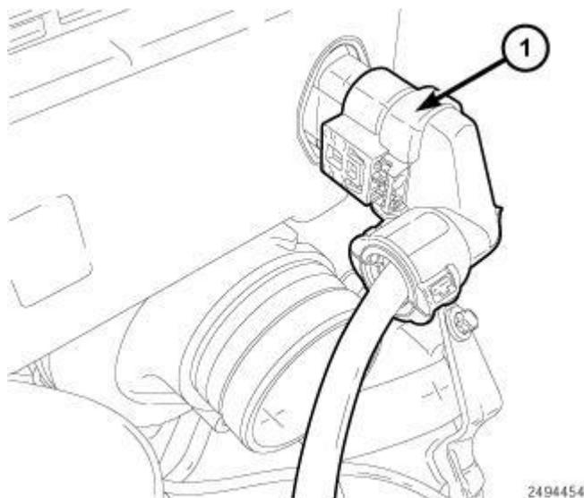
**Fig. 185: Turbocharger Actuator Harness Connector**
