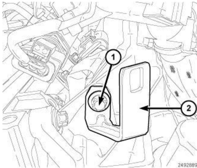
**Fig. 335: Wire Harness Support Bracket & Bolts**
