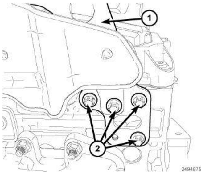
**Fig. 173: Engine Lifting Eye & Bolts**
