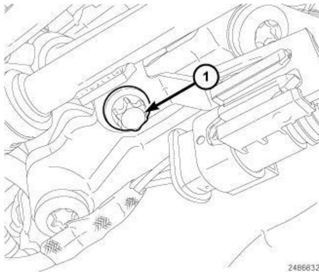
**Fig. 411: Lower Fuel Line Bracket Bolt**
