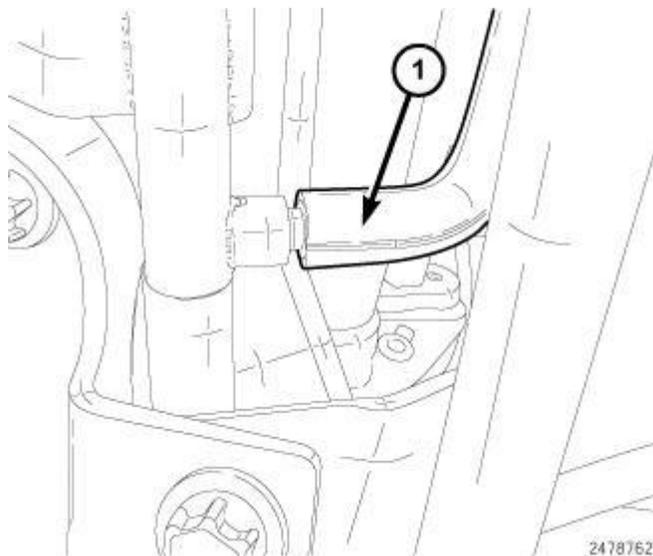
**Fig. 436: Vacuum Supply Line At EGR Solenoid**
