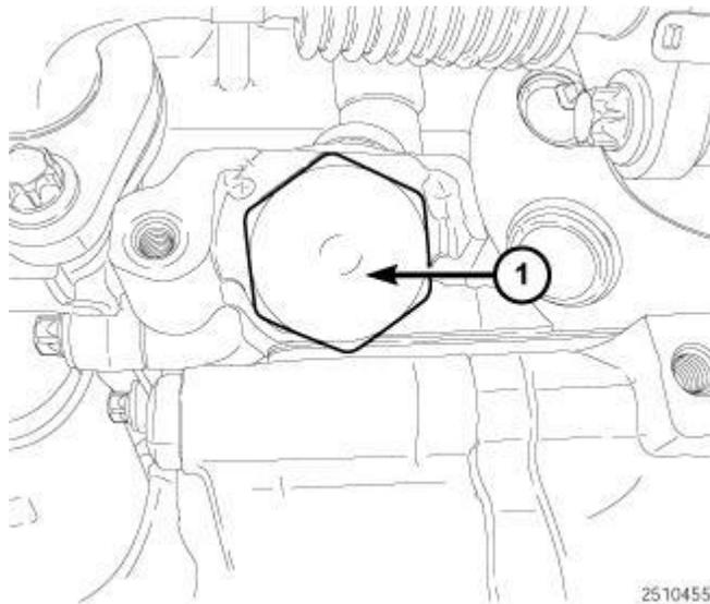
**Fig. 699: Timing Chain Tensioner**
