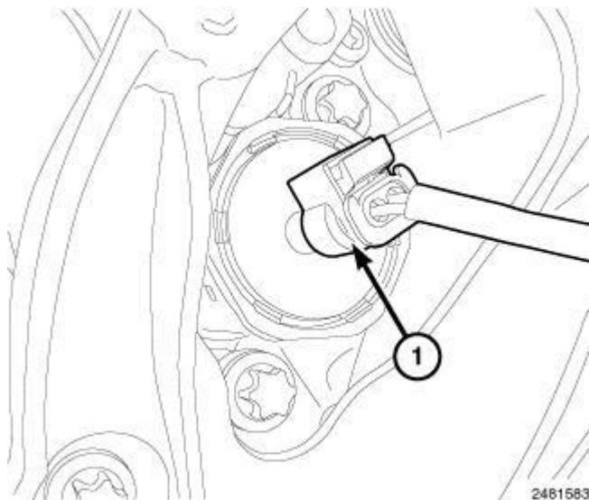
**Fig. 322: Piston Cooling Oil Control Valve Harness Connector**
