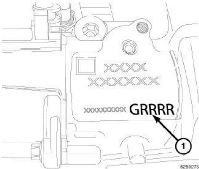
**Fig. 213: Bearing Selection Letters On Engine Block**
