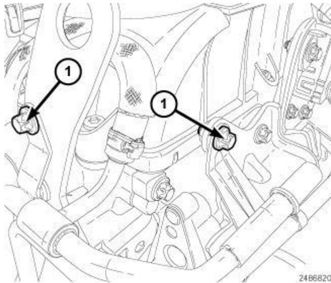
**Fig. 410: Upper Fuel Line Bracket Bolts**
