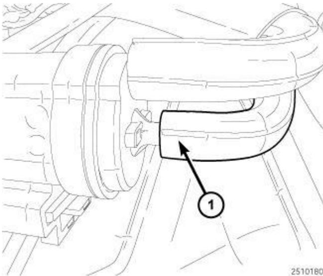
**Fig. 43: Coolant Pump Actuator Vacuum Line**
