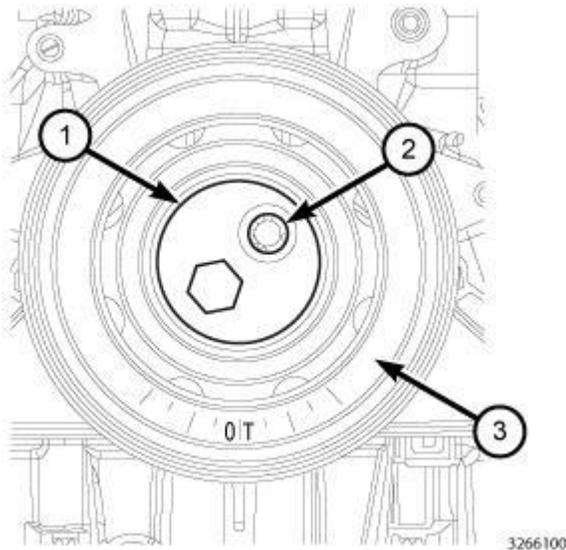
**Fig. 693: Vibration Damper Holder Tool, Vibration Damper & Bolts**
