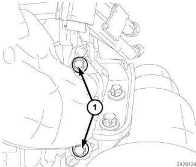
**Fig. 409: Identifying EGR Cooler Manifold Bolts**
