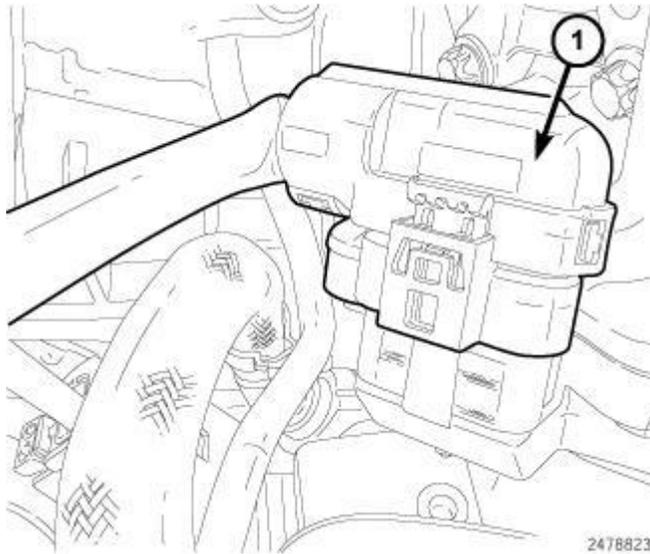
**Fig. 404: Identifying EGR Valve Harness Connector**
