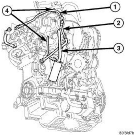
**Fig. 584: Turbocharger Lines And Hoses**
