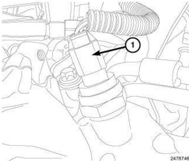
**Fig. 569: Identifying EGR Back Pressure Transducer Harness Connector**
