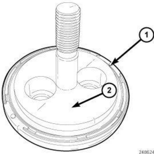
**Fig. 259: Front Crankshaft Oil Seal & Front Crankshaft Seal Adapter**
