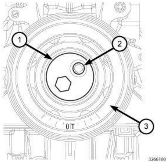
**Fig. 219: Vibration Damper Holder Tool, Vibration Damper & Bolts**
