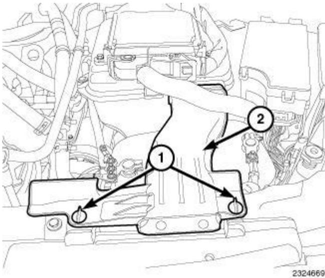
**Fig. 464: Quarter Turn Lock Tabs & Air Inlet Duct**
