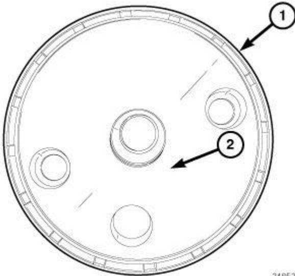
**Fig. 266: Rear Crankshaft Oil Seal & Rear Main Seal Ring Installer Adaptor**
