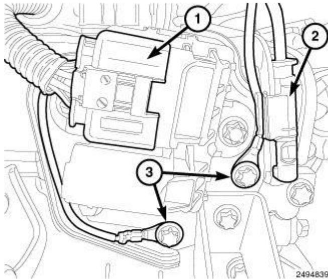
**Fig. 166: Identifying Glow Plug Module Harness Connector, Bolts & Turbocharger Exhaust Temperature Sensor Harness Connector**
