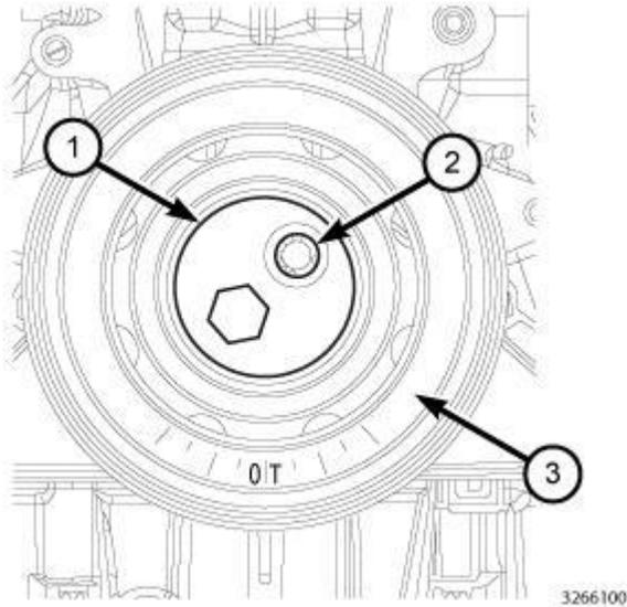
**Fig. 257: Vibration Damper Holder Tool, Vibration Damper & Bolts**
