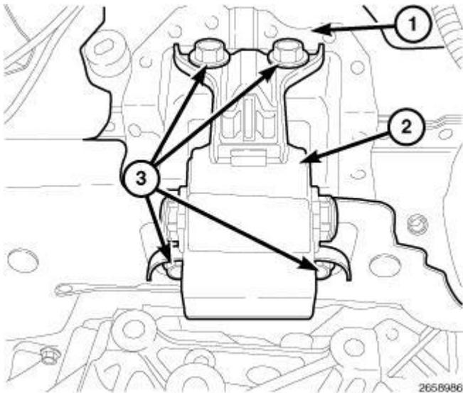
**Fig. 284: Left Side Engine Mount & Bolts**
