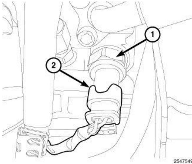
**Fig. 554: Identifying Fuel Temperature Sensor Harness Connector**
