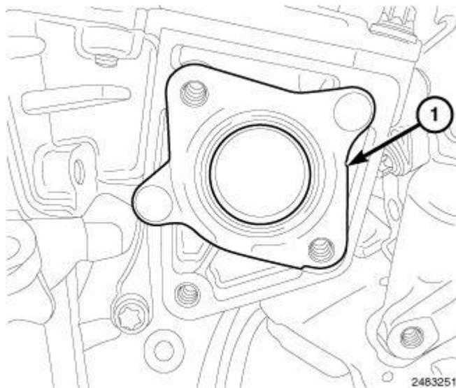
**Fig. 563: Installing/Removing EGR Tube Gasket Onto EGR Actuator**
