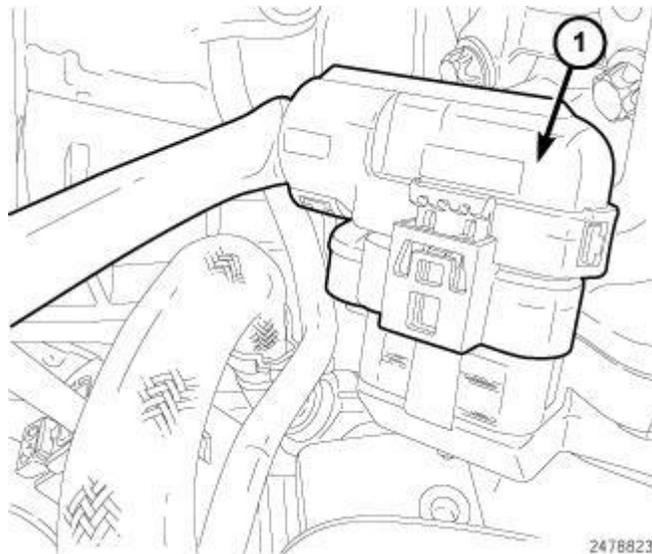
**Fig. 556: Identifying EGR Valve Harness Connector**
