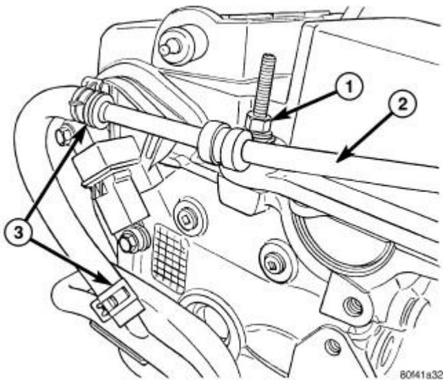
**Fig. 587: View Of Coolant Return Line Bracket**
