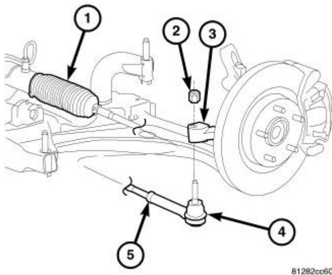
**Fig. 65: Removing/Installing Tie Rod Nut**
