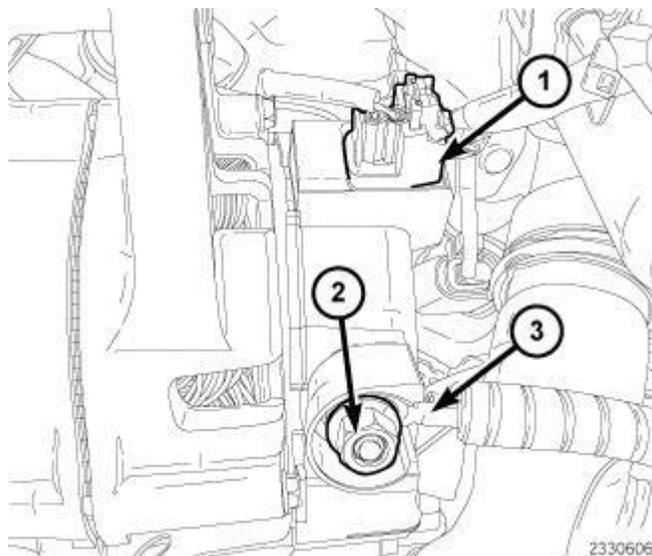
**Fig. 467: Battery Feed Wire, Generator Harness Connectors & Nut**
