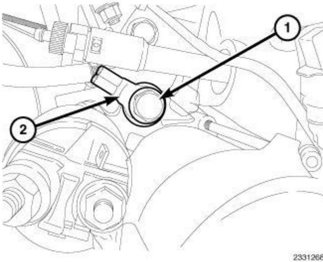
**Fig. 69: Battery Ground Cable At Engine Block**
