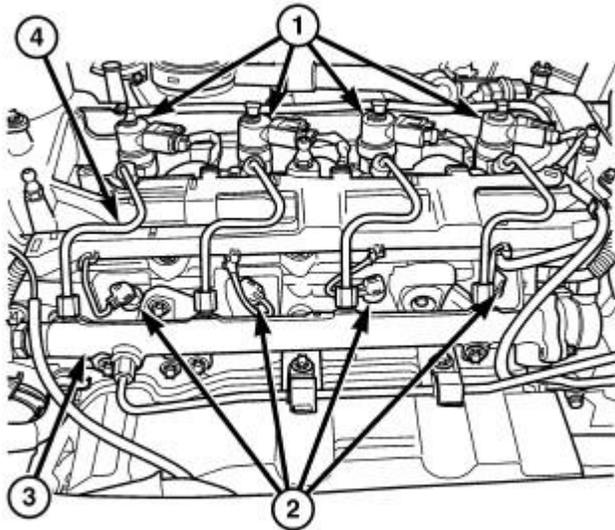
**Fig. 128: Fuel Injector And Glow Plug Locations**
