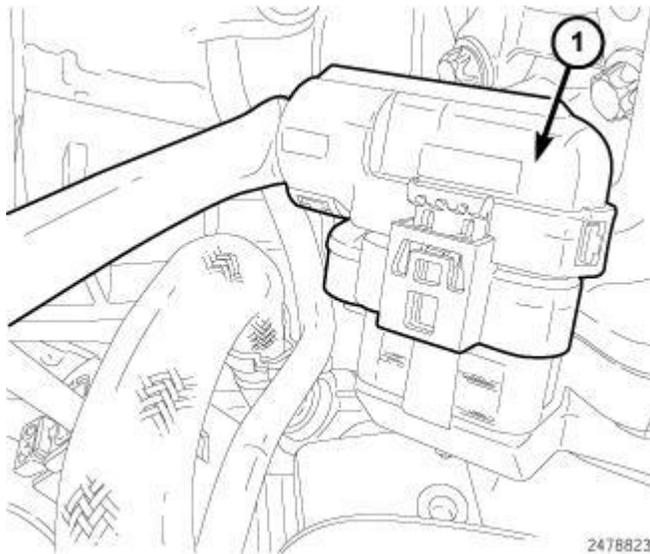
**Fig. 427: Identifying EGR Valve Harness Connector**
