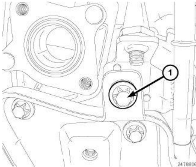
**Fig. 658: Vacuum Tube Bolt**
