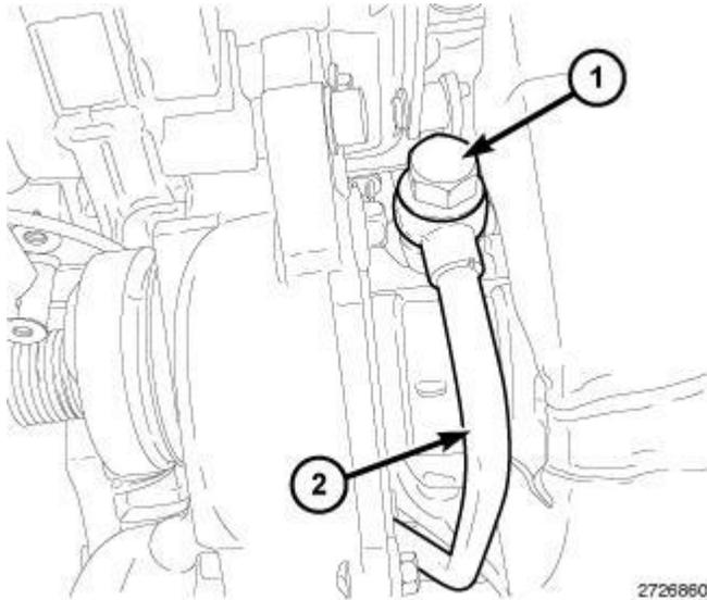
**Fig. 616: Oil Supply Line & Banjo Bolt At Turbocharger**
