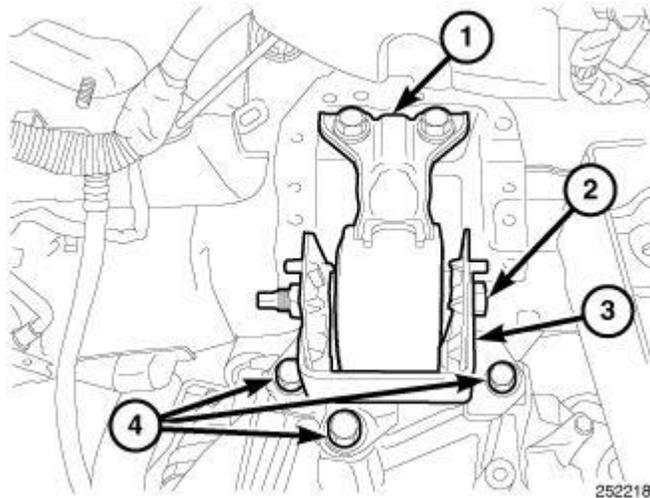
**Fig. 48: Left Engine Mount & Fasteners**
