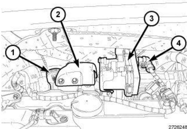
**Fig. 607: Identifying Catalytic Converter, Turbocharger Heat Shield, Catalytic Converter Band Clamp & Upstream Temperature Sensor**
