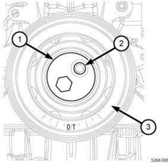
**Fig. 673: Vibration Damper Holder Tool, Vibration Damper & Bolts**
