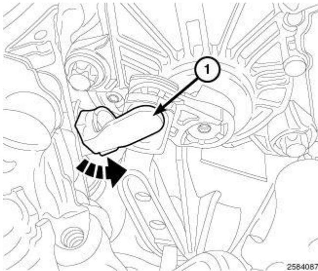
**Fig. 417: Installing Lock Clip On Swirl Valve Linkage**
