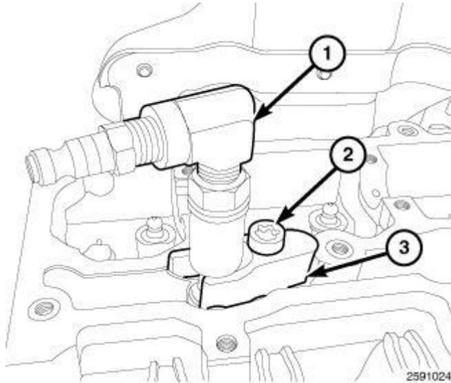
**Fig. 197: Compression Test Adapter, Tensioning Claw & Bolt**
