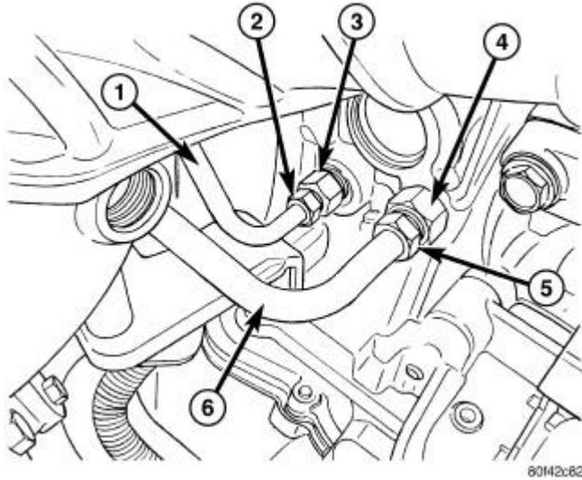
**Fig. 588: Oil Supply Line - Engine Block Fitting**
