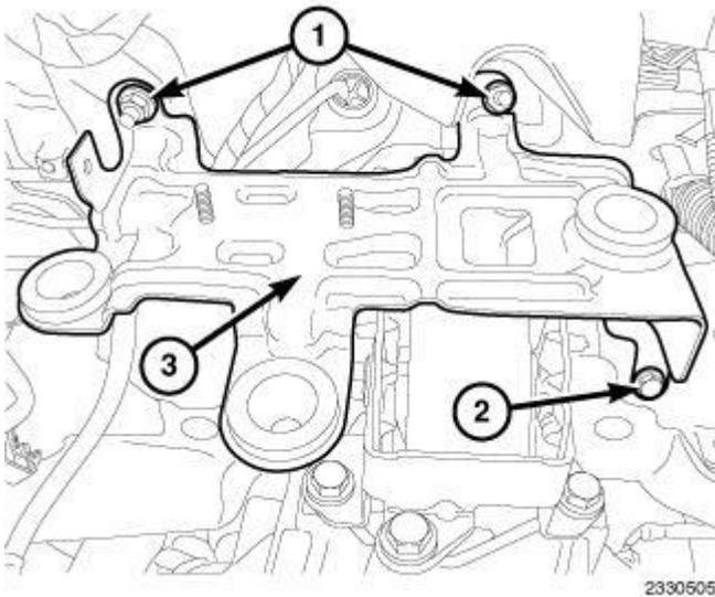
**Fig. 286: Air Cleaner Mounting Bracket, Nuts & Bolt**
