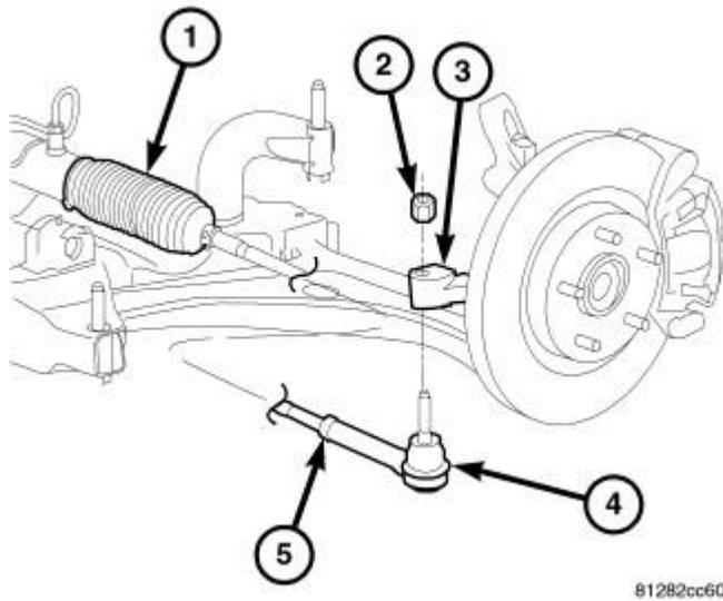
**Fig. 33: Removing/Installing Tie Rod Nut**
