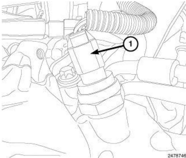
**Fig. 468: Identifying EGR Back Pressure Transducer Harness Connector**
