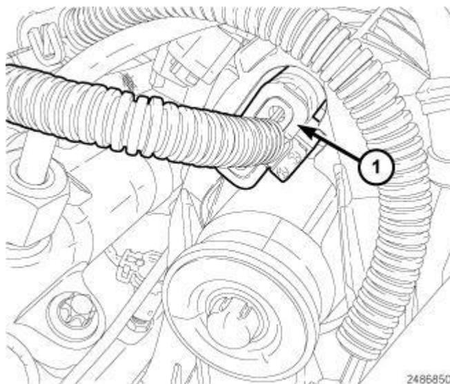
**Fig. 539: Swirl Valve Actuator Harness Connector**
