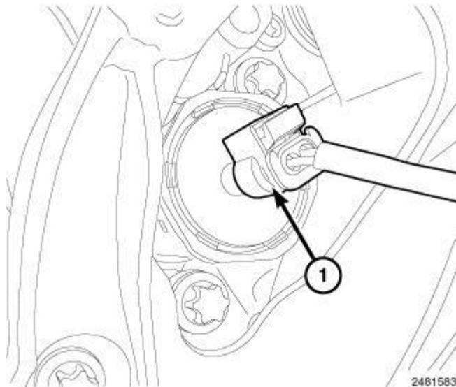
**Fig. 333: Piston Cooling Oil Control Valve Harness Connector**
