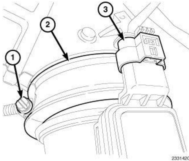
**Fig. 86: Mass Air Flow Sensor Harness Connector, Air Cleaner-To-Turbocharger Inlet Tube & Clamp**
