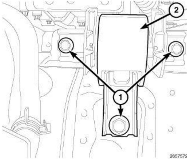
**Fig. 294: Engine Mount At Body Frame Rail & Bolts**
