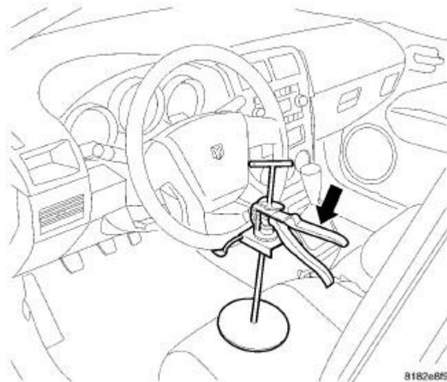
**Fig. 89: Steering Wheel Holding Tool**
