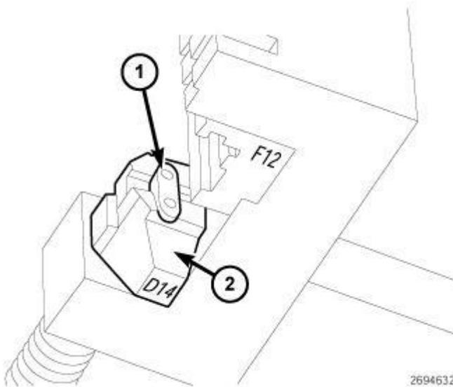
**Fig. 625: Placing Outer Plate Into Thrust Piece With Digit D14**
