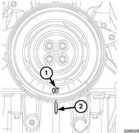
**Fig. 135: Crankshaft Alignment Timing Marks**
