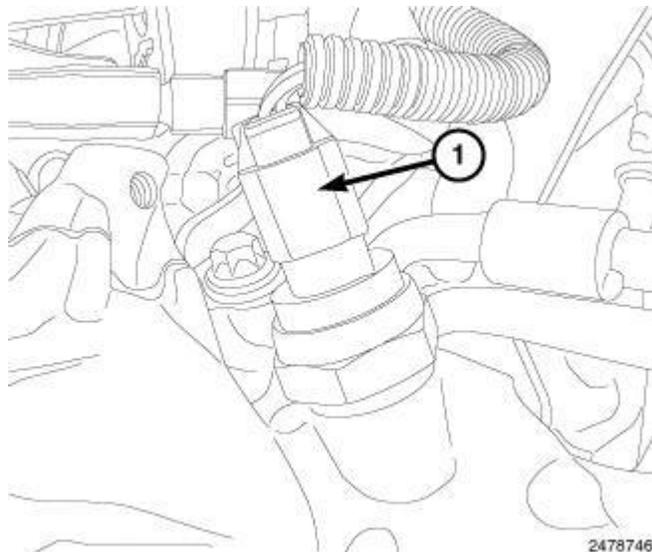
**Fig. 395: Identifying EGR Back Pressure Transducer Harness Connector**
