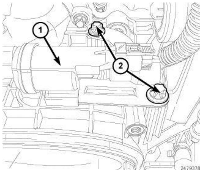
**Fig. 538: EGR Vacuum Solenoid & Bolts**
