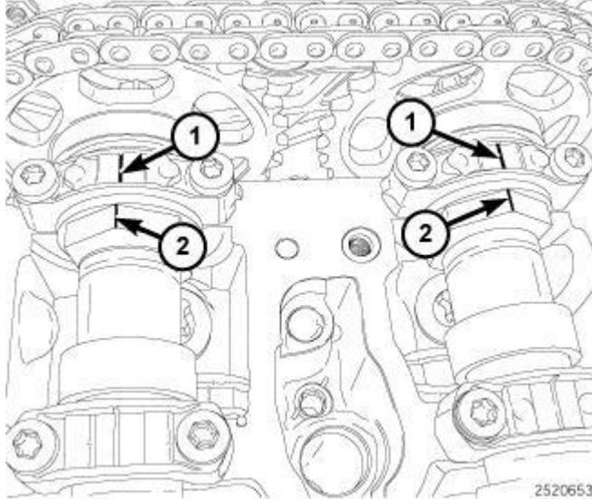
**Fig. 675: Ensuring Camshaft Mark Is Aligned With Bearing Cap Mark**
