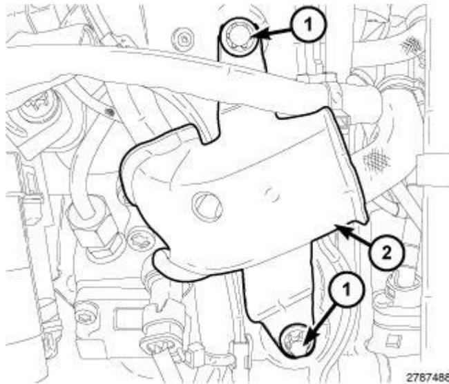
**Fig. 657: Identifying Bolts & Heat Shield**
