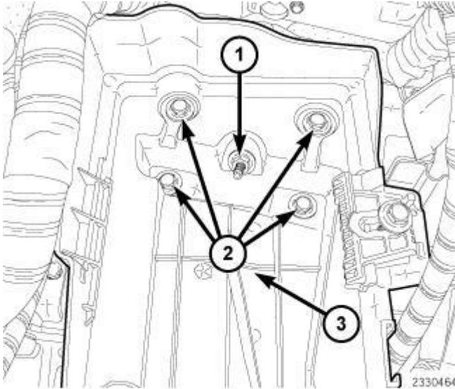
**Fig. 82: Battery Tray, Nut & Retaining Bolts**
