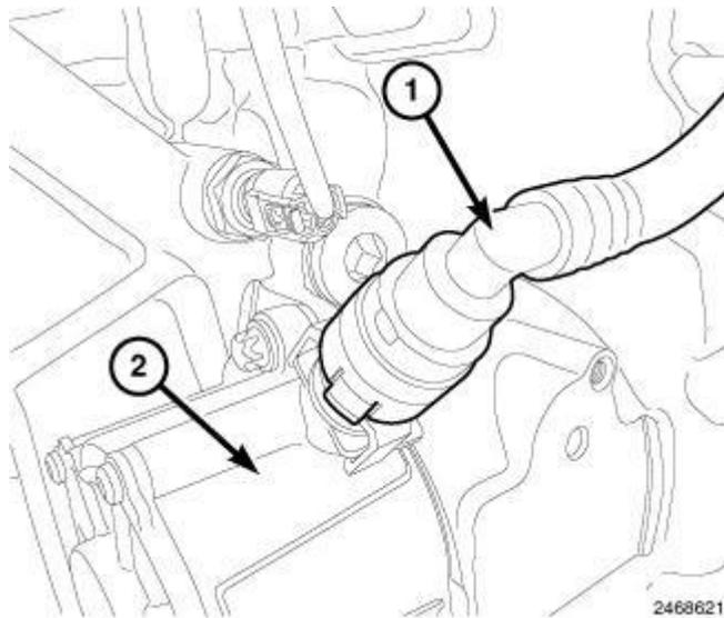
**Fig. 373: Vacuum Hose At Vacuum Pump**
