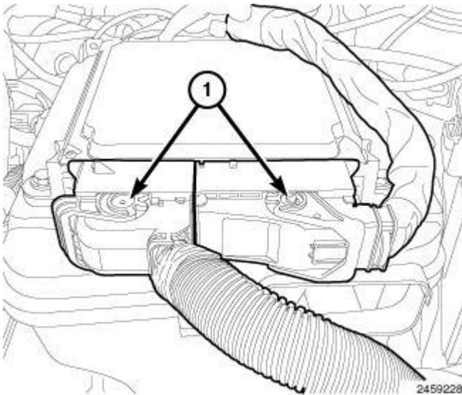
**Fig. 111: PCM Harness Connectors**
