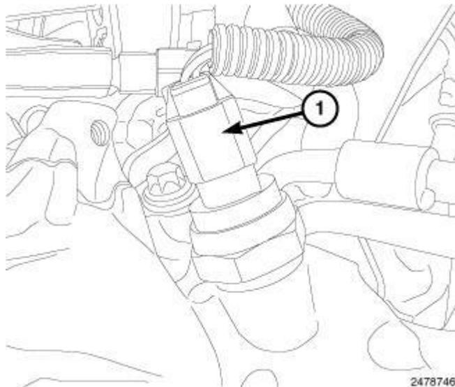
**Fig. 438: Identifying EGR Back Pressure Transducer Harness Connector**
