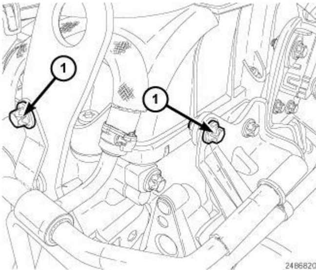
**Fig. 668: Upper Fuel Line Bracket Bolts**
