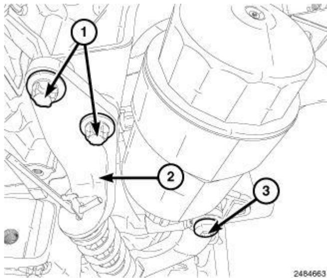
**Fig. 537: Accessory Drive Belt Tensioner & Bolts**
