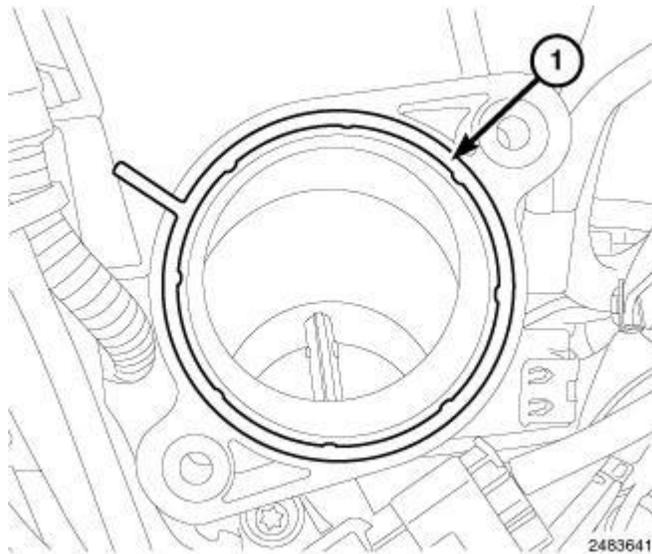
**Fig. 433: Installing/Removing EGR Tube Gasket Onto Mixing Chamber**
