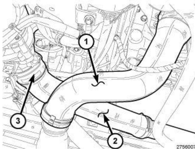
**Fig. 577: Identifying Front Upper & Lower Air Charge Hose**
