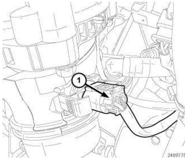
**Fig. 486: Identifying Charge Air Temperature Sensor Connectors**
