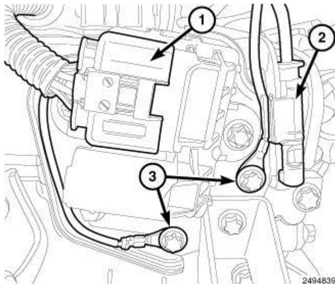
**Fig. 183: Identifying Glow Plug Module Harness Connector, Bolts & Turbocharger Exhaust Temperature Sensor Harness Connector**
