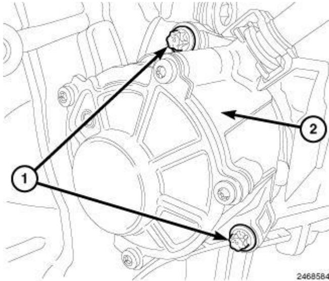
**Fig. 356: Vacuum Pump & Bolts**
