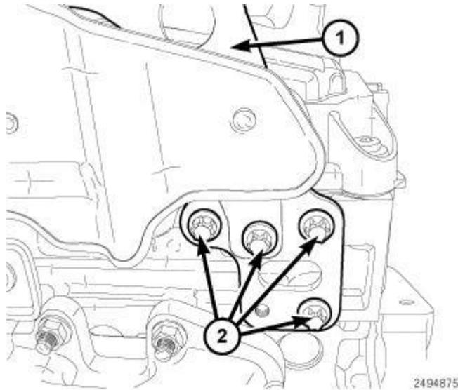
**Fig. 176: Engine Lifting Eye & Bolts**
