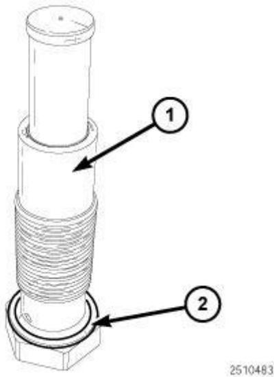
**Fig. 700: Sealing Washer & Timing Chain Tensioner**
