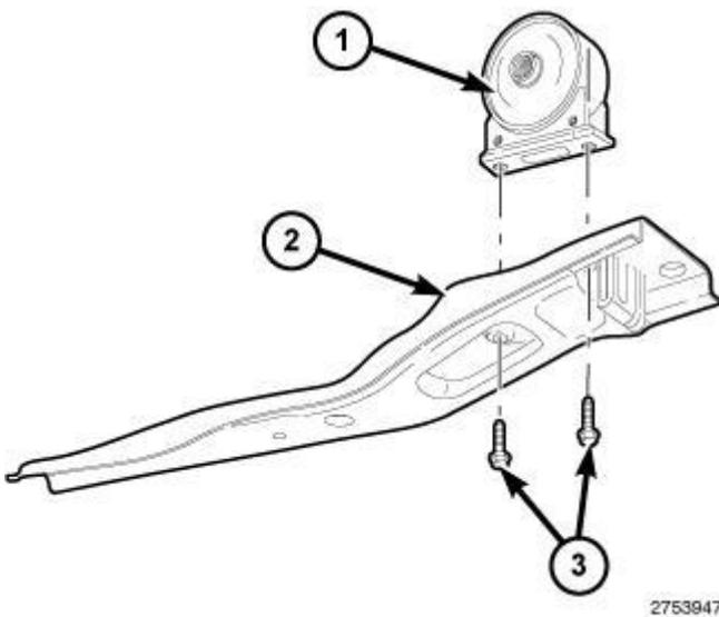
**Fig. 272: Front Engine Mount**
