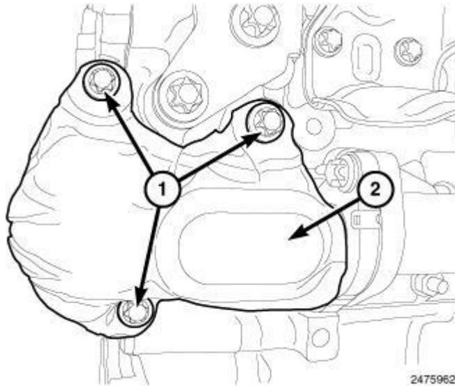
**Fig. 702: EGR Pipe Heat Shield & Bolts**
