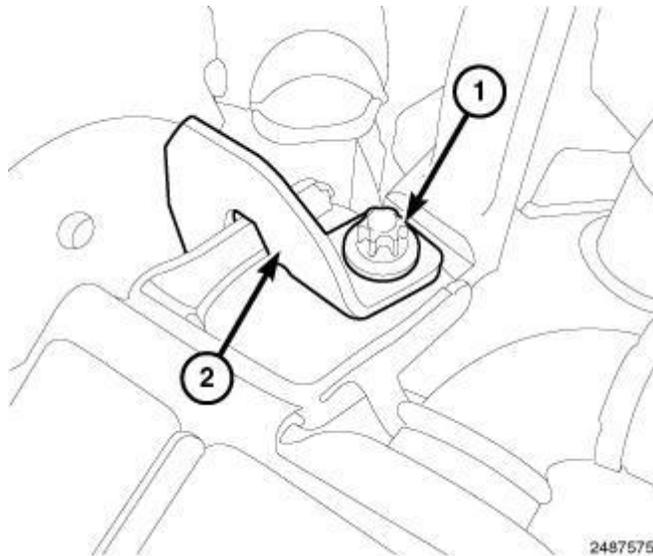
**Fig. 406: Upper EGR Cooler Bolt & Bracket**
