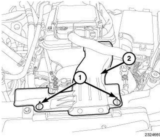
**Fig. 572: Quarter Turn Lock Tabs & Air Inlet Duct**
