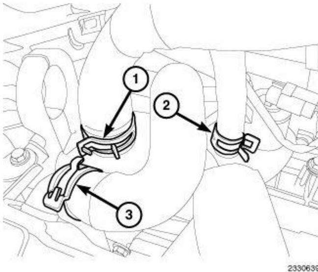
**Fig. 71: Heater Hoses At Engine**
