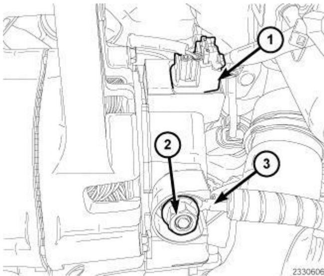
**Fig. 73: Battery Feed Wire, Generator Harness Connectors & Nut**
