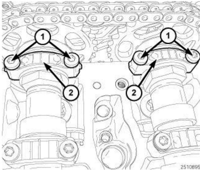
**Fig. 704: No. 1 Camshaft Bearing Caps & Bolts**
