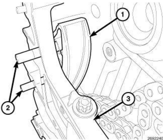
**Fig. 682: Timing Chain Guide, Guide Pins & Cylinder Head**
