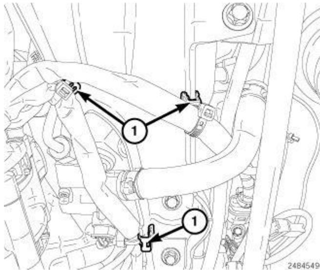
**Fig. 429: Wire Harness Retainers**
