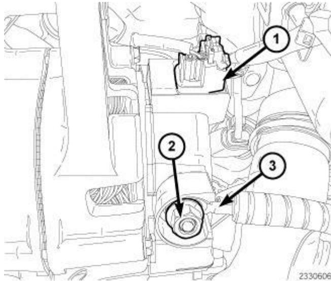
**Fig. 570: Battery Feed Wire, Generator Harness Connectors & Nut**
