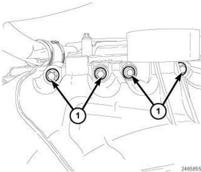
**Fig. 255: Front Oil Pan Bolts**
