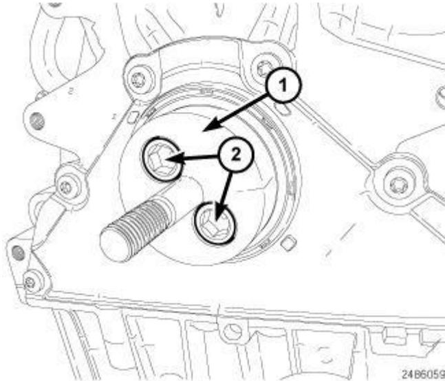
**Fig. 260: Front Crankshaft Seal Adapter & Bolts**
