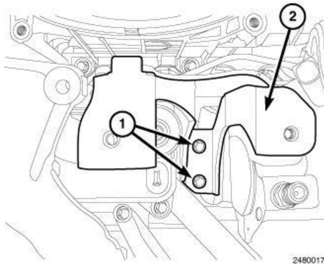
**Fig. 337: Intake Manifold Support Bracket & Bolts**
