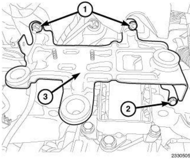
**Fig. 281: Air Cleaner Mounting Bracket, Nuts & Bolt**
