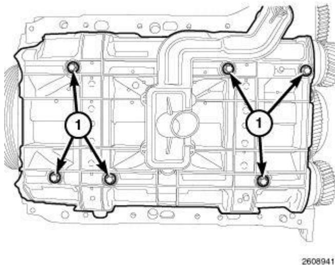
**Fig. 229: Oil Pump Pickup Bolts**
