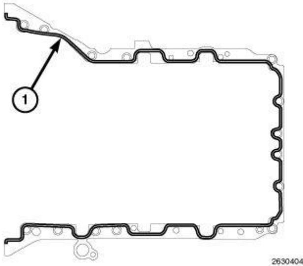
**Fig. 230: Applying Engine Sealant RTV Onto Oil Pan Mating Surface**
