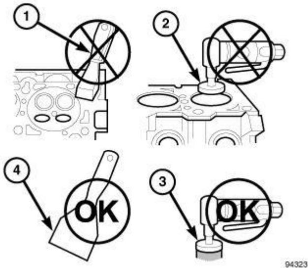
**Fig. 4: Proper Tool Usage For Surface Preparation**
