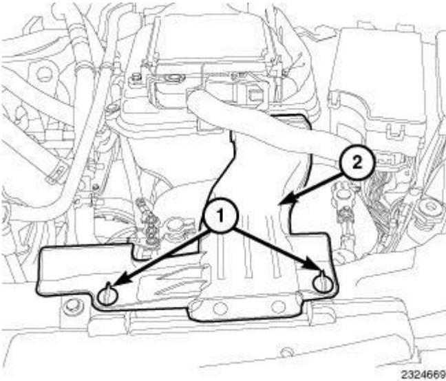
**Fig. 246: Quarter Turn Lock Tabs & Air Inlet Duct**
