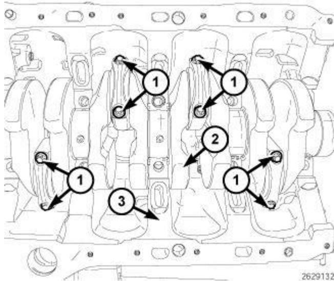
**Fig. 212: Identifying Crankshaft, Engine Block, Connecting Rod Bearing Caps & Bolts**
