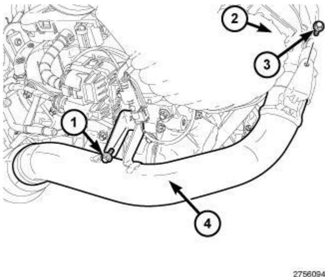
**Fig. 579: Rear Air Charge Tube & Bolts**
