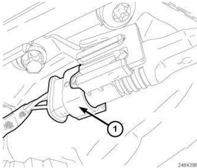
**Fig. 470: Knock Sensor Harness Connector**
