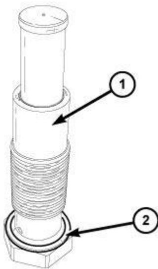
**Fig. 684: Sealing Washer & Timing Chain Tensioner**
