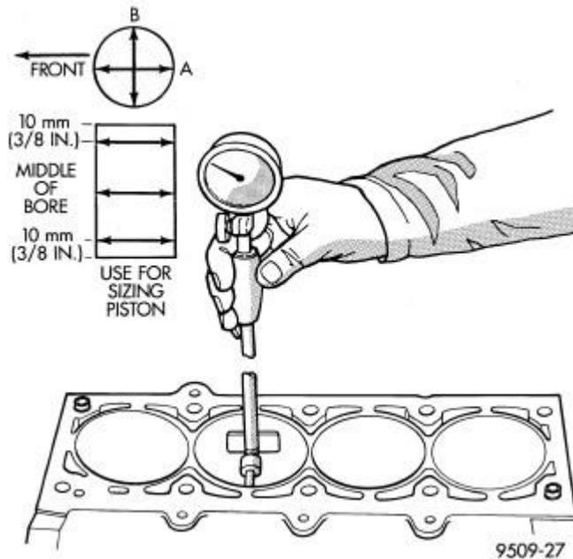
**Fig. 242: Checking Cylinder Bore Size**
