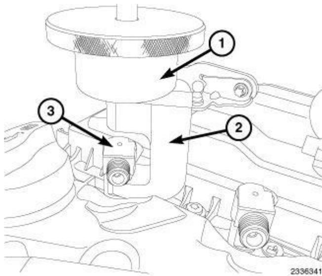
**Fig. 172: Puller, Extraction Claw & Fuel Injector**
