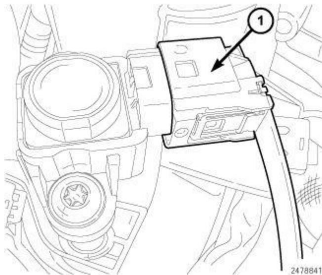
**Fig. 459: Boost Pressure Sensor Harness Connector**
