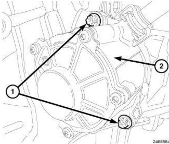
**Fig. 239: Vacuum Pump & Bolts**
