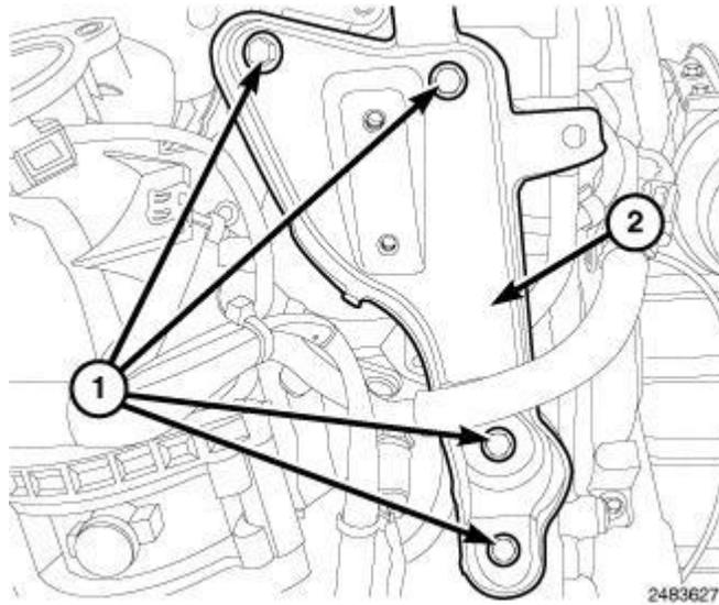
**Fig. 457: Identifying Bolts & EGR Support Bracket**
