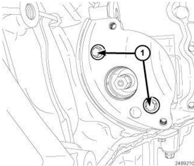
**Fig. 357: Oil Pump Retaining Bolts**
