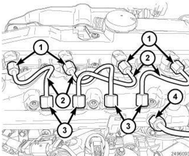
**Fig. 179: Identifying Fuel Injectors, High Pressure Fuel Tubes, Fuel Rail & High Pressure Feed Line**
