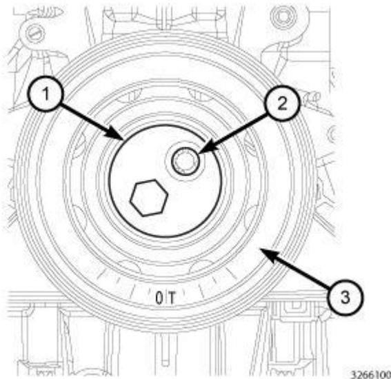
**Fig. 249: Vibration Damper Holder Tool, Vibration Damper & Bolts**
