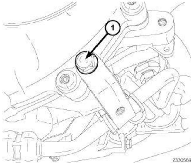
**Fig. 222: Power Steering Line Support Bracket Retaining Bolt**
