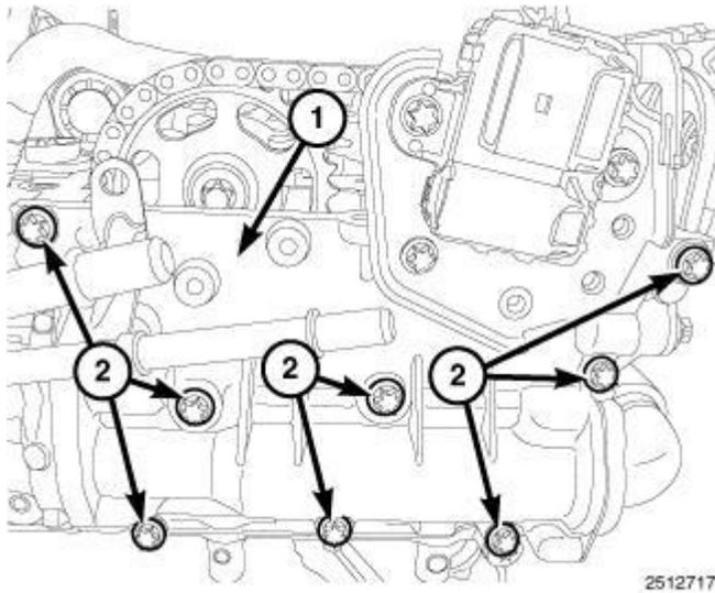
**Fig. 645: Timing Chain Upper Cover & Bolts**
