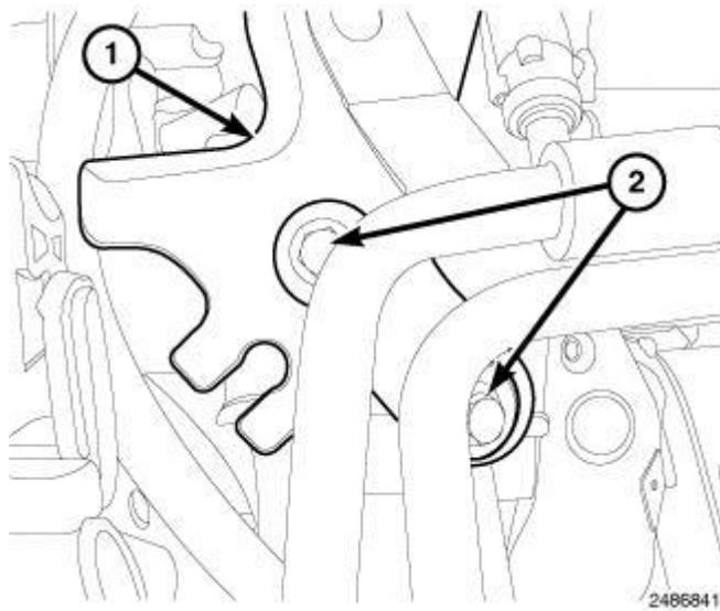
**Fig. 412: Engine Lifting Eye & Bolts**
