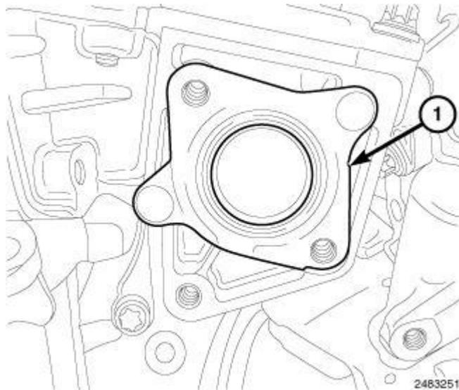
**Fig. 519: Installing/Removing EGR Tube Gasket Onto EGR Actuator**
