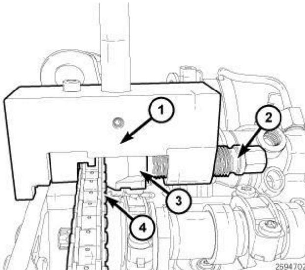
**Fig. 628: Riveting Press Tool, Timing Chain Thrust Spindle, Thrust Piece & Timing Chain**
