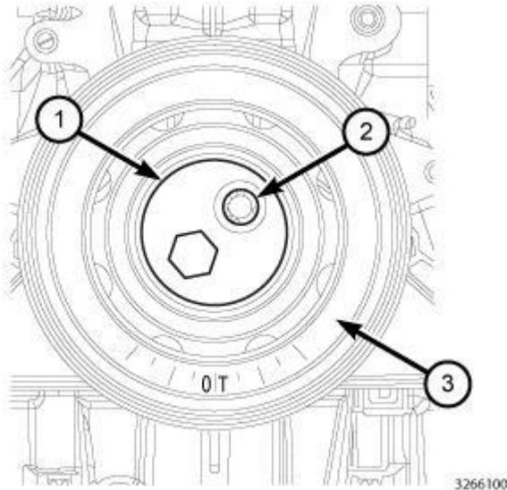
**Fig. 139: Vibration Damper Holder Tool, Vibration Damper & Bolts**
