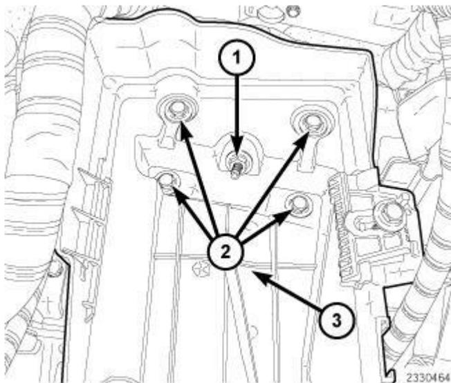
**Fig. 280: Battery Tray, Nut & Retaining Bolts**
