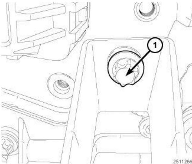
**Fig. 632: Bolt Securing CAC Tube To Glow Plug Module**
