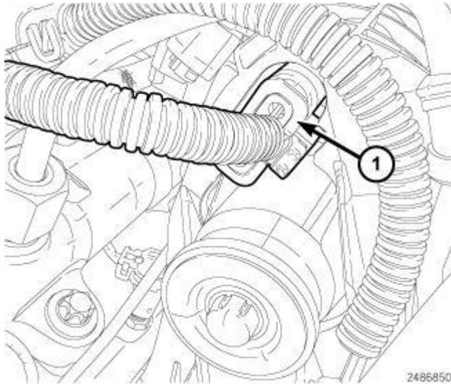
**Fig. 494: Swirl Valve Actuator Harness Connector**
