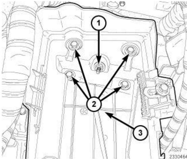
**Fig. 16: Battery Tray, Nut & Retaining Bolts**
