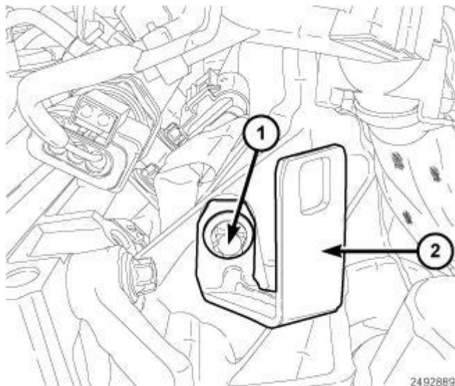
**Fig. 534: Wire Harness Support Bracket & Bolts**
