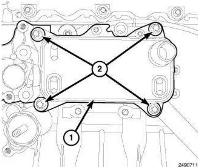
**Fig. 308: Oil Cooler Adapter & Bolts**
