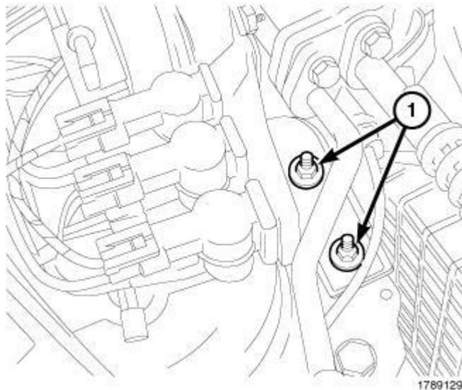
**Fig. 597: Nuts Securing Solenoid Mounting Bracket**
