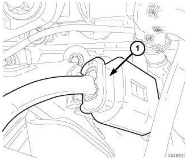
**Fig. 555: Identifying Fuel Quantity Control Valve Harness Connector**
