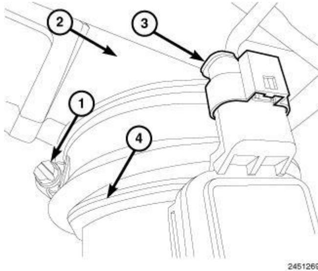
**Fig. 104: Mass Air Flow Sensor, Harness Connector, Turbocharger Inlet Tube & Clamp**
