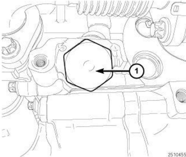
**Fig. 685: Timing Chain Tensioner**
