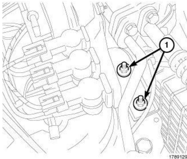
**Fig. 600: Nuts Securing Solenoid Mounting Bracket**
