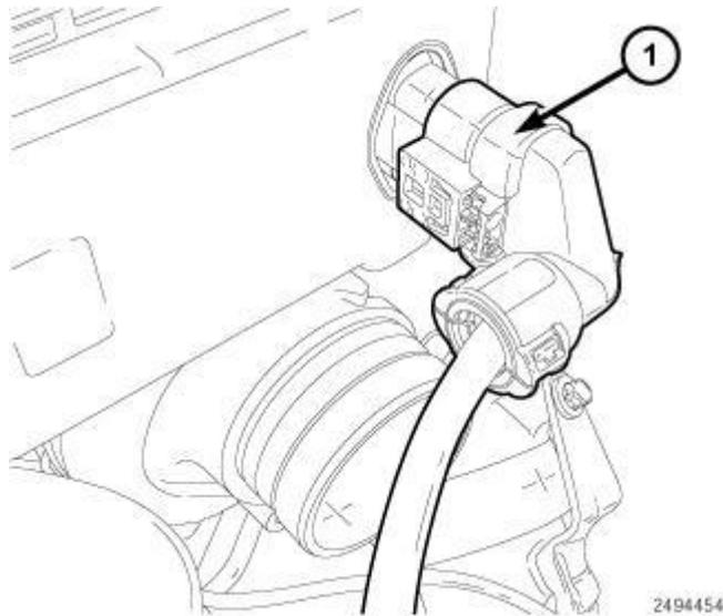
**Fig. 164: Turbocharger Actuator Harness Connector**
