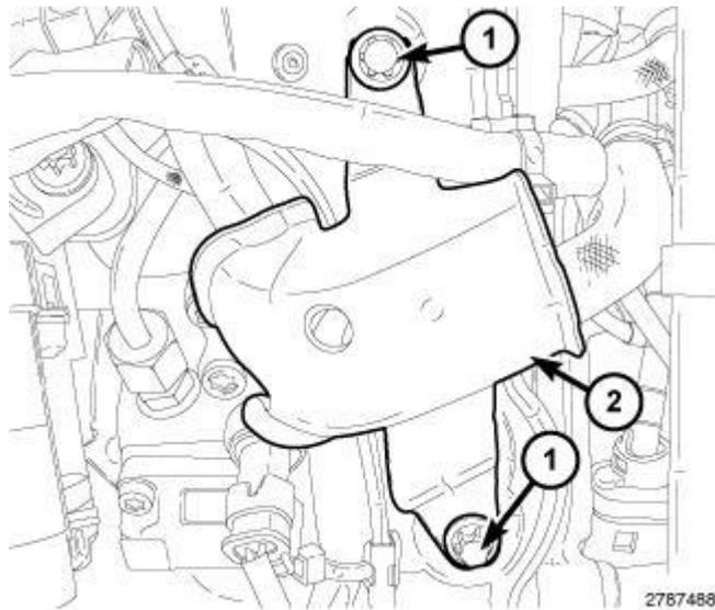
**Fig. 430: Identifying Bolts & Heat Shield**
