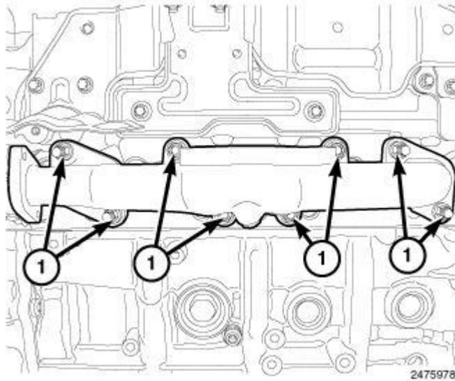
**Fig. 130: Exhaust Manifold Retaining Nuts**
