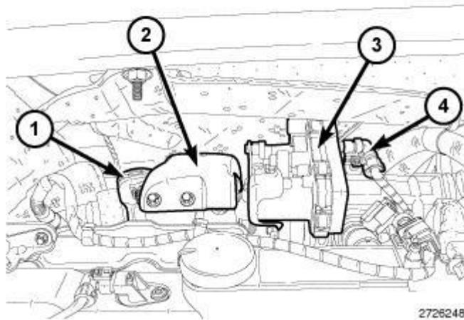
**Fig. 619: Identifying Catalytic Converter, Turbocharger Heat Shield, Catalytic Converter Band Clamp & Upstream Temperature Sensor**
