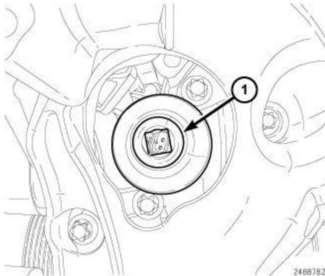
**Fig. 304: Removing/Installing Piston Cooling Oil Control Valve Using Shift Valve Socket**
