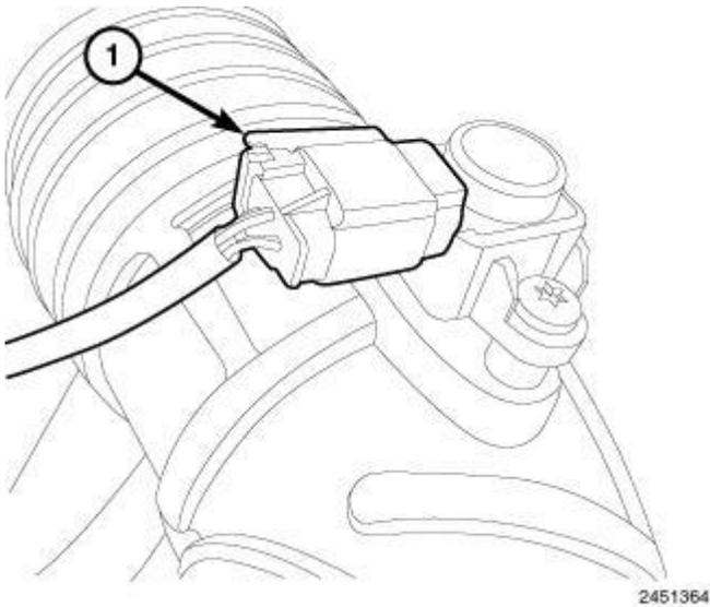
**Fig. 106: Intake Air Temperature/Boost Pressure Sensor**
