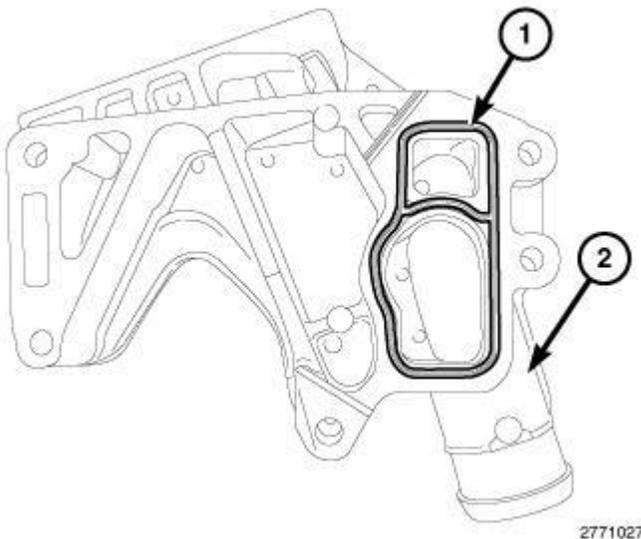
**Fig. 295: Engine Mount Carrier Bracket & Gasket**
