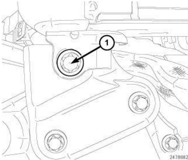
**Fig. 641: Lower EGR Cooler Bolt**
