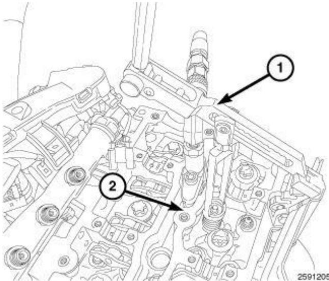
**Fig. 205: Valve Spring Compressor & Cylinder Head**
