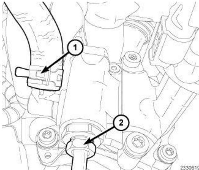
**Fig. 235: Power Steering Supply Line & Feed Line**
