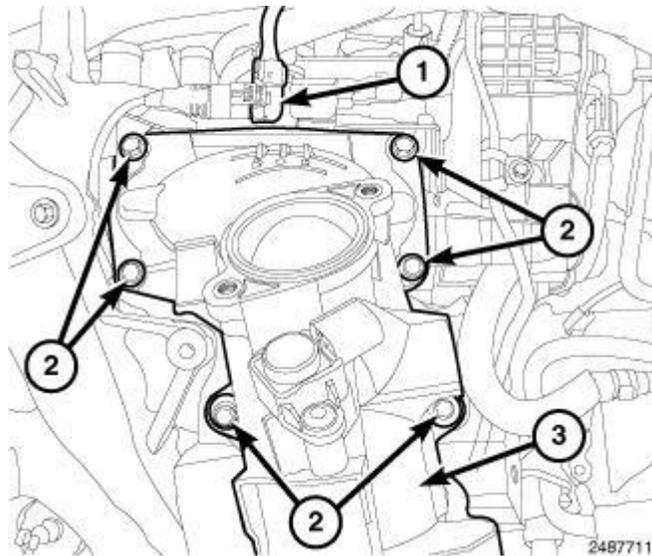
**Fig. 508: Knock Sensor Electrical Connector, Mixing Chamber & Bolts**
