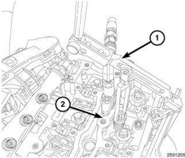
**Fig. 199: Valve Spring Compressor & Cylinder Head**
