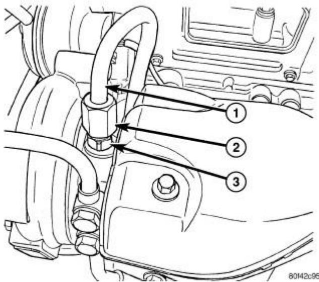
**Fig. 593: Oil Supply Line - Turbocharger Fitting**
