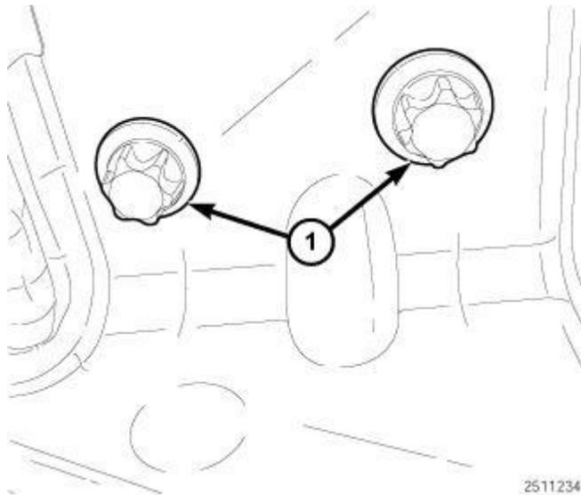
**Fig. 665: CAC Tube And Bracket Assembly Bolts**
