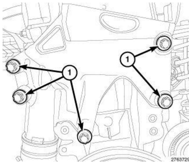
**Fig. 291: Engine Mount Carrier Bracket & Bolts**
