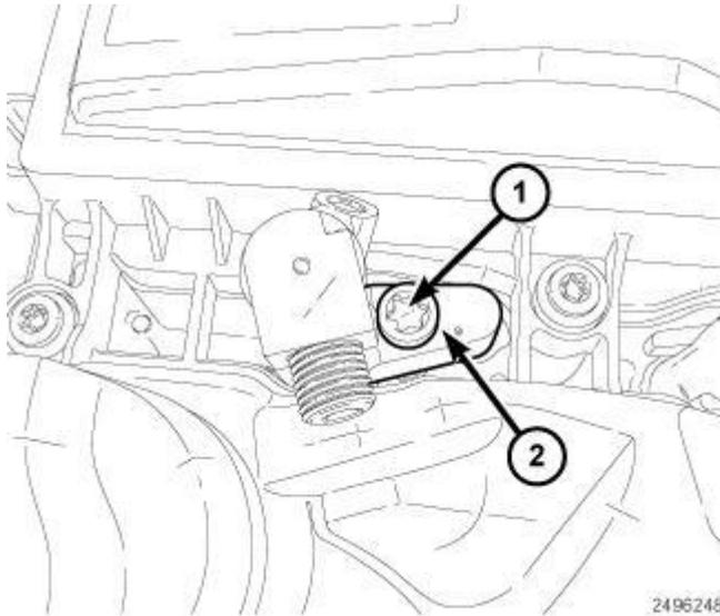
**Fig. 178: Identifying Bolt & Clamping Claw**
