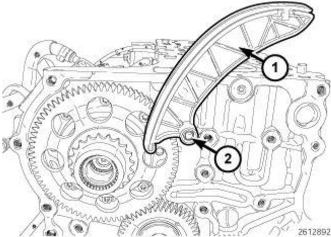
**Fig. 689: Tensioning Rail & Pin**
