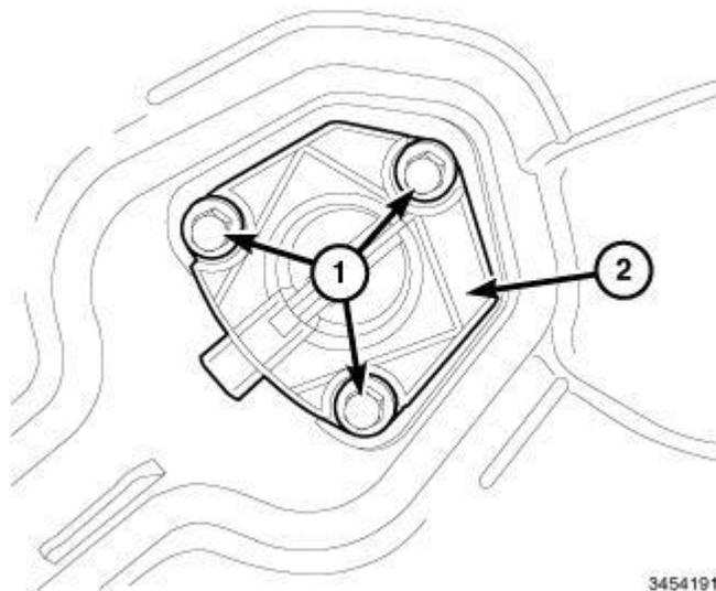
**Fig. 390: Oil Level Switch & Bolts**
