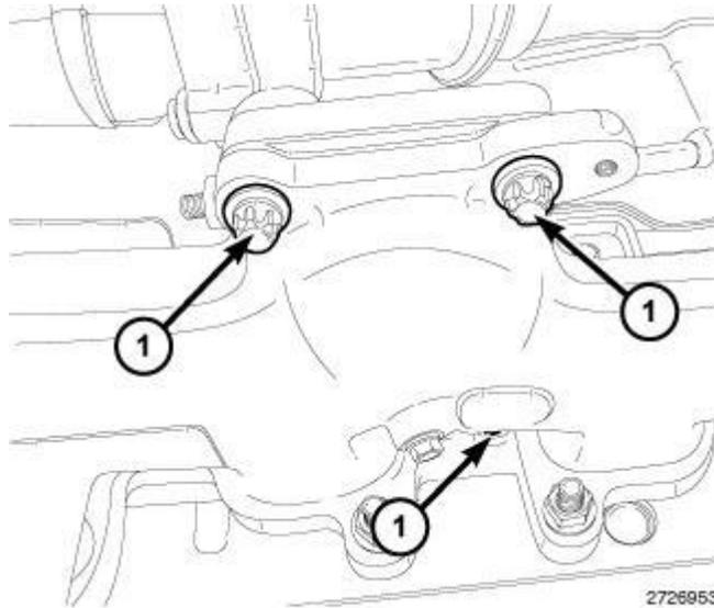
**Fig. 612: Turbocharger-To-Exhaust Manifold Mounting Bolts**
