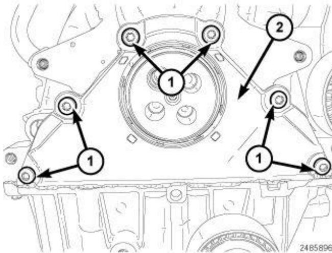
**Fig. 254: Front Oil Seal Carrier & Bolts**
