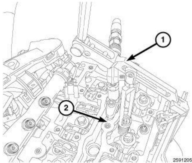
**Fig. 198: Valve Spring Compressor & Cylinder Head**
