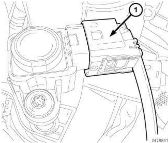
**Fig. 552: Boost Pressure Sensor Harness Connector**
