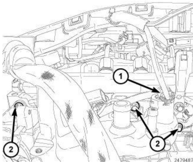
**Fig. 500: Coolant Temp Sensor & Cooling Manifold Bolts**
