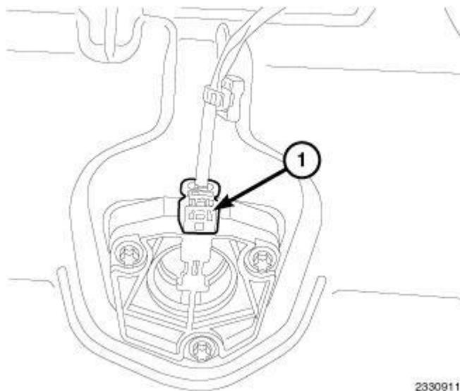
**Fig. 232: Oil Level Switch Wire Harness Connector**
