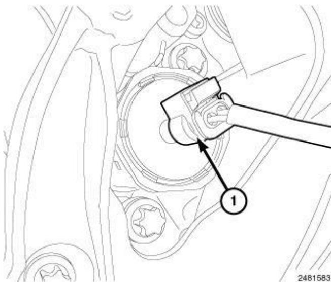
**Fig. 303: Piston Cooling Oil Control Valve Harness Connector**
