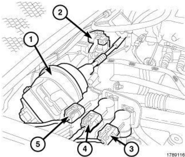
**Fig. 596: Wastegate Solenoid & Electrical Connectors**
