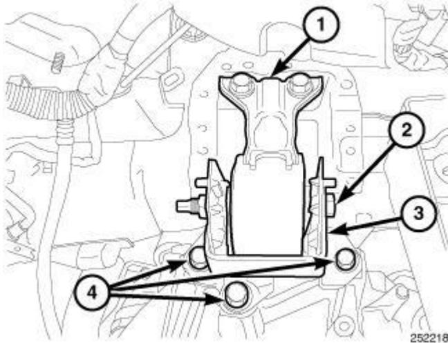
**Fig. 51: Left Engine Mount & Fasteners**
