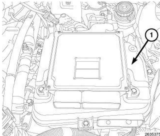
**Fig. 105: Air Cleaner Housing Assembly**
