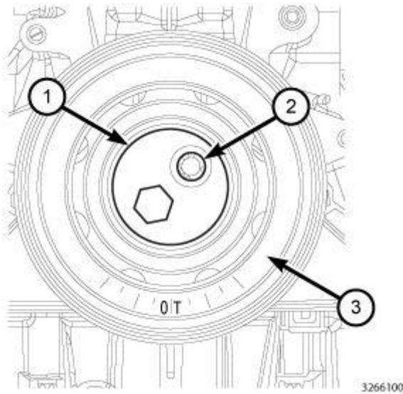
**Fig. 262: Vibration Damper Holder Tool, Vibration Damper & Bolts**
