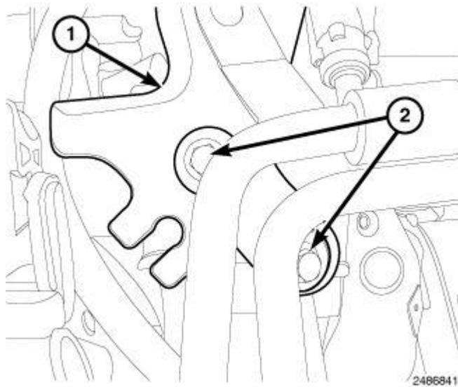
**Fig. 419: Engine Lifting Eye & Bolts**
