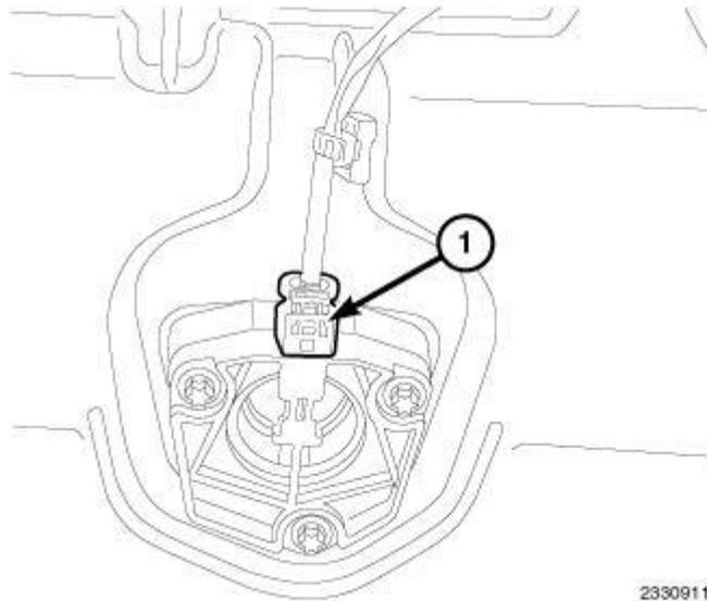
**Fig. 350: Oil Level Switch Wire Harness Connector**
