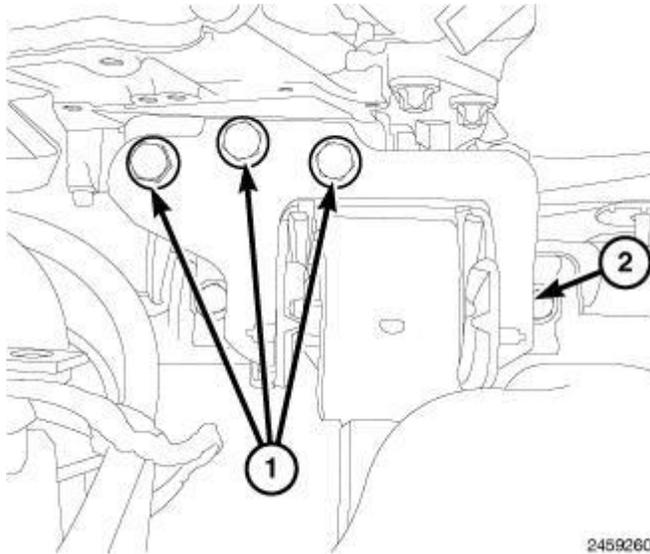
**Fig. 47: Engine Mount Through Bolt & Right Engine Mount Bolts**
