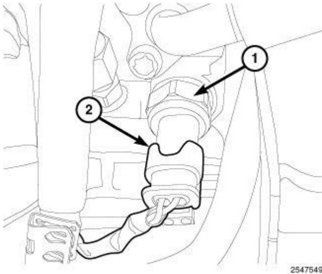
**Fig. 481: Identifying Fuel Temperature Sensor Harness Connector**
