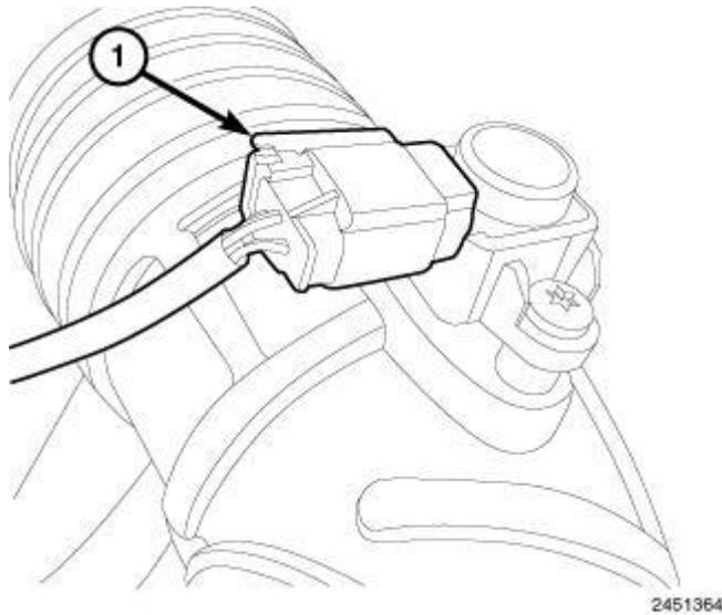
**Fig. 116: Intake Air Temperature/Boost Pressure Sensor**
