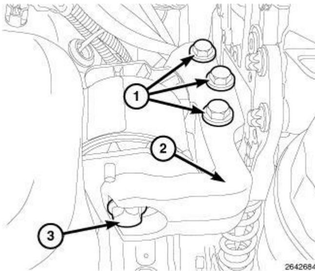
**Fig. 301: Engine Mount, Bracket & Through Bolt**
