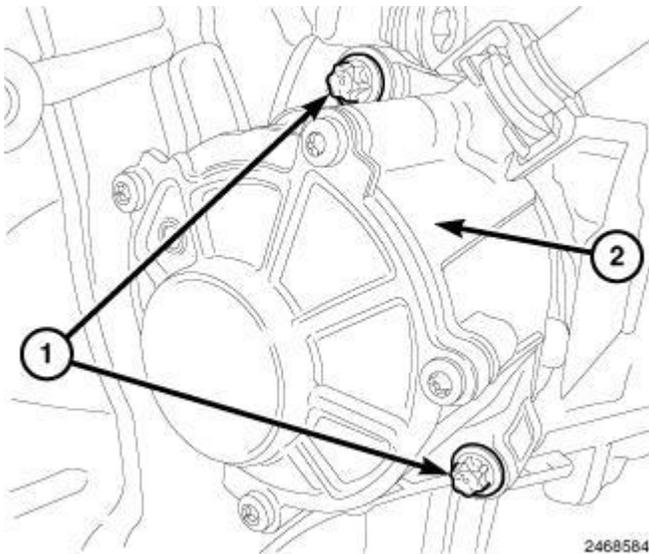
**Fig. 361: Vacuum Pump & Bolts**
