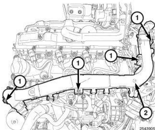
**Fig. 498: Lock Tabs & Engine Wire Harness**
