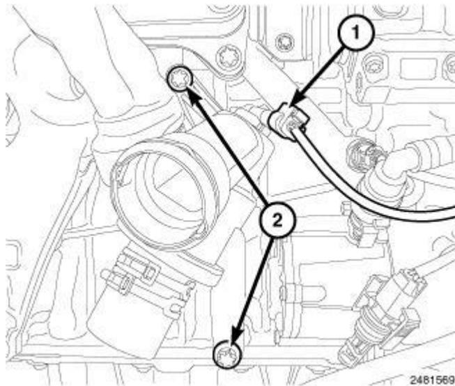
**Fig. 503: Identifying Thermostat Heater Connector & Upper Thermostat Housing Bolt**
