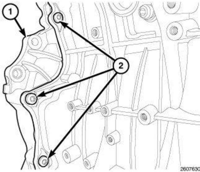
**Fig. 671: Locating Bolts At Backside Of Timing Cover**
