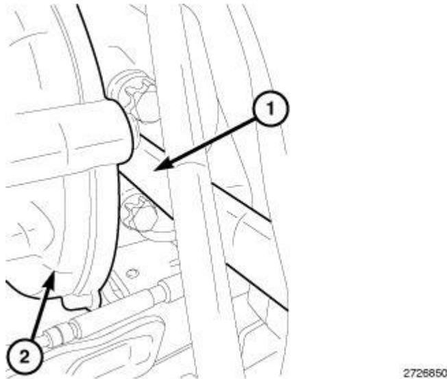
**Fig. 609: Oil Return Line At Turbocharger**
