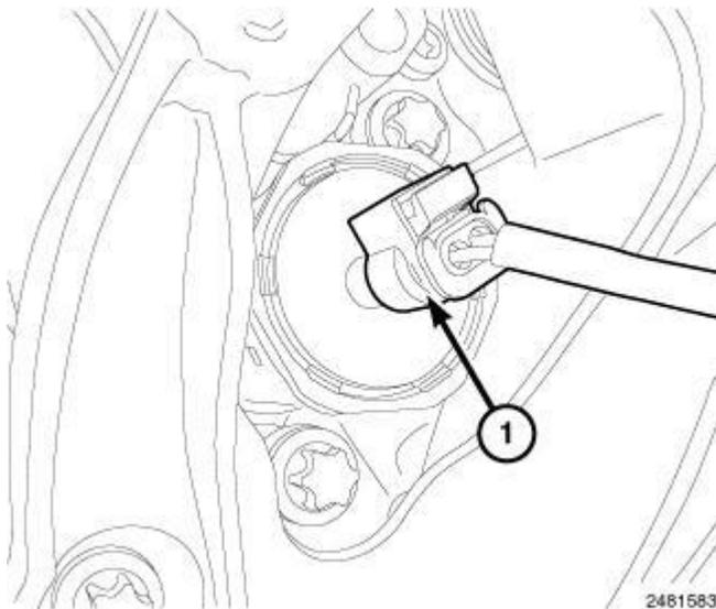
**Fig. 307: Piston Cooling Oil Control Valve Harness Connector**
