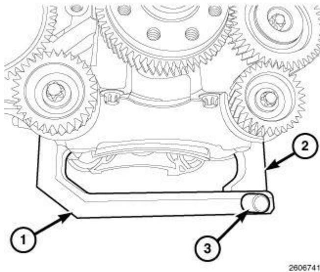
**Fig. 363: Removing/Installing Locking Pin At Balance Shaft Lock Tool Halves**
