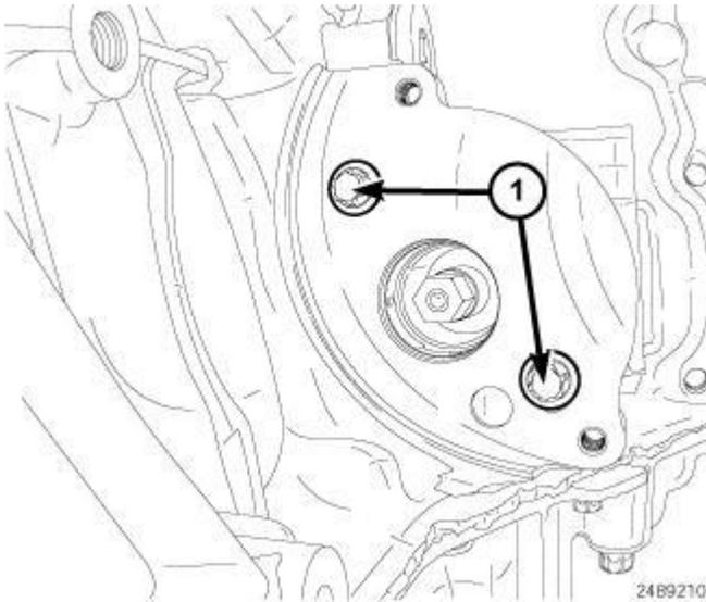
**Fig. 360: Oil Pump Retaining Bolts**
