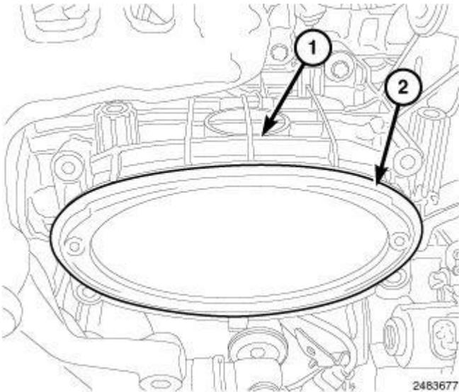
**Fig. 507: Intake Manifold & O-Ring Seal**
