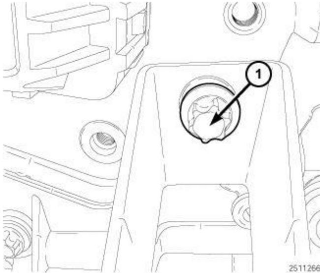
**Fig. 692: Bolt Securing CAC Tube To Glow Plug Module**
