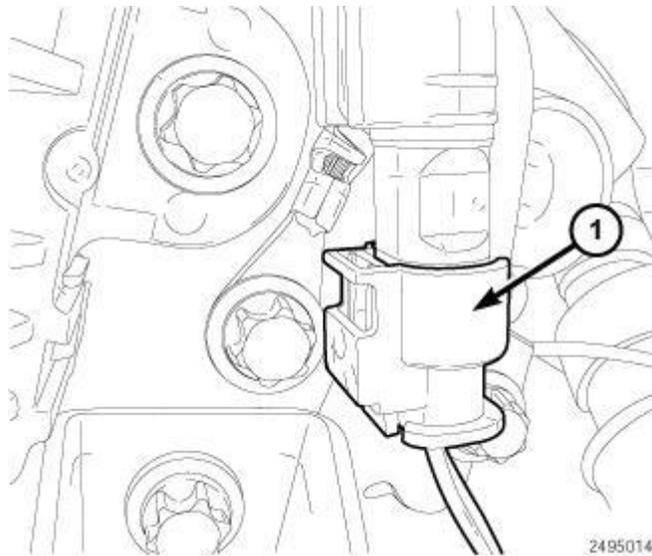
**Fig. 184: Turbocharger Exhaust Temperature Sensor Harness Connector**
