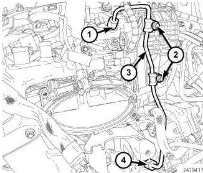
**Fig. 493: Identifying Fuel Rail, Bolts, High Pressure Fuel Tube & Pump**
