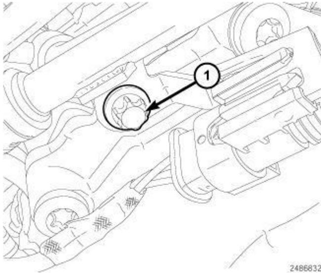
**Fig. 420: Lower Fuel Line Bracket Bolt**
