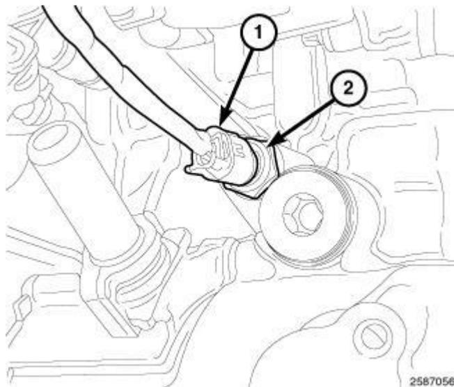
**Fig. 374: Oil Temperature Sensor Harness Connector & Sensor**
