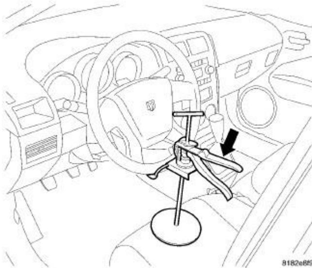
**Fig. 14: Steering Wheel Holding Tool**
