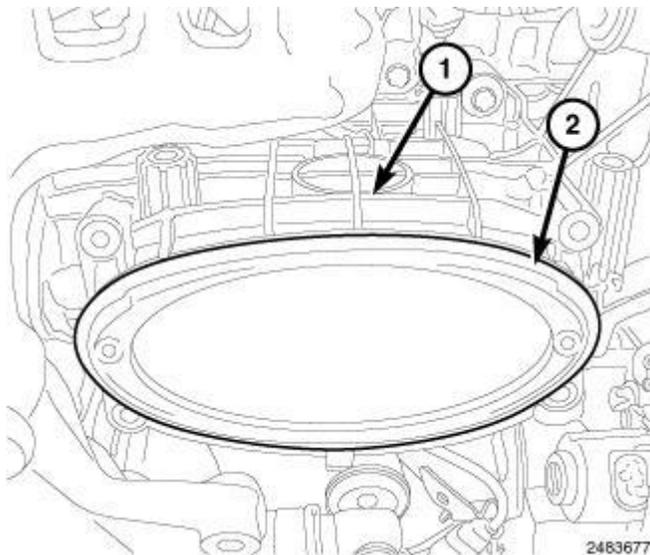
**Fig. 541: Intake Manifold & O-Ring Seal**
