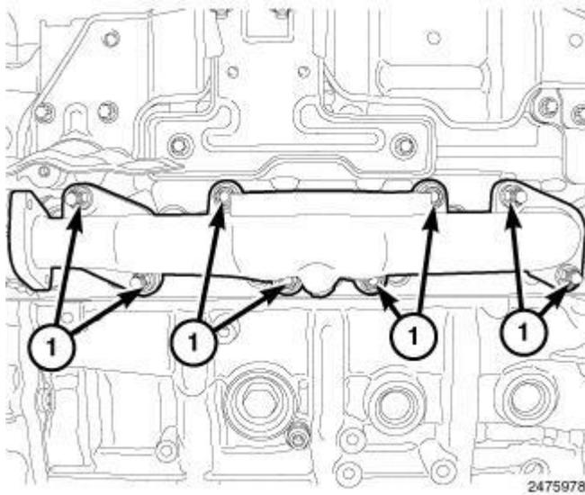
**Fig. 442: Exhaust Manifold Retaining Nuts**
