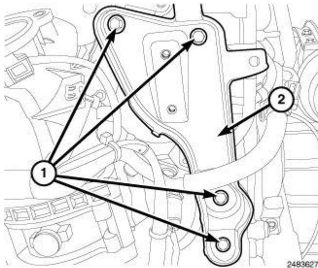
**Fig. 378: Identifying Bolts & EGR Support Bracket**
