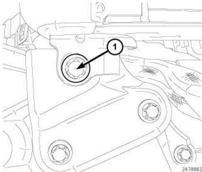
**Fig. 407: Lower EGR Cooler Bolt**
