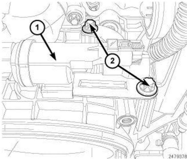
**Fig. 495: EGR Vacuum Solenoid & Bolts**
