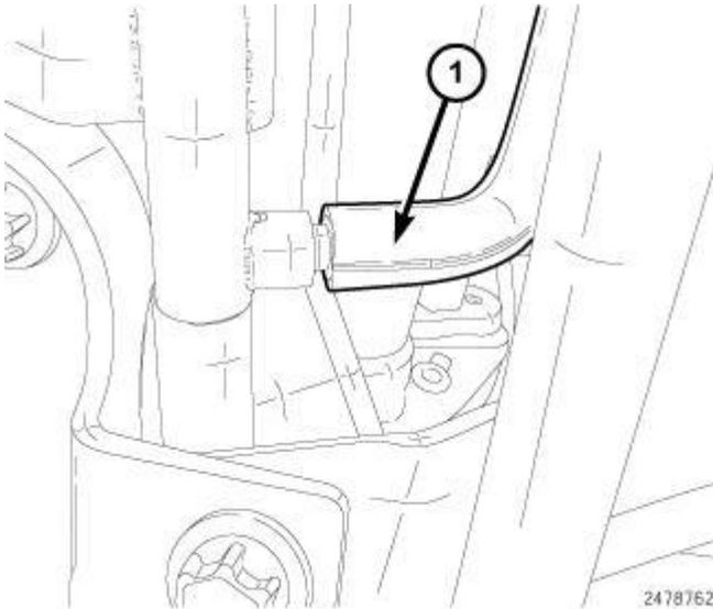
**Fig. 383: Vacuum Supply Line At EGR Solenoid**
