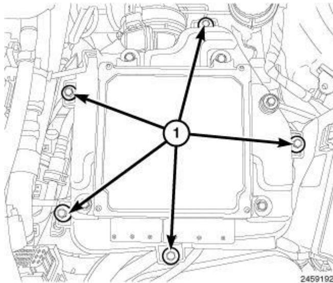
**Fig. 97: Air Cleaner Cover Screws**
