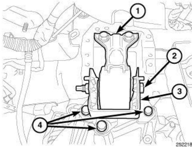
**Fig. 282: Left Engine Mount & Fasteners**
