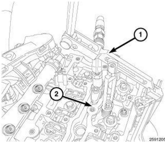
**Fig. 202: Valve Spring Compressor & Cylinder Head**
