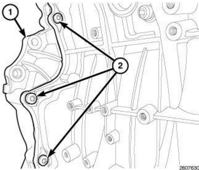
**Fig. 646: Locating Bolts At Backside Of Timing Cover**
