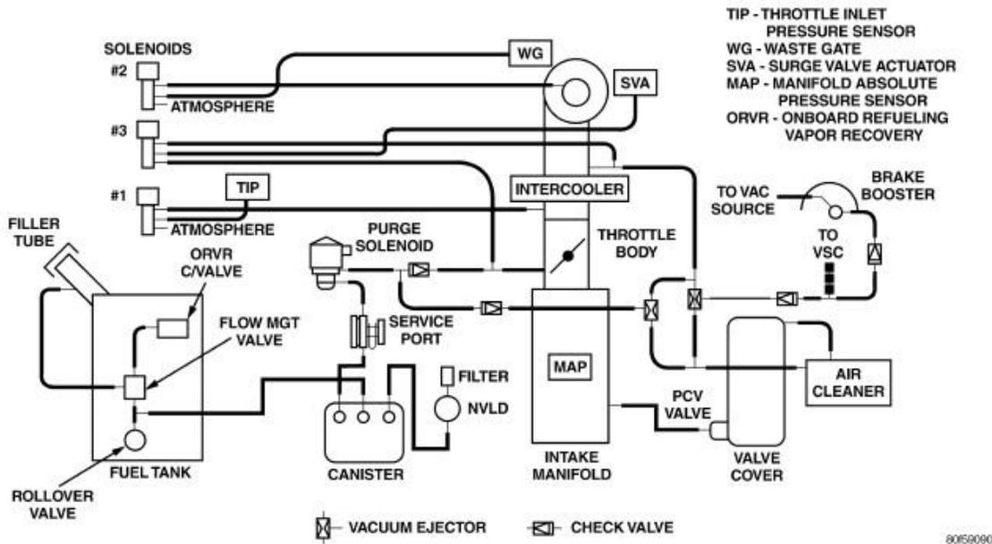
**Fig. 595: Vacuum Harness Schematic**
