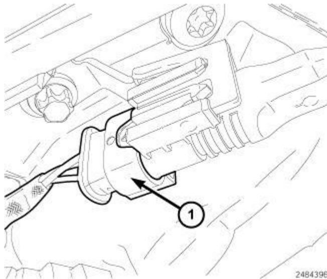
**Fig. 567: Knock Sensor Harness Connector**
