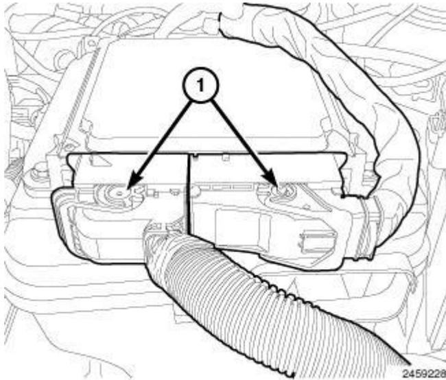
**Fig. 102: PCM Harness Connectors**
