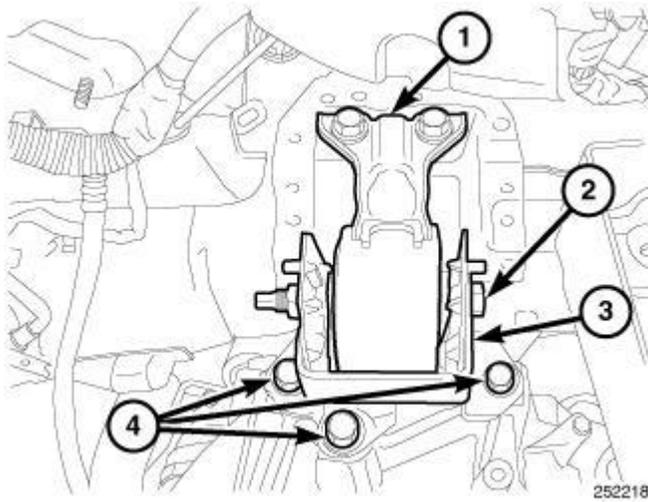
**Fig. 285: Left Engine Mount & Fasteners**
