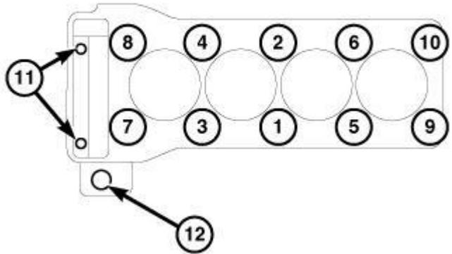
**Fig. 125: Cylinder Head Bolt Torque Sequence**
