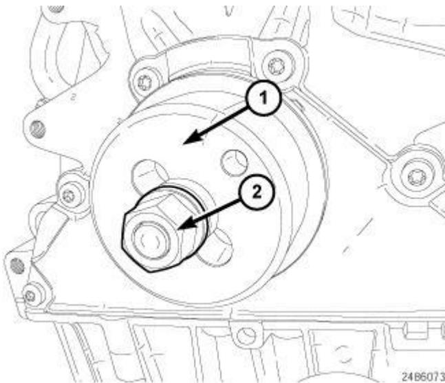
**Fig. 261: Front Crankshaft Seal Adapter & Nut**
