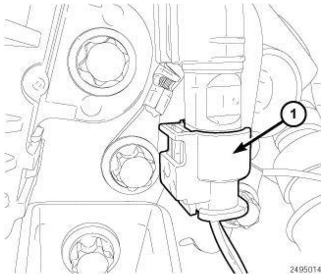
**Fig. 165: Turbocharger Exhaust Temperature Sensor Harness Connector**
