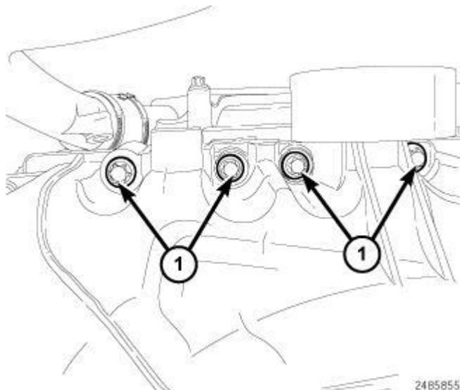
**Fig. 251: Front Oil Pan Bolts**
