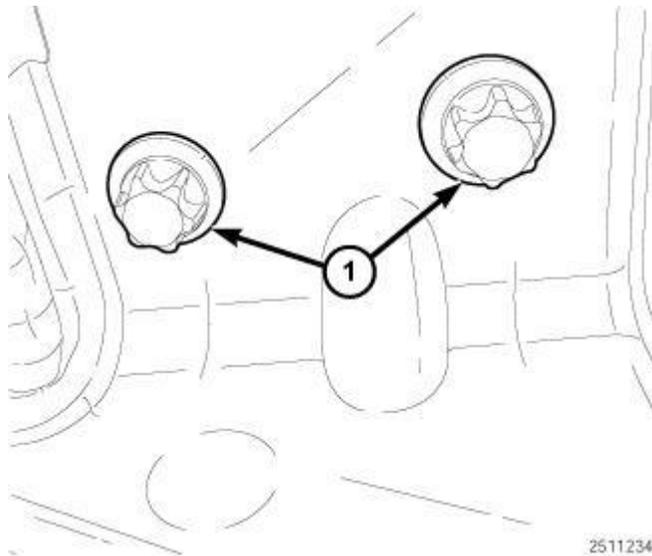
**Fig. 633: CAC Tube And Bracket Assembly Bolts**
