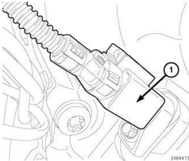
**Fig. 566: Crankshaft Position Sensor Harness Connector**
