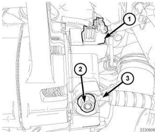
**Fig. 25: Battery Feed Wire, Generator Harness Connectors & Nut**
