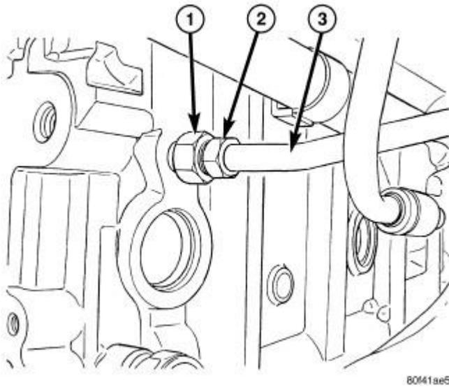
**Fig. 586: Coolant Supply Line - Engine Block Fitting**
