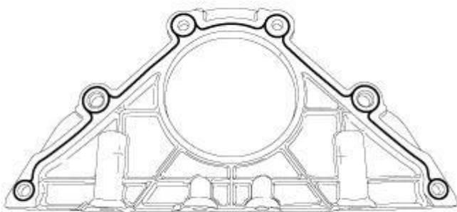
**Fig. 253: Applying Bead Of Engine Sealant RTV To Front Seal Carrier**
