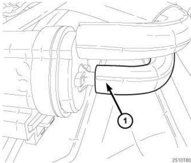
**Fig. 502: Coolant Pump Actuator Vacuum Line**
