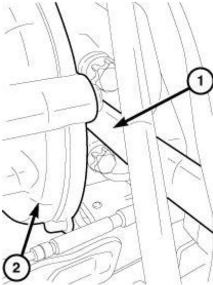
**Fig. 617: Oil Return Line At Turbocharger**
