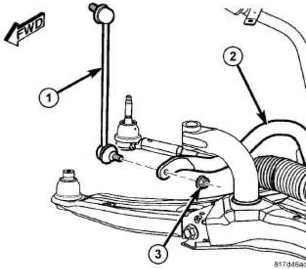
**Fig. 32: Stabilizer Link Mounting To Bar**
