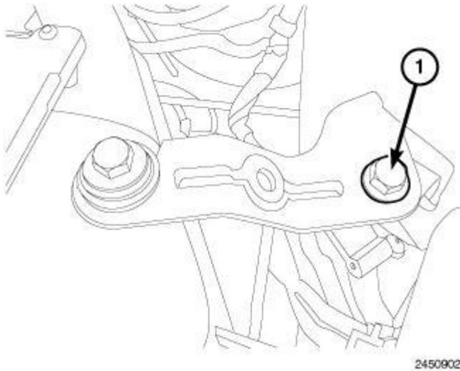
**Fig. 110: Air Cleaner Support Bracket Bolt**
