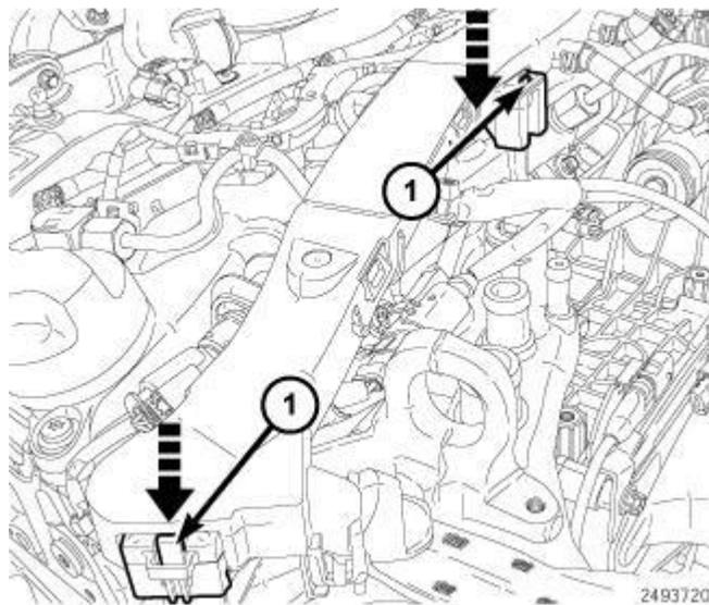
**Fig. 336: Positioning Wire Harness And Pushing Down To Lock Tabs**
