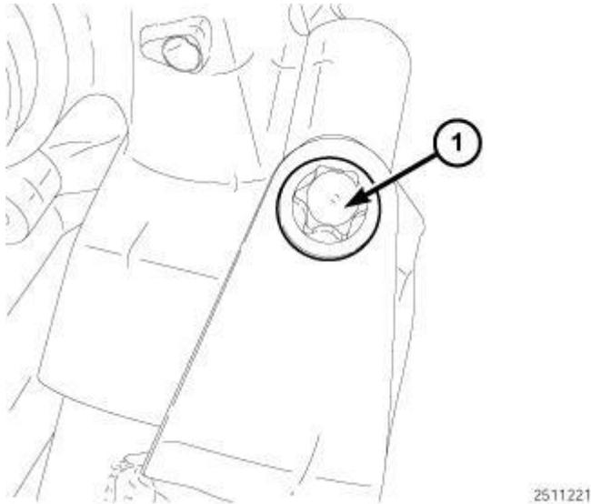
**Fig. 706: Charge Air Cooler CAC Tube Bolt**
