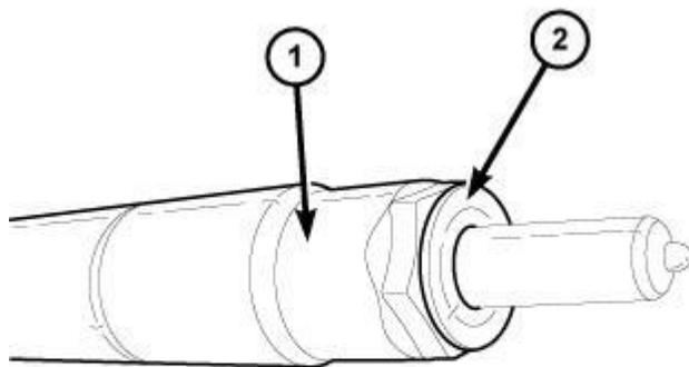
**Fig. 177: Injector & Sealing Ring**
