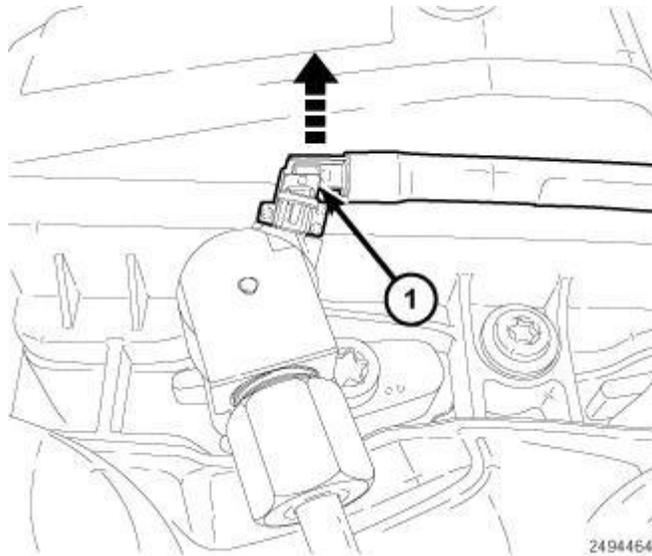
**Fig. 168: Releasing Lock Tab**
