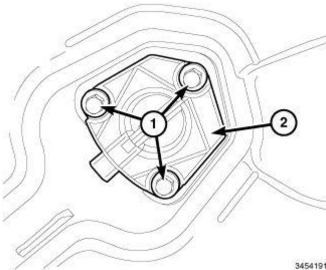
**Fig. 388: Oil Level Switch & Bolts**
