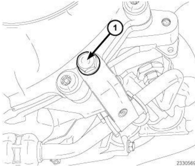
**Fig. 234: Power Steering Line Support Bracket Retaining Bolt**
