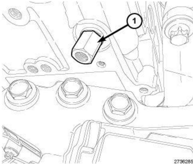
**Fig. 10: Test Adaptor Fitting**
