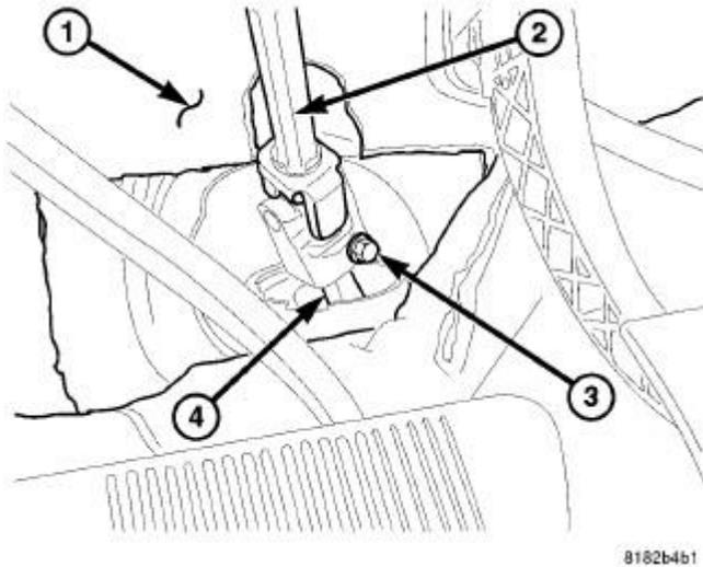
**Fig. 88: Lower Coupling Bolt**
