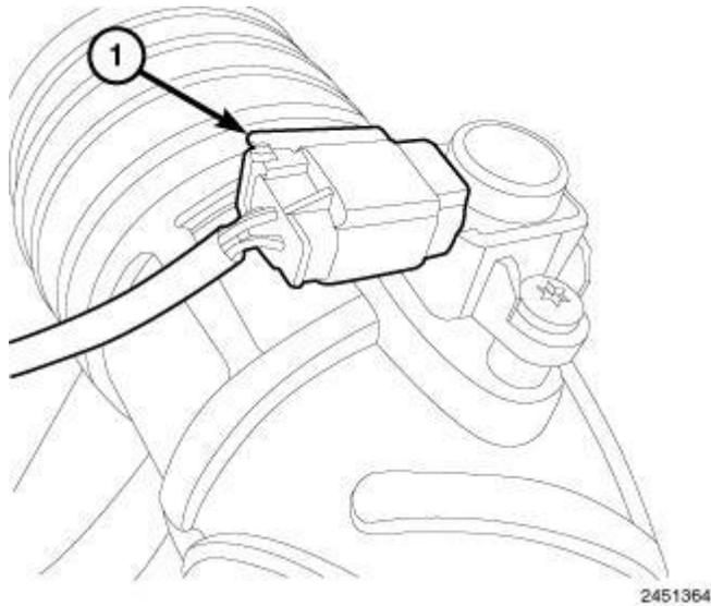
**Fig. 114: Intake Air Temperature/Boost Pressure Sensor**
