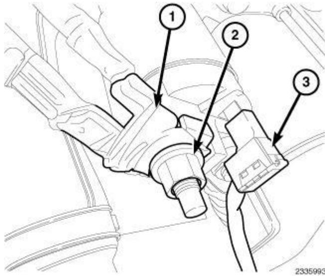
**Fig. 28: Battery Feed Wire To Starter, Starter Harness Connectors & Nut**
