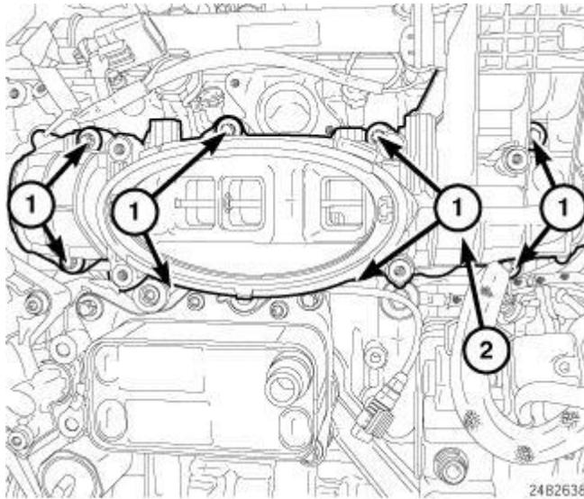
**Fig. 526: Intake Manifold & Bolts**
