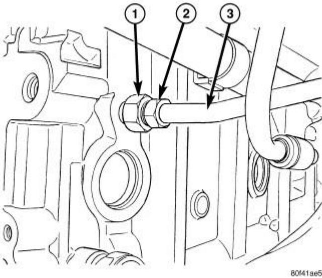
**Fig. 590: Coolant Supply Line - Engine Block Fitting**
