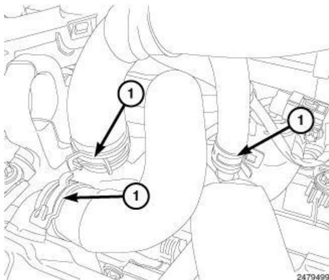
**Fig. 548: Locating Coolant Hoses**
