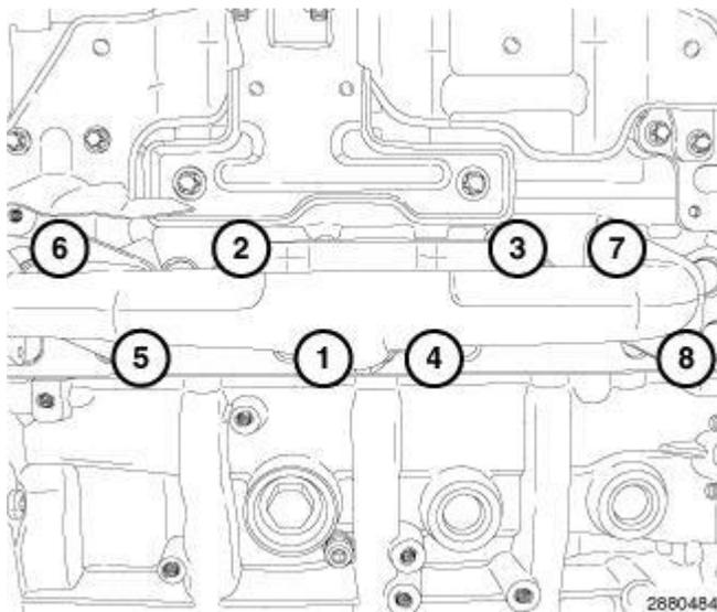
**Fig. 445: Exhaust Manifold Bolt Torque Sequence**
