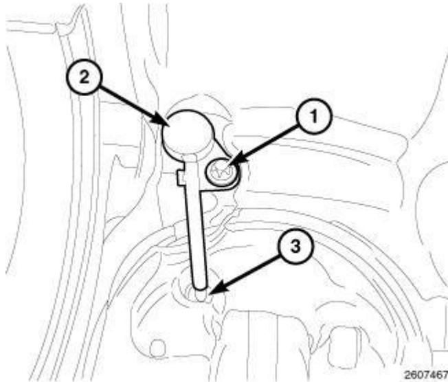
**Fig. 342: Removing & Installing Oil Jets**
