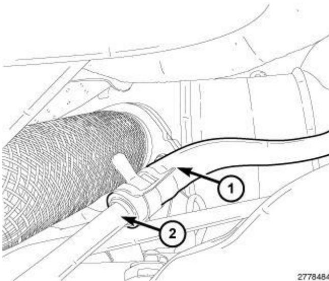
**Fig. 37: Power Steering Return Hose At Tube**
