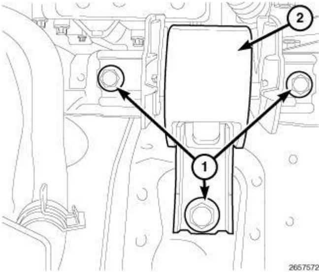
**Fig. 300: Engine Mount At Body Frame Rail & Bolts**
