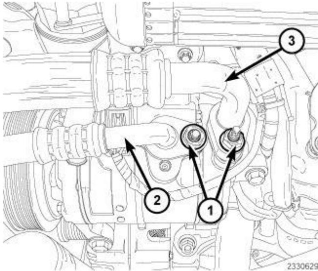
**Fig. 26: A/C Lines & Retaining Nuts**
