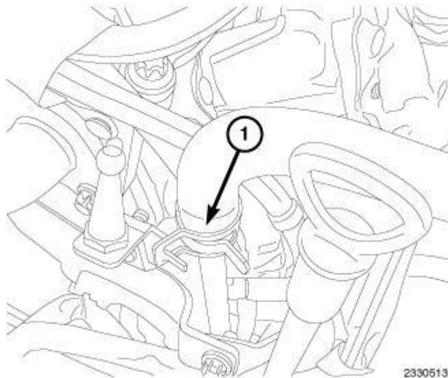
**Fig. 80: Brake Booster Vacuum Hose**
