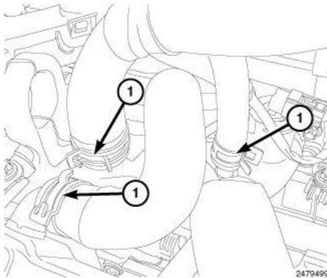
**Fig. 487: Locating Coolant Hoses**
