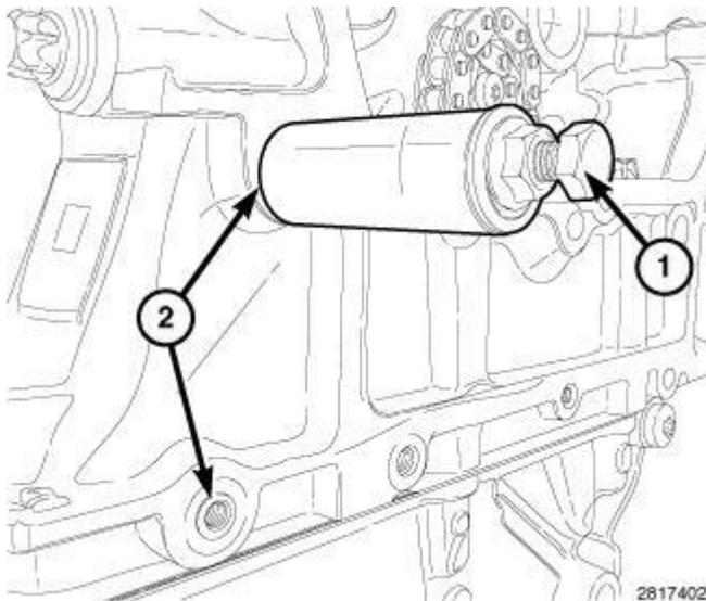
**Fig. 680: Extractor Bolt Tool & Timing Guide Pin**
