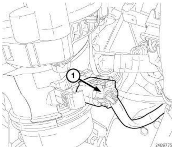
**Fig. 372: Identifying Charge Air Temperature Sensor Connectors**
