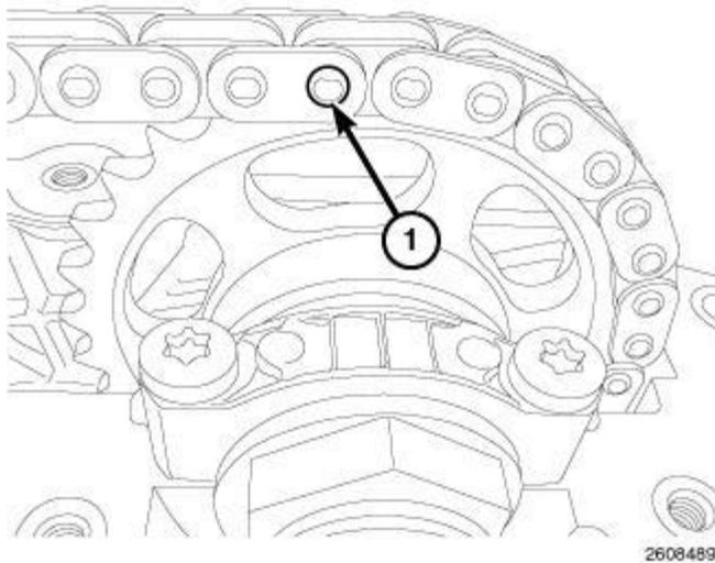
**Fig. 621: Timing Chain Pin At Chain Link**
