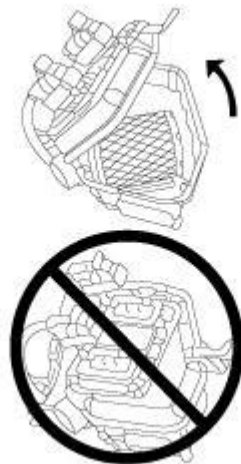
Fig. 62: Electrical Connectors At Powertrain Control Module (PCM) - DO NOT Unplug
