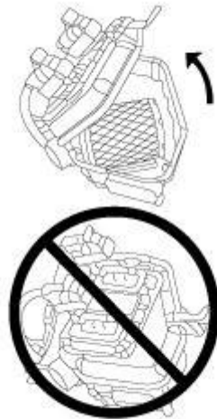
Fig. 65: Electrical Connectors At Powertrain Control Module (PCM) - DO NOT Unplug
