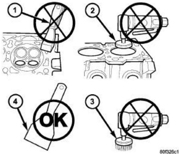
Fig. 76: Proper Tool Usage for Surface Preparation Courtesy of CHRYSLER LLC
