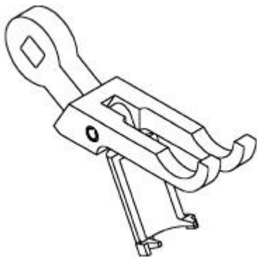
Fig. 45: Valve Spring Compressor - 8426
