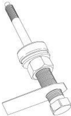
Fig. 40: Damper Installer - 8512A Courtesy of CHRYSLER LLC
