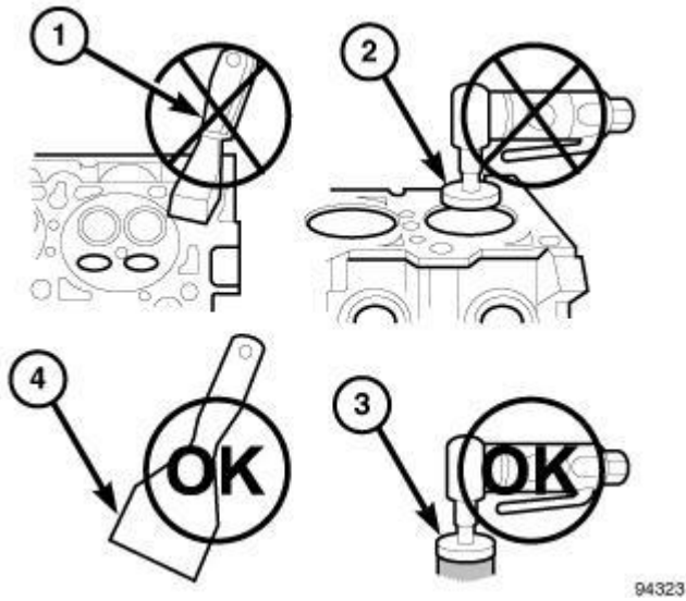
Fig. 3: Proper Tool Usage For Surface Preparation Courtesy of CHRYSLER GROUP, LLC
