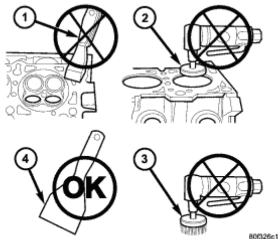
Fig. 4: PROPER TOOL USAGE FOR SURFACE PREPARATION
