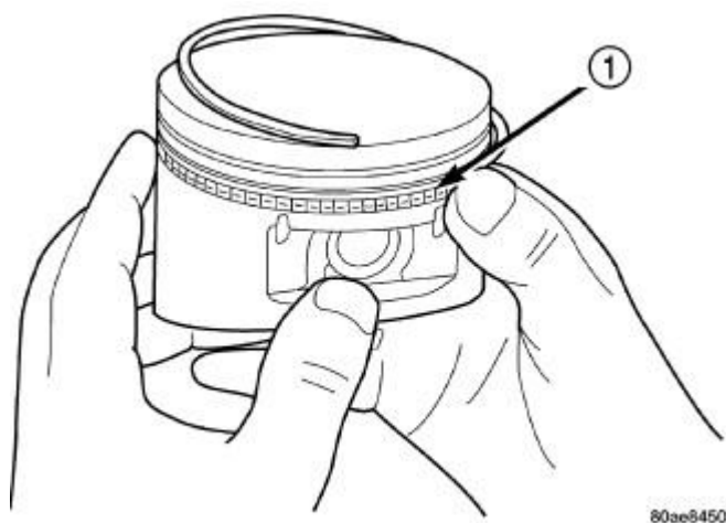
Fig. 96: Installing Piston Ring Side Rail Courtesy of CHRYSLER LLC
