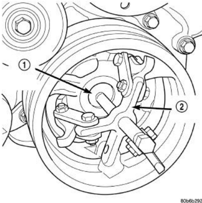
Fig. 133: Removing/Installing Damper Courtesy of CHRYSLER LLC
