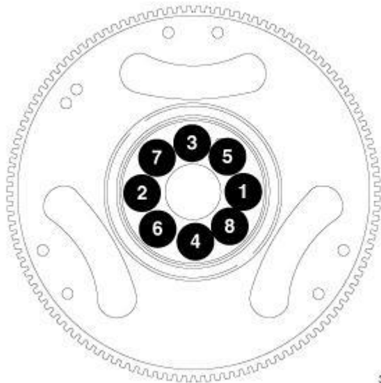
Fig. 209: Flex Plate Tightening Sequence
