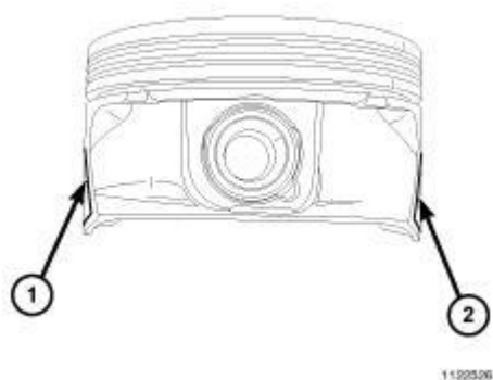
Fig. 204: Piston Diameter Measuring Points
