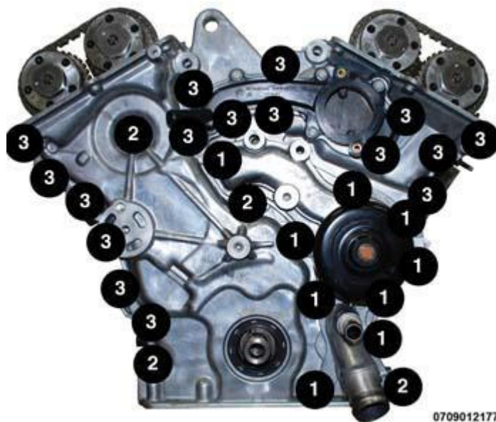
Fig. 613: Engine Timing Cover(s) Bolts Removing/Tightening Sequence Courtesy of CHRYSLER GROUP, LLC
