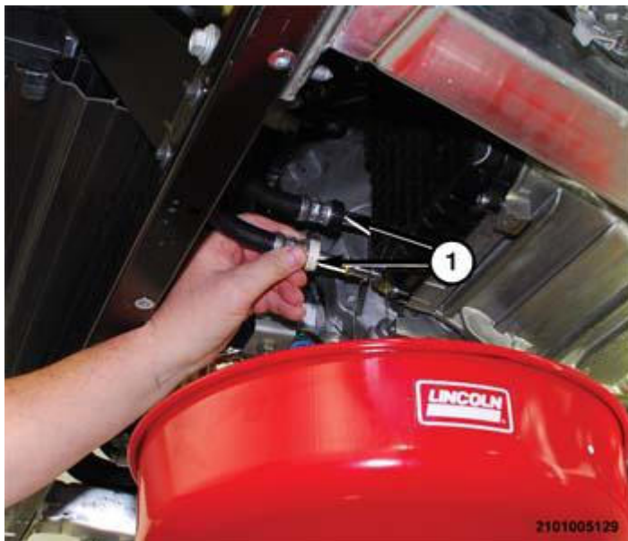
Fig. 24: Transmission Cooler Lines Courtesy of CHRYSLER GROUP, LLC
