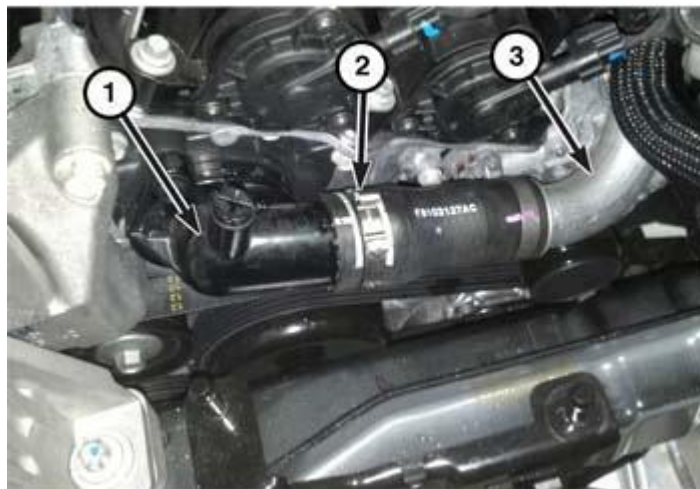
Fig. 632: Removing/Installing Thermostat Housing Courtesy of CHRYSLER GROUP, LLC
