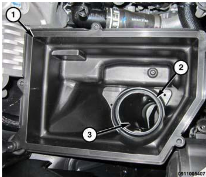
Fig. 77: Air Filter Body, Seal & Air Filter Body Courtesy of CHRYSLER GROUP, LLC
