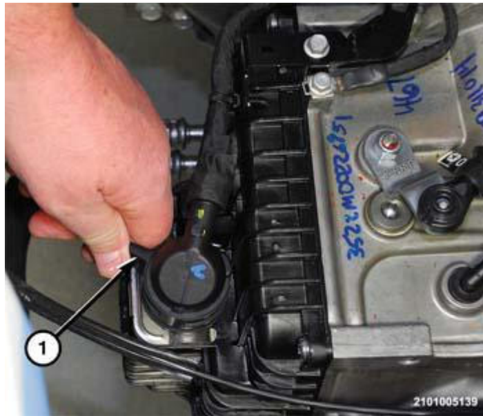
Fig. 35: Transmission Valve Body Solenoid Connector Courtesy of CHRYSLER GROUP, LLC
