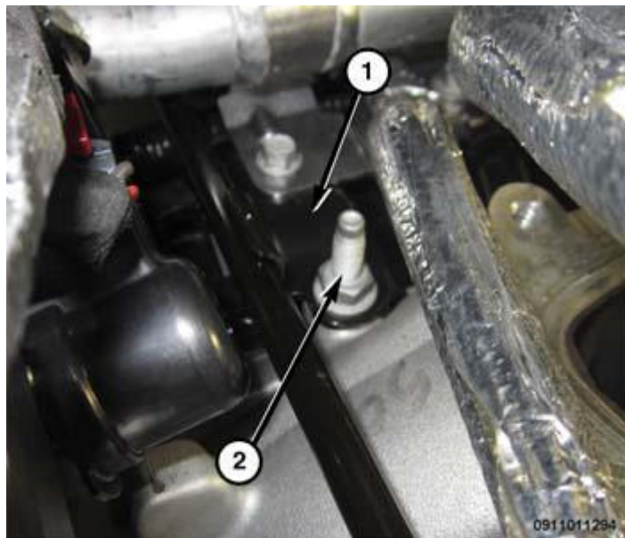
Fig. 248: Intake Manifold Left/Forward Support Bracket & Stud Bolt Courtesy of CHRYSLER GROUP, LLC
