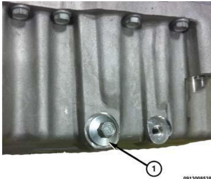
Fig. 461: Crankcase Drain Plug Courtesy of CHRYSLER GROUP, LLC
