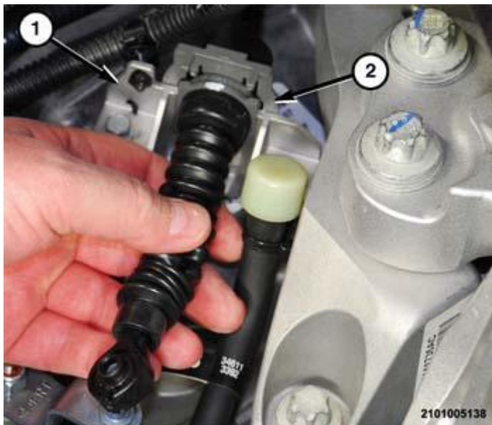
Fig. 30: View Of Shift Cable Housing & Mount Bracket
