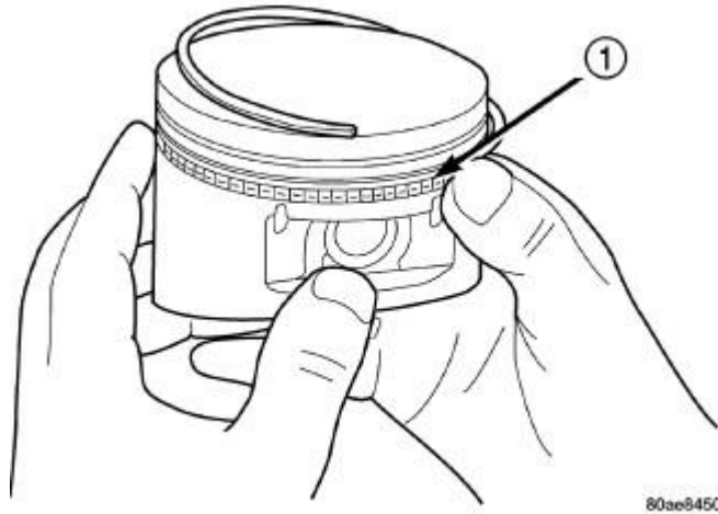
Fig. 374: Removing/Installing Piston Ring Side Rail Courtesy of CHRYSLER GROUP, LLC
