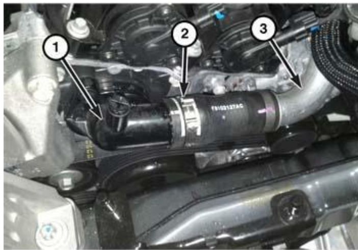
Fig. 604: Removing/Installing Thermostat Housing
