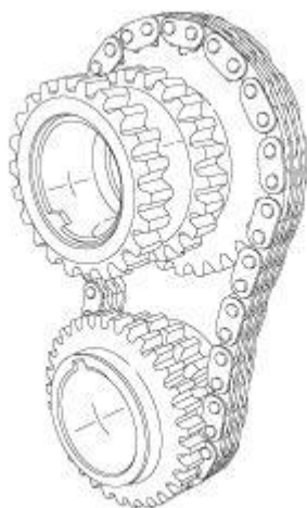
Fig. 554: Primary Chain, Idler Sprocket & Crankshaft Sprocket Courtesy of CHRYSLER GROUP, LLC
