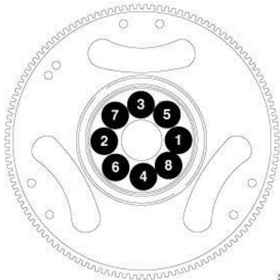
Fig. 209: Flex Plate Tightening Sequence Courtesy of CHRYSLER GROUP, LLC
