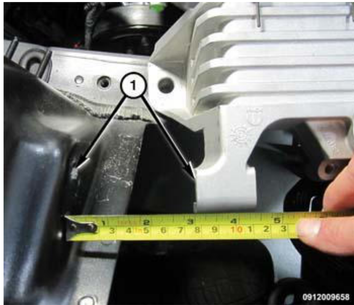
Fig. 316: Measuring Three Inches Courtesy of CHRYSLER GROUP, LLC
