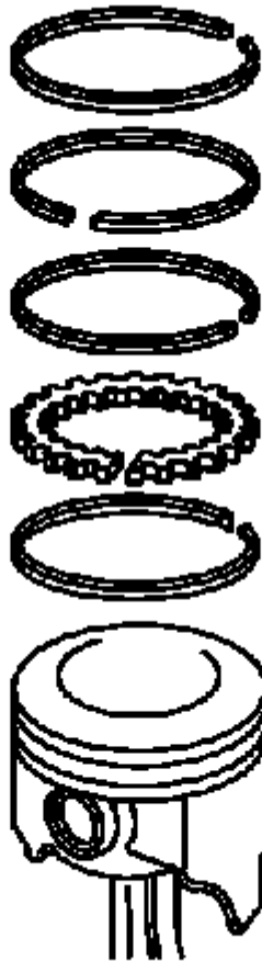
Fig. 471: Exploded View Of Piston Rings
