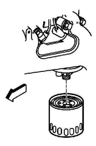
Fig. 232: View Of Oil Filter
