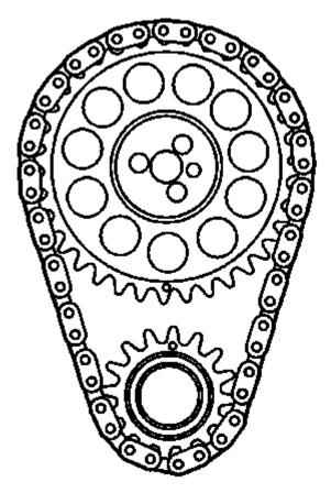
Fig. 204: View Of Camshaft & Crankshaft Sprocket Timing Marks Courtesy of GENERAL MOTORS COMPANY
