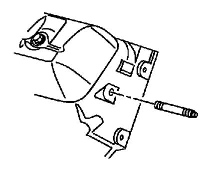
Fig. 151: View Of Generator Bracket Stud Courtesy of GENERAL MOTORS COMPANY
