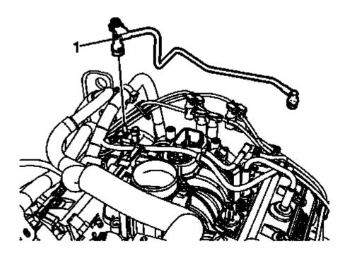
Fig. 306: View Of Tube Quick Connect Fitting Courtesy of GENERAL MOTORS COMPANY
