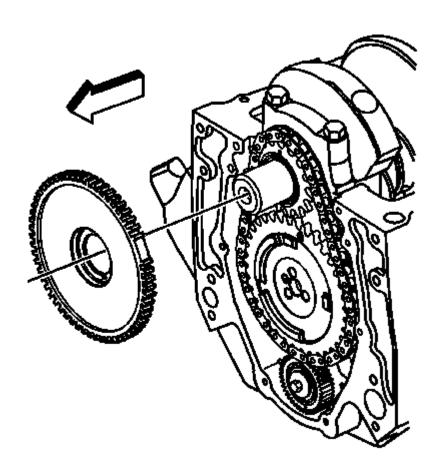
Fig. 389: View Of Crankshaft Position Sensor Reluctor Ring Courtesy of GENERAL MOTORS COMPANY
