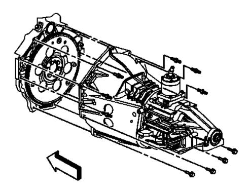
Fig. 243: Manual Transmission Bolts
