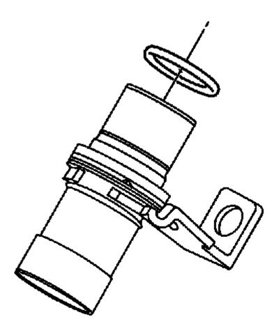
Fig. 386: View Of Crankshaft Position Sensor Seal O-Ring Courtesy of GENERAL MOTORS COMPANY
