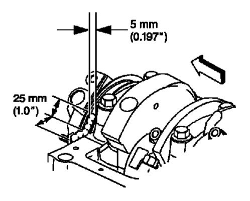
Fig. 630: Applying Adhesive To Engine Sides Front Cover To Engine Block Junction Courtesy of GENERAL MOTORS COMPANY
