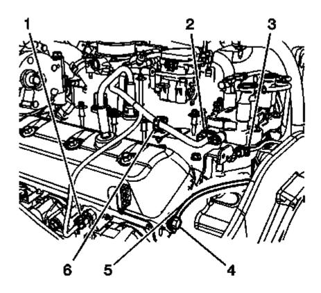
Fig. 313: Engine Coolant Temperature Sensor, Ignition Coil & Oil Pressure Sensor Courtesy of GENERAL MOTORS COMPANY
