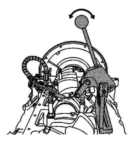
Fig. 471: Actuating Pivot Arm Assembly Handle Courtesy of GENERAL MOTORS COMPANY
