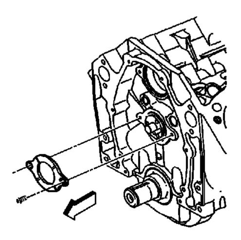
Fig. 220: View Of Camshaft Retainer & Bolts Courtesy of GENERAL MOTORS COMPANY
