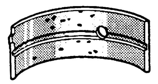
Fig. 449: Identifying Crankshaft Bearing Craters Or Pockets Courtesy of GENERAL MOTORS COMPANY
