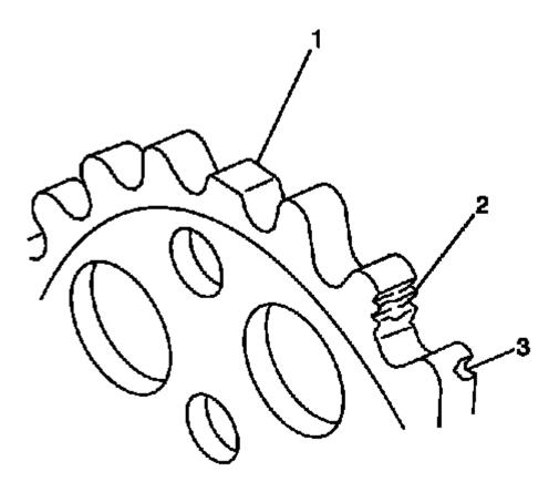
Fig. 499: Identifying Damaged Sprocket Teeth Courtesy of GENERAL MOTORS COMPANY
