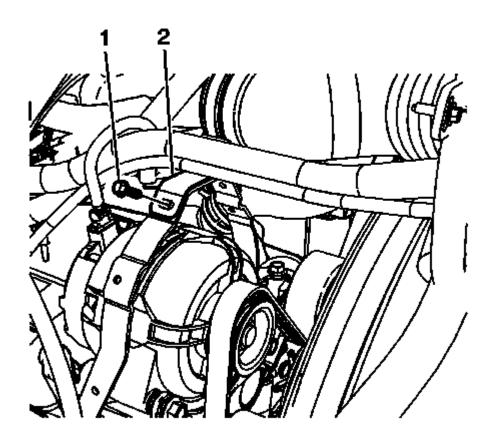
Fig. 273: Oil Level Indicator Tube Bolt & Bracket Courtesy of GENERAL MOTORS COMPANY
