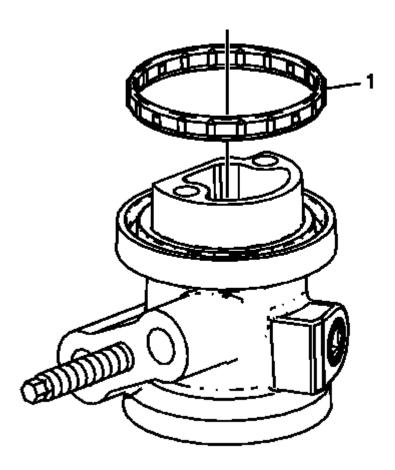
Fig. 226: Identifying Oil Filter Adapter Seal O-Ring Courtesy of GENERAL MOTORS COMPANY
