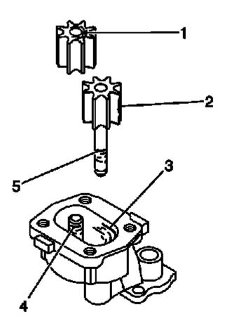
Fig. 529: Identifying Oil Pump Components Courtesy of GENERAL MOTORS COMPANY
