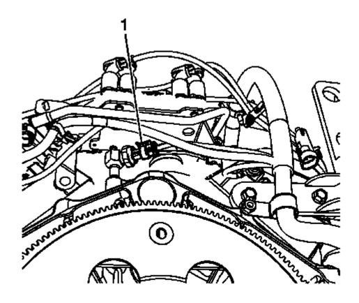
Fig. 265: View Of Oil Pressure Sensor Electrical Connector Courtesy of GENERAL MOTORS COMPANY
