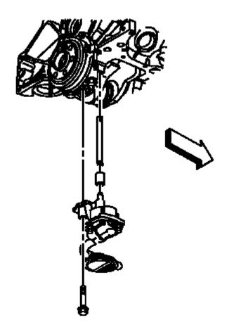
Fig. 283: Oil Pump & Mounting Bolt Courtesy of GENERAL MOTORS COMPANY
