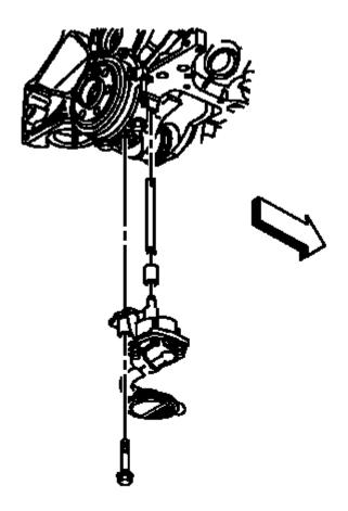
Fig. 280: Oil Pump & Mounting Bolt Courtesy of GENERAL MOTORS COMPANY
