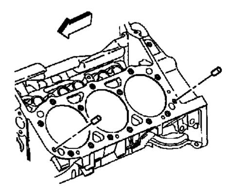
Fig. 366: View Of Cylinder Head Locator Pins Courtesy of GENERAL MOTORS COMPANY
