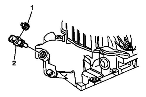
Fig. 561: ECT Sensor & Plug Courtesy of GENERAL MOTORS COMPANY
