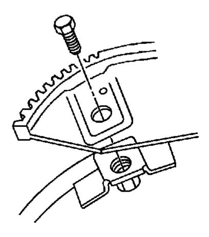
Fig. 318: Flywheel-To-Torque Converter Bolts
