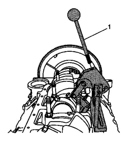
Fig. 464: Pivot Arm Assembly Handle Courtesy of GENERAL MOTORS COMPANY
