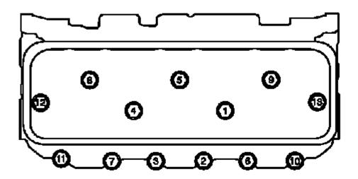
Fig. 161: Identifying Cylinder Head Bolt Tightening Sequence Courtesy of GENERAL MOTORS COMPANY
