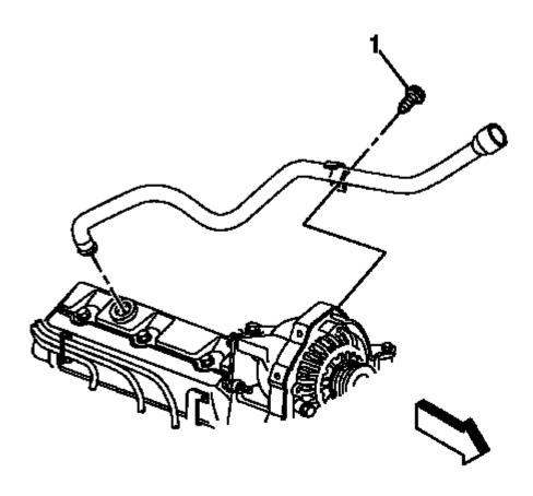
Fig. 37: View Oil Fill Tube Bolt Courtesy of GENERAL MOTORS COMPANY
