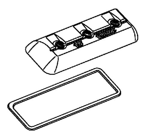
Fig. 96: View Of Rocker Arm Cover And Gasket Courtesy of GENERAL MOTORS COMPANY
