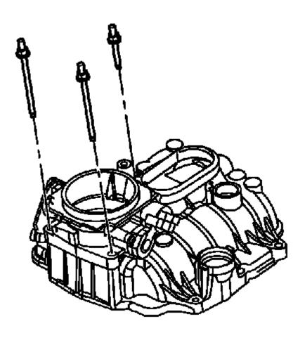
Fig. 541: View Of Throttle Body & Attaching Studs Courtesy of GENERAL MOTORS COMPANY
