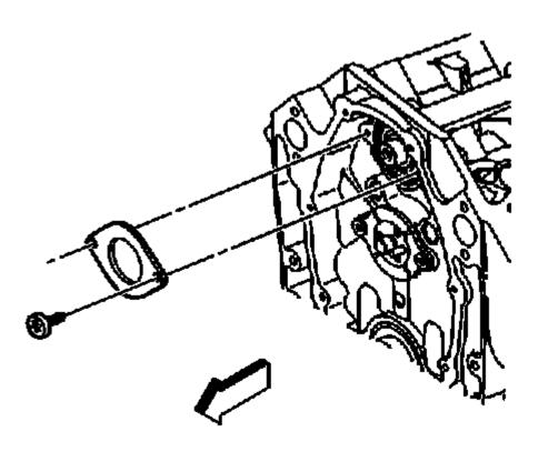
Fig. 207: View of Balance Shaft Retainer & Bolts Courtesy of GENERAL MOTORS COMPANY
