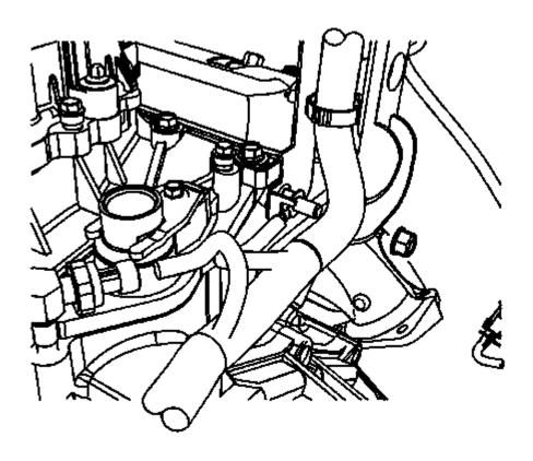
Fig. 84: Engine Wiring Harness Ground Nut Courtesy of GENERAL MOTORS COMPANY
