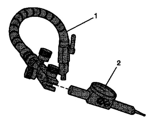
Fig. 466: View Of Swivel Base & Dial Indicator Courtesy of GENERAL MOTORS COMPANY
