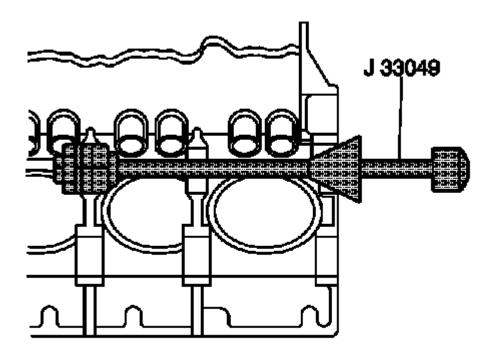
Fig. 490: Removing/Installation Camshaft Inner Bearing Using J 33049 Courtesy of GENERAL MOTORS COMPANY
