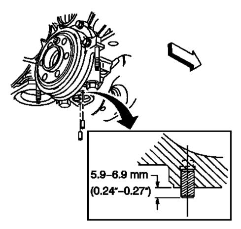
Fig. 282: Oil Pump Locator Pins
