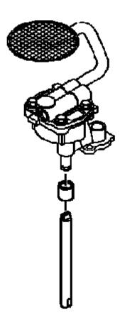
Fig. 523: View Of Oil Pump Driveshaft & Oil Pump Driveshaft Retainer Courtesy of GENERAL MOTORS COMPANY
