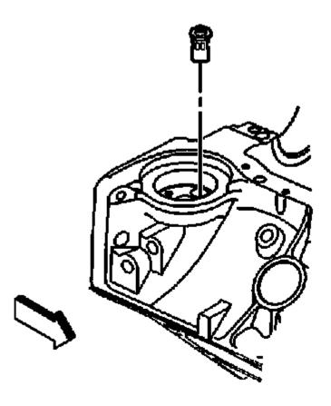
Fig. 424: Identifying Oil Filter Bypass Valve Courtesy of GENERAL MOTORS COMPANY
