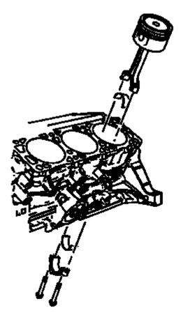
Fig. 602: View Of Connecting Rod & Piston Assembly Courtesy of GENERAL MOTORS COMPANY
