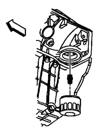
Fig. 231: View Of Oil Filter & Adapter Courtesy of GENERAL MOTORS COMPANY
