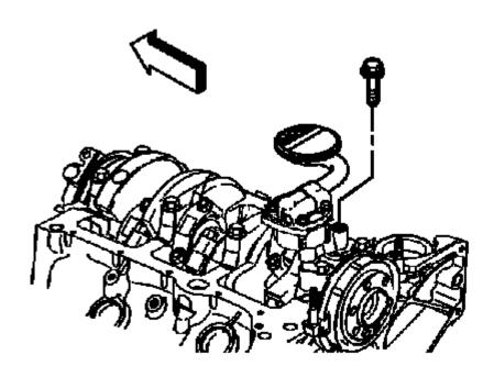
Fig. 382: View Of Oil Pump Bolt Courtesy of GENERAL MOTORS COMPANY
