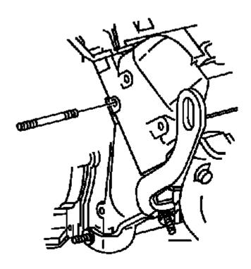
Fig. 148: Locating Power Steering Pump Mounting Bracket Stud Courtesy of GENERAL MOTORS COMPANY
