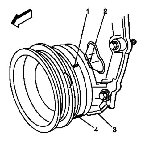
Fig. 114: View Of Crankshaft Balancer Alignment Mark & Engine Front Cover Alignment Tab Courtesy of GENERAL MOTORS COMPANY
