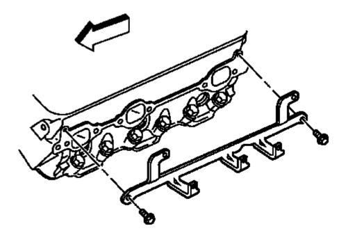
Fig. 135: Locating Spark Plug Wire Support Courtesy of GENERAL MOTORS COMPANY
