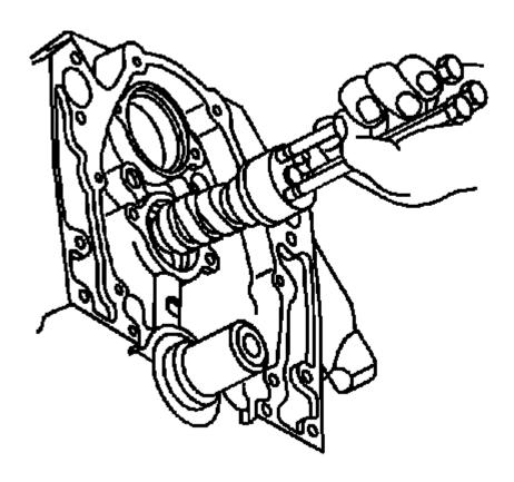
Fig. 222: Using Bolts To Handle Camshaft
