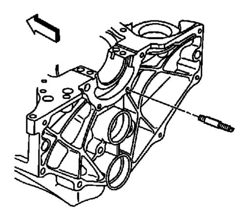
Fig. 592: Locating Crankshaft Rear Oil Seal Housing Retainer Stud Courtesy of GENERAL MOTORS COMPANY
