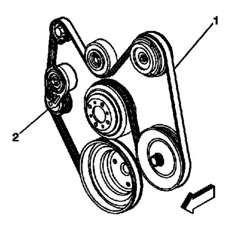
Fig. 11: Drive Belt Routing & Tensioner (W/ A/C)
