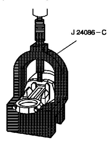
Fig. 439: Removing/Installing Piston Pin
