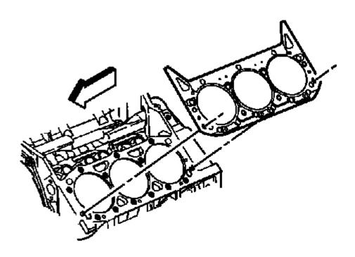
Fig. 138: View Of Cylinder Head Gasket And Alignment Pins - Left Courtesy of GENERAL MOTORS COMPANY
