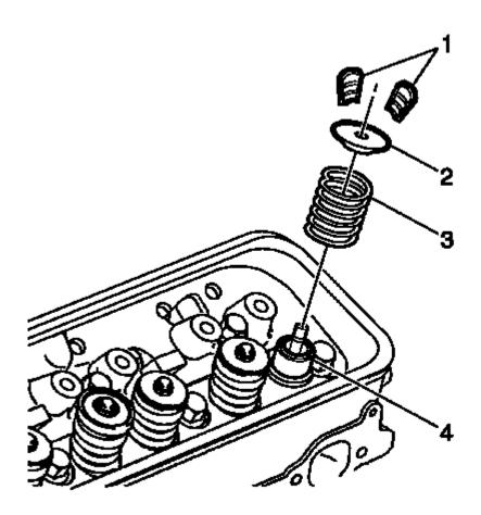
Fig. 507: Identifying Valve Components
