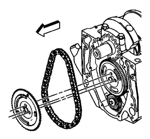
Fig. 393: Camshaft Sprocket And Camshaft Timing Chain Courtesy of GENERAL MOTORS COMPANY
