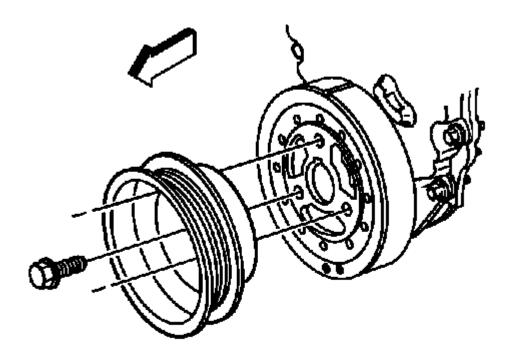
Fig. 165: View Of Crankshaft Pulley & Bolts Courtesy of GENERAL MOTORS COMPANY
