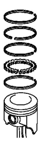
Fig. 441: Exploded View Of Piston Rings
