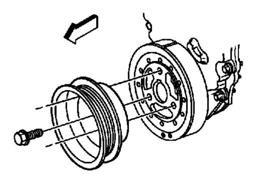
Fig. 341: View Of Crankshaft Pulley & Bolts Courtesy of GENERAL MOTORS COMPANY
