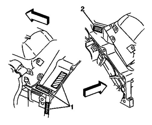
Fig. 6: Engine VIN Locations
