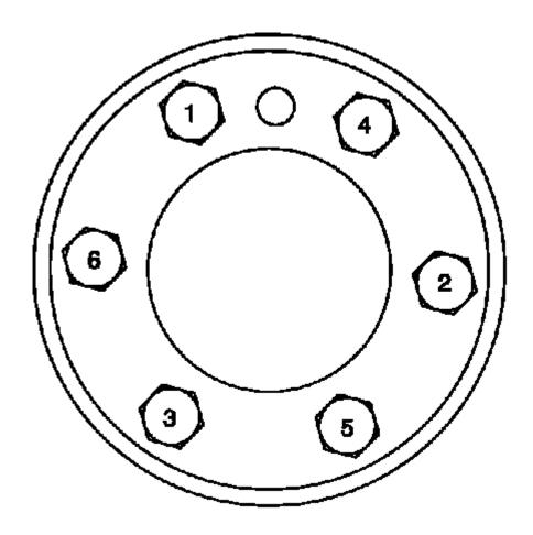
Fig. 695: Identifying Flywheel Bolt Tightening Sequence Courtesy of GENERAL MOTORS COMPANY
