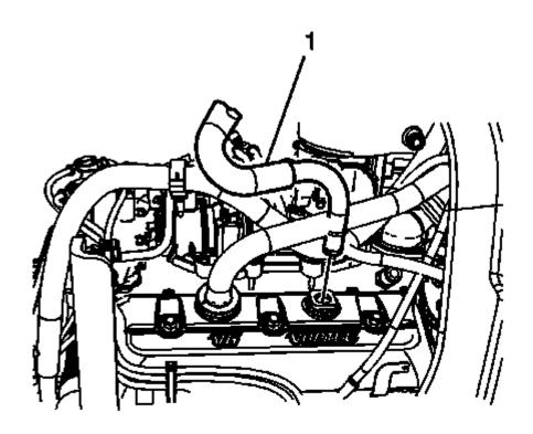
Fig. 106: View Of Positive Crankcase Ventilation (PCV) Hose Courtesy of GENERAL MOTORS COMPANY
