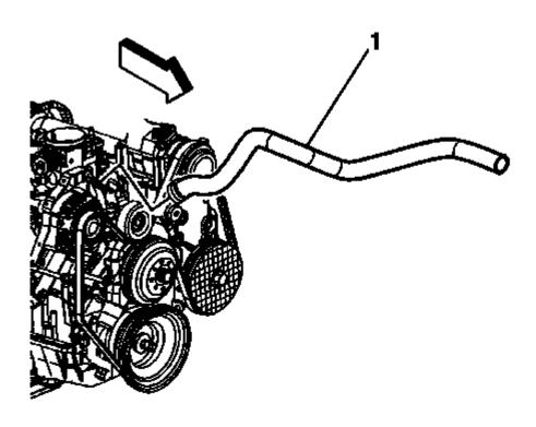
Fig. 70: View Of Radiator Inlet Hose Courtesy of GENERAL MOTORS COMPANY
