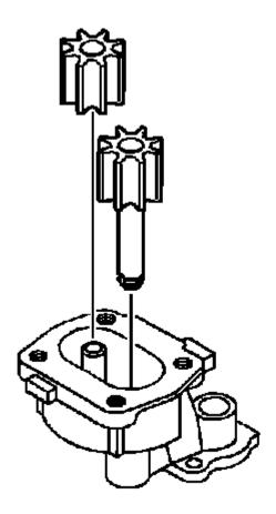
Fig. 531: View Of Oil Pump Drive Gear & Driven Gear Courtesy of GENERAL MOTORS COMPANY
