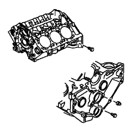
Fig. 418: Engine Block Oil Gallery Plugs Courtesy of GENERAL MOTORS COMPANY
