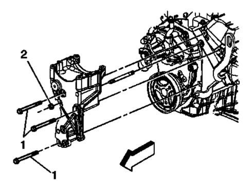
Fig. 131: P/S Pump Rear Bracket Front Nut **Courtesy of GENERAL MOTORS COMPANY**
