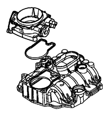
Fig. 47: View Of Throttle Body & Gasket Courtesy of GENERAL MOTORS COMPANY
