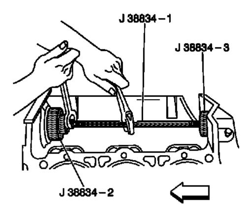
Fig. 218: Installing Balance Shaft Rear Bearing Courtesy of GENERAL MOTORS COMPANY
