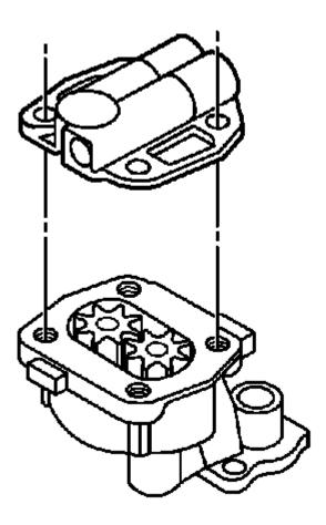
Fig. 532: View Of Oil Pump Cover Courtesy of GENERAL MOTORS COMPANY
