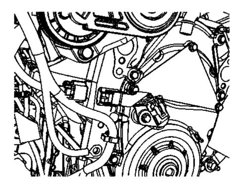
Fig. 180: Camshaft Position (CMP) Sensor Wiring Harness Jumper Courtesy of GENERAL MOTORS COMPANY
