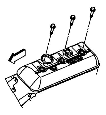
Fig. 681: Valve Rocker Arm Cover Bolts (Left)
