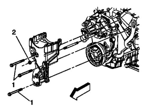
Fig. 149: P/S Pump Rear Bracket Front Nut Courtesy of GENERAL MOTORS COMPANY
