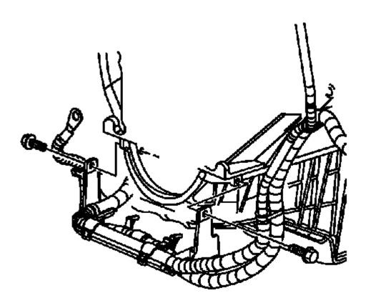
Fig. 261: View Of Battery Cable Bracket Bolts Courtesy of GENERAL MOTORS COMPANY
