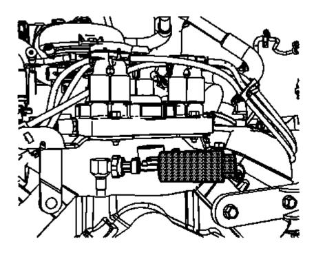
Fig. 266: Fuel Pump/Oil Pressure Sensor Courtesy of GENERAL MOTORS COMPANY
