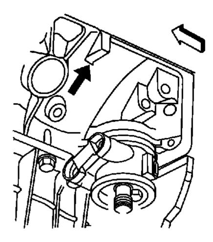
Fig. 19: View Of Square Tab At Rear Of Engine Block Courtesy of GENERAL MOTORS COMPANY
