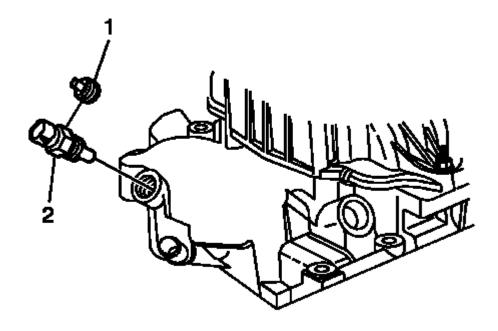
Fig. 544: ECT Sensor & Plug Courtesy of GENERAL MOTORS COMPANY
