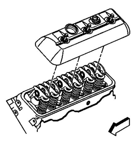
Fig. 94: Rocker Arm Cover Courtesy of GENERAL MOTORS COMPANY
