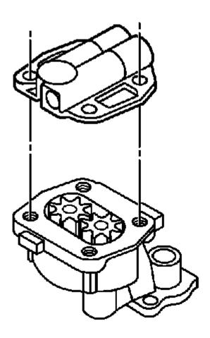
Fig. 526: View Of Oil Pump Cover Courtesy of GENERAL MOTORS COMPANY
