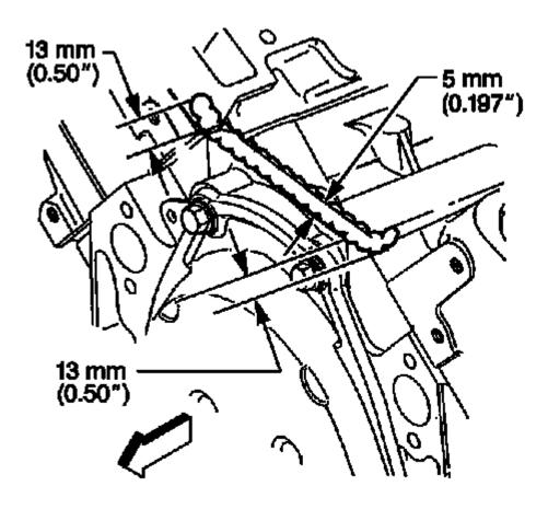
Fig. 670: Applying Adhesive To Front Top Of Engine Block Courtesy of GENERAL MOTORS COMPANY
