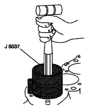
Fig. 603: Installing Piston & Connecting Rod Assembly Into Engine Courtesy of GENERAL MOTORS COMPANY
