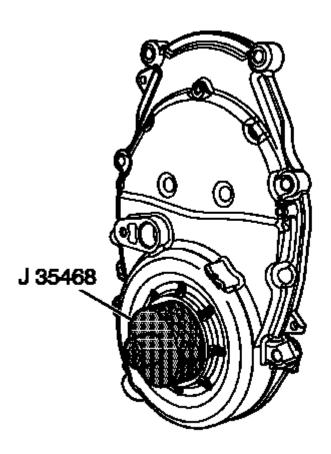
Fig. 174: Installing Front Seal Courtesy of GENERAL MOTORS COMPANY
