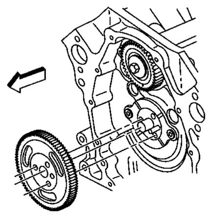
Fig. 219: View Of Balance Shaft Drive Gear Courtesy of GENERAL MOTORS COMPANY
