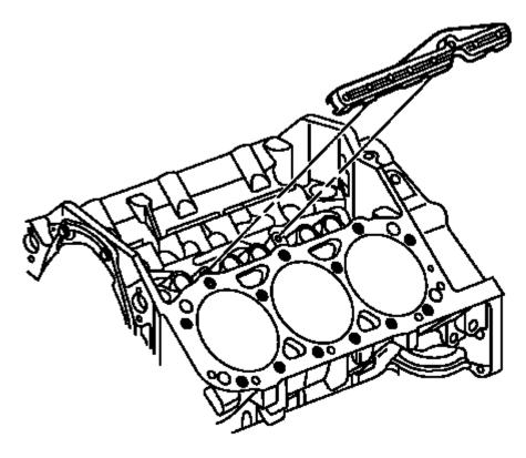
Fig. 129: View Of Valve Lifter Pushrod Guides Courtesy of GENERAL MOTORS COMPANY
