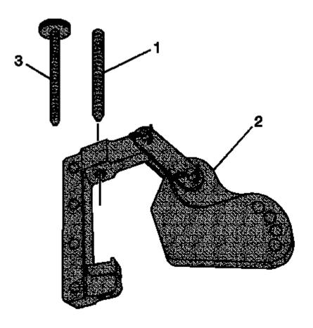
Fig. 457: Pivot Arm Assembly Screw
