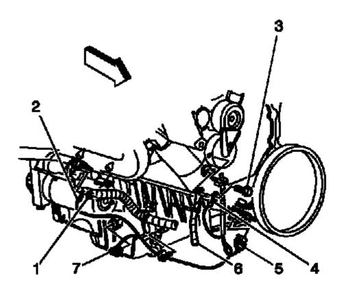
Fig. 260: View Of Oil Level Sensor Electrical Connector, CKP Electrical Connector & Battery Ground Bolt
