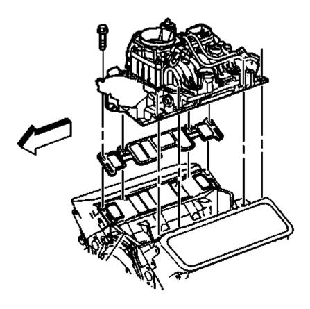
Fig. 672: View Of Intake Manifold Assembly & Bolts Courtesy of GENERAL MOTORS COMPANY
