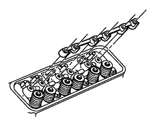
Fig. 108: View Of Valve Rocker Arm Supports
