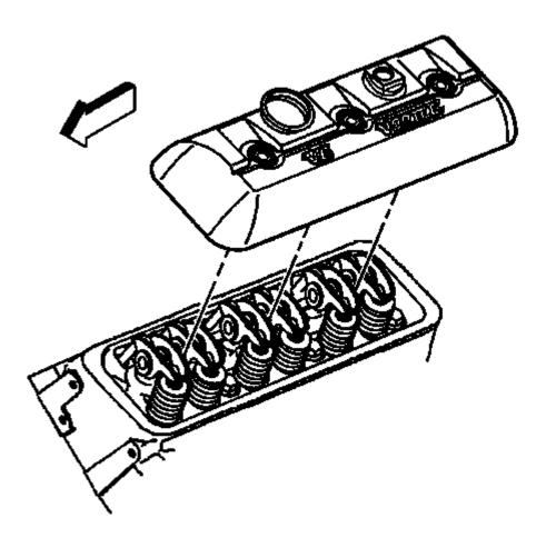
Fig. 345: Valve Rocker Arm Cover (Left)
