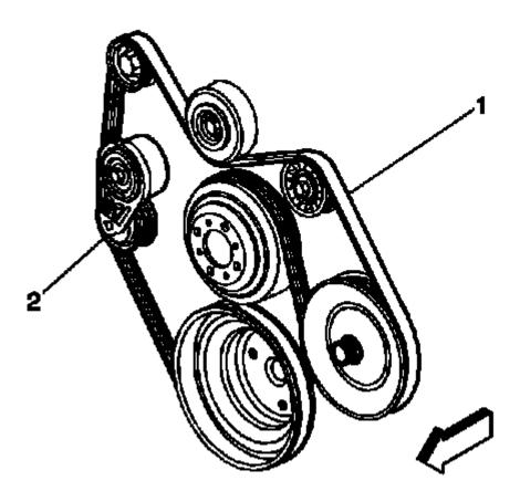
Fig. 9: Drive Belt Routing & Tensioner (W/O A/C) Courtesy of GENERAL MOTORS COMPANY
