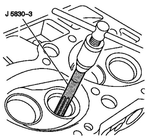
Fig. 516: Reaming Exhaust Valve Guide Using J 5830-3 Courtesy of GENERAL MOTORS COMPANY
