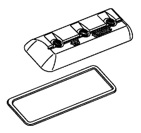
Fig. 679: View Of Rocker Arm Cover And Gasket Courtesy of GENERAL MOTORS COMPANY
