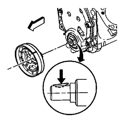
Fig. 641: Identifying Crankshaft Balancer & Key Courtesy of GENERAL MOTORS COMPANY
