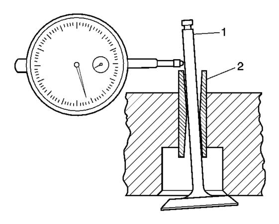
Fig. 515: Inspecting For Excessive Valve Stem To Guide Clearance Courtesy of GENERAL MOTORS COMPANY
