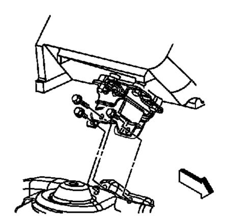
Fig. 20: View Of Right Side (Left Side Similar) Engine Mount To Engine Mount Bracket Bolts Courtesy of GENERAL MOTORS COMPANY
