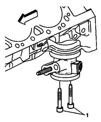
Fig. 639: Identifying Oil Filter Adapter Bolts
