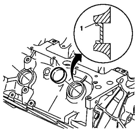
Fig. 573: Engine Block Core Hole Chamfer Courtesy of GENERAL MOTORS COMPANY
