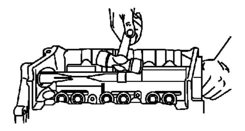
Fig. 399: Removing Balance Shaft
