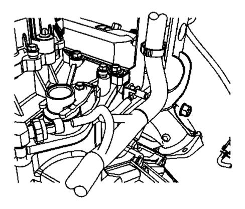
Fig. 67: Engine Wiring Harness Ground Nut Courtesy of GENERAL MOTORS COMPANY
