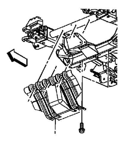
Fig. 176: View Of Engine Protection Shield **Courtesy of GENERAL MOTORS COMPANY**
