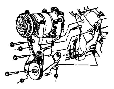
Fig. 72: View Of Power Steering Pump Bracket Courtesy of GENERAL MOTORS COMPANY
