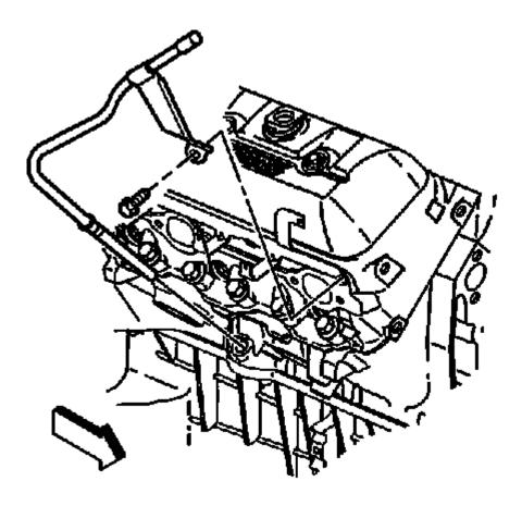
Fig. 336: Oil Level Indicator Tube
