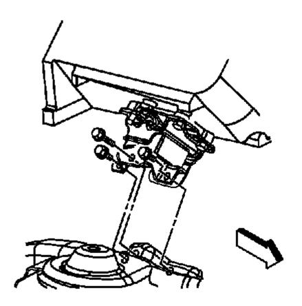
Fig. 26: View Of Right Side (Left Side Similar) Engine Mount To Engine Mount Bracket Bolts Courtesy of GENERAL MOTORS COMPANY
