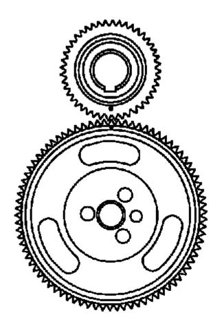
Fig. 216: Aligning Balance Shaft Drive Gear & Balance Shaft Driven Gear Timing Marks Courtesy of GENERAL MOTORS COMPANY
