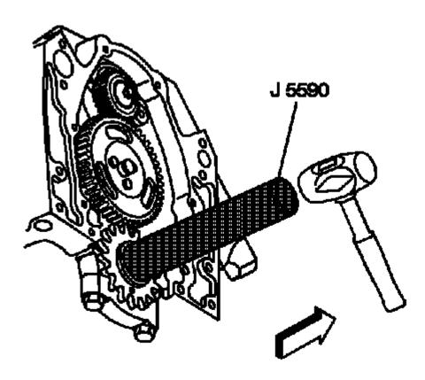
Fig. 200: Crankshaft Sprocket Courtesy of GENERAL MOTORS COMPANY
