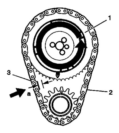
Fig. 391: Checking Camshaft Timing Chain Free Play Courtesy of GENERAL MOTORS COMPANY
