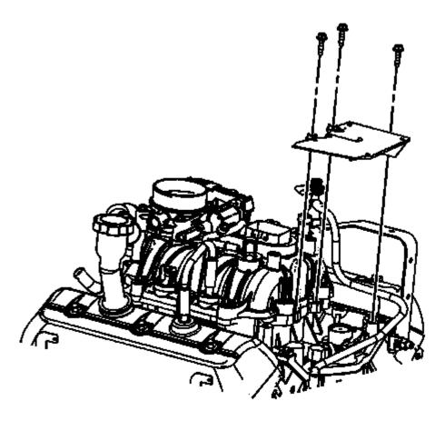
Fig. 351: View Of Ignition Coil Bracket & Bolts Courtesy of GENERAL MOTORS COMPANY
