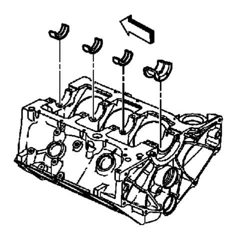
Fig. 453: View Of Crankshaft Bearings At Engine Block Courtesy of GENERAL MOTORS COMPANY
