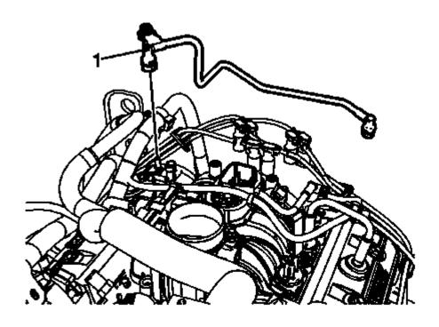
Fig. 311: View Of Tube Quick Connect Fitting Courtesy of GENERAL MOTORS COMPANY
