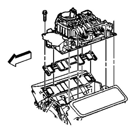
Fig. 355: View Of Intake Manifold Assembly & Bolts Courtesy of GENERAL MOTORS COMPANY
