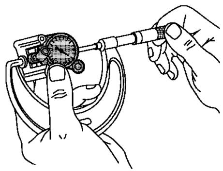
Fig. 598: Measuring Bore Gauge With Micrometer Courtesy of GENERAL MOTORS COMPANY
