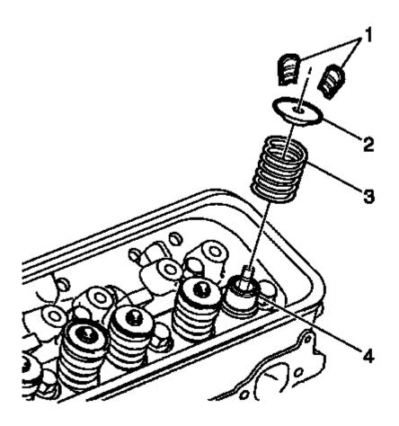
Fig. 118: Identifying Valve Components
