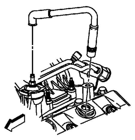
Fig. 58: Locating PCV Valve Hose At Valve & Rocker Cover Courtesy of GENERAL MOTORS COMPANY
