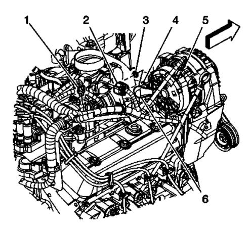
Fig. 86: View Of Engine Wiring Harness & Components Courtesy of GENERAL MOTORS COMPANY
