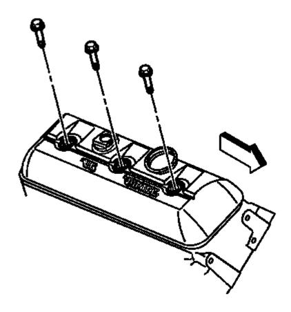
Fig. 684: View Of Valve Rocker Arm Cover Bolts (Right)
