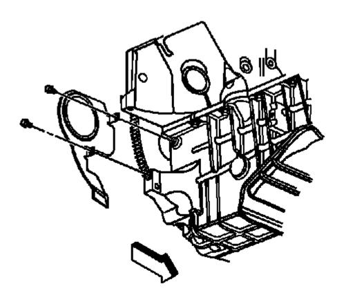
Fig. 240: Transmission Cover Courtesy of GENERAL MOTORS COMPANY
