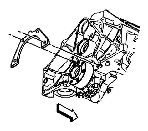
Fig. 289: Locating Crankshaft Rear Oil Seal Housing Gasket Courtesy of GENERAL MOTORS COMPANY
