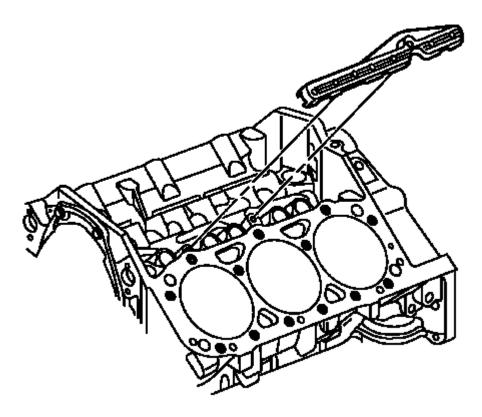
Fig. 647: View Of Valve Lifter Pushrod Guides Courtesy of GENERAL MOTORS COMPANY
