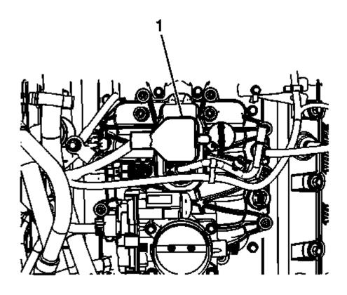
Fig. 61: View Of Control Port Injector Module Courtesy of GENERAL MOTORS COMPANY
