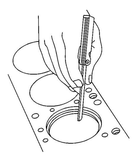
Fig. 438: Measuring Piston Ring End Gap Courtesy of GENERAL MOTORS COMPANY
