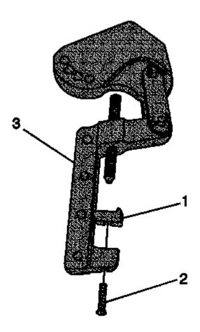
Fig. 456: Pivot Arm Assembly Foot & Bolt Courtesy of GENERAL MOTORS COMPANY
