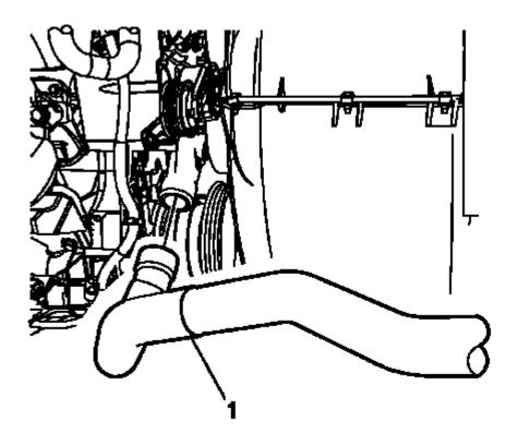
Fig. 301: Radiator Outlet Hose Courtesy of GENERAL MOTORS COMPANY
