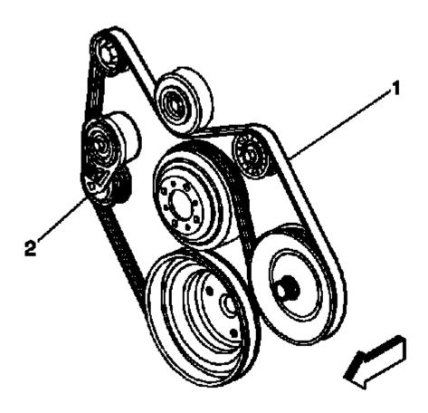
Fig. 12: Drive Belt Routing & Tensioner (W/O A/C)
