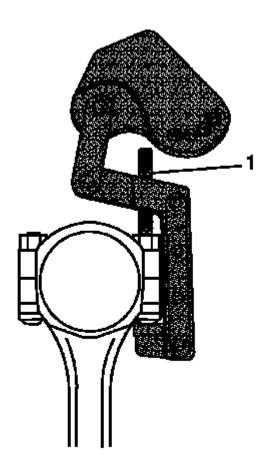
Fig. 459: Small End Of Connecting Rod Bolt Screw Courtesy of GENERAL MOTORS COMPANY
