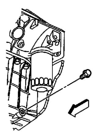
Fig. 254: Identifying Oil Drain Plug Courtesy of GENERAL MOTORS COMPANY
