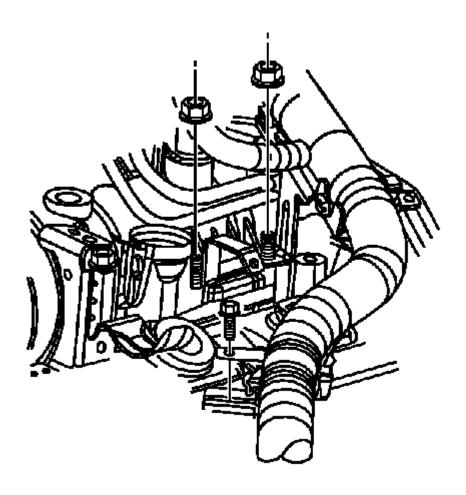
Fig. 100: View Of Engine Wiring Harness Bracket & Nuts Courtesy of GENERAL MOTORS COMPANY
