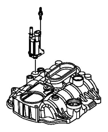
Fig. 548: Purge Solenoid & Nut Courtesy of GENERAL MOTORS COMPANY
