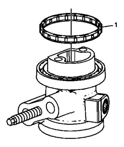
Fig. 227: Identifying Oil Filter Adapter Seal O-Ring Courtesy of GENERAL MOTORS COMPANY
