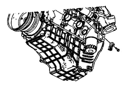
Fig. 412: View Of Knock Sensor & Bolt Courtesy of GENERAL MOTORS COMPANY
