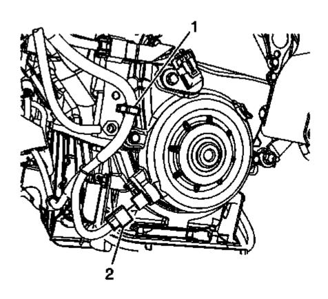
Fig. 188: Crankshaft Position (CKP) Sensor Electrical Connector & Clip Courtesy of GENERAL MOTORS COMPANY
