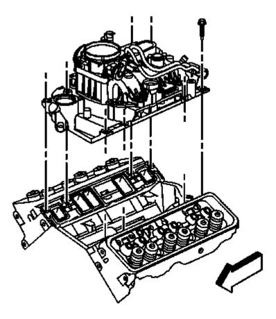
Fig. 77: Intake Manifold Courtesy of GENERAL MOTORS COMPANY
