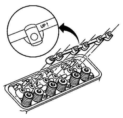
Fig. 665: Locating Arrow On Valve Rocker Arm Support Courtesy of GENERAL MOTORS COMPANY
