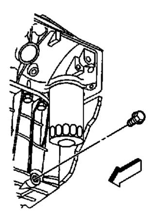
Fig. 326: Identifying Oil Drain Plug Courtesy of GENERAL MOTORS COMPANY
