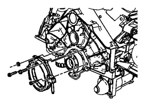
Fig. 287: Crankshaft Rear Oil Seal Housing Courtesy of GENERAL MOTORS COMPANY
