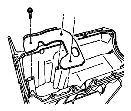
Fig. 537: View Of Oil Pan Baffle Bolts & Baffle Courtesy of GENERAL MOTORS COMPANY
