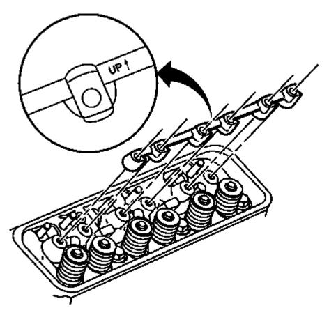
Fig. 111: Locating Arrow On Valve Rocker Arm Support **Courtesy of GENERAL MOTORS COMPANY**
