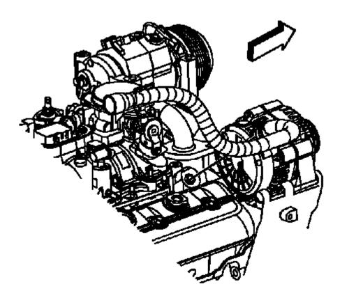
Fig. 89: Heater Inlet Hose At Water Pump Courtesy of GENERAL MOTORS COMPANY
