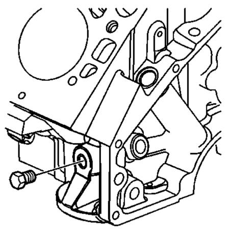
Fig. 696: View Of Engine Block Left Oil Gallery Plug Courtesy of GENERAL MOTORS COMPANY
