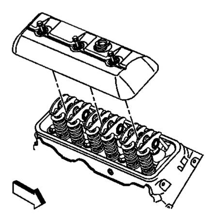
Fig. 105: Rocker Arm Cover Courtesy of GENERAL MOTORS COMPANY
