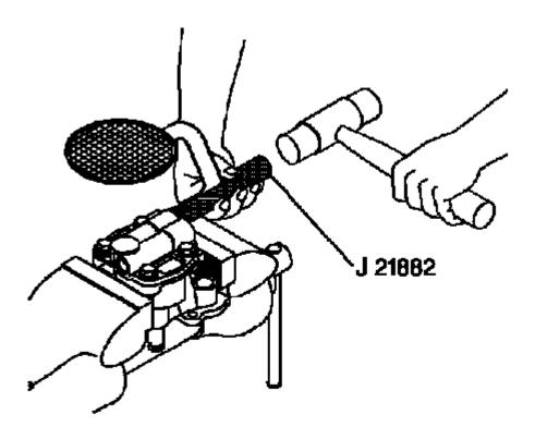
Fig. 534: Oil Pump Screen & Pump Body Courtesy of GENERAL MOTORS COMPANY
