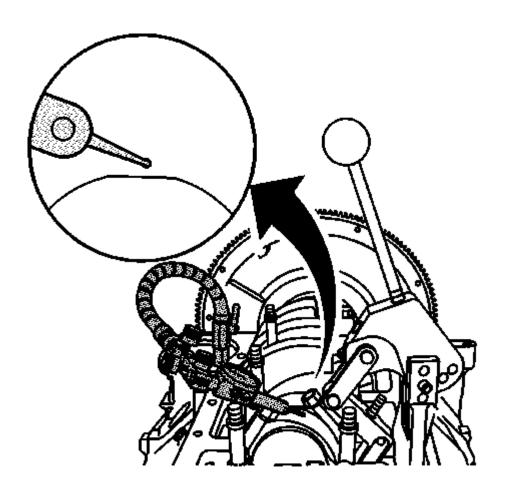
Fig. 469: Proper Indicator Positioning Courtesy of GENERAL MOTORS COMPANY
