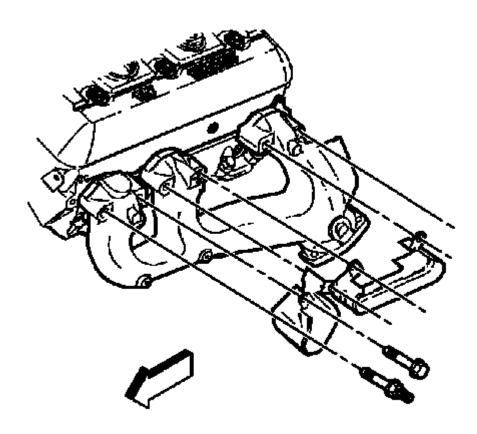
Fig. 331: View Of Exhaust Manifold Bolts & Studs Courtesy of GENERAL MOTORS COMPANY
