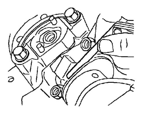
Fig. 479: Measuring Connecting Rod Side Clearance Courtesy of GENERAL MOTORS COMPANY
