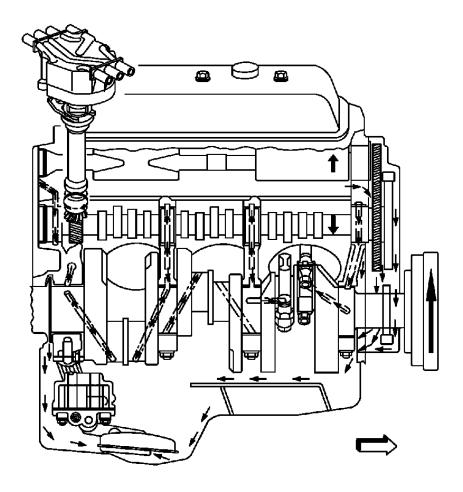
Fig. 698: Cutaway View Of Engine Lubrication System Courtesy of GENERAL MOTORS COMPANY
