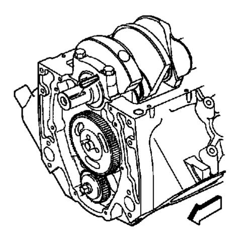
Fig. 395: Locating Crankshaft Balancer Key Courtesy of GENERAL MOTORS COMPANY
