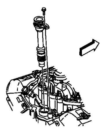
Fig. 352: View Of Oil Pump Drive Shaft Courtesy of GENERAL MOTORS COMPANY
