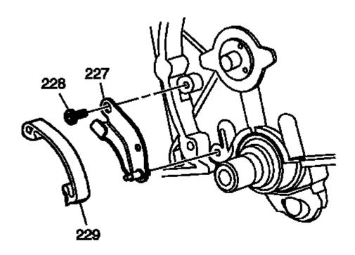
Fig. 390: View Of Timing Chain Tensioner Bracket, Bolt & Shoe Courtesy of GENERAL MOTORS COMPANY
