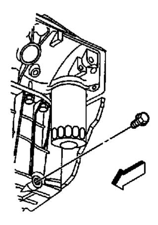
Fig. 636: Identifying Oil Drain Plug Courtesy of GENERAL MOTORS COMPANY
