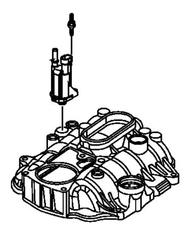
Fig. 557: Purge Solenoid & Nut Courtesy of GENERAL MOTORS COMPANY
