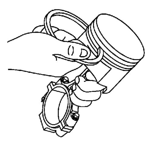
Fig. 434: Inserting Piston Ring Into Ring Groove Courtesy of GENERAL MOTORS COMPANY
