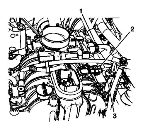
Fig. 60: View Of Throttle Body Actuator, Manifold Absolute Pressure (MAP) Sensor & Evaporative Emission (EVAP) Canister Purge Solenoid Valve Courtesy of GENERAL MOTORS COMPANY
