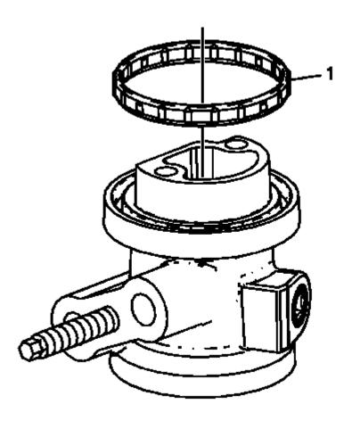
Fig. 637: Identifying Oil Filter Adapter Seal O-Ring Courtesy of GENERAL MOTORS COMPANY
