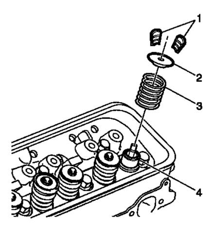
Fig. 121: Identifying Valve Components
