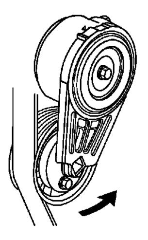
Fig. 8: Releasing Drive Belt Tension
