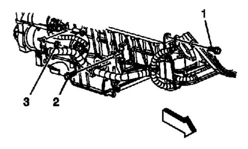
Fig. 321: Positive Battery Cable Clip Bolt Courtesy of GENERAL MOTORS COMPANY
