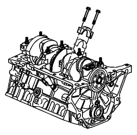
Fig. 604: View Of Bearing, Bearing Cap & Bolts Courtesy of GENERAL MOTORS COMPANY
