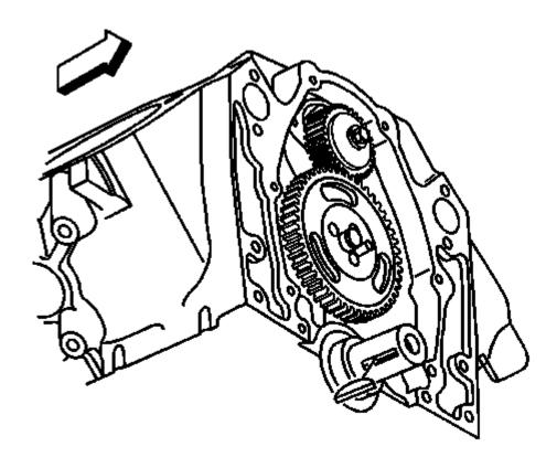
Fig. 199: Crankshaft Balancer Key Courtesy of GENERAL MOTORS COMPANY
