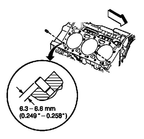
Fig. 157: Installing Cylinder Head Locator Pins Courtesy of GENERAL MOTORS COMPANY
