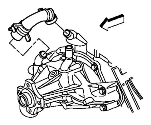
Fig. 688: View Of Water Pump Inlet Hose & Clamps Courtesy of GENERAL MOTORS COMPANY
