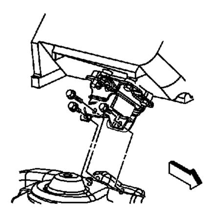
Fig. 309: View Of Right Side (Left Side Similar) Engine Mount To Engine Mount Bracket Bolts Courtesy of GENERAL MOTORS COMPANY
