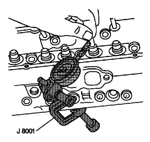
Fig. 514: Measuring Valve Stem-To-Guide Clearance Using J 8001 Courtesy of GENERAL MOTORS COMPANY
