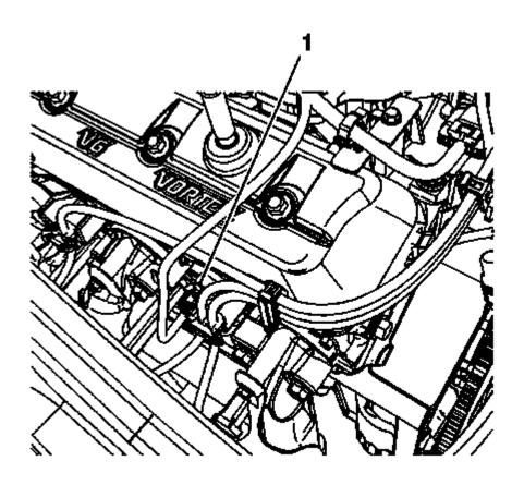
Fig. 99: View Of Engine Coolant Temperature (ECT) Sensor Electrical Connector Courtesy of GENERAL MOTORS COMPANY
