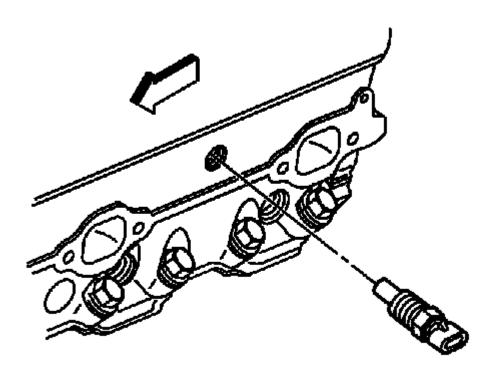
Fig. 359: View Of Engine Coolant Temperature Sensor Courtesy of GENERAL MOTORS COMPANY
