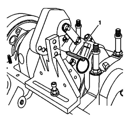
Fig. 463: Inserting Pin Courtesy of GENERAL MOTORS COMPANY
