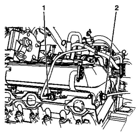
Fig. 147: View Of Harness Ground Bolt Courtesy of GENERAL MOTORS COMPANY
