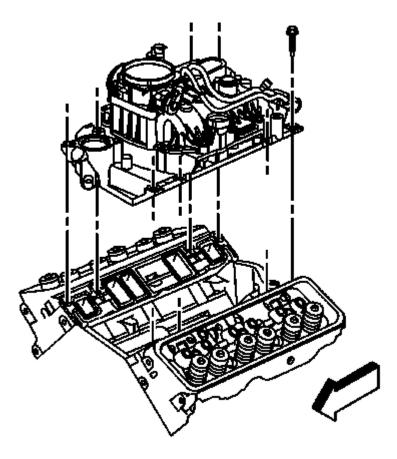
Fig. 73: Intake Manifold Courtesy of GENERAL MOTORS COMPANY
