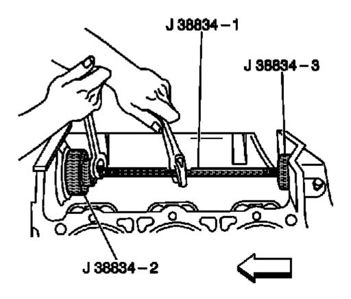
Fig. 497: Installing Balance Shaft Rear Bearing Courtesy of GENERAL MOTORS COMPANY
