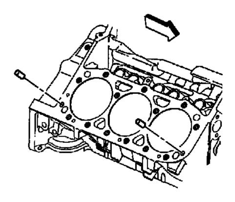
Fig. 156: Cylinder Head Locator Pins Courtesy of GENERAL MOTORS COMPANY
