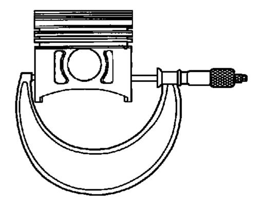
Fig. 599: Measuring Piston Outside Diameter Using Micrometer Courtesy of GENERAL MOTORS COMPANY
