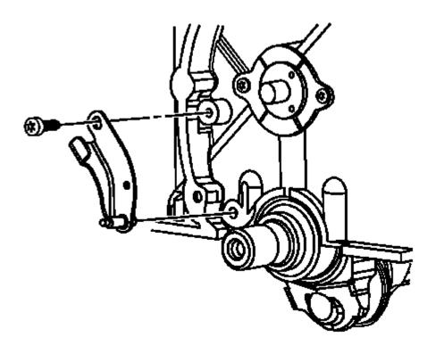
Fig. 198: Timing Chain Tensioner Bracket
