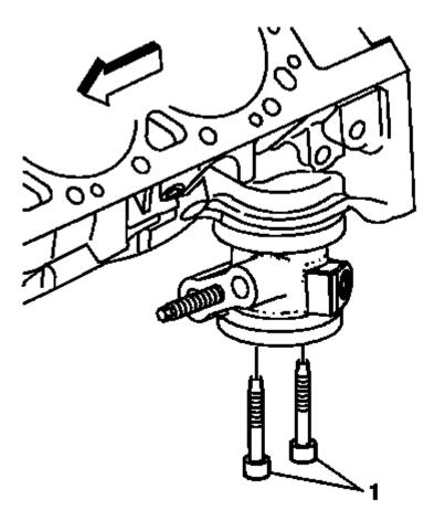
Fig. 229: Identifying Oil Filter Adapter Bolts
