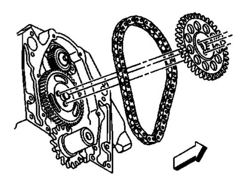
Fig. 201: Camshaft Sprocket & Camshaft Timing Chain Courtesy of GENERAL MOTORS COMPANY
