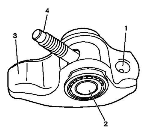
Fig. 500: Pushrod Socket, Roller Pivot & Valve Stem Tip Courtesy of GENERAL MOTORS COMPANY
