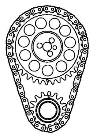
Fig. 191: View Of Camshaft & Crankshaft Sprocket Timing Marks Courtesy of GENERAL MOTORS COMPANY
