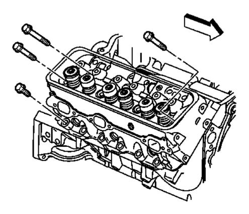
Fig. 660: Locating Cylinder Head Bolts (Right)
