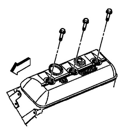
Fig. 344: Valve Rocker Arm Cover Bolts (Left)
