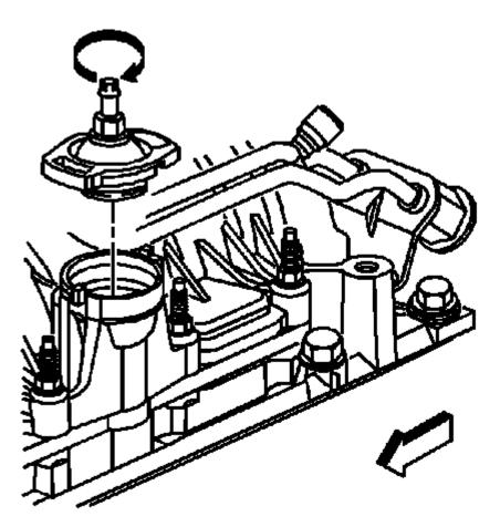
Fig. 53: PCV Valve Cover Courtesy of GENERAL MOTORS COMPANY
