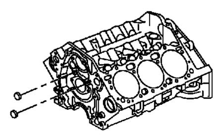
Fig. 572: Front Of Engine Block Front Oil Gallery Plugs Or Balls Courtesy of GENERAL MOTORS COMPANY
