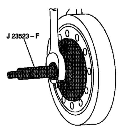
Fig. 170: Installing Crankshaft Balancer Using J 23523-F Courtesy of GENERAL MOTORS COMPANY
