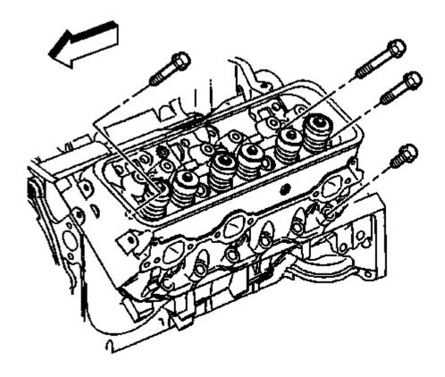
Fig. 136: Locating Cylinder Head Bolts (Left)
