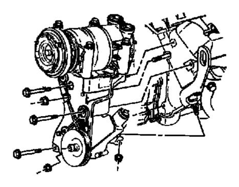
Fig. 79: View Of Power Steering Pump Bracket Courtesy of GENERAL MOTORS COMPANY
