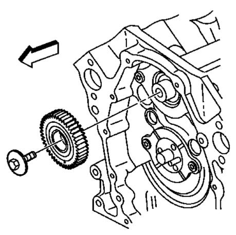
Fig. 397: Locating Balance Shaft Driven Gear Courtesy of GENERAL MOTORS COMPANY
