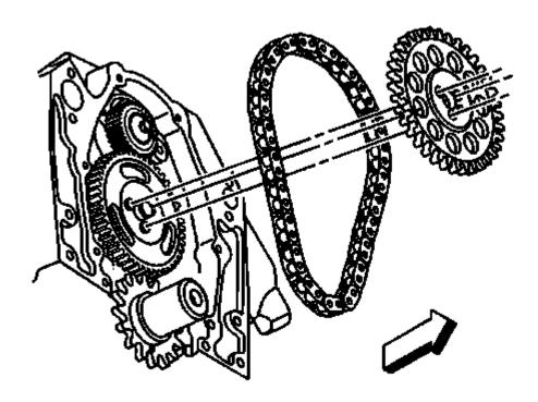
Fig. 194: Camshaft Sprocket & Camshaft Timing Chain Courtesy of GENERAL MOTORS COMPANY
