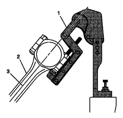
Fig. 462: Pivot Arm Assembly Link, Plane & Connecting Rod Beam Courtesy of GENERAL MOTORS COMPANY
