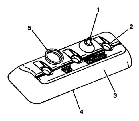
Fig. 536: Valve Rocker Arm Cover Courtesy of GENERAL MOTORS COMPANY
