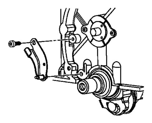
Fig. 197: Timing Chain Tensioner Bracket
