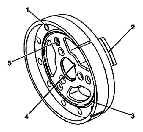
Fig. 480: Crankshaft Balancer Cleaning & Inspection Areas Courtesy of GENERAL MOTORS COMPANY
