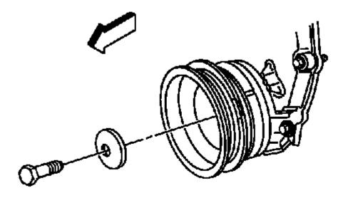
Fig. 340: View Of Crankshaft Balancer Washer & Bolt Courtesy of GENERAL MOTORS COMPANY
