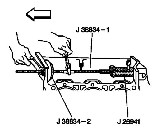
Fig. 494: Balance Shaft Rear Bearing Courtesy of GENERAL MOTORS COMPANY
