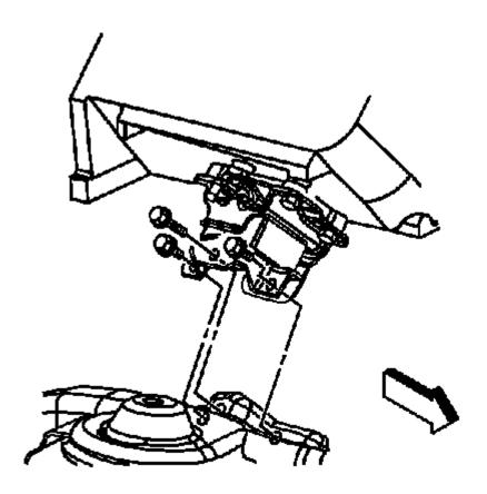
Fig. 27: View Of Right Side (Left Side Similar) Engine Mount To Engine Mount Bracket Bolts Courtesy of GENERAL MOTORS COMPANY
