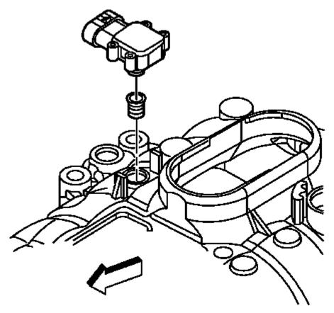
Fig. 48: MAP Sensor Courtesy of GENERAL MOTORS COMPANY
