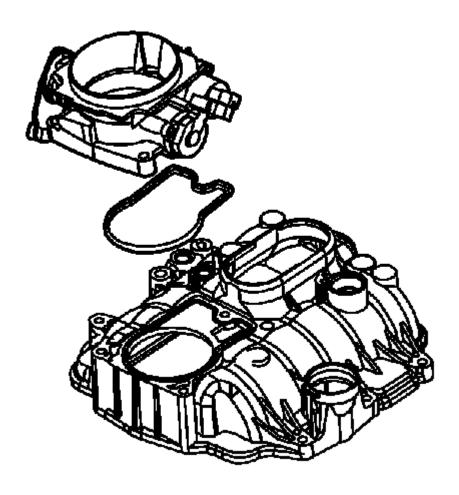
Fig. 563: View Of Throttle Body & Gasket Courtesy of GENERAL MOTORS COMPANY
