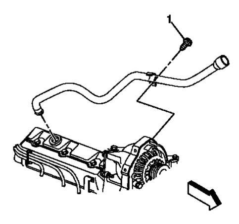
Fig. 36: View Oil Fill Tube Bolt Courtesy of GENERAL MOTORS COMPANY
