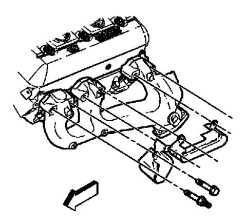
Fig. 691: View Of Exhaust Manifold Bolts & Studs Courtesy of GENERAL MOTORS COMPANY
