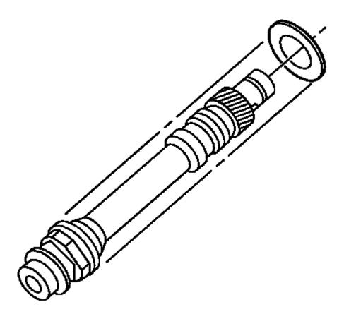
Fig. 675: Oil Pump Drive Shaft & Gasket Courtesy of GENERAL MOTORS COMPANY
