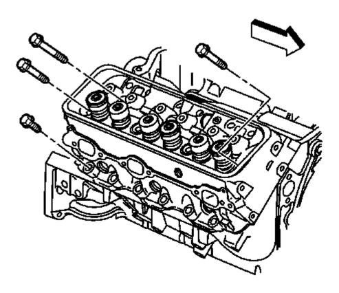
Fig. 160: Locating Cylinder Head Bolts (Right)
