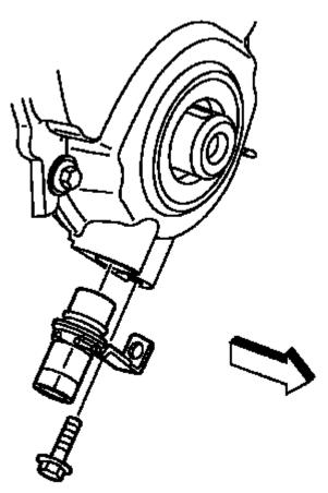
Fig. 626: View Of CKP Sensor & Bolt Courtesy of GENERAL MOTORS COMPANY
