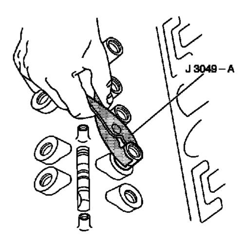
Fig. 127: Using J 3049-A To Remove Sticking Valve Lifters Courtesy of GENERAL MOTORS COMPANY
