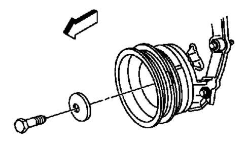
Fig. 173: View Of Crankshaft Balancer Washer & Bolt Courtesy of GENERAL MOTORS COMPANY
