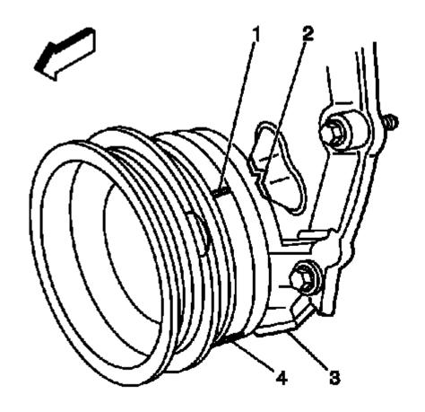
Fig. 668: View Of Crankshaft Balancer Alignment Mark & Engine Front Cover Alignment Tab Courtesy of GENERAL MOTORS COMPANY
