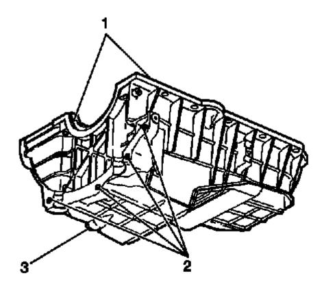
Fig. 538: Oil Pan Cleaning & Inspection Areas Courtesy of GENERAL MOTORS COMPANY
