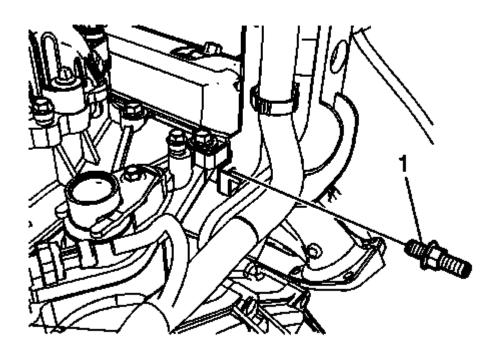
Fig. 68: Engine Wiring Harness Bracket Stud Courtesy of GENERAL MOTORS COMPANY
