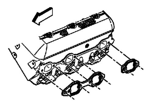
Fig. 690: Exhaust Manifold Gaskets
