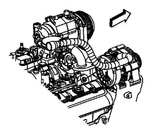
Fig. 63: Heater Inlet Hose At Water Pump Courtesy of GENERAL MOTORS COMPANY
