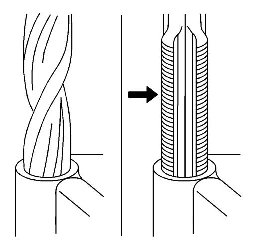
Fig. 569: Drilling & Tapping Damaged Threads Courtesy of GENERAL MOTORS COMPANY
