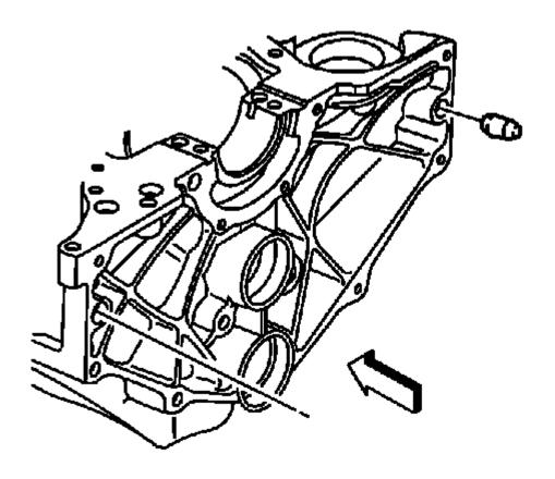
Fig. 417: Identifying Transmission Locator Dowel Straight Pin Courtesy of GENERAL MOTORS COMPANY
