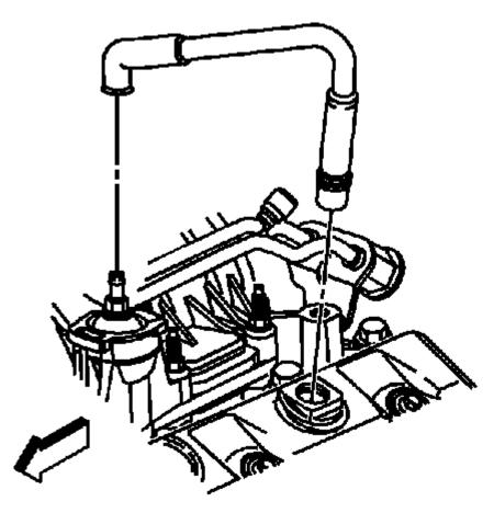
Fig. 93: Locating PCV Valve Hose At Valve & Rocker Cover Courtesy of GENERAL MOTORS COMPANY
