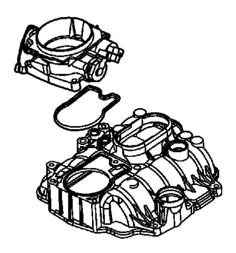
Fig. 542: View Of Throttle Body & Gasket Courtesy of GENERAL MOTORS COMPANY
