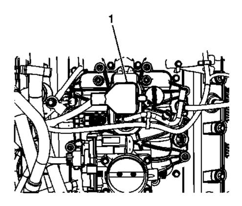
Fig. 87: View Of Control Port Injector Module Courtesy of GENERAL MOTORS COMPANY
