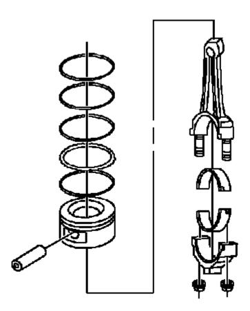
Fig. 430: Piston & Connecting Rod Components Courtesy of GENERAL MOTORS COMPANY
