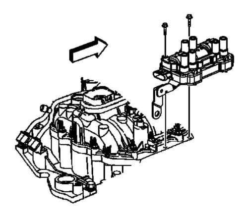
Fig. 545: View Of Studs And Ignition Coil Courtesy of GENERAL MOTORS COMPANY
