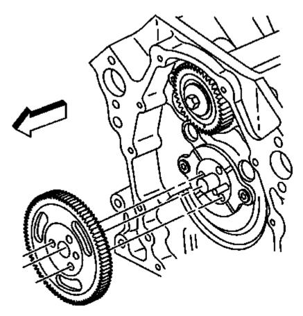
Fig. 212: View Of Balance Shaft Drive Gear Courtesy of GENERAL MOTORS COMPANY
