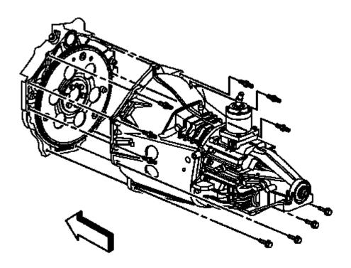
Fig. 257: Manual Transmission Bolts
