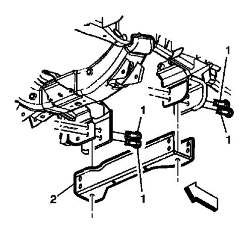
Fig. 238: View Of Crossbar Bolts & Bar (2WD)
