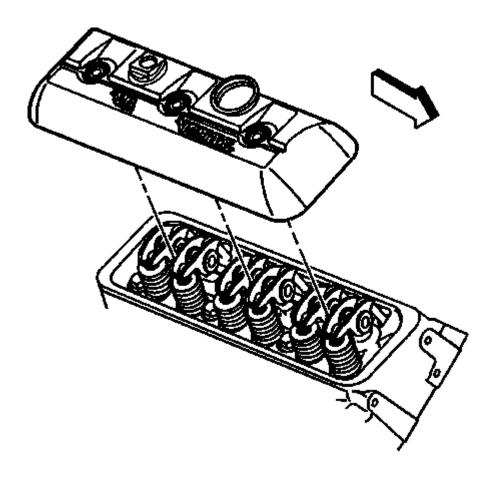
Fig. 683: Valve Rocker Arm Cover (Right)
