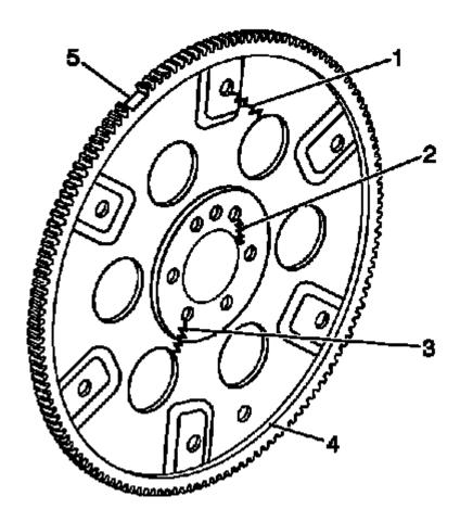
Fig. 482: Flywheel Inspection Areas (Automatic Transmission)
