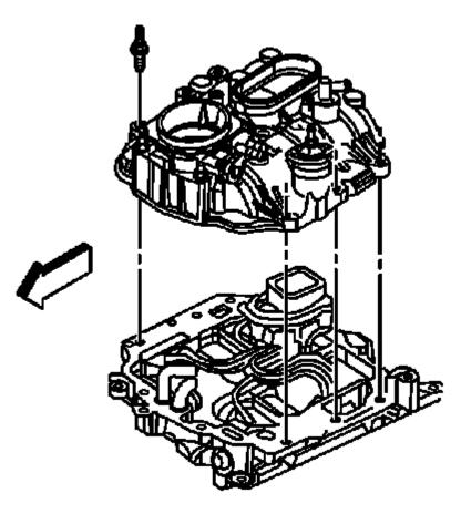
Fig. 42: Upper Intake Manifold Courtesy of GENERAL MOTORS COMPANY
