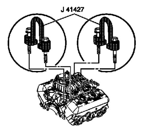
Fig. 307: Engine Lift Brackets J 41427 Courtesy of GENERAL MOTORS COMPANY
