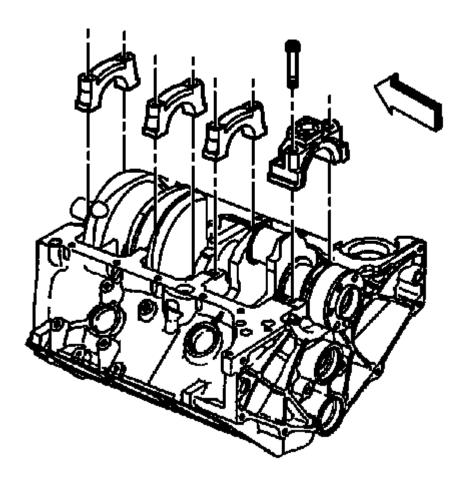
Fig. 477: Crankshaft Bearing Caps Courtesy of GENERAL MOTORS COMPANY
