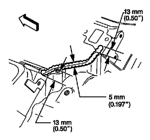
Fig. 671: Applying Adhesive To Rear Top Of Engine Block Courtesy of GENERAL MOTORS COMPANY
