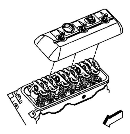
Fig. 97: Rocker Arm Cover Courtesy of GENERAL MOTORS COMPANY
