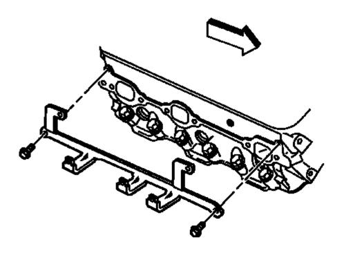
Fig. 368: Spark Plug Wire Support
