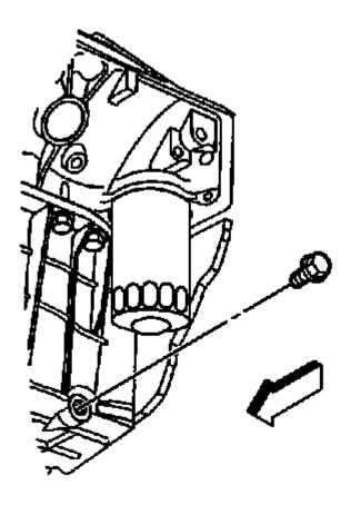
Fig. 236: Identifying Oil Drain Plug Courtesy of GENERAL MOTORS COMPANY
