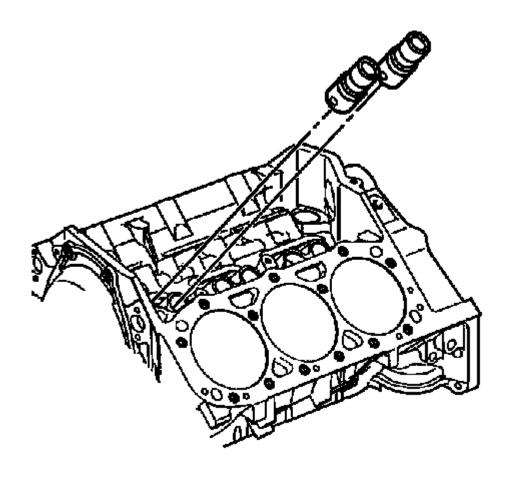
Fig. 126: View Of Valve Lifters
