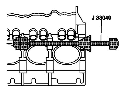
Fig. 493: Removing/Installation Camshaft Inner Bearing Using J 33049 Courtesy of GENERAL MOTORS COMPANY
