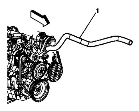
Fig. 81: View Of Radiator Inlet Hose Courtesy of GENERAL MOTORS COMPANY
