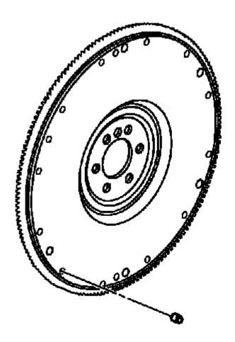
Fig. 292: Locating Flywheel Weights (Manual Transmission)
