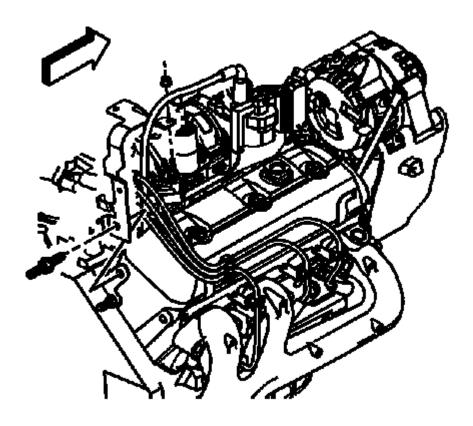
Fig. 312: View Of Engine Wiring Harness Rear Bracket Nut Courtesy of GENERAL MOTORS COMPANY
