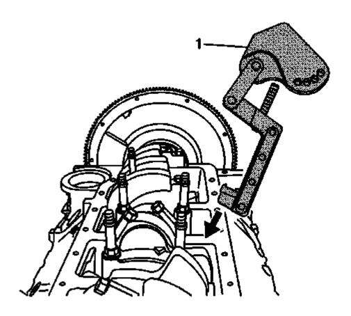
Fig. 458: Pivot Arm Assembly & Connecting Rod Courtesy of GENERAL MOTORS COMPANY
