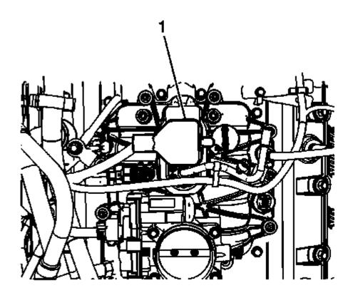
Fig. 38: View Of Control Port Injector Module Courtesy of GENERAL MOTORS COMPANY
