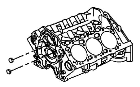
Fig. 422: Front Of Engine Block Front Oil Gallery Plugs Or Balls Courtesy of GENERAL MOTORS COMPANY
