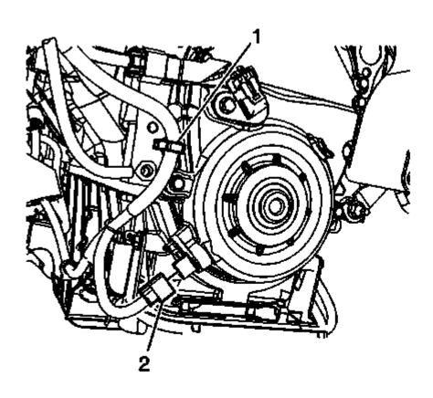
Fig. 177: Crankshaft Position (CKP) Sensor Electrical Connector & Clip Courtesy of GENERAL MOTORS COMPANY
