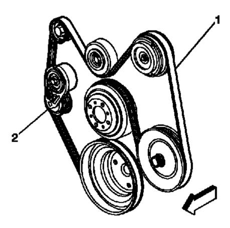
Fig. 10: Drive Belt Routing & Tensioner (W/ A/C)
