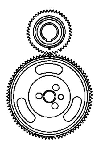
Fig. 615: Aligning Balance Shaft Drive Gear & Balance Shaft Driven Gear Timing Marks Courtesy of GENERAL MOTORS COMPANY
