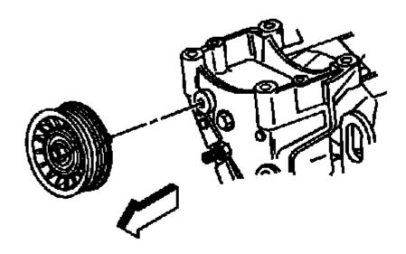
Fig. 18: Drive Belt Idler Pulley (W/O AC)
