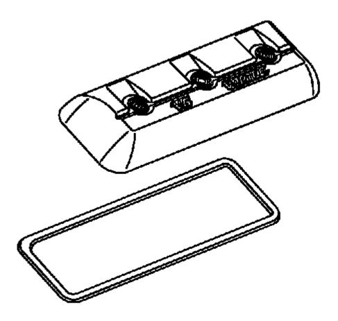
Fig. 95: View Of Rocker Arm Cover And Gasket Courtesy of GENERAL MOTORS COMPANY
