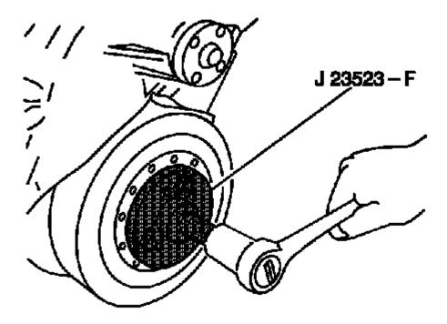
Fig. 166: Removing Crankshaft Balancer Using J 23523-F Courtesy of GENERAL MOTORS COMPANY
