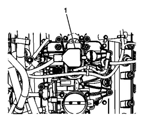
Fig. 65: View Of Control Port Injector Module Courtesy of GENERAL MOTORS COMPANY
