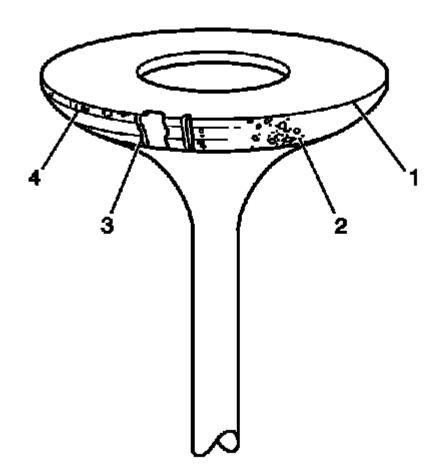
Fig. 518: Inspecting Valve Face For Burning, Pitting & Cracking Courtesy of GENERAL MOTORS COMPANY
