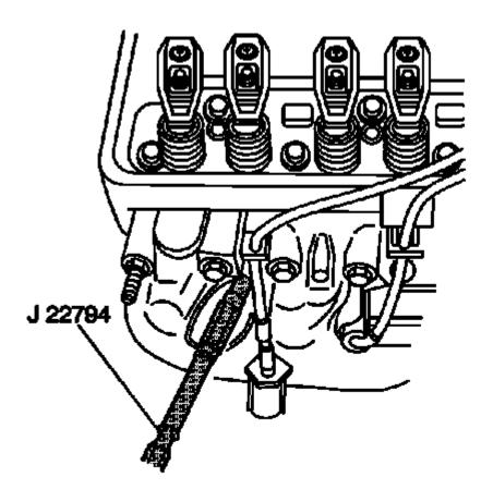
Fig. 124: View Of J 22794 In Spark Plug Hole Courtesy of GENERAL MOTORS COMPANY
