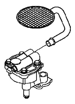
Fig. 524: View Of Oil Pump Pipe & Screen
