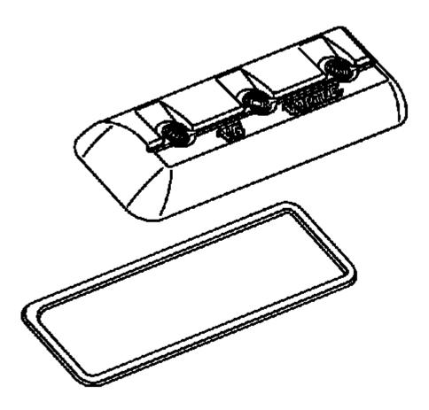
Fig. 104: View Of Rocker Arm Cover And Gasket Courtesy of GENERAL MOTORS COMPANY
