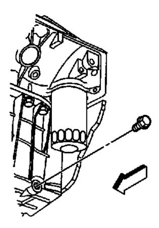
Fig. 323: Identifying Oil Drain Plug Courtesy of GENERAL MOTORS COMPANY
