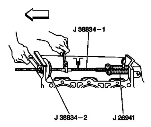
Fig. 217: Balance Shaft Rear Bearing Courtesy of GENERAL MOTORS COMPANY
