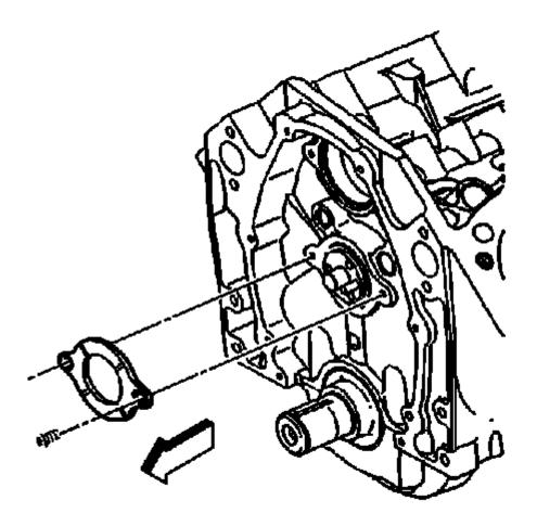
Fig. 223: View Of Camshaft Retainer & Bolts Courtesy of GENERAL MOTORS COMPANY
