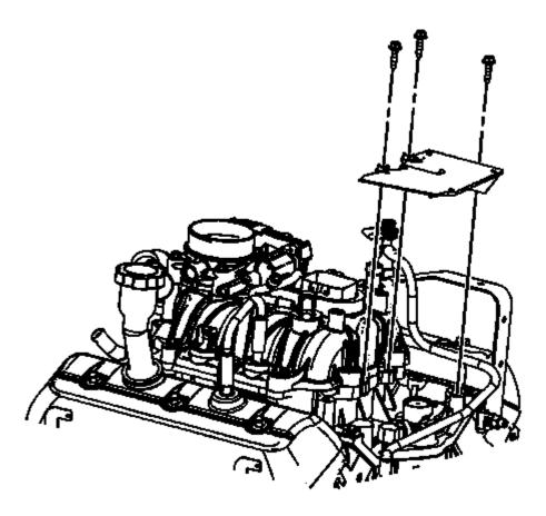
Fig. 677: View Of Ignition Coil Bracket & Bolts Courtesy of GENERAL MOTORS COMPANY
