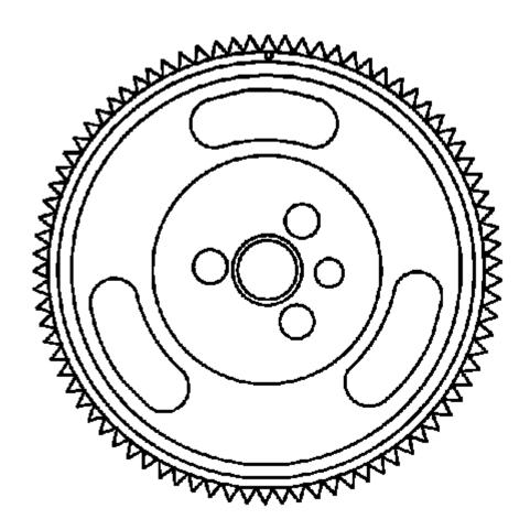
Fig. 496: Balance Shaft Drive Gear Camshaft Timing Mark Courtesy of GENERAL MOTORS COMPANY
