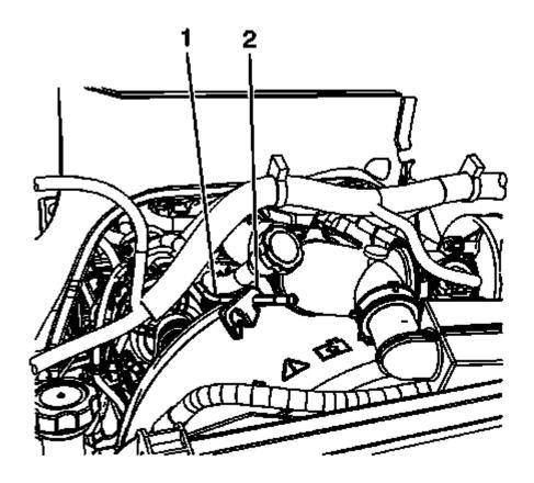
Fig. 279: View Of Oil Level Indicator Tube & Air Conditioning Line Retainer Clip Courtesy of GENERAL MOTORS COMPANY
