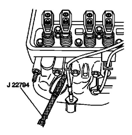
Fig. 115: View Of J 22794 In Spark Plug Hole **Courtesy of GENERAL MOTORS COMPANY**
