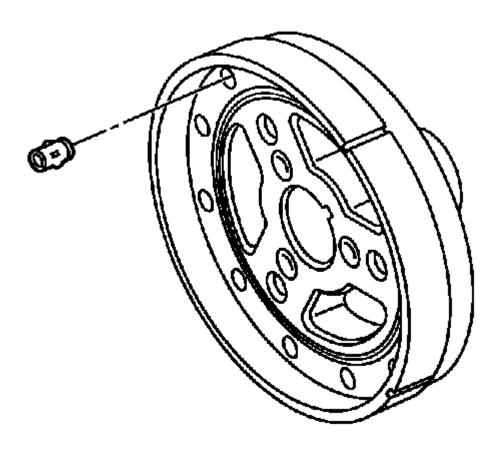
Fig. 168: View Of Crankshaft Balancer Weights Courtesy of GENERAL MOTORS COMPANY
