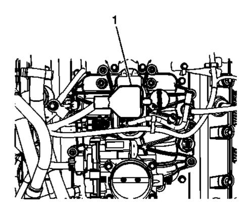
Fig. 303: View Of Control Port Injector Module Courtesy of GENERAL MOTORS COMPANY
