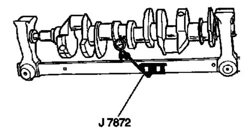
Fig. 447: Measuring Crankshaft Runout Courtesy of GENERAL MOTORS COMPANY
