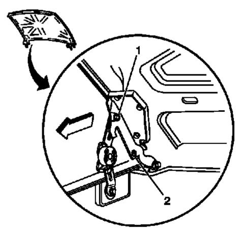
Fig. 295: Identifying Hood Hinge Normal And Service Position Bolt Holes Courtesy of GENERAL MOTORS COMPANY
