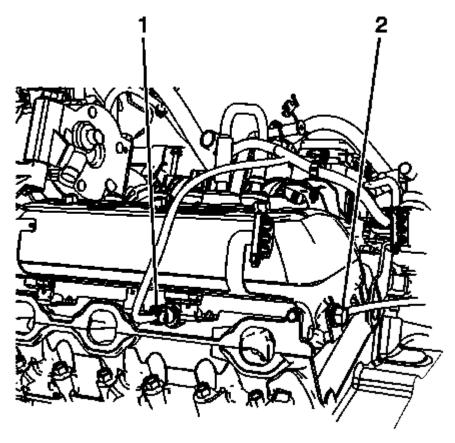
Fig. 133: View Of Harness Ground Bolt Courtesy of GENERAL MOTORS COMPANY
