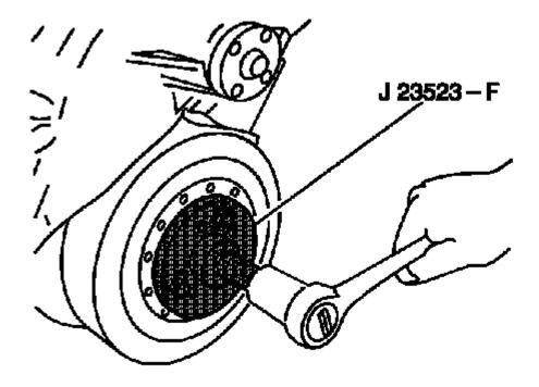
Fig. 342: Removing Crankshaft Balancer Using J 23523-F Courtesy of GENERAL MOTORS COMPANY
