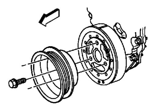
Fig. 643: View Of Crankshaft Pulley & Bolts Courtesy of GENERAL MOTORS COMPANY
