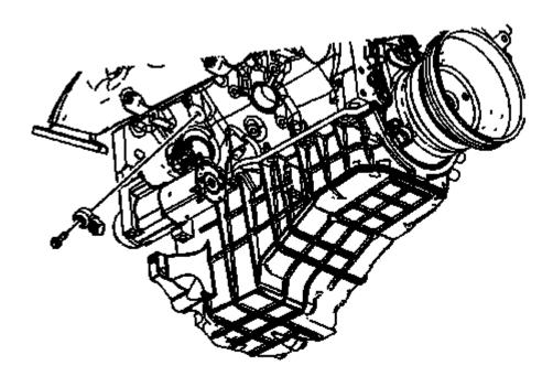
Fig. 413: View Of Knock Sensor & Bolt Courtesy of GENERAL MOTORS COMPANY
