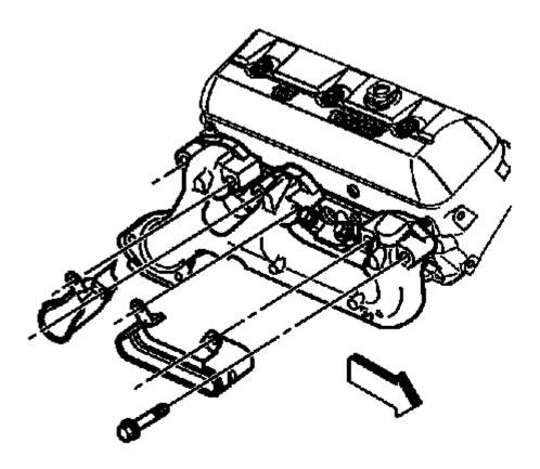
Fig. 693: Exhaust Manifold Bolts
