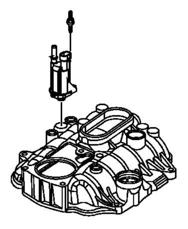
Fig. 49: Purge Solenoid & Nut Courtesy of GENERAL MOTORS COMPANY
