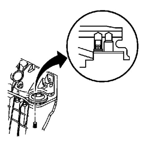
Fig. 234: View Of Oil Filter Bypass Valve Courtesy of GENERAL MOTORS COMPANY
