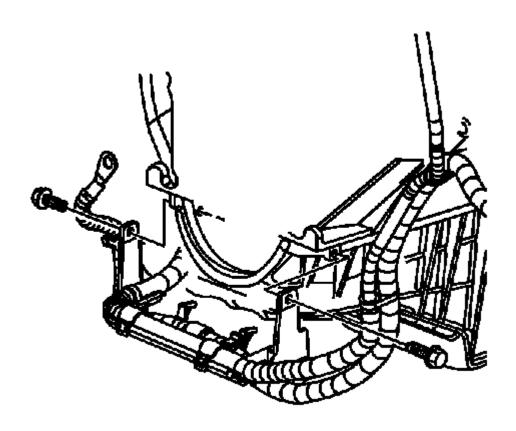
Fig. 320: View Of Battery Cable Bracket Bolts Courtesy of GENERAL MOTORS COMPANY
