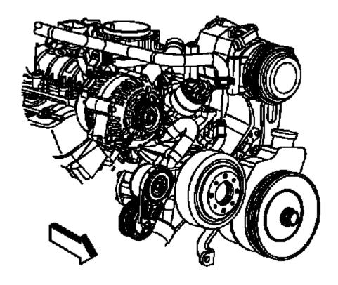
Fig. 90: Intake Manifold Hose Courtesy of GENERAL MOTORS COMPANY
