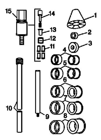
Fig. 492: Camshaft Bearing Service Kit Components Courtesy of GENERAL MOTORS COMPANY
