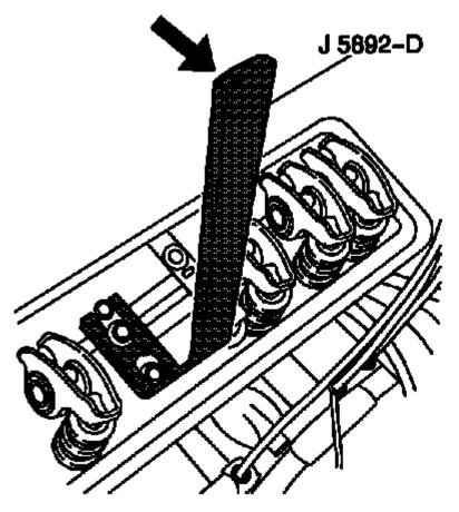
Fig. 116: View Of J 5892--D, Valve Rocker Arm Bolt & Washer Courtesy of GENERAL MOTORS COMPANY
