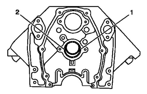
Fig. 491: Locating Camshaft Bearing Lubrication Hole At 3 & 9 O'clock Positions Courtesy of GENERAL MOTORS COMPANY
