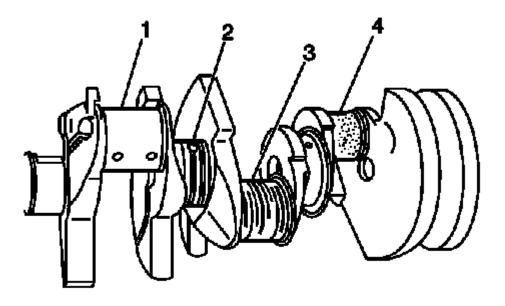
Fig. 444: Identifying Different Crankshaft Journal Wear Patterns Courtesy of GENERAL MOTORS COMPANY
