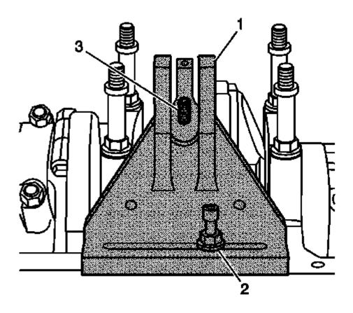
Fig. 461: Aligning Center Of Base W/Pivot Arm Assembly Screw Courtesy of GENERAL MOTORS COMPANY
