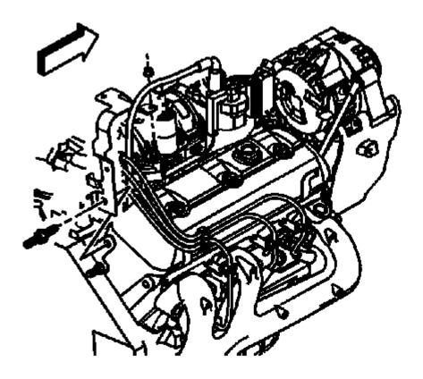
Fig. 305: View Of Engine Wiring Harness Rear Bracket Nut Courtesy of GENERAL MOTORS COMPANY
