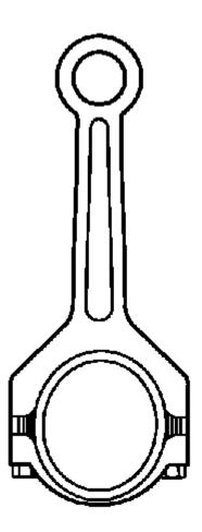
Fig. 436: View Of Connecting Rod Courtesy of GENERAL MOTORS COMPANY
