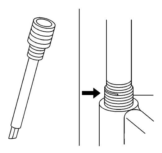
Fig. 570: View Of Thread Insert Courtesy of GENERAL MOTORS COMPANY
