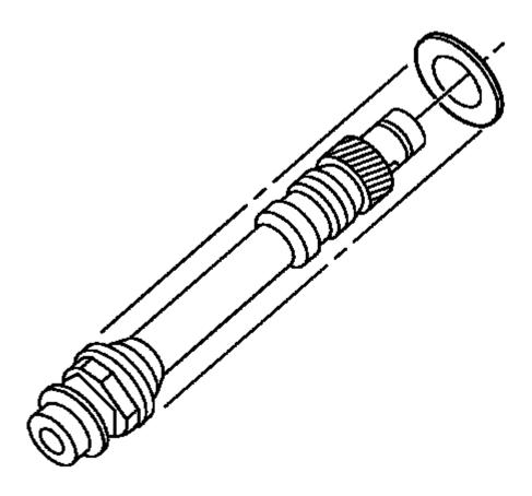
Fig. 353: Oil Pump Drive Shaft & Gasket Courtesy of GENERAL MOTORS COMPANY
