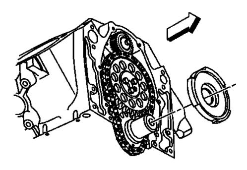
Fig. 189: CKP Sensor Reluctor Ring Courtesy of GENERAL MOTORS COMPANY
