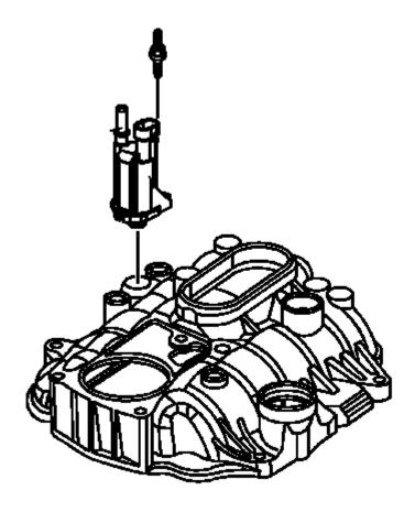
Fig. 50: Purge Solenoid & Nut Courtesy of GENERAL MOTORS COMPANY
