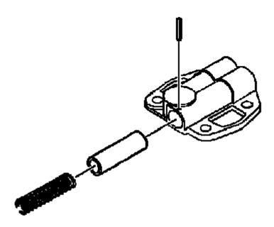
Fig. 530: View Of Oil Pump Pressure Relief Valve, Spring & Spring Straight Pin Courtesy of GENERAL MOTORS COMPANY
