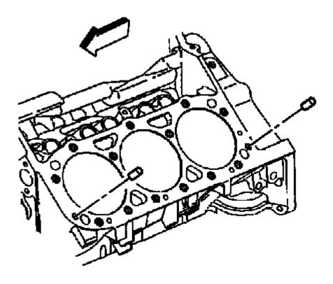
Fig. 139: View Of Cylinder Head Locator Pins Courtesy of GENERAL MOTORS COMPANY
