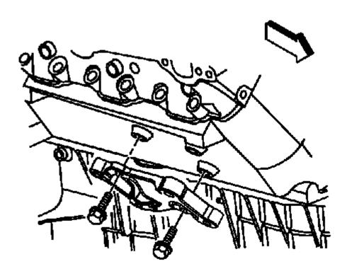
Fig. 24: View Of Right Side (Left Side Similar) Engine Mount Side Bracket & Bolts Courtesy of GENERAL MOTORS COMPANY
