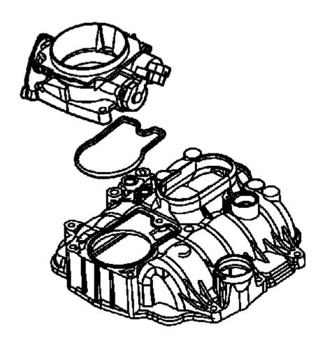
Fig. 52: View Of Throttle Body & Gasket Courtesy of GENERAL MOTORS COMPANY
