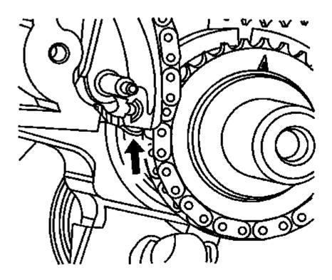
Fig. 202: Timing Chain Tensioner Shoe Courtesy of GENERAL MOTORS COMPANY
