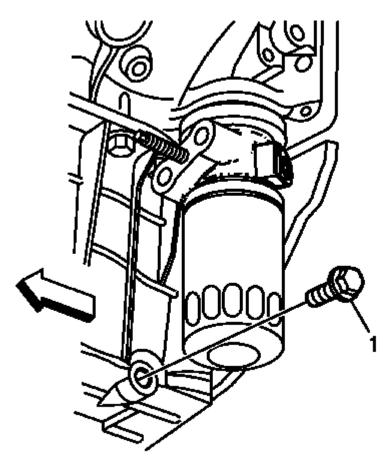
Fig. 327: Identifying Oil Pan Drain Plug Courtesy of GENERAL MOTORS COMPANY
