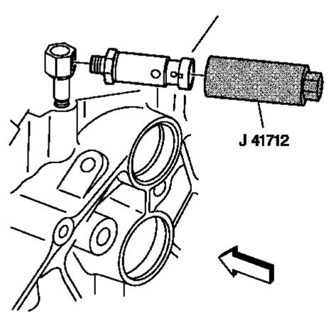
Fig. 415: View Of Engine Oil Pressure Gage Sensor Courtesy of GENERAL MOTORS COMPANY
