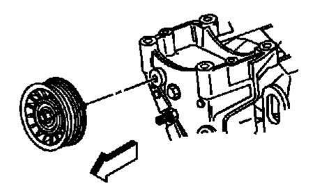
Fig. 17: Drive Belt Idler Pulley (W/O AC)
