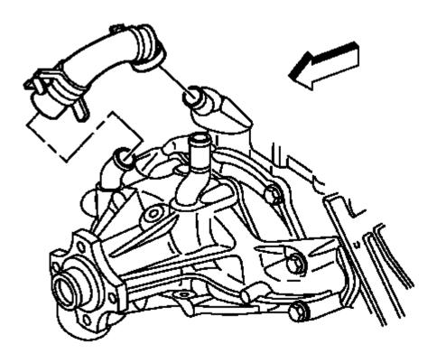
Fig. 80: View Of Water Pump Inlet Hose & Clamps Courtesy of GENERAL MOTORS COMPANY
