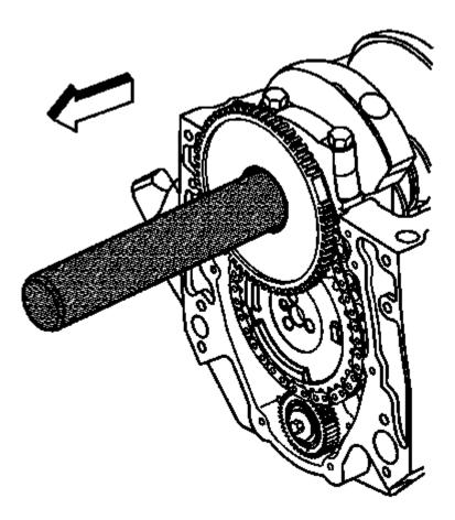
Fig. 622: Installing Crankshaft Position Sensor Reluctor Ring Courtesy of GENERAL MOTORS COMPANY
