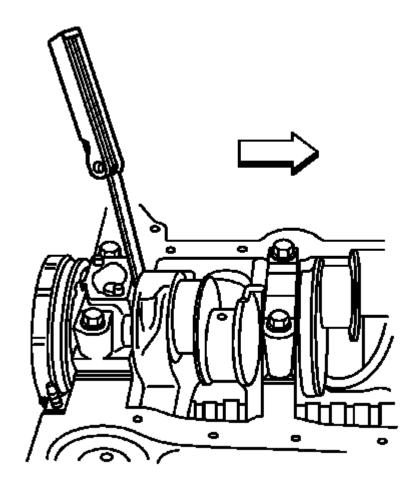
Fig. 591: Measuring Crankshaft End Play Courtesy of GENERAL MOTORS COMPANY
