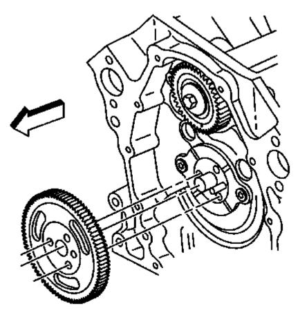
Fig. 611: View Of Balance Shaft Drive Gear Courtesy of GENERAL MOTORS COMPANY
