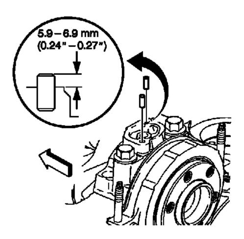
Fig. 627: Oil Pump Locator Pins
