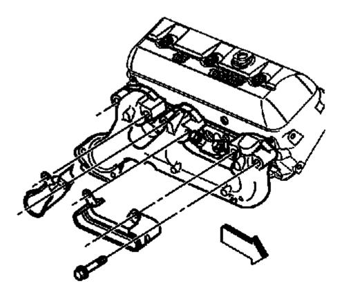
Fig. 333: Exhaust Manifold Bolts
