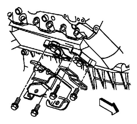
Fig. 32: View Of Right Side (Left Side Similar) Engine Mount Bolts Courtesy of GENERAL MOTORS COMPANY
