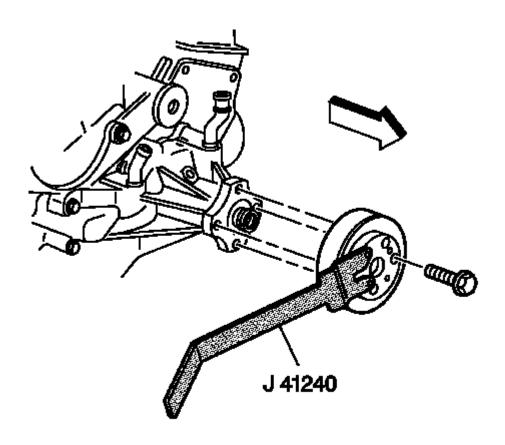
Fig. 337: View Of Fan, Water Pump Pulley & Bolts Courtesy of GENERAL MOTORS COMPANY
