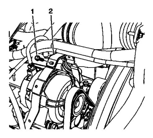
Fig. 278: Oil Level Indicator Tube Bolt & Bracket Courtesy of GENERAL MOTORS COMPANY
