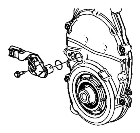
Fig. 387: Camshaft Position Sensor & Bolt Courtesy of GENERAL MOTORS COMPANY
