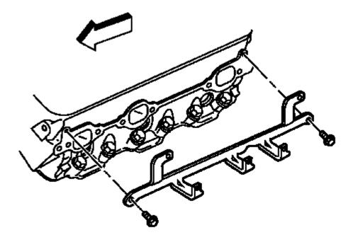
Fig. 145: Locating Spark Plug Wire Support Courtesy of GENERAL MOTORS COMPANY
