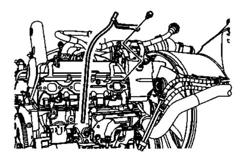
Fig. 275: Oil Level Indicator Tube Bolt & Tube Courtesy of GENERAL MOTORS COMPANY
