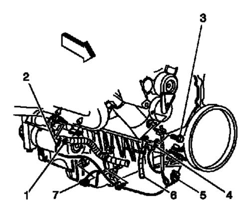
Fig. 299: View Of Oil Level Sensor Electrical Connector, CKP Electrical Connector & Battery Ground Bolt
