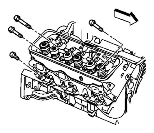
Fig. 153: Locating Cylinder Head Bolts (Right)
