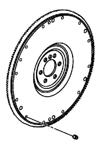
Fig. 483: Locating Flywheel Weights (Manual Transmission)
