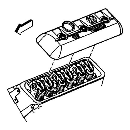
Fig. 680: Valve Rocker Arm Cover (Left)
