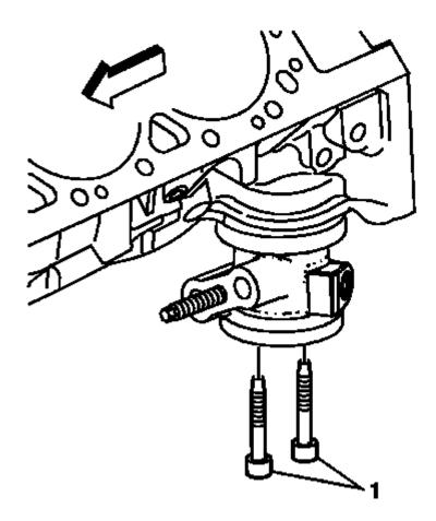
Fig. 224: Identifying Oil Filter Adapter Bolts Courtesy of GENERAL MOTORS COMPANY
