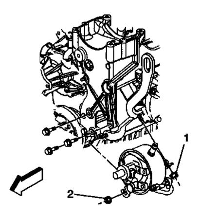
Fig. 150: View Of Power Steering (P/S) Pump Rear Bracket Nut And P/S Pump Rear Bracket Front Nut
