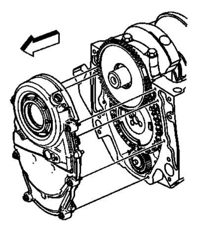
Fig. 388: Engine Front Cover Courtesy of GENERAL MOTORS COMPANY
