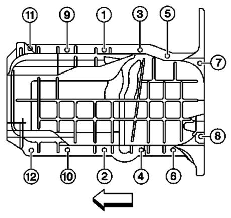
Fig. 635: Oil Pan Bolts & Nuts Tightening Sequence Courtesy of GENERAL MOTORS COMPANY
