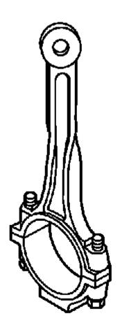
Fig. 437: Identifying Twisted Connecting Rod Courtesy of GENERAL MOTORS COMPANY
