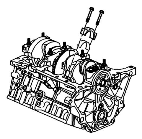
Fig. 403: View Of Bearing, Bearing Cap & Bolts Courtesy of GENERAL MOTORS COMPANY
