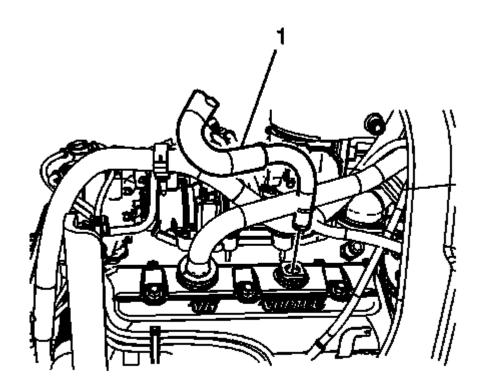
Fig. 101: View Of Positive Crankcase Ventilation (PCV) Hose Courtesy of GENERAL MOTORS COMPANY
