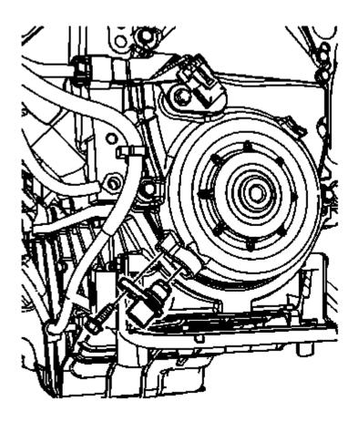
Fig. 178: CKP Sensor Bolt And Sensor Courtesy of GENERAL MOTORS COMPANY
