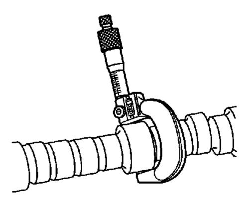
Fig. 487: Measuring Engine Camshaft Journals Courtesy of GENERAL MOTORS COMPANY
