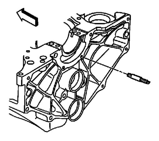
Fig. 407: Locating Crankshaft Rear Oil Seal Housing Retainer Stud **Courtesy of GENERAL MOTORS COMPANY**
