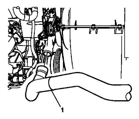
Fig. 316: Radiator Outlet Hose Courtesy of GENERAL MOTORS COMPANY
