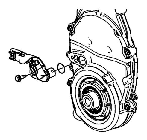
Fig. 624: Camshaft Position Sensor & Bolt Courtesy of GENERAL MOTORS COMPANY
