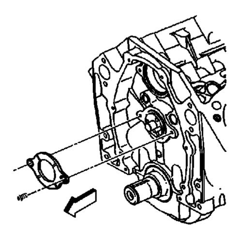
Fig. 607: View Of Camshaft Retainer & Bolts
