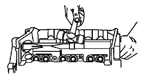
Fig. 208: Removing Balance Shaft
