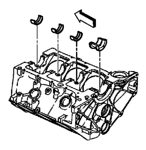
Fig. 473: View Of Crankshaft Bearings At Engine Block Courtesy of GENERAL MOTORS COMPANY
