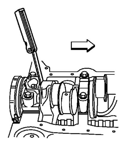
Fig. 448: Measuring Crankshaft End Play Courtesy of GENERAL MOTORS COMPANY
