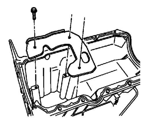
Fig. 539: View Of Oil Pan Baffle Bolts & Baffle Courtesy of GENERAL MOTORS COMPANY
