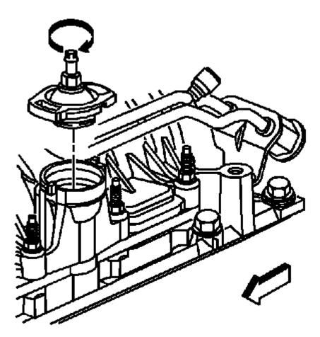
Fig. 46: PCV Valve Cover Courtesy of GENERAL MOTORS COMPANY
