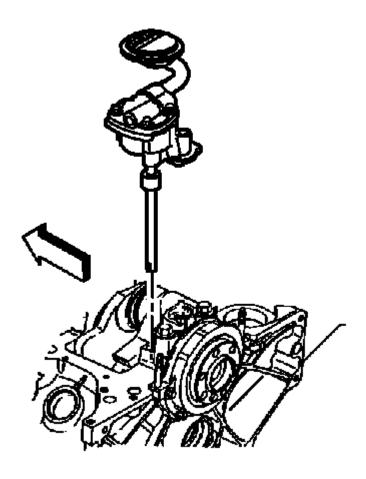
Fig. 628: View Of Oil Pump Courtesy of GENERAL MOTORS COMPANY
