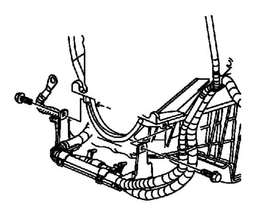
Fig. 239: View Of Battery Cable Bracket Bolts Courtesy of GENERAL MOTORS COMPANY
