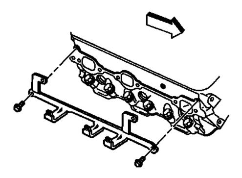
Fig. 662: Spark Plug Wire Support
