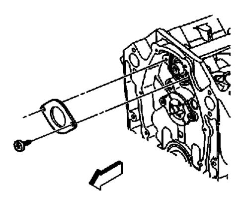
Fig. 609: View of Balance Shaft Retainer & Bolts Courtesy of GENERAL MOTORS COMPANY
