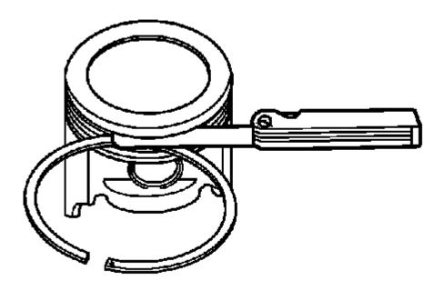
Fig. 435: Measuring Piston Ring Side Clearance Courtesy of GENERAL MOTORS COMPANY
