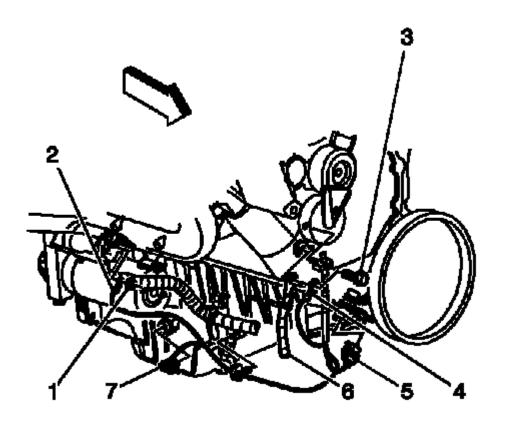
Fig. 319: View Of Oil Level Sensor Electrical Connector, CKP Electrical Connector & Battery Ground Bolt
