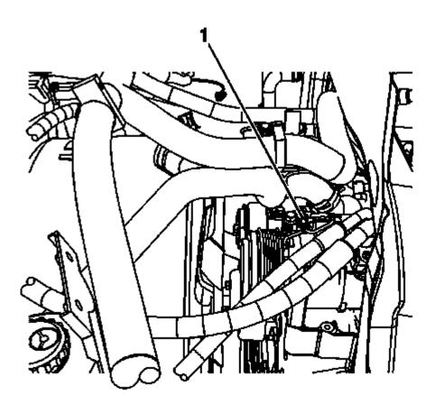
Fig. 315: A/C Compressor Clutch Courtesy of GENERAL MOTORS COMPANY
