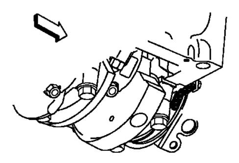
Fig. 248: Applying Adhesive To Sides Of Front Cover To Engine Block Junction At Oil Pan Sealing **Surfaces**
