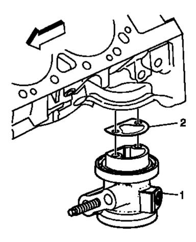
Fig. 377: Identifying Oil Filter Adapter And Oil Filter Adapter Gasket Courtesy of GENERAL MOTORS COMPANY
