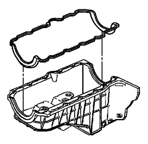
Fig. 250: View Of Oil Pan Gasket Courtesy of GENERAL MOTORS COMPANY
