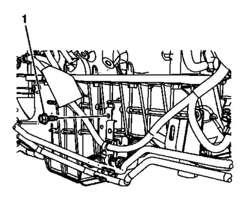
Fig. 241: Transmission Tube Bracket Courtesy of GENERAL MOTORS COMPANY
