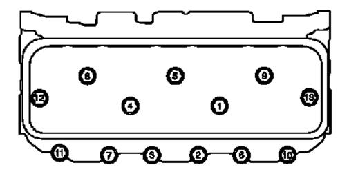
Fig. 144: Identifying Cylinder Head Bolt Tightening Sequence Courtesy of GENERAL MOTORS COMPANY
