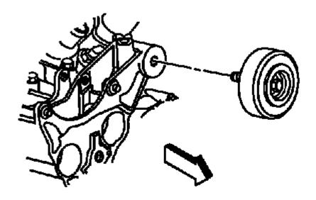
Fig. 15: Drive Belt Right Idler Pulley
