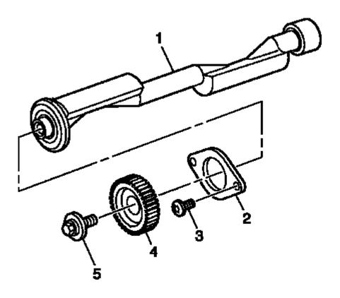
Fig. 495: Balance Shaft Cleaning & Inspection Areas Courtesy of GENERAL MOTORS COMPANY
