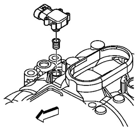
Fig. 51: MAP Sensor Courtesy of GENERAL MOTORS COMPANY
