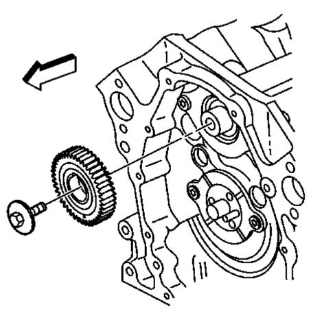
Fig. 206: Locating Balance Shaft Driven Gear Courtesy of GENERAL MOTORS COMPANY
