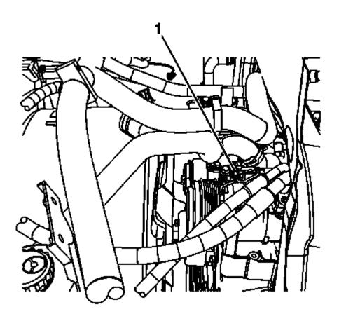
Fig. 302: A/C Compressor Clutch Courtesy of GENERAL MOTORS COMPANY
