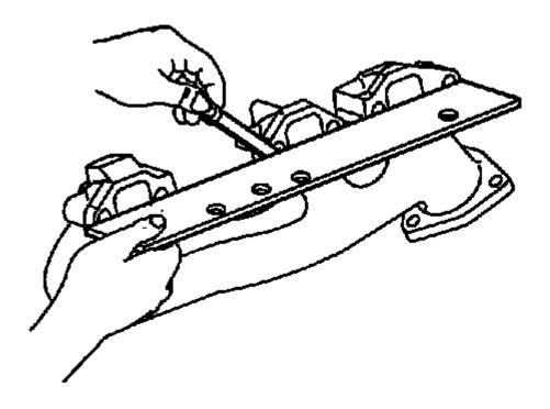
Fig. 567: Measuring Exhaust Manifold Flanges Alignment Courtesy of GENERAL MOTORS COMPANY
