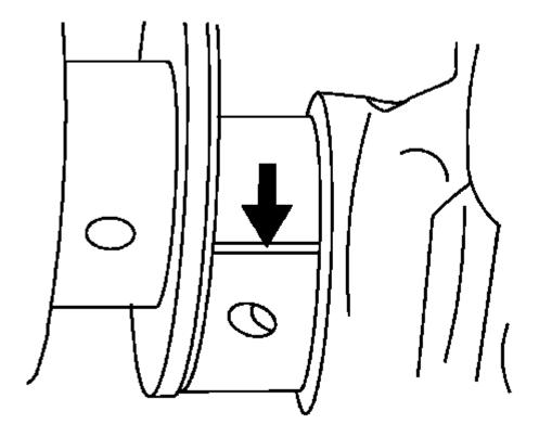
Fig. 475: View Of Plastic Gage Over Crankshaft Journal Courtesy of GENERAL MOTORS COMPANY
