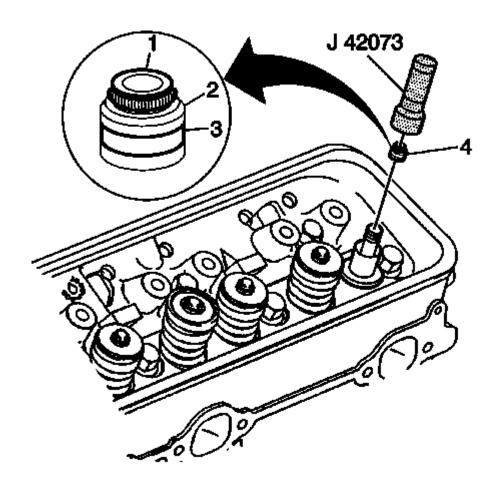
Fig. 519: Exhaust Valve Oil Stem Seal Courtesy of GENERAL MOTORS COMPANY
