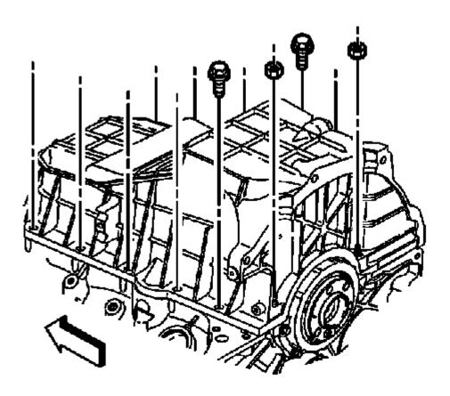
Fig. 379: Locating Oil Pan Bolts & Nuts Courtesy of GENERAL MOTORS COMPANY
