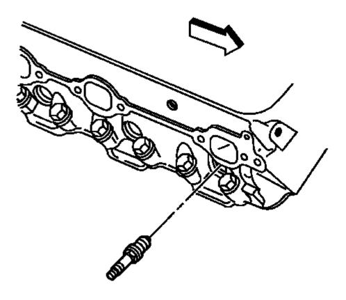
Fig. 367: Locating Spark Plugs Courtesy of GENERAL MOTORS COMPANY
