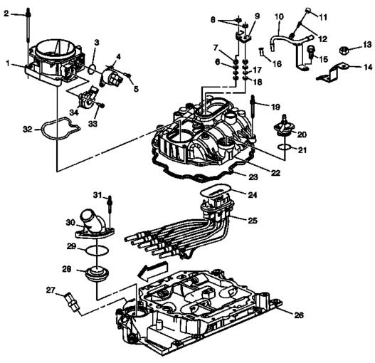
Fig. 1: Upper and Lower Intake Manifold View Courtesy of GENERAL MOTORS COMPANY
