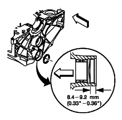
Fig. 575: Installing Expansion Cup Plug Into Balance Shaft Rear Bearing Bole Courtesy of GENERAL MOTORS COMPANY
