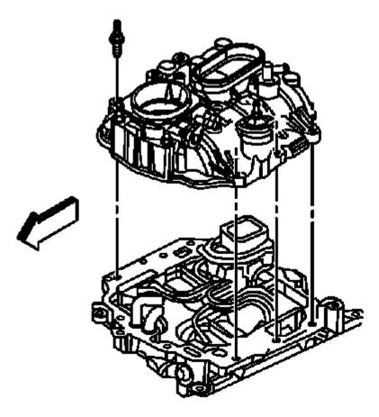
Fig. 57: Upper Intake Manifold Courtesy of GENERAL MOTORS COMPANY
