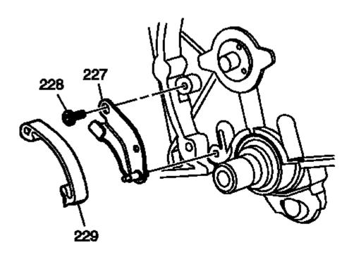
Fig. 621: View Of Timing Chain Tensioner Bracket, Bolt & Shoe Courtesy of GENERAL MOTORS COMPANY
