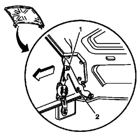
Fig. 317: Identifying Hood Hinge Normal And Service Position Bolt Holes Courtesy of GENERAL MOTORS COMPANY
