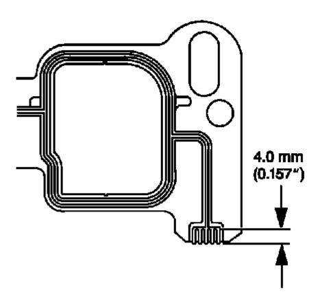
Fig. 669: Applying Patch Of Adhesive To Cylinder Head Side Of Intake Manifold Gasket Courtesy of GENERAL MOTORS COMPANY
