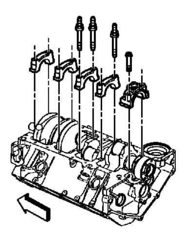
Fig. 455: Bearing Cap Bolts, Cap & Bearing Half Courtesy of GENERAL MOTORS COMPANY
