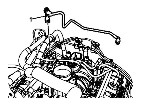
Fig. 59: View Of Tube Quick Connect Fitting Courtesy of GENERAL MOTORS COMPANY
