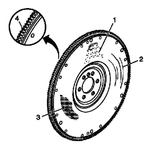
Fig. 484: Flywheel Inspection Areas (Manual Transmission)
