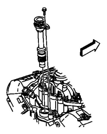
Fig. 676: View Of Oil Pump Drive Shaft
