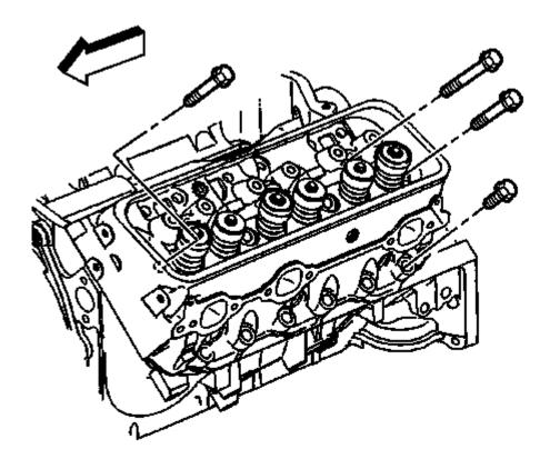
Fig. 363: Locating Cylinder Head Bolts (Left)
