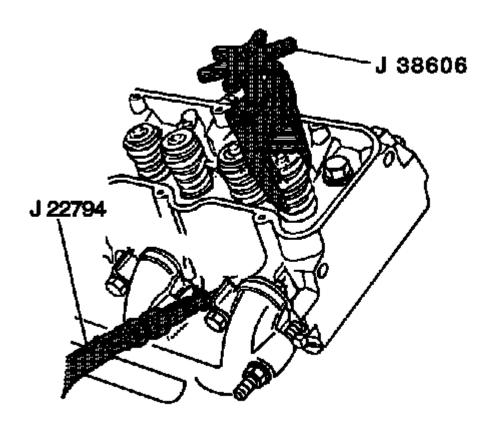
Fig. 123: Using J 38606 & J 5892-D To Remove Valve Spring Courtesy of GENERAL MOTORS COMPANY
