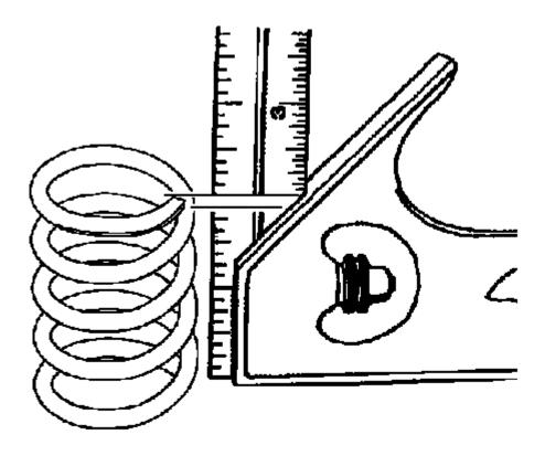
Fig. 512: Inspecting Valve Spring For Squareness Courtesy of GENERAL MOTORS COMPANY
