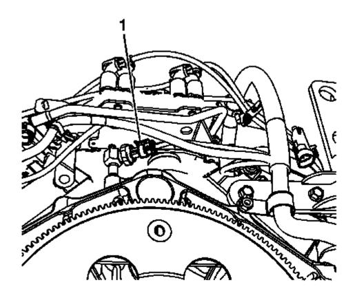
Fig. 85: View Of Oil Pressure Sensor Electrical Connector Courtesy of GENERAL MOTORS COMPANY
