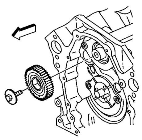
Fig. 610: Locating Balance Shaft Driven Gear Courtesy of GENERAL MOTORS COMPANY
