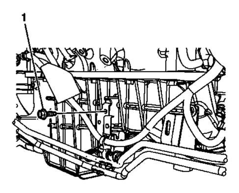
Fig. 259: Transmission Tube Bracket
