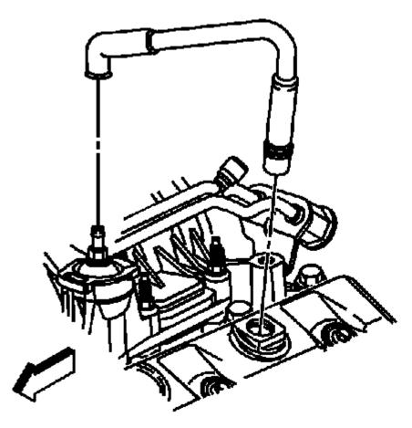
Fig. 82: Locating PCV Valve Hose At Valve & Rocker Cover Courtesy of GENERAL MOTORS COMPANY
