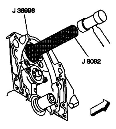
Fig. 209: Installing Balance Shaft
