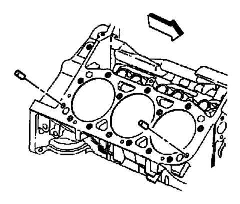
Fig. 372: Cylinder Head Locator Pins Courtesy of GENERAL MOTORS COMPANY
