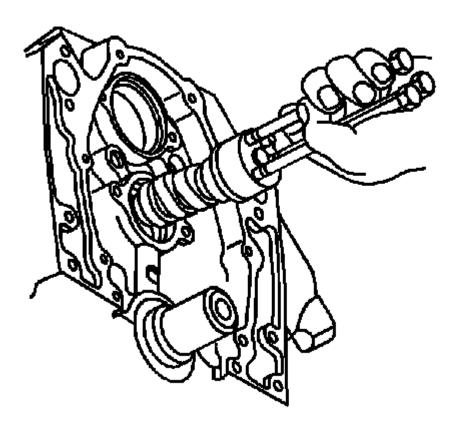
Fig. 221: Using Bolts To Handle Camshaft
