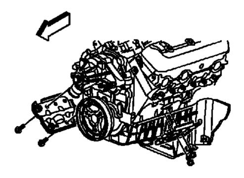
Fig. 34: Engine Mount Adapter Mounting Bolts Courtesy of GENERAL MOTORS COMPANY
