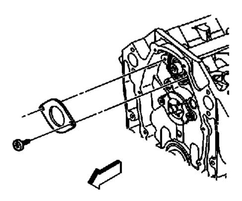
Fig. 398: View of Balance Shaft Retainer & Bolts Courtesy of GENERAL MOTORS COMPANY
