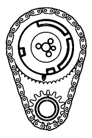
Fig. 498: View Of Sprockets & Chain Courtesy of GENERAL MOTORS COMPANY
