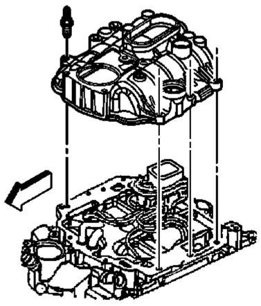
Fig. 556: Identifying Upper Intake Manifold Attaching Studs Courtesy of GENERAL MOTORS COMPANY
