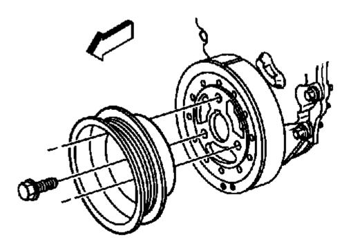
Fig. 171: View Of Crankshaft Pulley & Bolts
