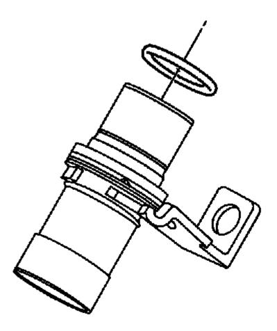
Fig. 625: View Of Crankshaft Position Sensor Seal O-Ring Courtesy of GENERAL MOTORS COMPANY
