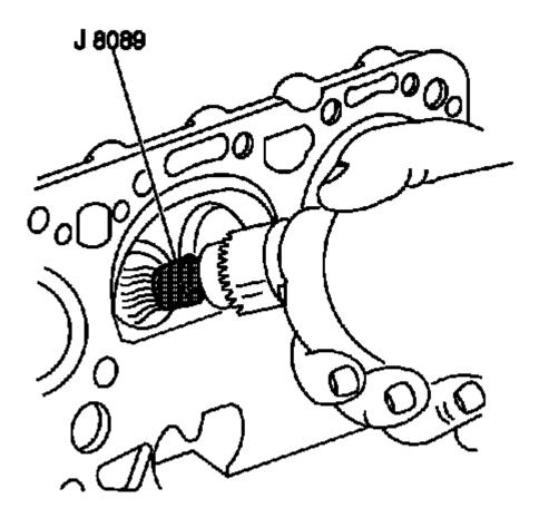
Fig. 509: Cleaning Carbon Using J 8089
