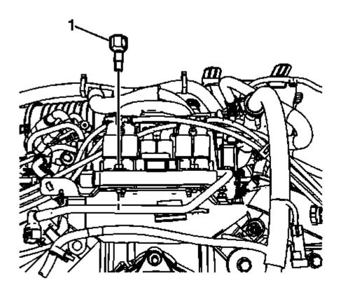
Fig. 267: Oil Pressure Sensor Fitting Courtesy of GENERAL MOTORS COMPANY
