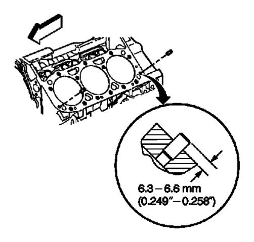
Fig. 140: Installing Cylinder Head Locator Pins Courtesy of GENERAL MOTORS COMPANY
