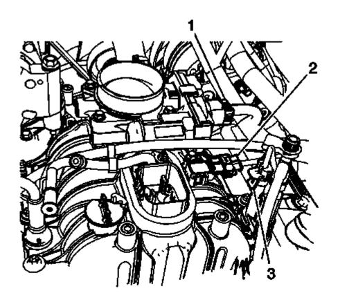
Fig. 88: View Of Throttle Body Actuator, Manifold Absolute Pressure (MAP) Sensor & Evaporative Emission (EVAP) Canister Purge Solenoid Valve Courtesy of GENERAL MOTORS COMPANY
