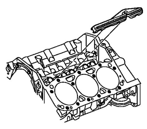
Fig. 373: View Of Valve Lifter Pushrod Guides Courtesy of GENERAL MOTORS COMPANY
