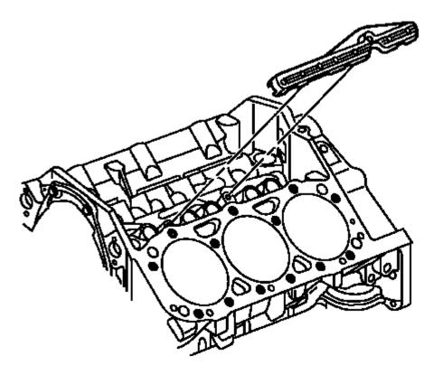
Fig. 125: View Of Valve Lifter Pushrod Guides Courtesy of GENERAL MOTORS COMPANY
