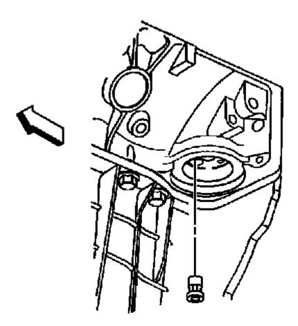
Fig. 233: View Of Oil Filter Bypass Valve Courtesy of GENERAL MOTORS COMPANY
