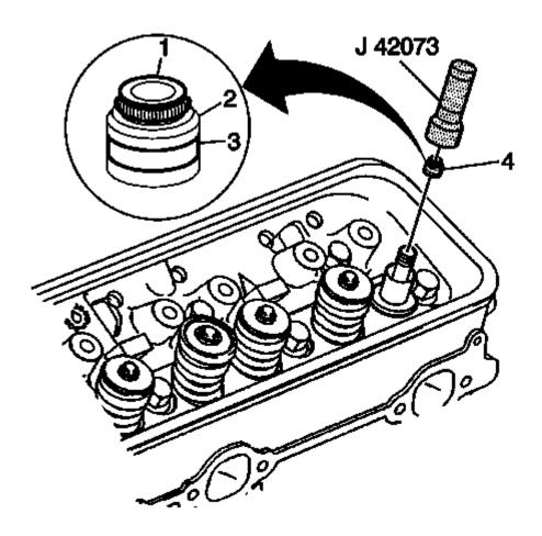
Fig. 119: Exhaust Valve Oil Stem Seal Courtesy of GENERAL MOTORS COMPANY
