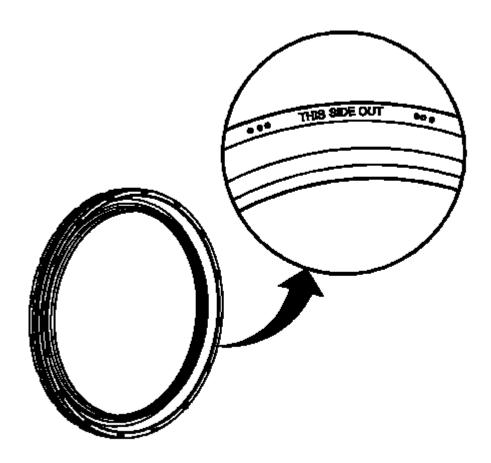
Fig. 286: Identifying Crankshaft Rear Oil Seal Courtesy of GENERAL MOTORS COMPANY
