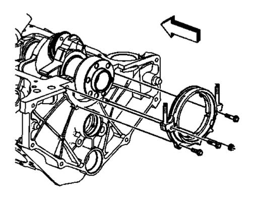
Fig. 594: View Of Crankshaft Rear Oil Housing Courtesy of GENERAL MOTORS COMPANY
