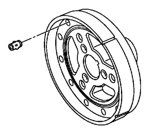
Fig. 640: View Of Crankshaft Balancer Weights Courtesy of GENERAL MOTORS COMPANY
