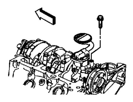
Fig. 629: View Of Oil Pump Bolt Courtesy of GENERAL MOTORS COMPANY
