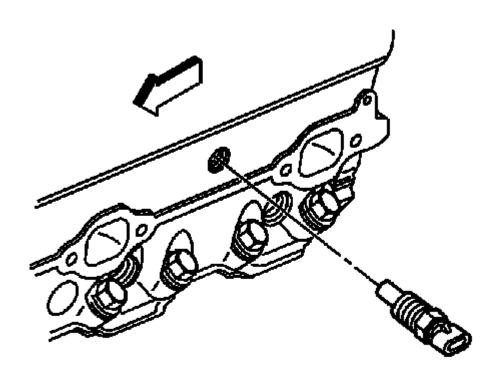
Fig. 134: View Of Engine Coolant Temperature Sensor Courtesy of GENERAL MOTORS COMPANY
