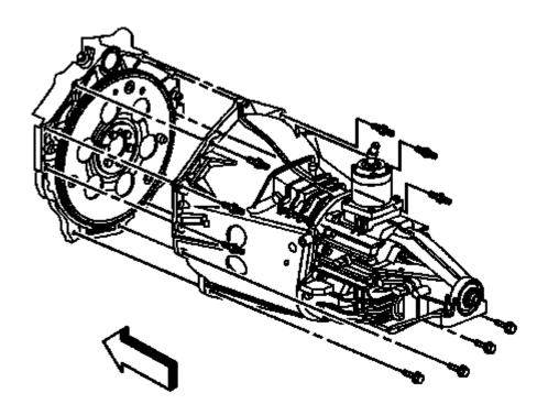
Fig. 255: Manual Transmission Bolts
