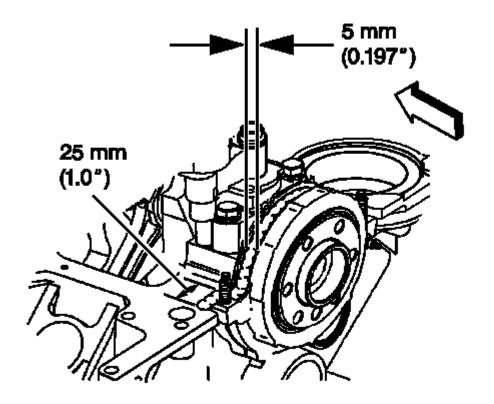
Fig. 249: Applying Adhesive To Entire Length Of Rear Oil Seal Housing To Engine Block Junction At Oil Pan Sealing Surfaces
