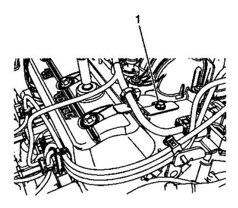
Fig. 91: View Coil Wiring Harness Bracket Nut Courtesy of GENERAL MOTORS COMPANY
