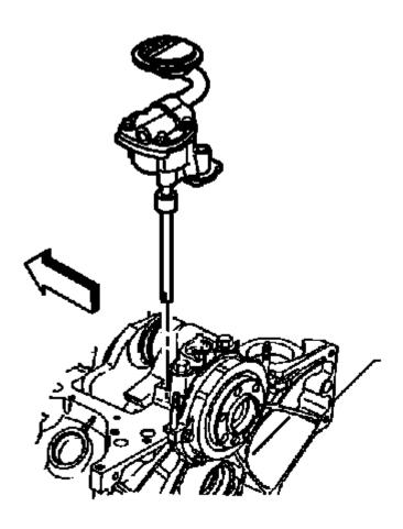
Fig. 383: View Of Oil Pump Courtesy of GENERAL MOTORS COMPANY
