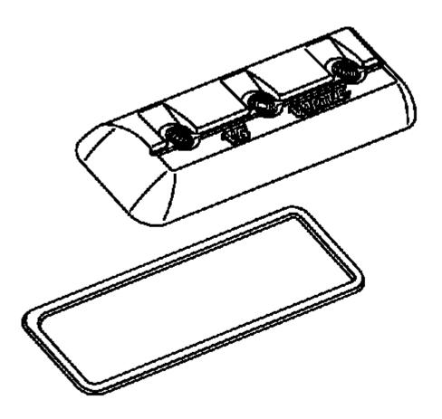
Fig. 682: View Of Rocker Arm Cover And Gasket Courtesy of GENERAL MOTORS COMPANY
