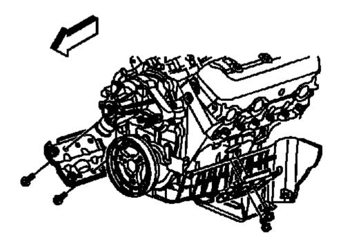
Fig. 35: Engine Mount Adapter Mounting Bolts Courtesy of GENERAL MOTORS COMPANY
