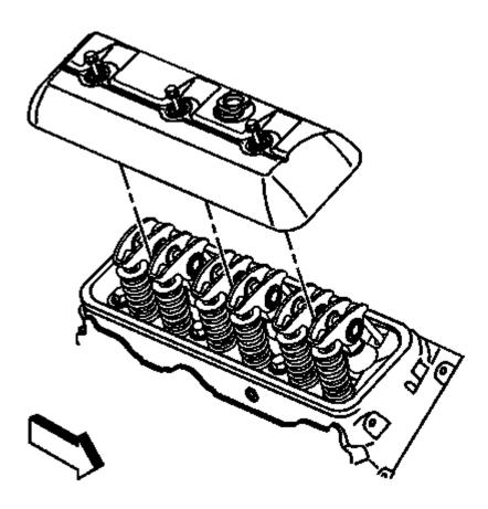
Fig. 102: Rocker Arm Cover Courtesy of GENERAL MOTORS COMPANY
