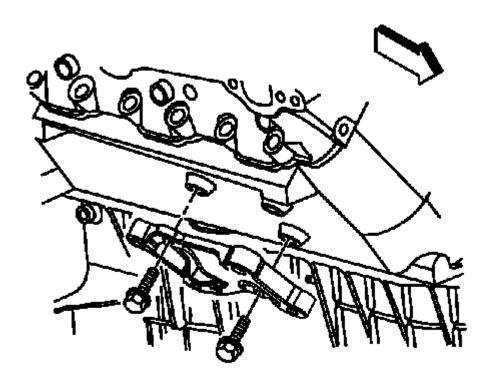
Fig. 31: View Of Right Side (Left Side Similar) Engine Mount Side Bracket & Bolts Courtesy of GENERAL MOTORS COMPANY
