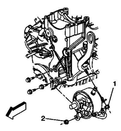
Fig. 130: View Of Power Steering (P/S) Pump Rear Bracket Nut And P/S Pump Rear Bracket Front Nut
