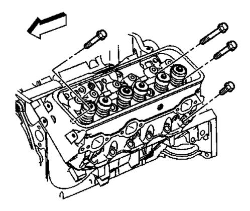
Fig. 651: Locating Cylinder Head Bolts (Left)
