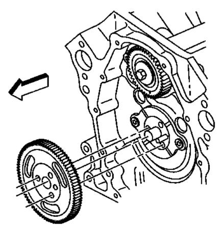
Fig. 205: View Of Balance Shaft Drive Gear **Courtesy of GENERAL MOTORS COMPANY**
