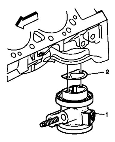
Fig. 228: Identifying Oil Filter Adapter And Oil Filter Adapter Gasket Courtesy of GENERAL MOTORS COMPANY
