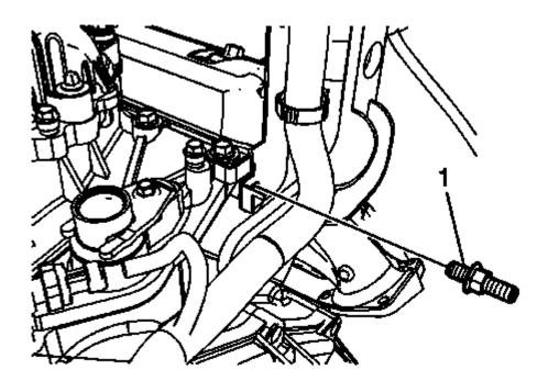
Fig. 83: Engine Wiring Harness Bracket Stud Courtesy of GENERAL MOTORS COMPANY
