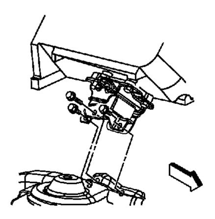
Fig. 33: View Of Right Side (Left Side Similar) Engine Mount To Engine Mount Bracket Bolts Courtesy of GENERAL MOTORS COMPANY
