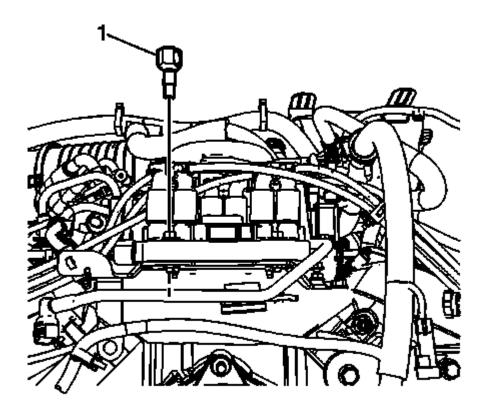
Fig. 268: Oil Pressure Sensor Fitting
