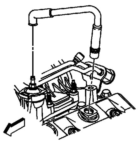
Fig. 41: Locating PCV Valve Hose At Valve & Rocker Cover Courtesy of GENERAL MOTORS COMPANY
