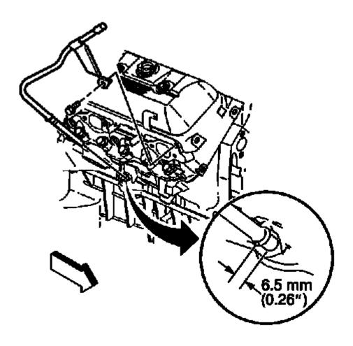
Fig. 685: Applying Sealant & Installing Oil Level Indicator Tube & Bolt Courtesy of GENERAL MOTORS COMPANY
