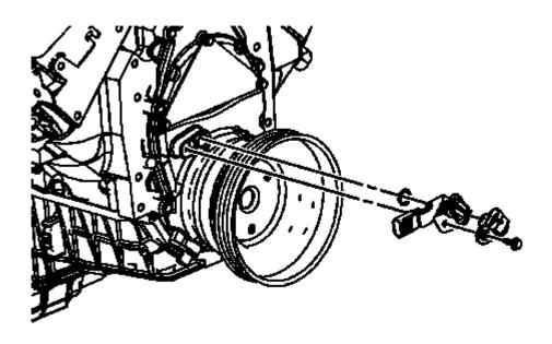
Fig. 181: View Of CMP Sensor & Bolt Courtesy of GENERAL MOTORS COMPANY
