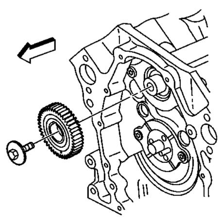
Fig. 211: Locating Balance Shaft Driven Gear Courtesy of GENERAL MOTORS COMPANY
