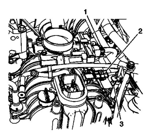
Fig. 64: View Of Throttle Body Actuator, Manifold Absolute Pressure (MAP) Sensor & Evaporative Emission (EVAP) Canister Purge Solenoid Valve Courtesy of GENERAL MOTORS COMPANY
