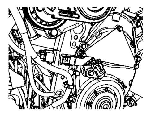
Fig. 185: Camshaft Position (CMP) Sensor Wiring Harness Jumper Courtesy of GENERAL MOTORS COMPANY
