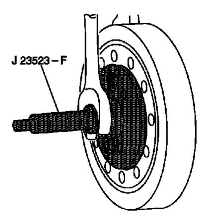
Fig. 642: Installing Crankshaft Balancer Using J 23523-F Courtesy of GENERAL MOTORS COMPANY
