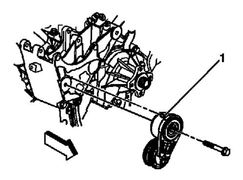
Fig. 14: Drive Belt Tensioner Locating Pin Courtesy of GENERAL MOTORS COMPANY
