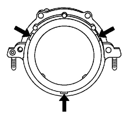
Fig. 284: Crankshaft Rear Oil Seal Notches
