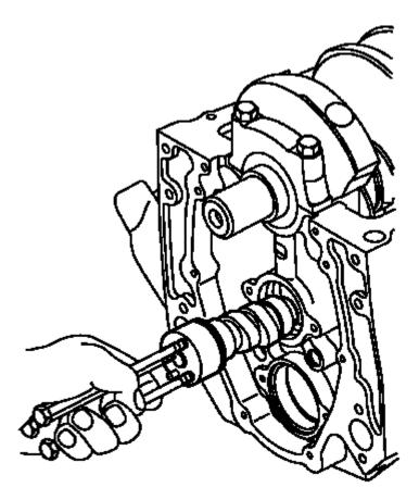
Fig. 401: Handling Camshaft Using Three 5/16-18 X 4.0 Inch Bolts Courtesy of GENERAL MOTORS COMPANY
