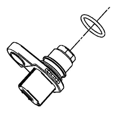
Fig. 186: CKP Sensor O-Ring Seal Courtesy of GENERAL MOTORS COMPANY
