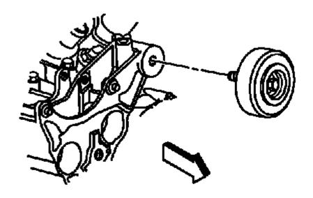
Fig. 16: Drive Belt Right Idler Pulley
