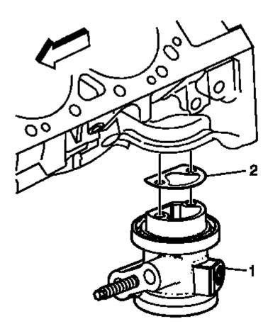
Fig. 638: Identifying Oil Filter Adapter And Oil Filter Adapter Gasket Courtesy of GENERAL MOTORS COMPANY
